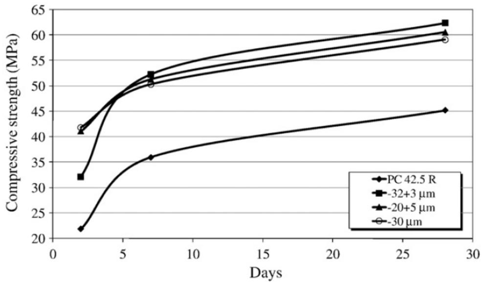
Figure 2.7: Compressive strengths of PC 42.5 R sample with additions of  $-32+3 \mu\text{m}$ ,  $-20+5 \mu\text{m}$  and  $-30 \mu\text{m}$  size fractions [29]
