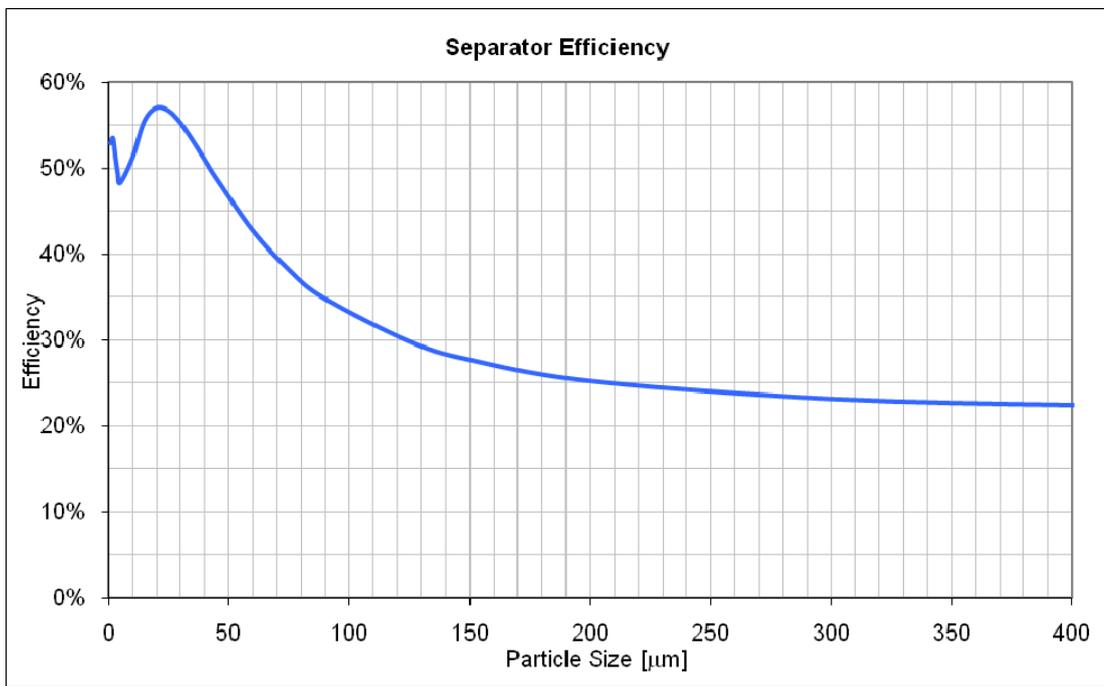
Figure E.4: Separator Performance and Efficiency Curves for Roller Press System (Individual Operation)
