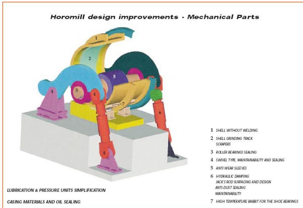
Figure 2.1: Mechanical Parts of HOROMILL® [25]
