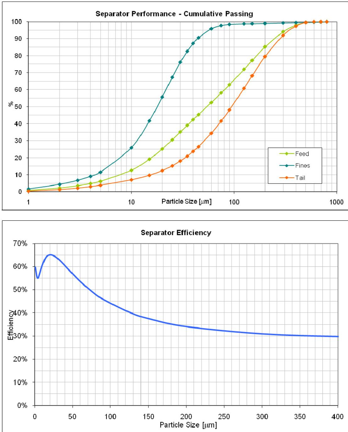
Figure E.1: Separator Performance and Efficiency Curves for COMPLEX® Grinding System
