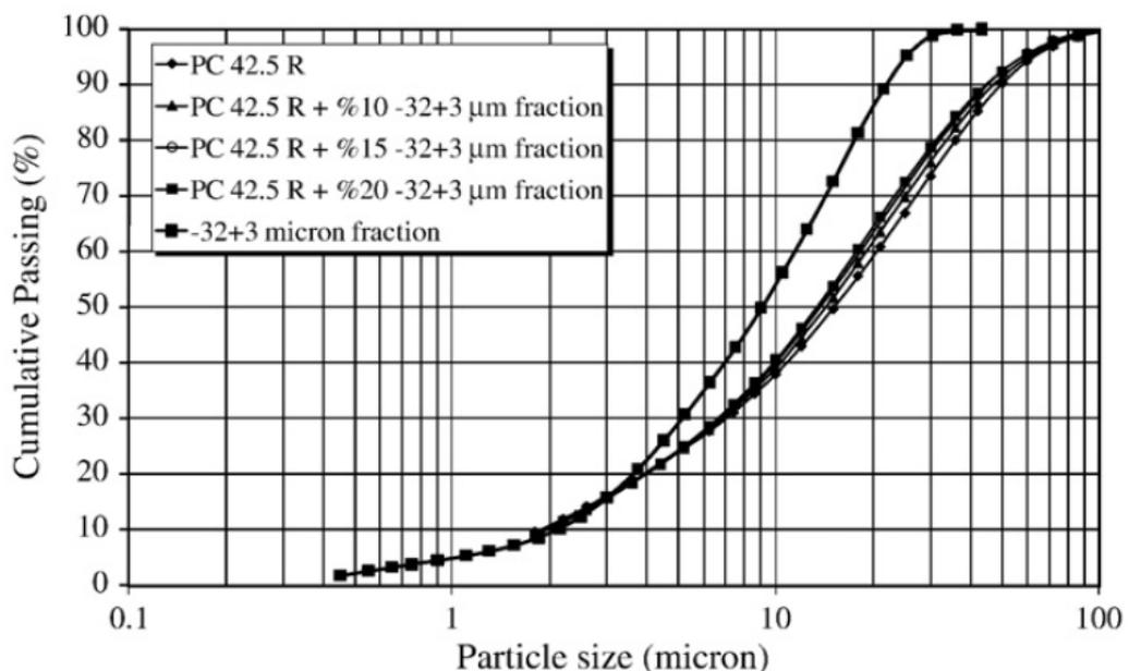
Figure 2.4: Laser particle size distributions of PC 42.5 R samples including varying addition amounts of  $-32+3\ \mu\text{m}$  fraction [29]
