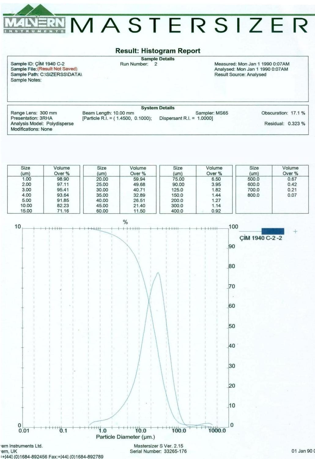
Figure A.1: Particle size analysis of Ball Mill Product in COMFLEX® Grinding System
