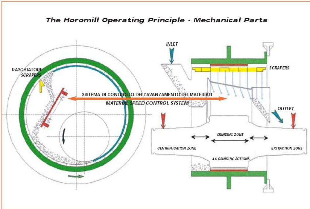
Figure 2.2: Operating Principle of HOROMILL® [25]
