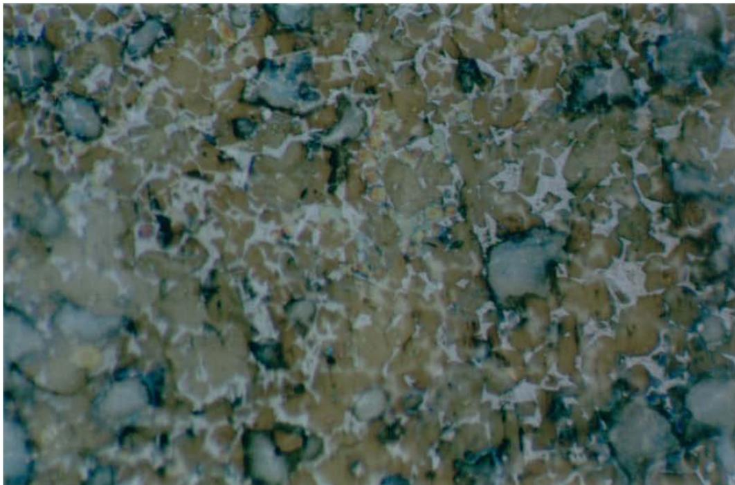
Figure H.2: Alite Crystals with Different Sizes
