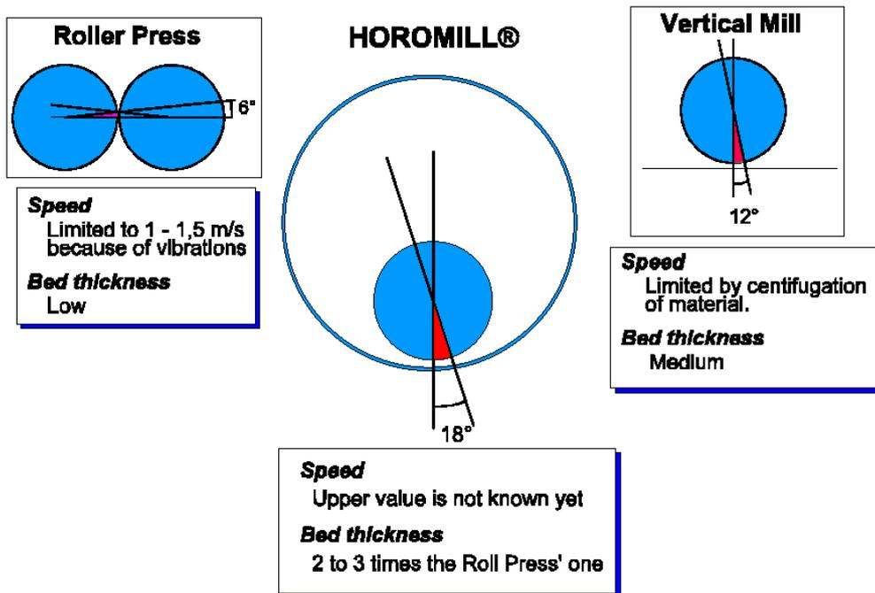
Figure 2.3: Angles of nip at different grinding systems [5]
