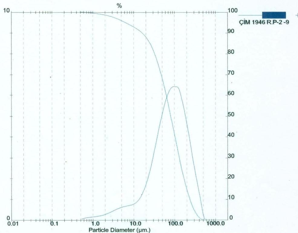
Figure B.4: Particle size analysis of tailings from Roller Press separator (While on individual production)
