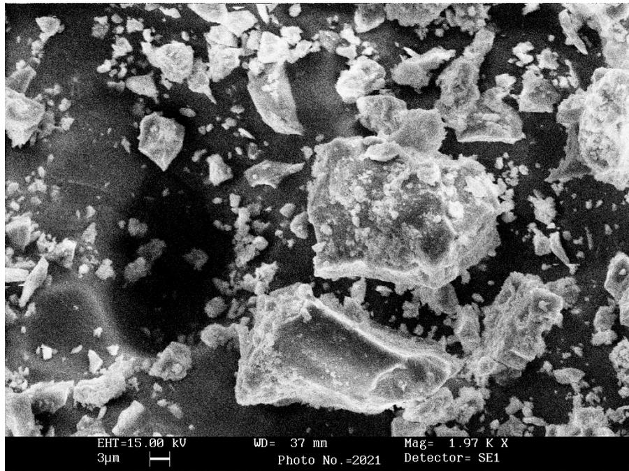
Figure F.4: SEM photographs of Ball Mill Product (Denizli Cement Plant-Cement Mill.1)
