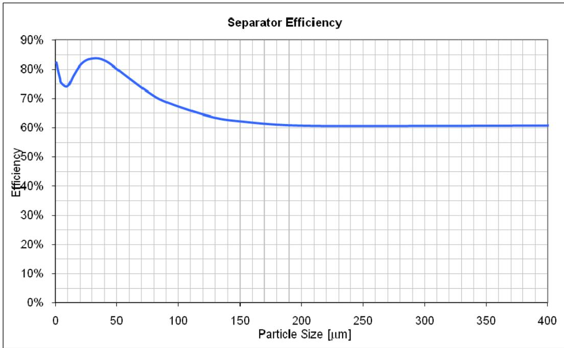
Figure E.2: Separator Performance and Efficiency Curves for Ball Mill Operation in COMPLEX® Grinding System
