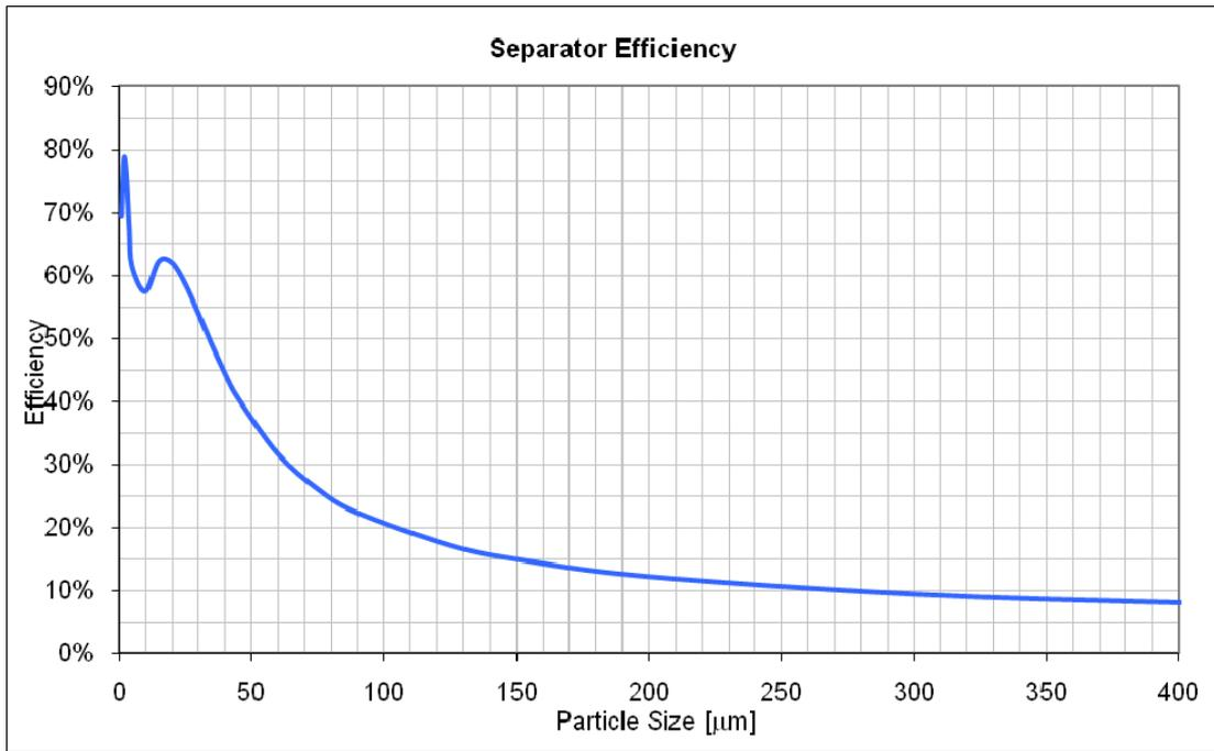
Figure E.3: Separator Performance and Efficiency Curves for Horomill® System
