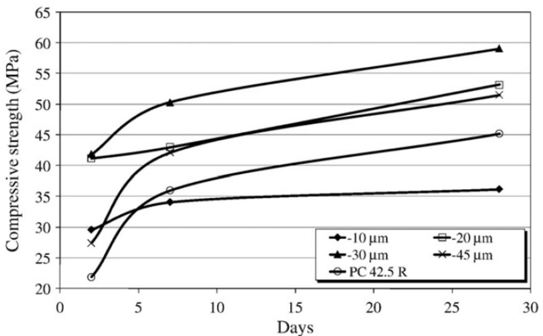
Figure 2.6: Compressive strength values of PC 42.5 R sample and different size fractions of that sample [29]
