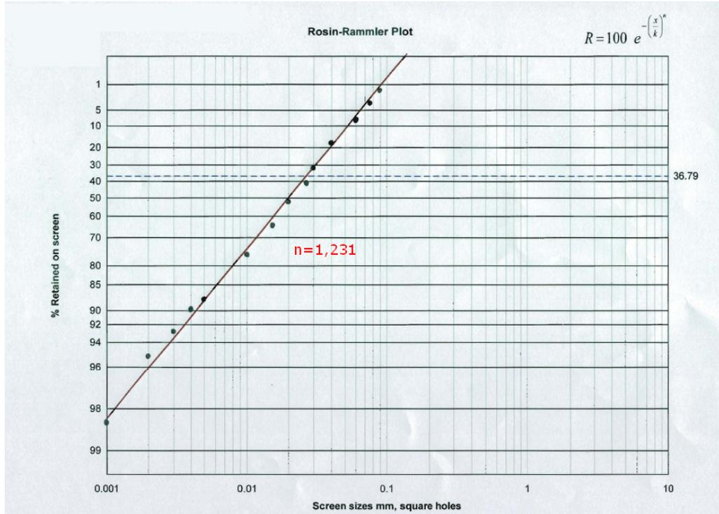
Figure C.1: Rosin-Rammler Distribution Graph of COMPLEX® Grinding System Product
