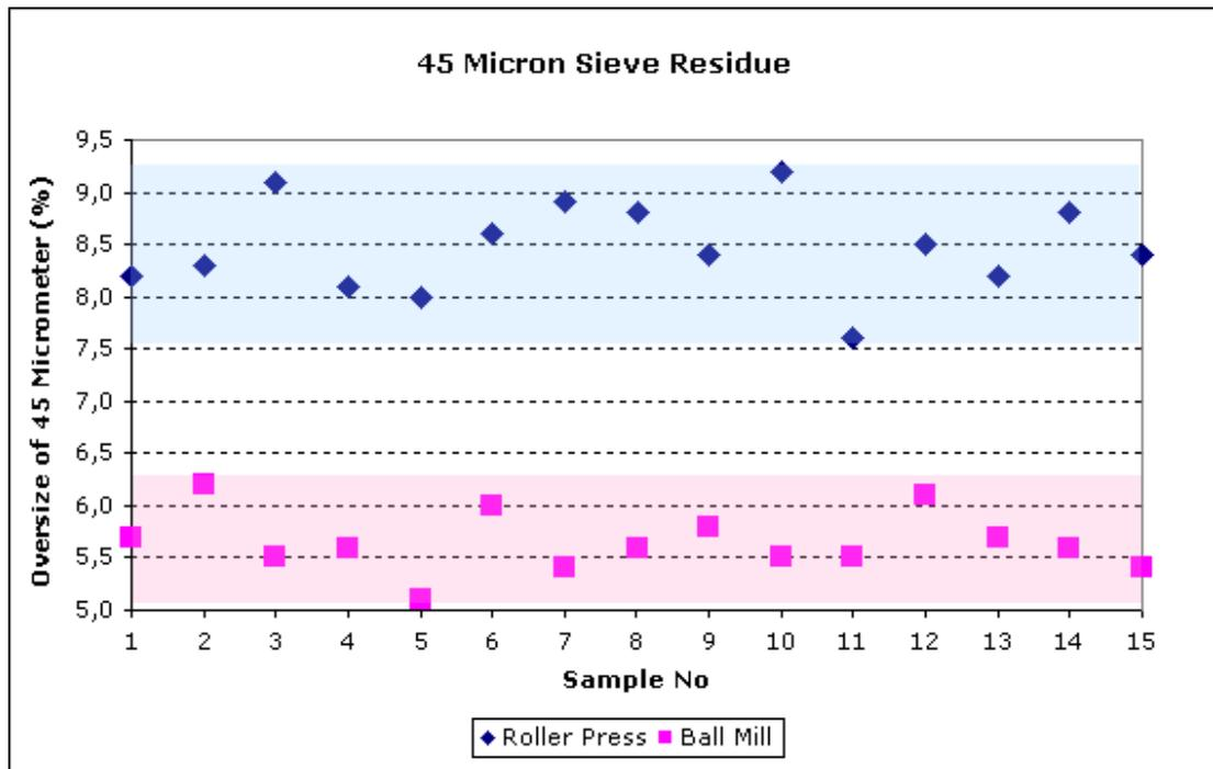
Figure 4.1: Sieve residues of 15 samples from different grinding systems
