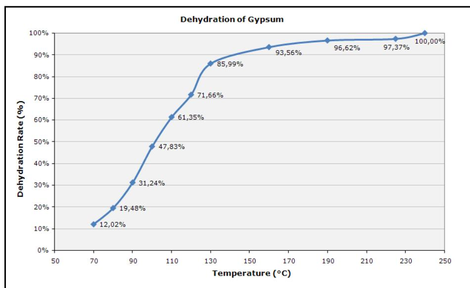
Figure 4.3: Dehydration behavior of the gypsum that was used in the study
