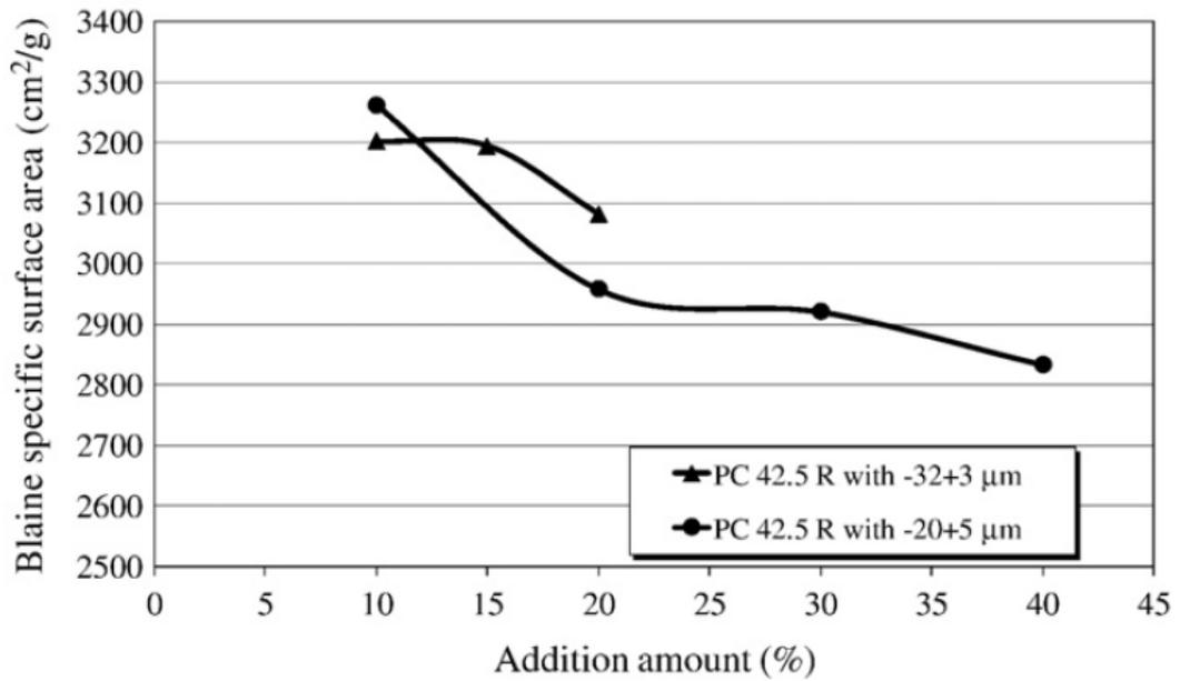
Figure 2.5: Specific surface area values of PC 42.5 R samples with additions of varying -32+3 μm and -20+5 μm fractions [29]
