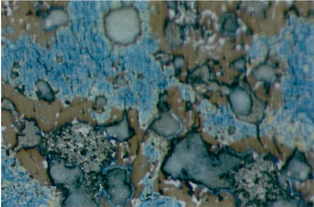
FigureH.3: Coarse Alite Crystals, Free CaO Sets, Ideal Sized Belite Crystals
