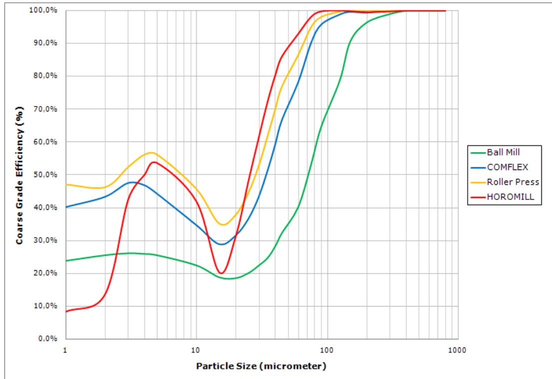
Figure D.1: Tromp Curve for COMPLEX® Grinding System
