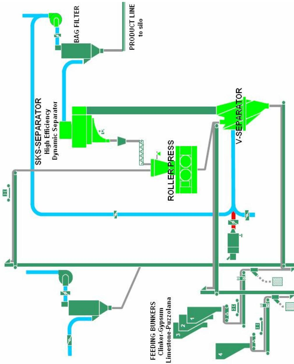
Figure I.3: Simple Flowsheet of Roller Press Grinding System
