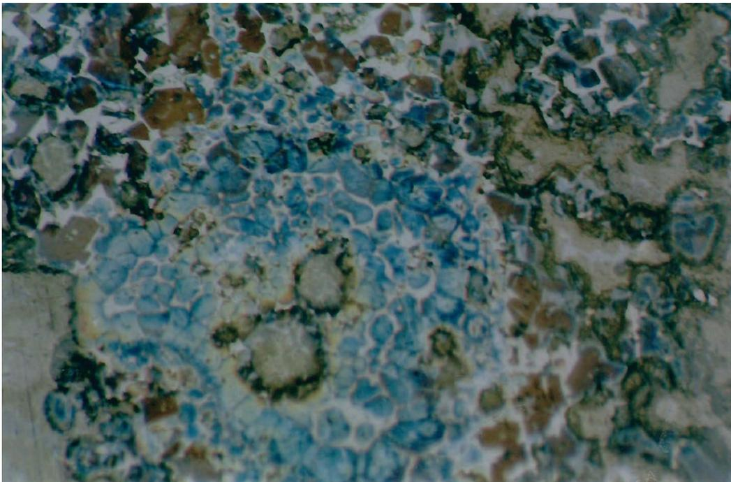
Figure H.4: Coarse Belite Crystals with Irregular Shapes
