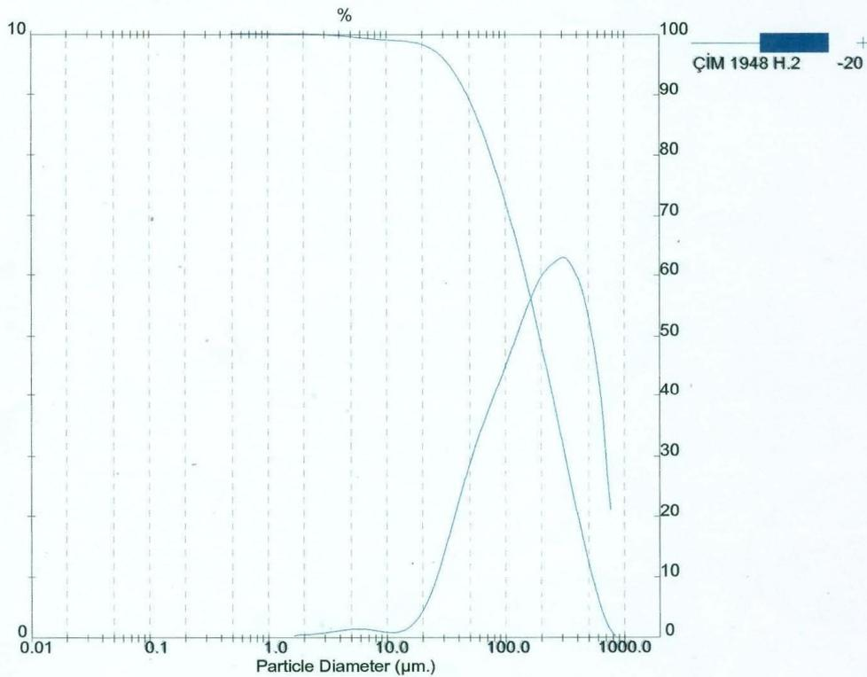
Figure B.3: Particle size analysis of tailings from Horomill® separator
