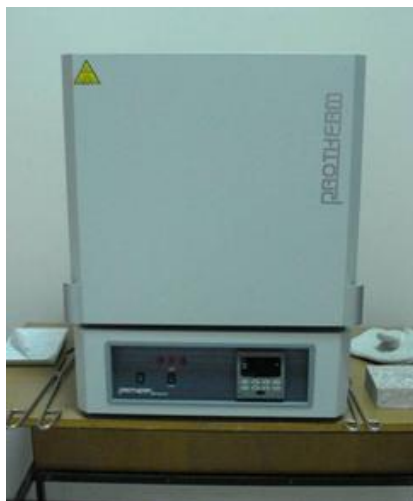
Figure 3.6 Box furnace used in heat treatment of precursors.
