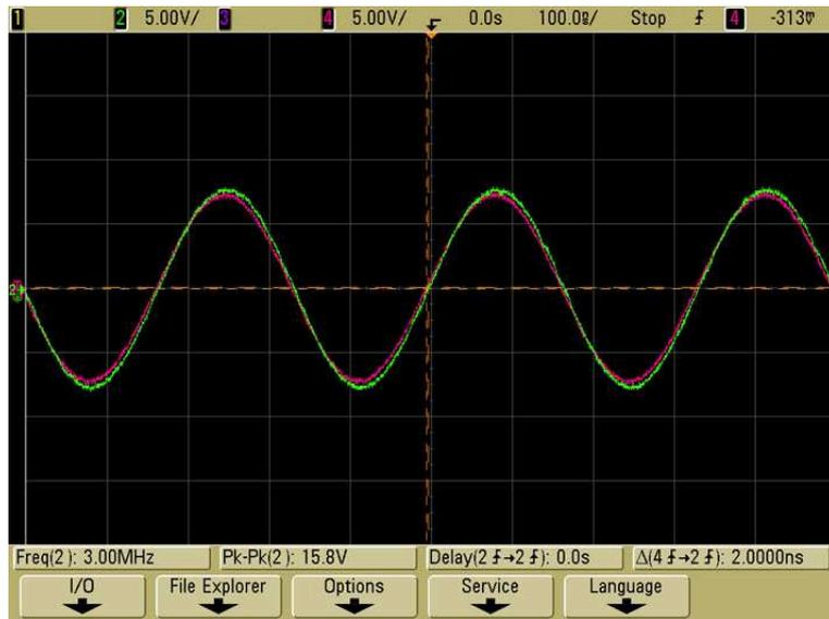
Figure 5.10: Test result for phase shifter circuit ( $R_V = 4 \Omega$ )
