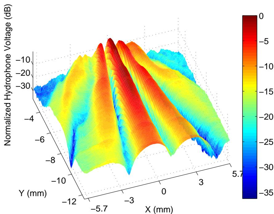
Figure 6.9: The view of the two dimensional focusing point captured with 0.1 mm resolution. Focusing point measured at  $Y=5.81 \text{ mm}$ . ( $f=3 \text{ MHz}$ ,  $V_{p-p}=10 \text{ V}$ , 10 cycles sinusoidal signal)
