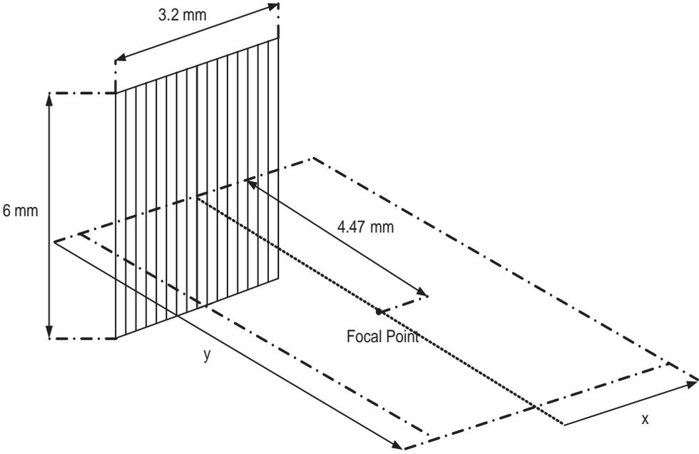
Figure 6.4: Schematic view of X-Y plane that was used to obtain the coordinates of focal point
