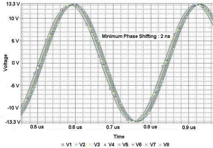
Figure 5.6: Simulation result of phase shifter circuit with minimum  $R_v$  value ( $R_v=4 \Omega$ )
