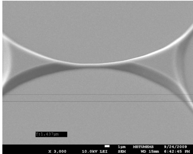
Figure 4.15: SEM image of remaining oxide layer between two membrane cavities
