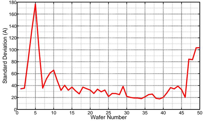
Figure 4.6: Standard thickness deviation of 12000 Å thermal oxidation process
