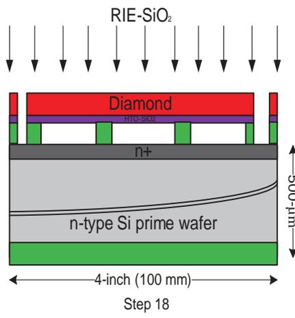
Figure 4.41: Process steps 16 to 18, Step 16 : Bonded wafers: SiO<sub>2</sub> etching with RIE, Step 17 : Bonded wafers: Diamond etching with RIE and photoresist stripping, Step 18 : Bonded wafers: SiO<sub>2</sub> etching with RIE
