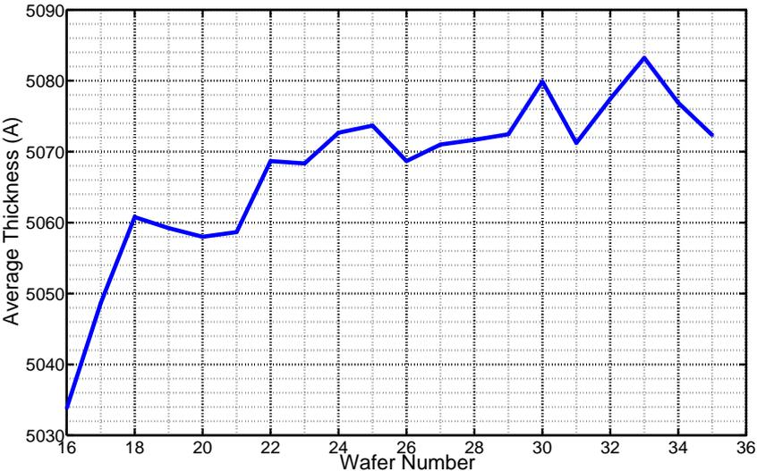
Figure 4.3: Average oxide thickness measurements of 5050 Å thermal oxidation process
