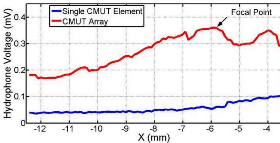
Figure 6.11: The view of the two dimensional focusing point captured with 0.1 mm resolution. (Normalized hydrophone voltages is used ). (  $f=3$  MHz,  $V_{p-p}=10$  V, 10 cycles sinusoidal signal)
