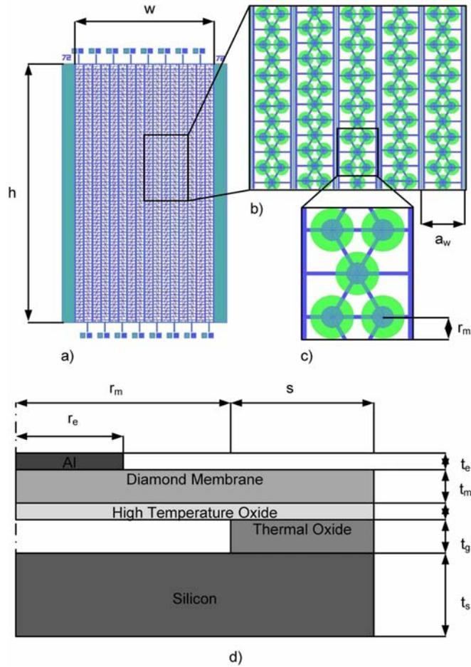
Figure 3.6: Physical dimensions of  $72\ \mu\text{m}$  1-D CMUT array
