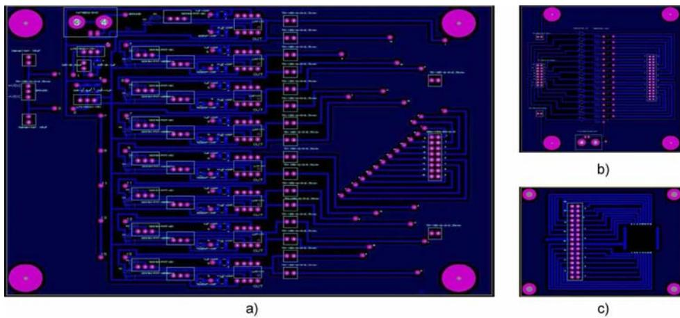
Figure B.1: a)The layout of phase shifter circuit board, b)The layout of T-bias board, c)The layout of the fanout board
