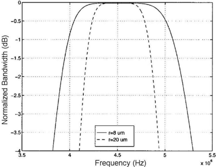
Figure 2.5: The bandwidth comparison of CMUT devices with different membrane radii [43]
