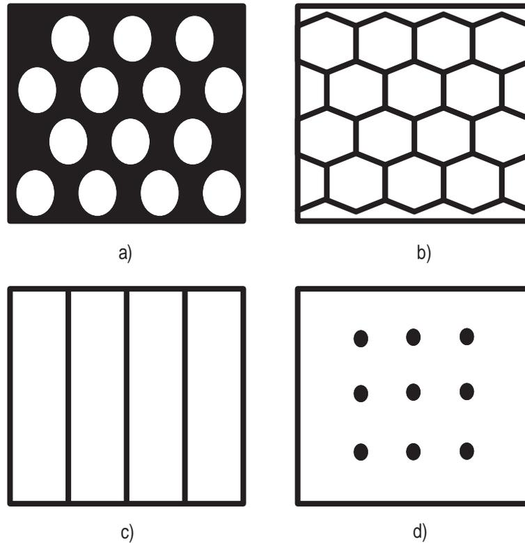
Figure 2.2: a) Circular membranes, b) Hexagon membranes, c) Rectangle membranes, d) Tent membranes [27]
