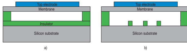
Figure 2.6: a) Conventional CMUT structure, b) PostCMUT structure [46]
