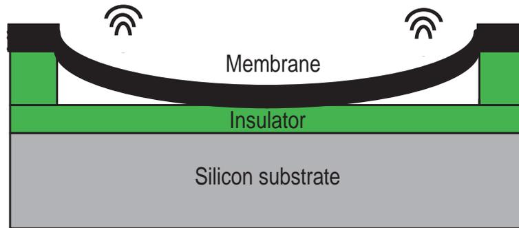
Figure 2.1: Collapse operation regime of CMUT devices [21]
