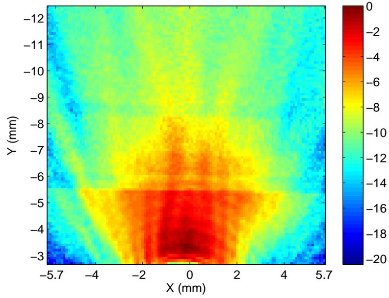
Figure 6.5: Analysis result of the 7<sup>th</sup> element of 1-D CMUT array with 0.1 mm resolution on X-Y plane (  $f=3$  MHz,  $V_{p-p}=10$  V, 10 cycles sinusoidal signal)
