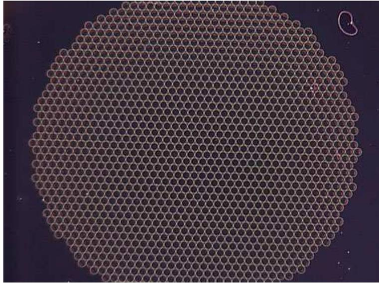
Figure 4.31: The microscope image of robust 120  $\mu\text{m}$  single CMUT
