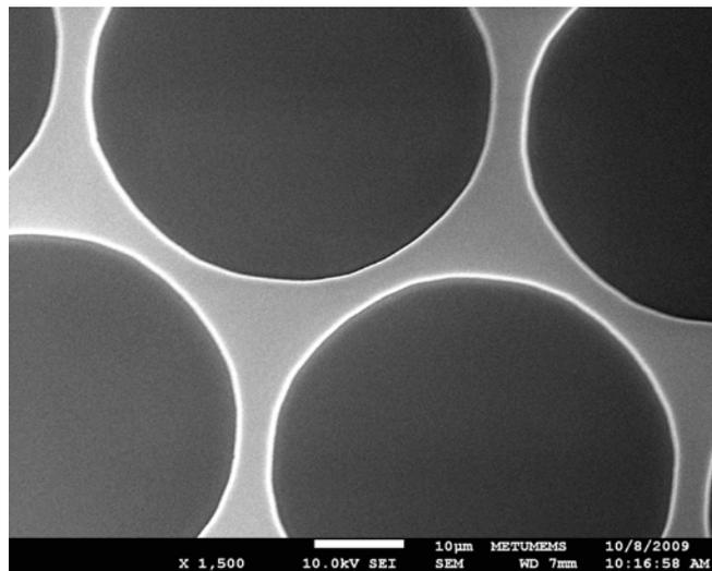
Figure 4.16: SEM image of dry oxide etching with RIE
