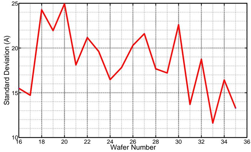
Figure 4.4: Standard thickness deviation of 5050 Å thermal oxidation process
