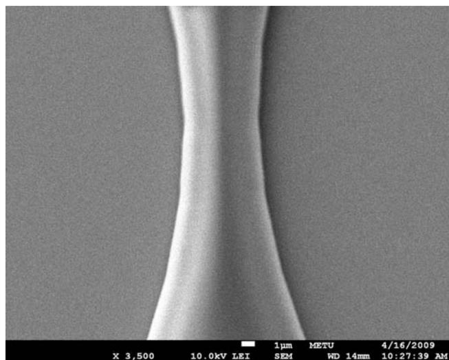
Figure 4.13: SEM image of patterned photoresist material between two adjacent cells
