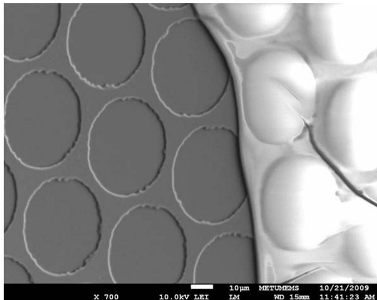
Figure 4.21: SEM image of cracks on CMUT devices with silicon dioxide membrane
