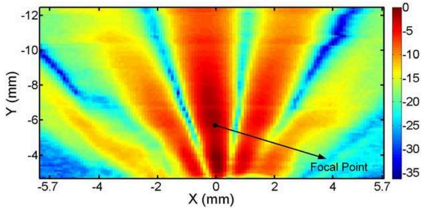
Figure 6.8: 2-D scanning hydrophone results of focusing measurement. It was obtained with 0.1 mm resolution. Focusing point measured at  $Y=5.81$  mm. ( $f=3$  MHz,  $V_{p-p}=10$  V, 10 cycles sinusoidal signal)
