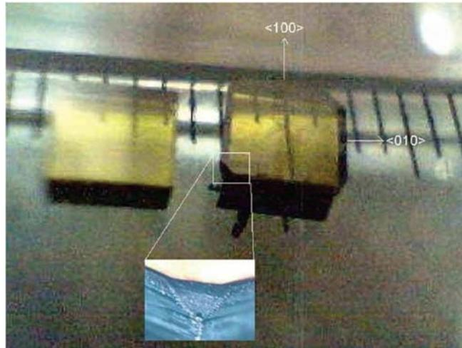
Figure 2.9: Fabricated 7 mm x 8 mm x 5 mm SCD plate [60]
