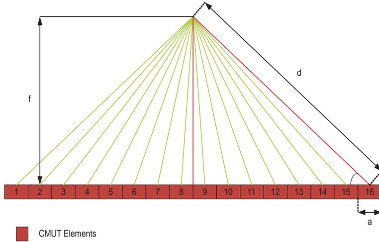
Figure 5.1: The example of the focusing point using 16 elements of 1-D CMUT
