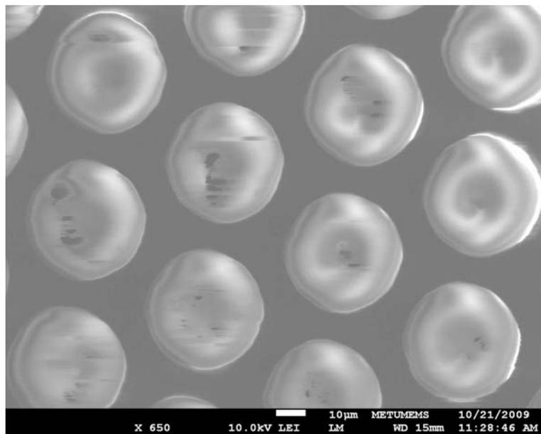
Figure 4.19: SEM image of silicon dioxide membrane CMUT cells
