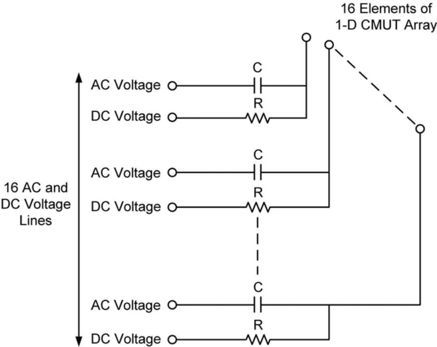
Figure 5.8: The schematic of T-Bias circuit consisting capacitors and resistors
