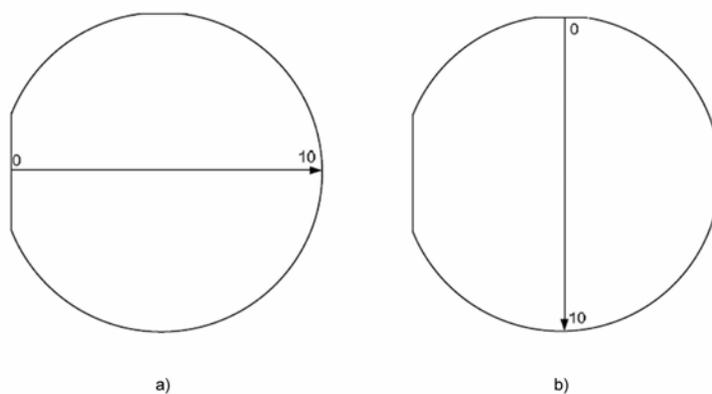
Figure 4.22: a) Left-to-right (LR) thickness scan, b) Top-to-bottom (TB) thickness scan
