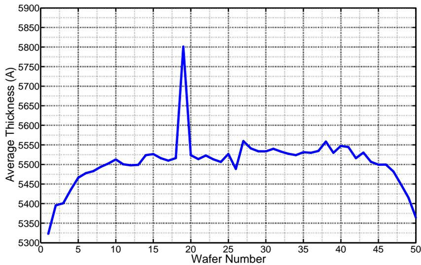
Figure 4.1: Average oxide thickness measurements of 5500 Å thermal oxidation process
