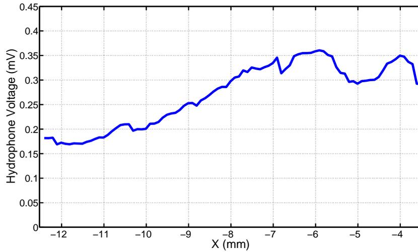
Figure 6.10: The view of the focusing point captured with 0.1 mm resolution along the center axis. (Normalized hydrophone voltages is used ). (  $f=3$  MHz,  $V_{p-p}=10$  V, 10 cycles sinusoidal signal)
