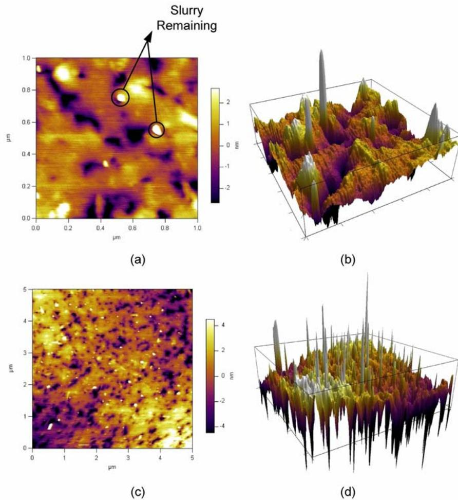
Figure 4.26: a) 2D AFM measurement view of UNCD layer  $1 \mu\text{m} \times 1 \mu\text{m}$ ,  $R_q=1.325 \text{ nm}$ ,  $R_a=0.907 \text{ nm}$ , b) 3D AFM measurement view of UNCD layer  $1 \mu\text{m} \times 1 \mu\text{m}$ , c) 2D AFM measurement view of UNCD layer  $5 \mu\text{m} \times 5 \mu\text{m}$ ,  $R_q=2.227 \text{ nm}$ ,  $R_a=1.641 \text{ nm}$ , d) 3D AFM measurement view of UNCD layer  $5 \mu\text{m} \times 5 \mu\text{m}$
