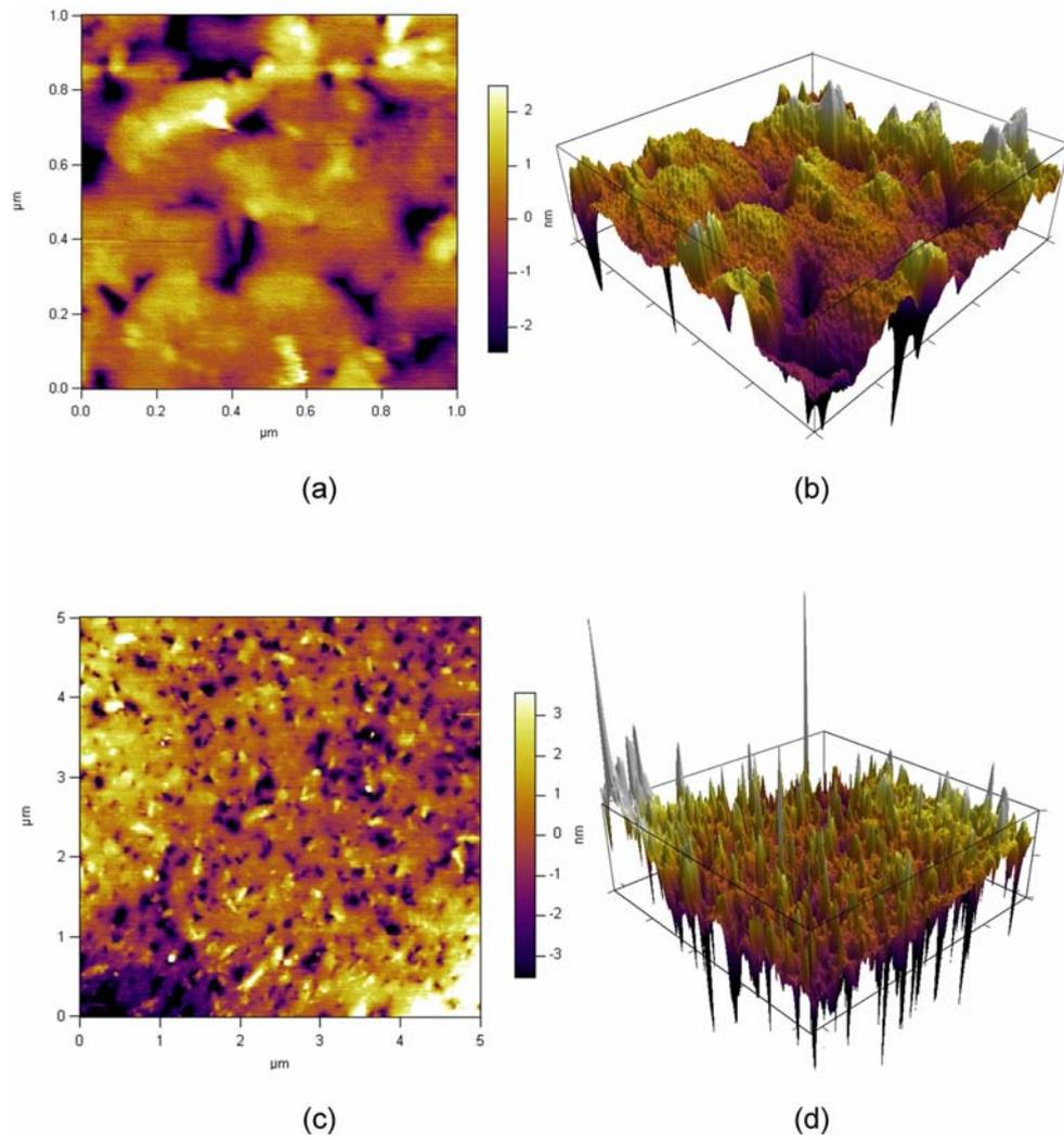
Figure 4.27: a) 2D AFM measurement view of UNCD layer  $1 \mu\text{m} \times 1 \mu\text{m}$ ,  $R_q=1.222 \text{ nm}$ ,  $R_a=0.833 \text{ nm}$ , b) 3D AFM measurement view of UNCD layer  $1 \mu\text{m} \times 1 \mu\text{m}$ , c) 2D AFM measurement view of UNCD layer  $5 \mu\text{m} \times 5 \mu\text{m}$ ,  $R_q=1.757 \text{ nm}$ ,  $R_a=1.231 \text{ nm}$ , d) 3D AFM measurement view of UNCD layer  $5 \mu\text{m} \times 5 \mu\text{m}$
