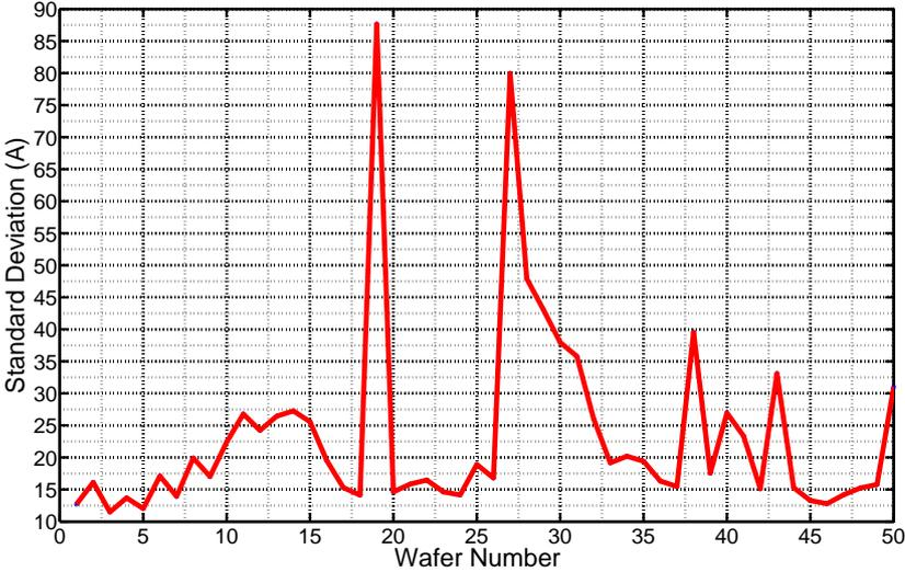
Figure 4.2: Standard thickness deviation of 5500 Å thermal oxidation process
