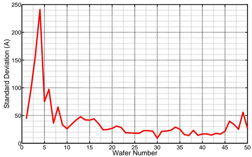
Figure 4.10: Standard thickness deviation of 15000 Å thermal oxidation process
