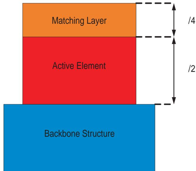
Figure 1.3: Basic structure for piezoelectric transducer [11]
