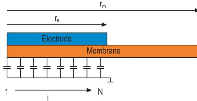
Figure 3.3: Membrane and air gap with small capacitors [66]
