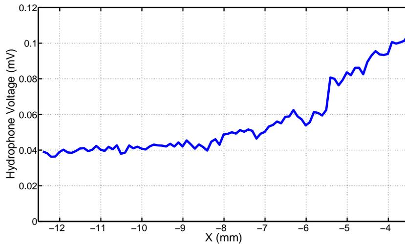
Figure 6.7: Measured voltage distribution of the single element at the axial distance on the normal to the CMUT center plane ( $f=3$  MHz,  $V_{p-p}=10$  V, 10 cycles sinusoidal signal)
