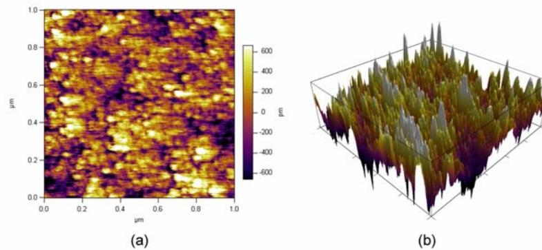
Figure 4.28: a) AFM measurement of PECVD oxide in planar view 1 μm x 1 μm, b) AFM measurement of PECVD oxide in 3D view 1 μm x 1 μm,  $R_q=0.327$  nm,  $R_a=0.255$  nm
