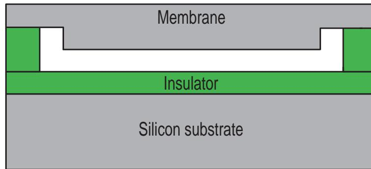
Figure 2.3: The basic structure of piston shape membrane CMUT [28]
