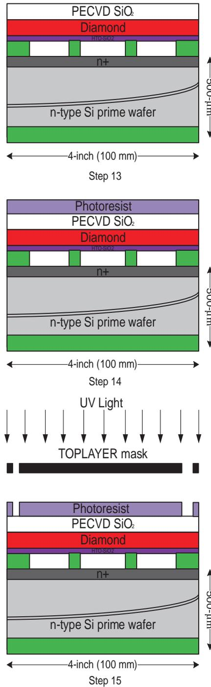
Figure 4.40: Process steps 13 to 15, Step 13 : Bonded wafers: PECVD SiO<sub>2</sub> covering of diamond surface, Step 14 : Bonded wafers: Photoresist covering, Step 15 : Bonded wafers: Photoresist patterning with toplayer mask
