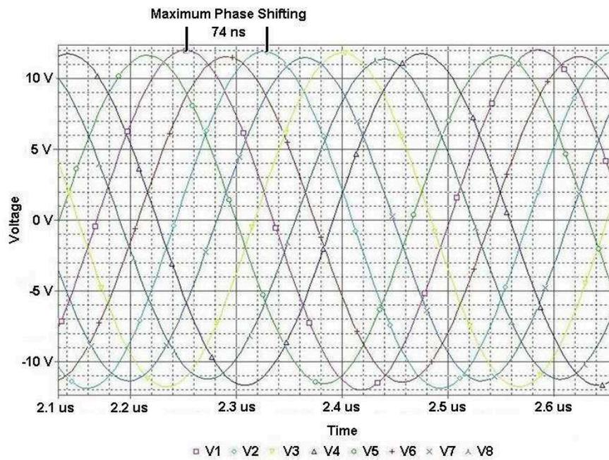
Figure 5.7: Simulation result of phase shifter circuit with maximum  $R_v$  value ( $R_v=200 \Omega$ )
