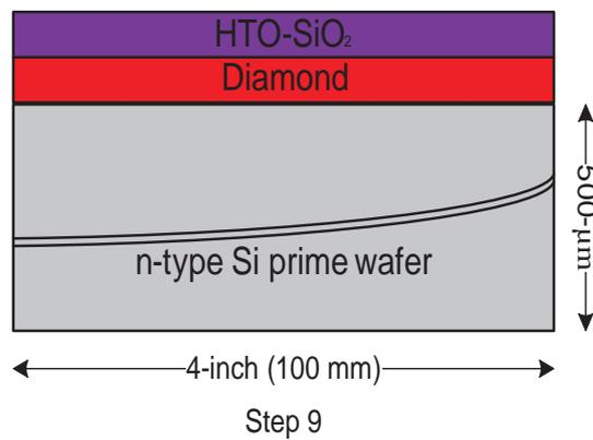
Figure 4.38: Process steps 7 to 9, Step 7 : Bottom wafer: Photoresist stripping with  $O_2$  plasma, Step 8 : Top wafer: Silicon wafer with diamond layer, Step 9 : Top wafer: HTO- $SiO_2$  deposition in LPCVD furnace
