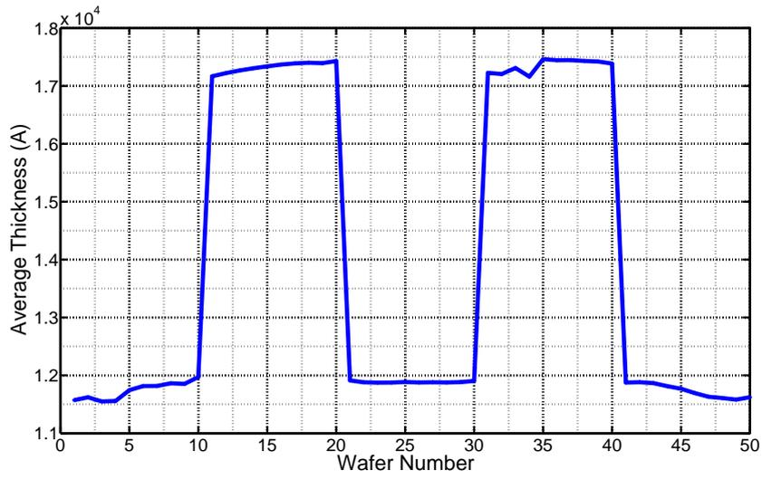
Figure 4.7: Average oxide thickness measurements of 17000 Å thermal oxidation process
