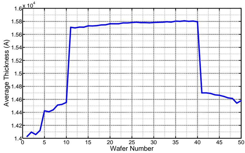
Figure 4.9: Average oxide thickness measurements of 15000 Å thermal oxidation process
