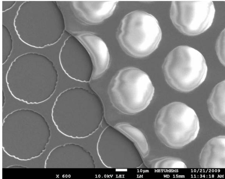
Figure 4.20: SEM image of cracks on CMUT devices with silicon dioxide membrane
