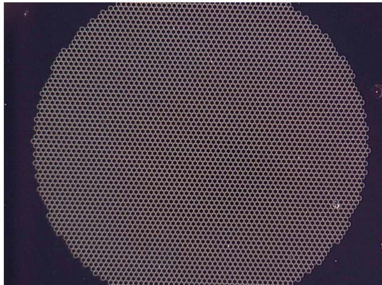
Figure 4.30: The microscope image of robust 72  $\mu\text{m}$  single CMUT
