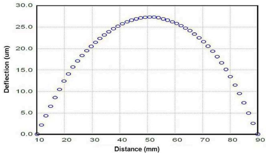
Figure 4.24: Stress and wafer bow measurement of DOI wafer. Wafer bow: 27  $\mu\text{m}$ , Tensile stress: 22 MPa
