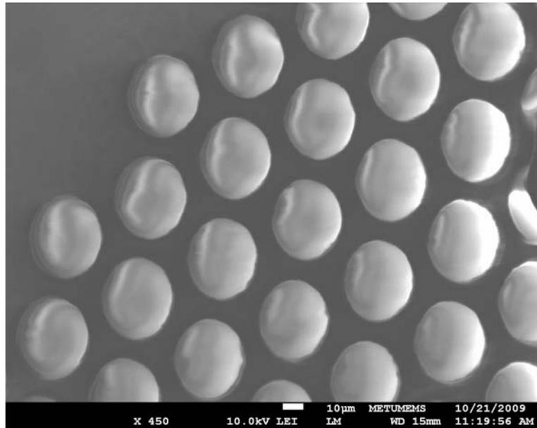
Figure 4.18: SEM image of silicon dioxide membrane CMUT cells
