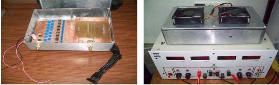
Figure 5.9: Phase shifter and bias T board is packaged in a box
