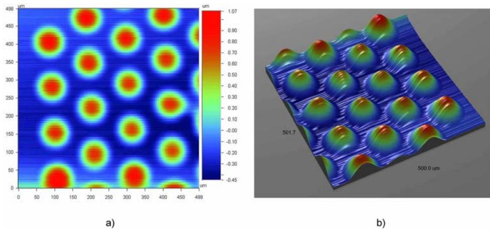
Figure 4.32: a) The planar view of 120  $\mu\text{m}$  single CMUT membranes, b) The 3D Dektak image of 120  $\mu\text{m}$  single CMUT membranes
