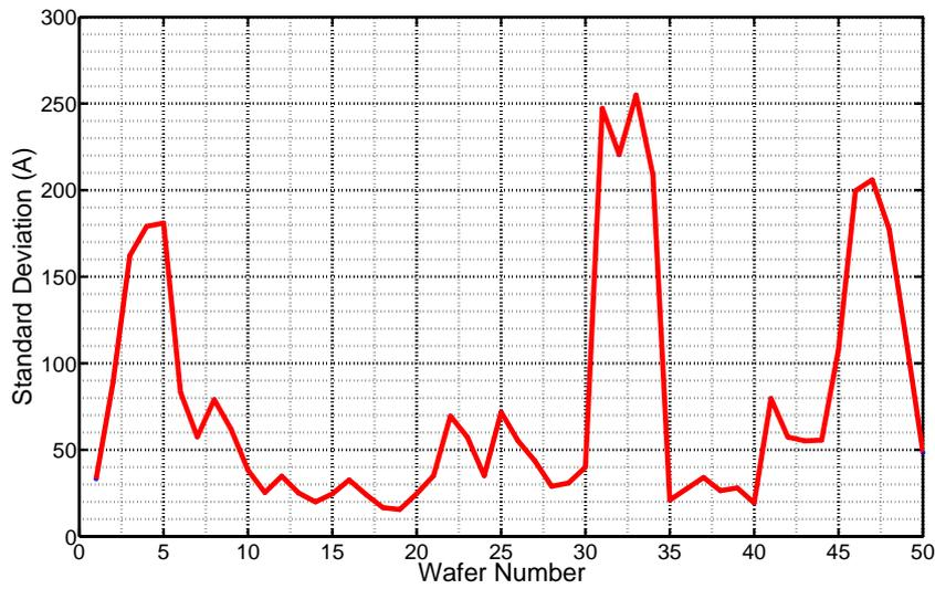
Figure 4.8: Standard thickness deviation of 17000 Å thermal oxidation process
