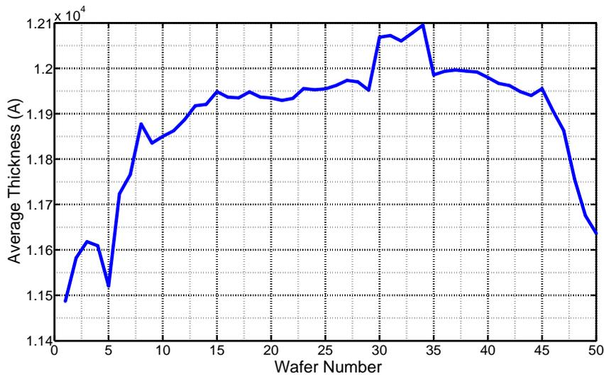
Figure 4.5: Average oxide thickness measurements of 12000 Å thermal oxidation process
