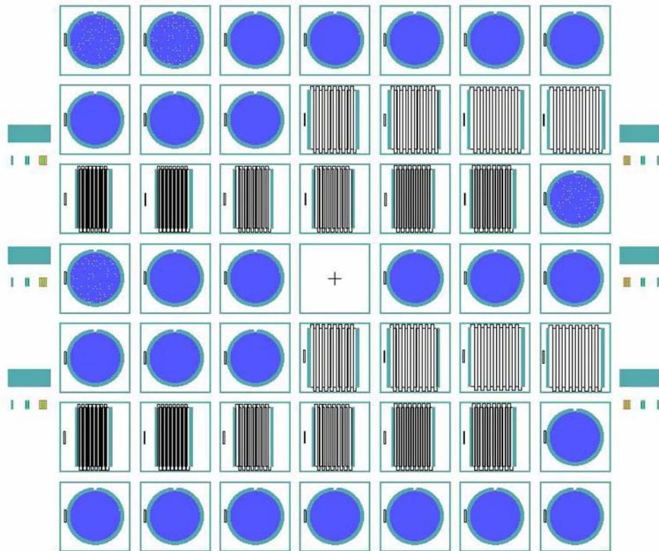
Figure 3.7: Floor planning of 1-D CMUT arrays and single CMUT designs
