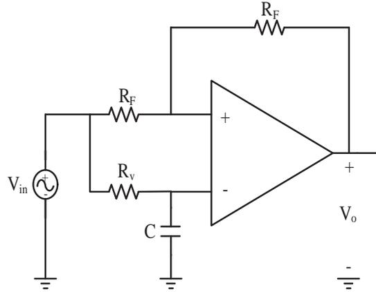
Figure 5.3: Basic block of phase shifter electronics
