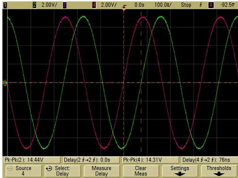
Figure 5.11: Test result for phase shifter circuit ( $R_V = 200 \Omega$ )
