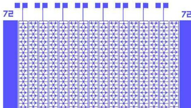
Figure 4.35: Metal mask of 1-D CMUT array with  $72\ \mu\text{m}$
