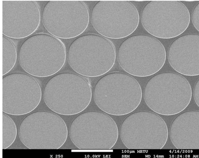
Figure 4.12: SEM image of the patterned photoresist material
