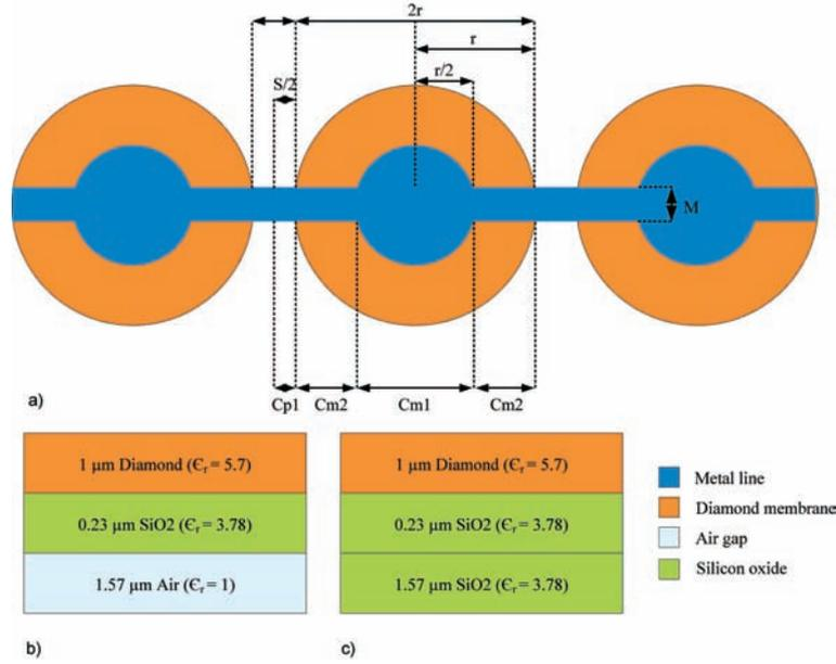
Figure 3.8: a) The physical variables of CMUT cell dimensions, b) Physical structure under the membrane, c) Physical structure under the metal lines where there is no air gap
