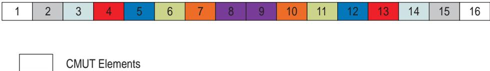
Figure 5.4: Same colored elements are excited with the same phase signals
