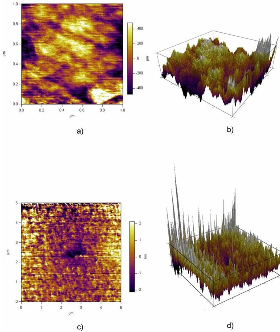
Figure 4.33: a) 2D AFM measurement view of polished HTO layer  $1 \mu\text{m} \times 1 \mu\text{m}$ , b) 3D AFM measurement view of polished HTO layer  $1 \mu\text{m} \times 1 \mu\text{m}$ , c) 2D AFM measurement view of polished HTO layer  $5 \mu\text{m} \times 5 \mu\text{m}$ , d) 3D AFM measurement view of polished HTO layer  $5 \mu\text{m} \times 5 \mu\text{m}$
