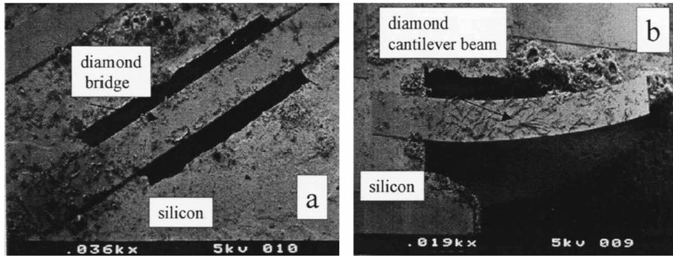
Figure 2.10: a) Fabricated diamond bridge, b) and cantilever beam [63]
