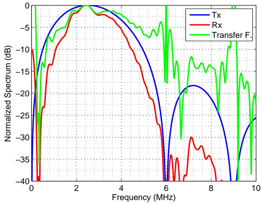
Figure 6.13: Normalized frequency response of CMUT array. ( $f=3$  MHz,  $V_{p-p}=10$  V, 1 cycle sinusoidal signal)
