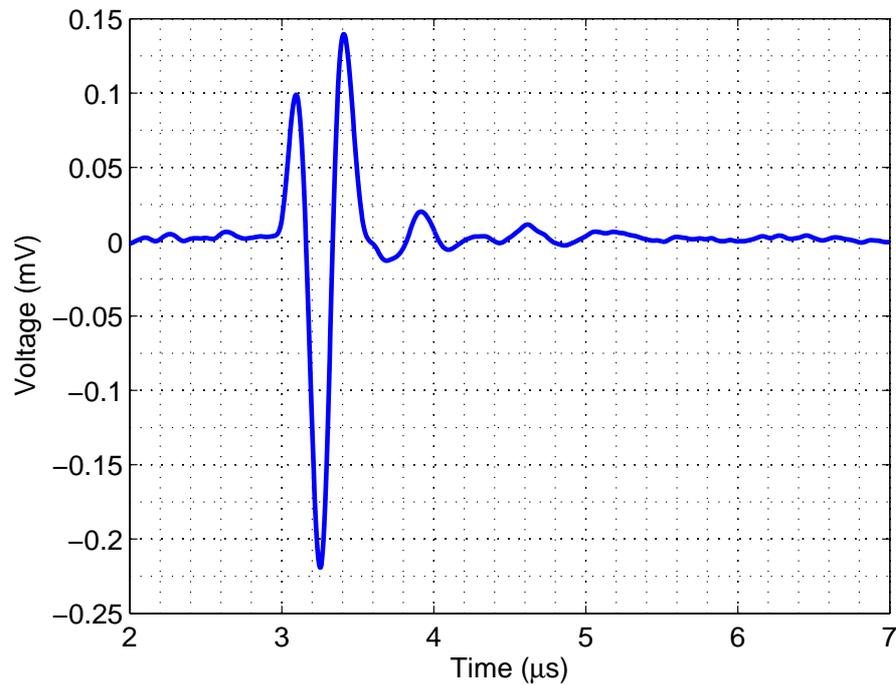
Figure 6.12: The hydrophone voltages of CMUT array. (  $f=3$  MHz,  $V_{p-p}=10$  V, 1 cycle sinusoidal signal)
