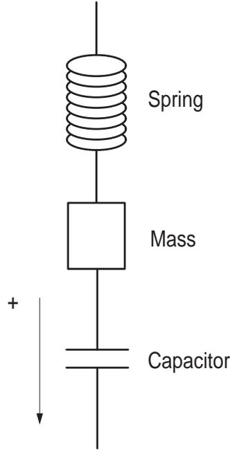
Figure 3.2: Lumped model of CMUT element [14]
