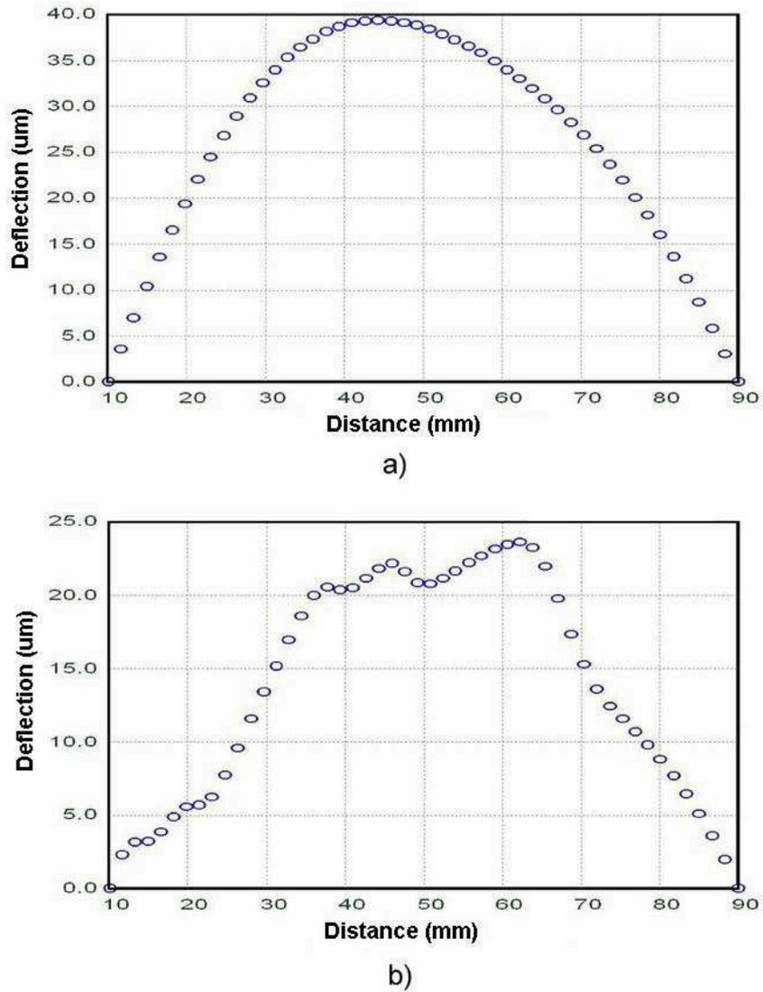
Figure 4.25: a) DOI wafer with compressive stress. Wafer bow:  $39 \mu\text{m}$ , Compressive stress: 217 MPa, b) DOI wafer with tensile stress. Wafer bow:  $37 \mu\text{m}$ , Tensile stress: 160 MPa
