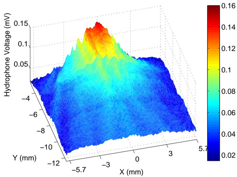
Figure 6.6: 2-D scanning measurement of the 7<sup>th</sup> element of 1-D CMUT array (  $f=3$  MHz,  $V_{p-p}=10$  V, 10 cycles sinusoidal signal)
