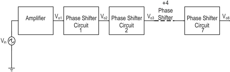
Figure 5.5: Designed phase shifter circuit
