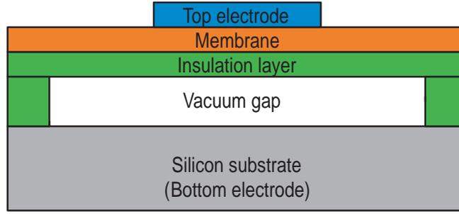
Figure 3.1: Typical membrane structure
