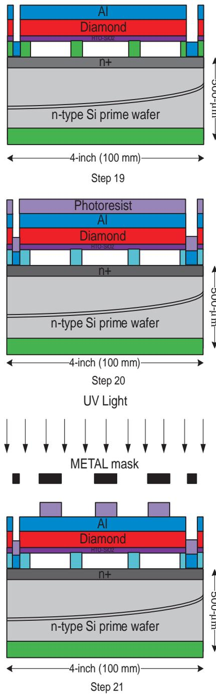
Figure 4.42: Process steps 19 to 21, Step 19 : Bonded wafers: Aluminum covering, Step 20 : Bonded wafers: Photoresist covering, Step 21 : Bonded wafers: Photoresist patterning with metal mask
