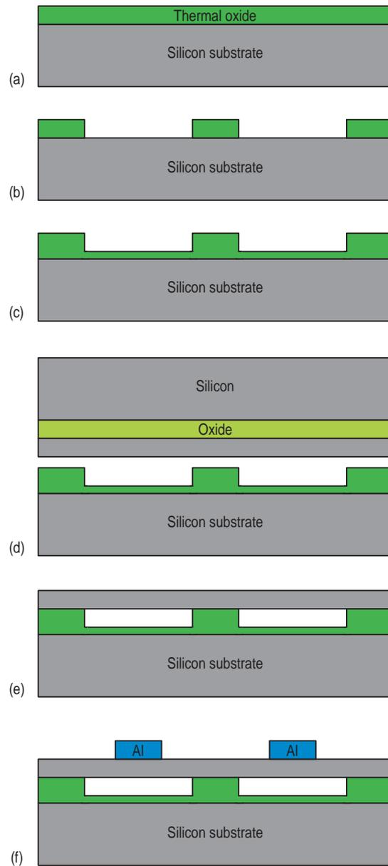
Figure 2.8: Fabrication of the CMUT devices using silicon fusion bonding [47]. (a) Thermal oxide growing on silicon wafer, (b) Etching the thermal oxide to form the CMUT membranes, (c) Thermal oxide grown in order to prevent possible electrical shorts between the substrate and top electrode, (d) Prime and SOI wafer are brought together in vacuum conditions, (e) CMUT device with silicon membrane, (f) Sputtered aluminum electrodes at the top of the CMUT membranes
