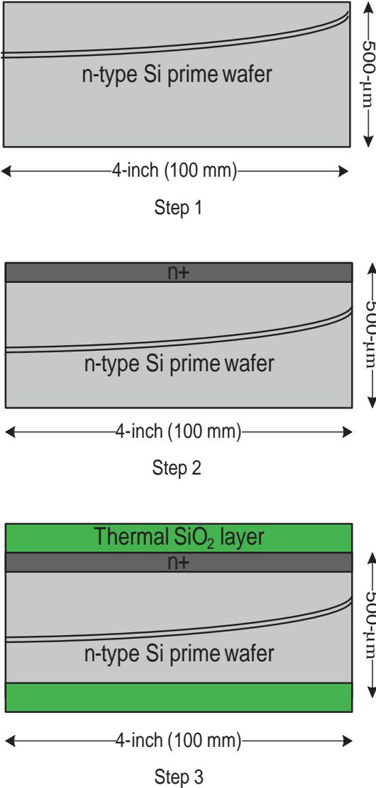
Figure 4.36: Process steps 1 to 3, Step 1: Bottom wafer: n-type silicon wafer, Step 2 : Bottom wafer: P doing for conductive surface, Step 3 : Bottom wafer: Thermal oxide growth
