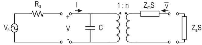
Figure 3.4: Electrical equivalent circuit of CMUT device [18]
