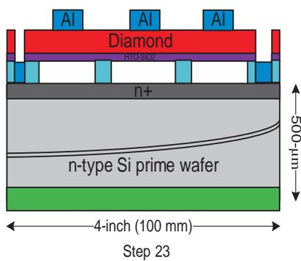
Figure 4.43: Process Step 22 : Bonded wafers: Aluminum etch with chemicals and photoresist stripping with O<sub>2</sub> plasma
