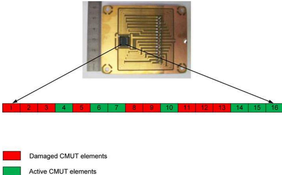
Figure 6.3: Location and condition of elements of 1-D CMUT array
