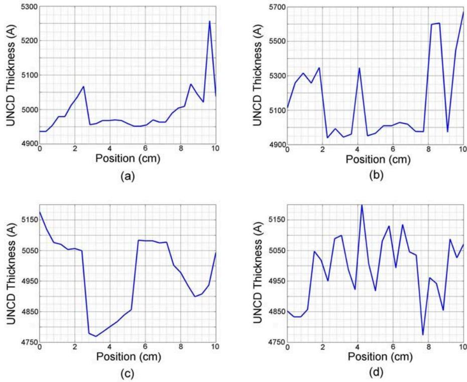
Figure 4.23: a) First wafer LR thickness measurement, b) First wafer TB thickness measurement, c) Second wafer LR thickness measurement, d) Second wafer TB thickness measurement
