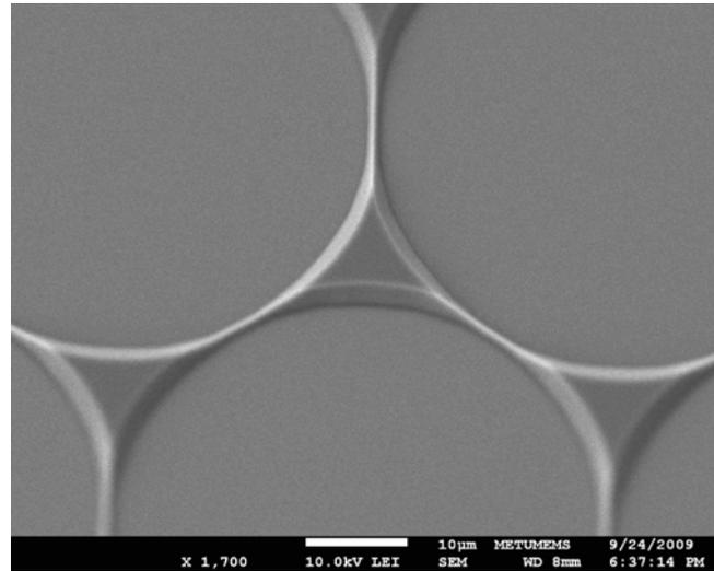
Figure 4.14: SEM image of membrane cavities after BOE method
