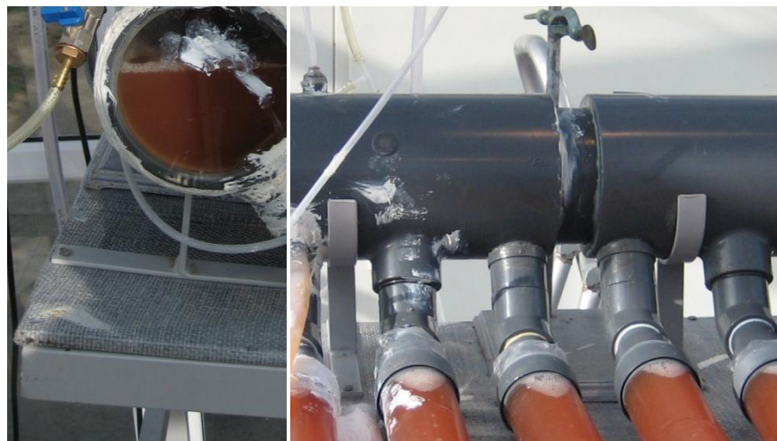
Figure 3-8 The handles covering the header manifold of the tubular photobioreactor
