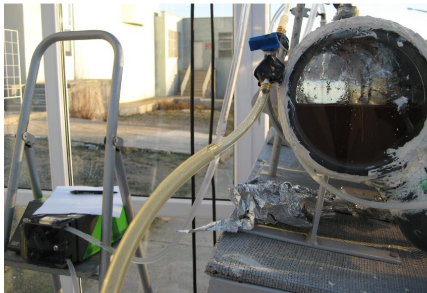
Figure 3-11 The start-up and the headspace of the tubular photobioreactor
