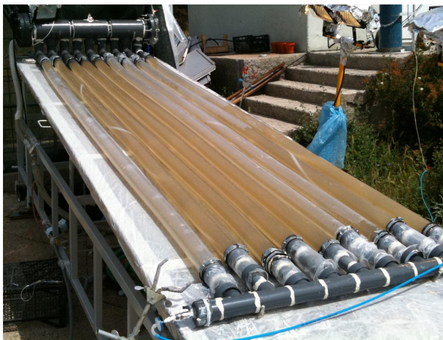
Figure 4-10 Picture of the tubular PBR during RUN: 062010 just after the start-up for RUN: 062010
