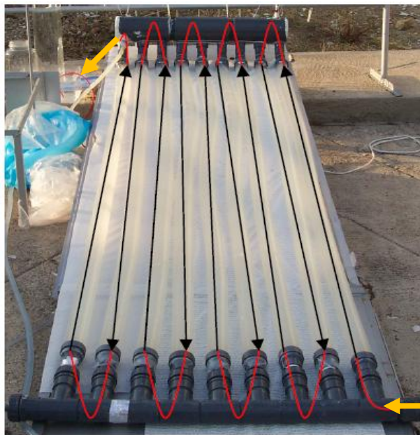
Figure 3-5 Integration and direction of the cooling coils inside the tubular photobioreactor
