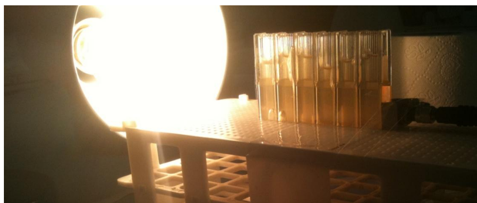
Figure 4-60 Experimental setup for measuring the photon counts and light intensities of the dark fermenter effluents.
