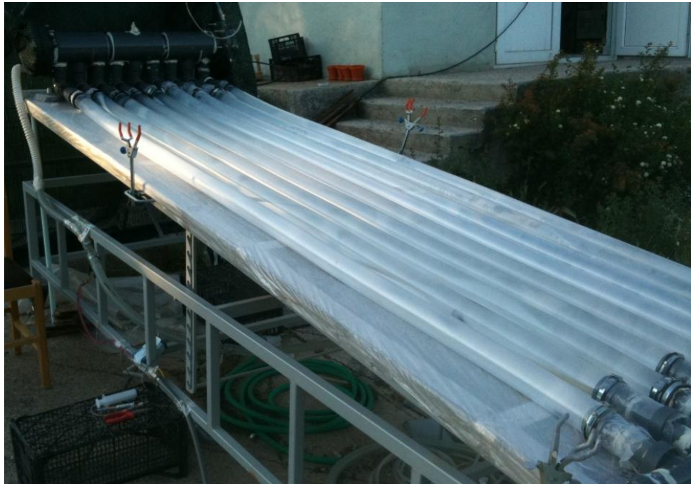
Figure 3-10 The water filled tubular photobioreactor under air pressure test
