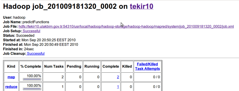
Figure 3.3.1 The web based user interface of Hadoop gives information about the status of submitted jobs. Therefore, a user can monitor its own job.
