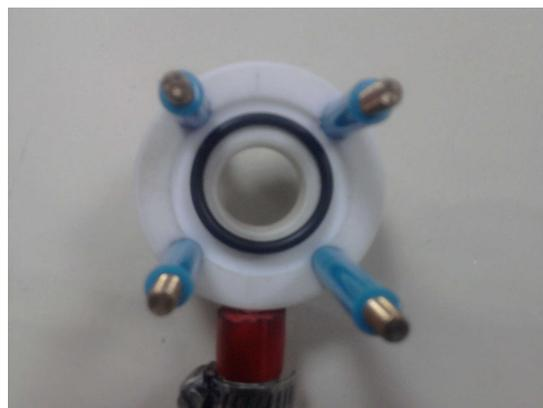
Figure 5.16: The Teflon Separator
