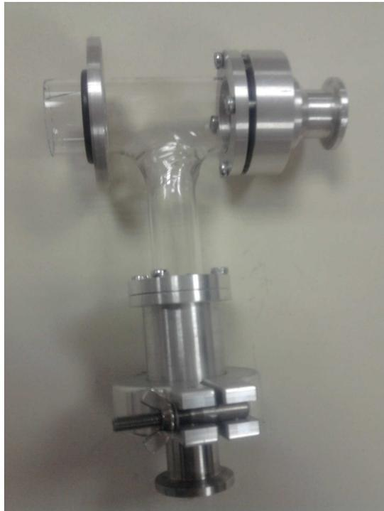
Figure 5.17: The Vacuum Gradient Part
