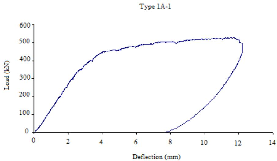
Figure 4.15 Load-Deflection Diagram (Type 1A-1)
