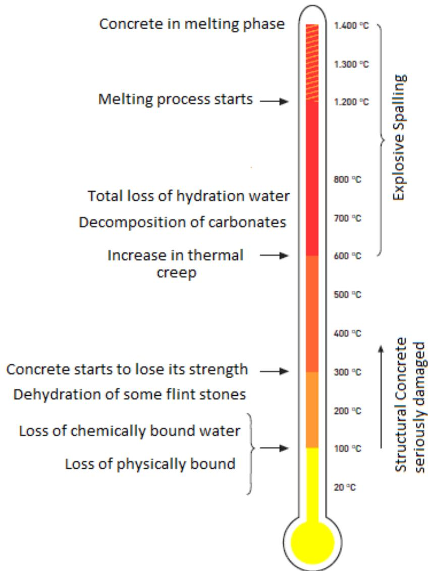
Figure 2.1 Behavior of Concrete under Temperature Effect [6]
