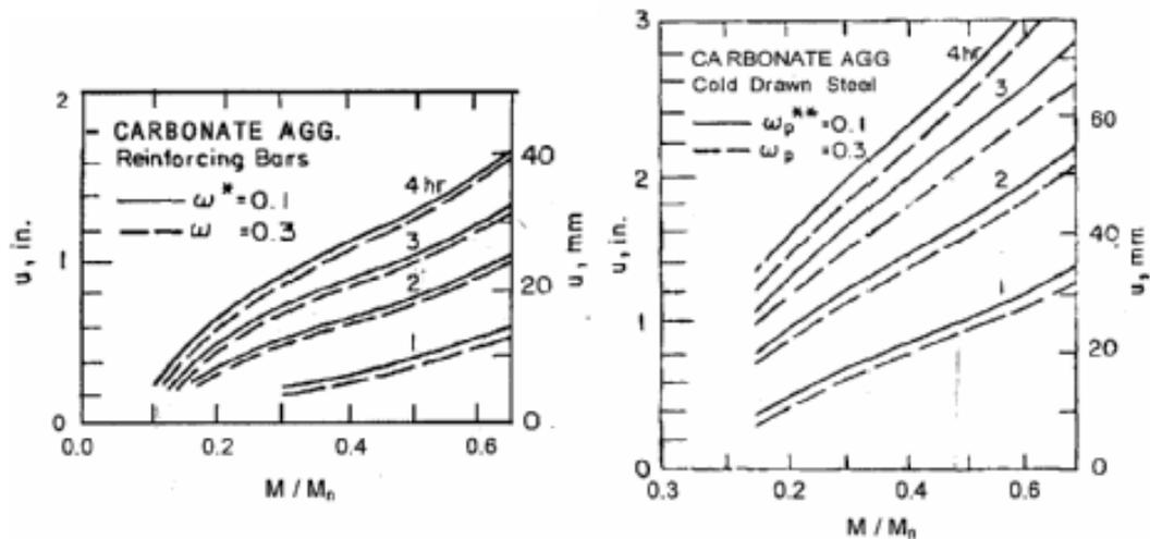
Figure I.1 Fire Endurance of Concrete Slabs as Influenced by Aggregate Type, Reinforcing steel Type, Moment Intensity and  $u$  [2]
