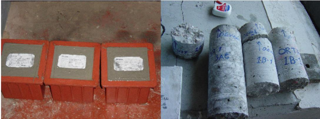
Figure 3.16 Compression Test Samples
