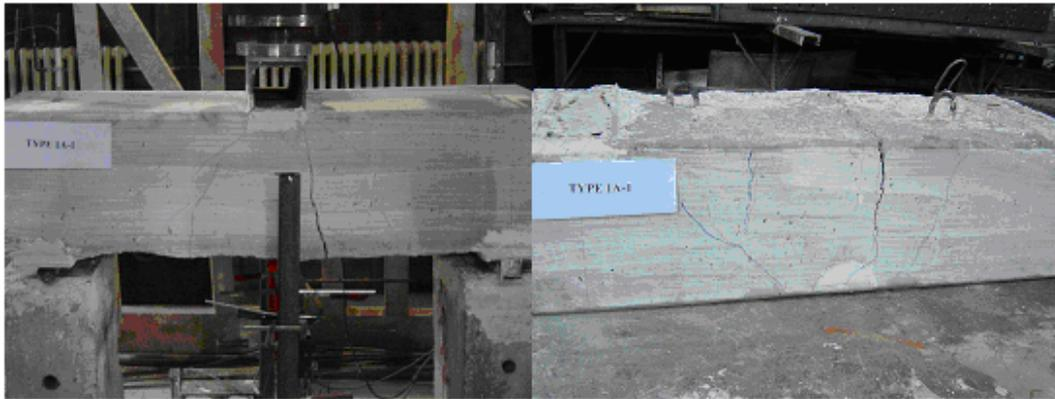
Figure 4.14 Type 1A-1 Specimen after Static Loading Test
