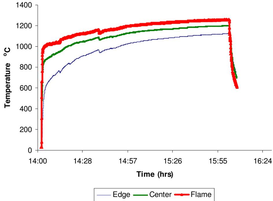
Figure 4.7 Temperature Data Gained from Second Fire Test
