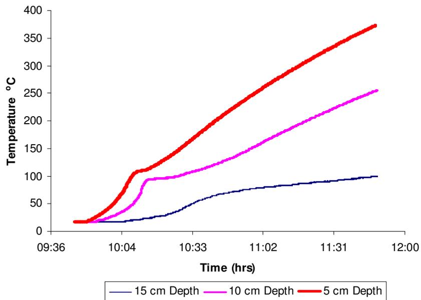
Figure 4.4 Temperature Distributions in the Specimen Measured from Hot Surface
