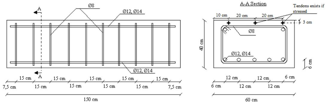
Figure 3.5 Configuration of Reinforcement
