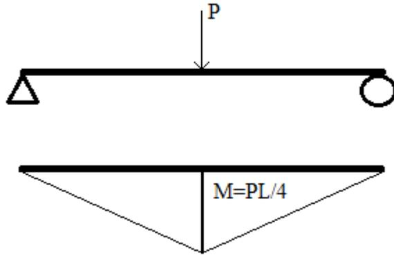
Figure 5.4 Simply Supported Beam
