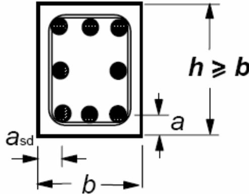
Figure 2.4 Cross-Section Properties According to Eurocode 2 [3]
