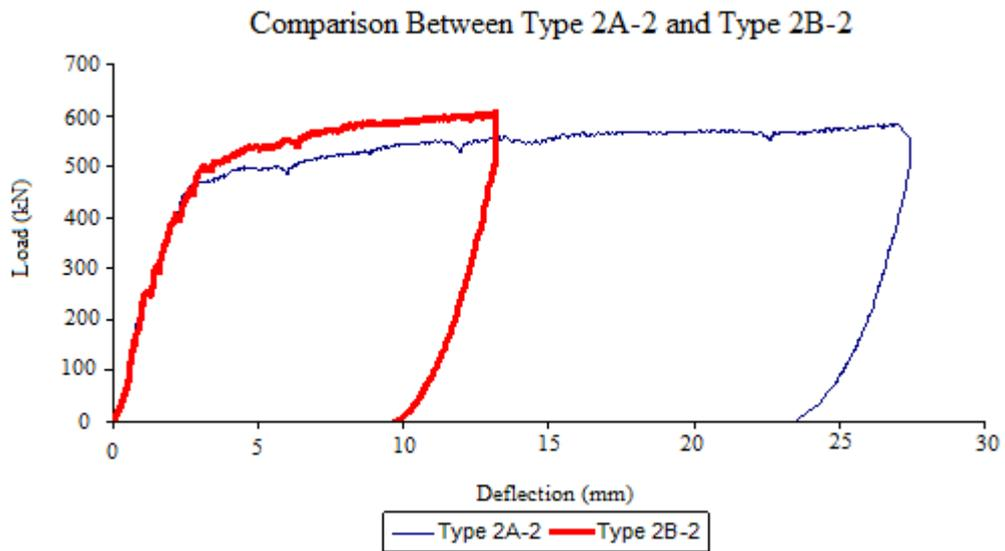
Figure F.3 Load-Deflection Diagram (Type 2A-2, Type 2B-2)
