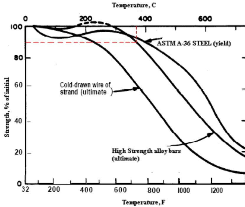
Figure 5.2 Strength of Certain Steels at High Temperatures [2]
