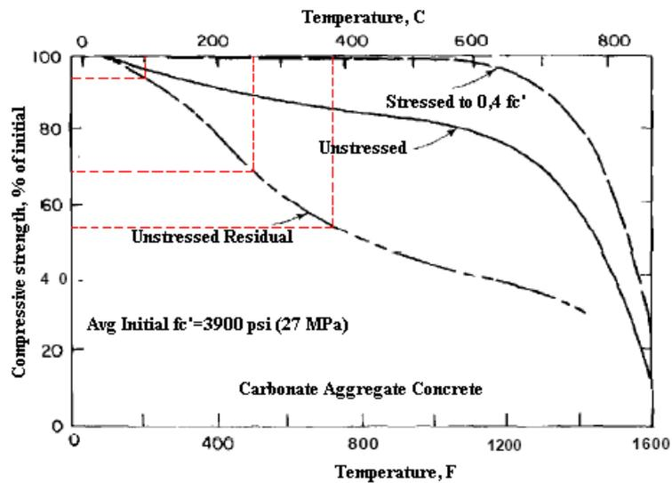
Figure 5.3 Compressive Strength of Carbonate Aggregate Concrete at High Temperature and After Cooling [2]
