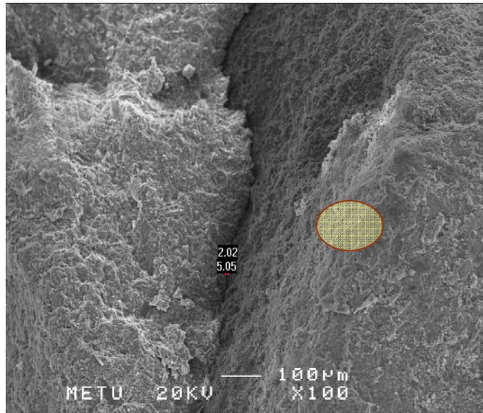
Figure 4.31 Internal Cracking in the Core
