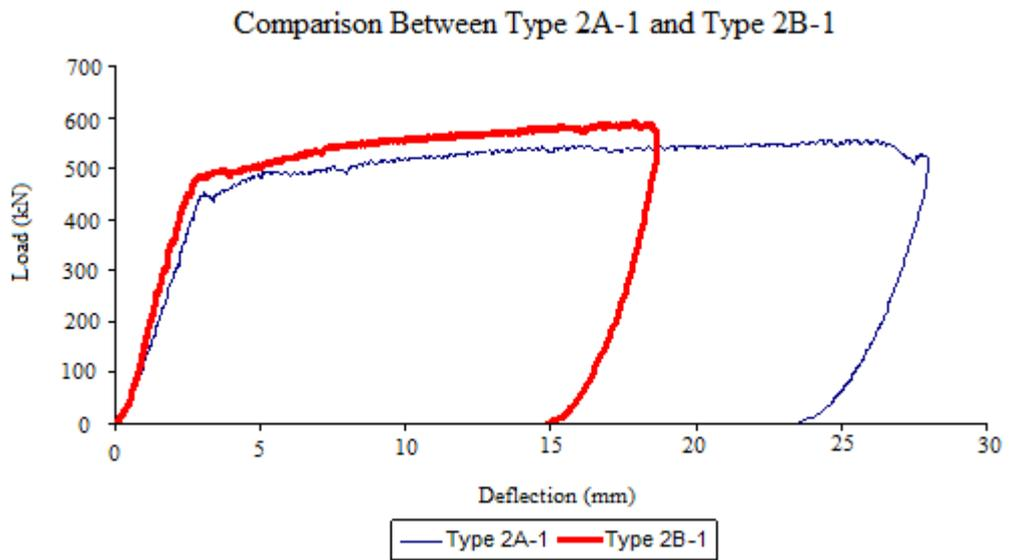
Figure F.4 Load-Deflection Diagram (Type 2A-1, Type 2B-1)
