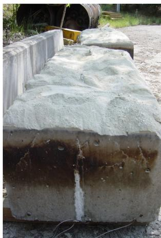
Figure 4.5 Concrete Face After Fire Test (Type 1B-1)
