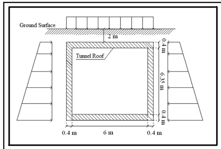
Figure 3.1 Tunnel Cross-Section and Loads
