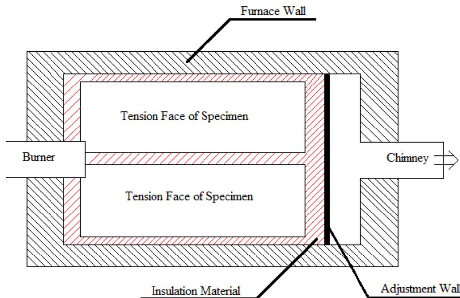
Figure 3.12 Plan View of Inside of Furnace
