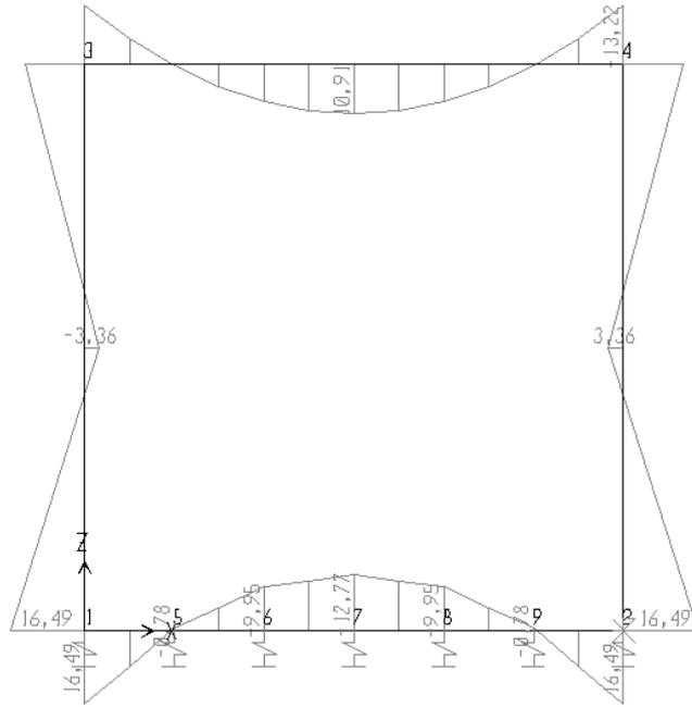
Figure B.4 Moment Diagram (M3-3) (Ton-m)
