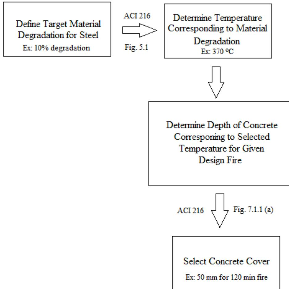
Figure 5.8 Concrete Cover Decision Algorithm
