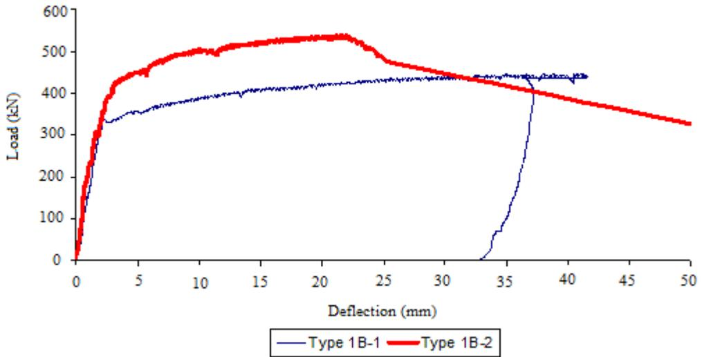
Figure E.3 Load-Deflection Diagram (Type 1B-1, Type 1B-2)
