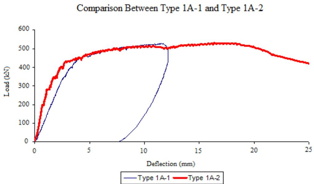
Figure E.1 Load-Deflection Diagram (Type 1A-1, Type 1A-2)
