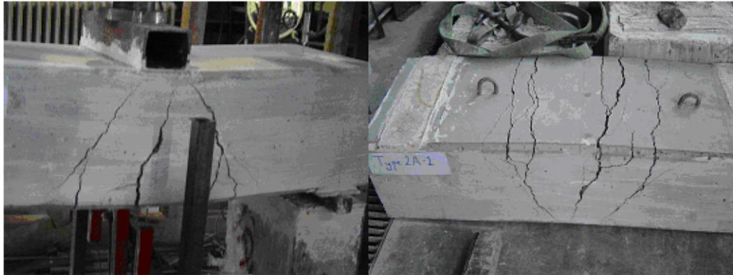
Figure 4.20 Type 2A-2 Specimen after Static Loading Test
