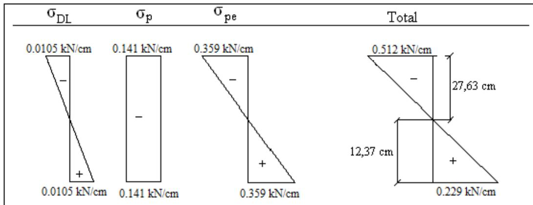
Figure C.3 Stress Distributions after Pre-stressing Losses
