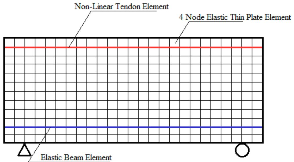
Figure 5.6 Components of the LARSA 4D Model
