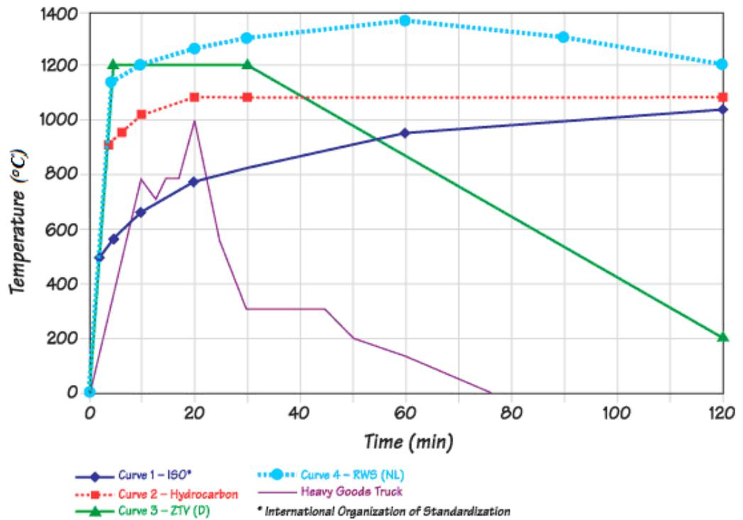
Figure 2.3 Fire-Air Temperature Curves for Tunnels [8]
