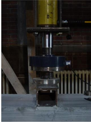
Figure 3.14 Load Cell
