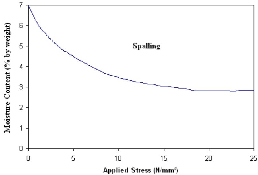
Figure 2.2 Explosive Spalling Relationship of Moisture Content and Pressure [18]
