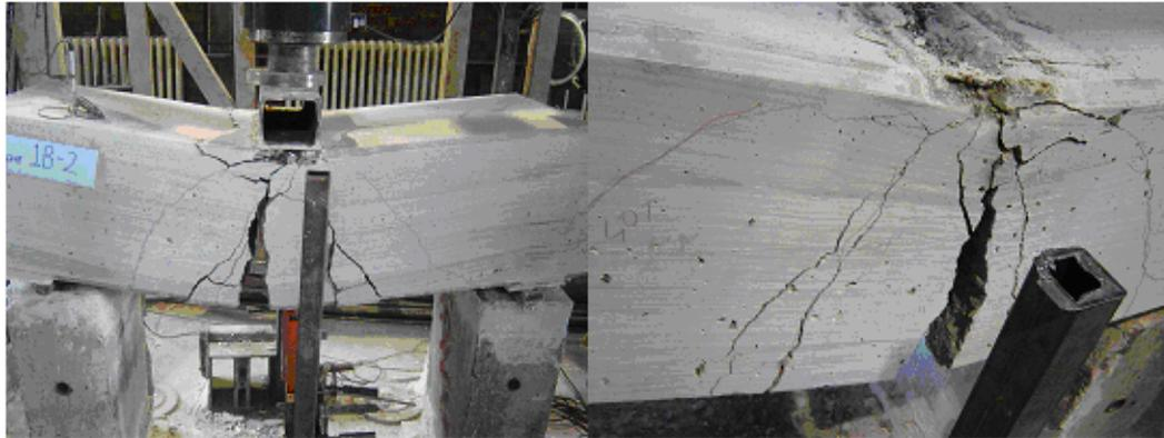
Figure 4.24 Type 1B-2 Specimen after Static Loading Test
