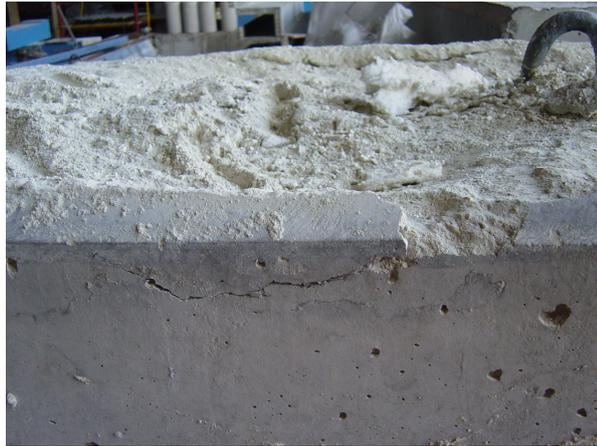
Figure 4.8 Concrete Face After Fire Test (Type 1A-1)
