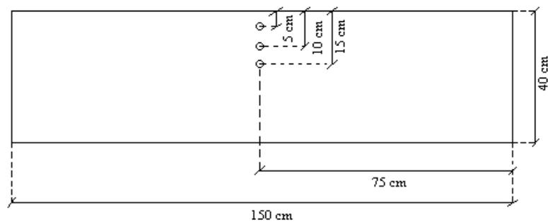
Figure 5.1 Locations of Thermocouples
