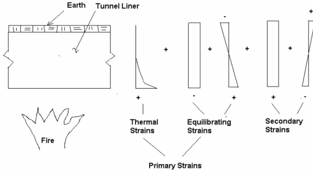
Figure 5.5 Total Strain Distribution [15]
