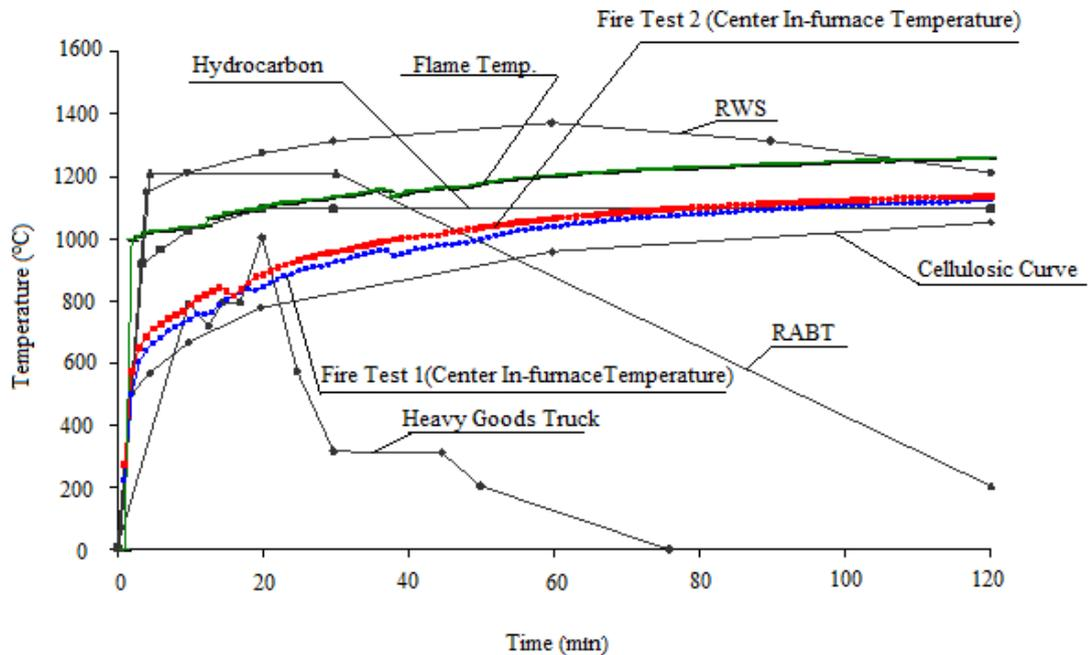
Figure 4.10 Temperature Curves after Tests
