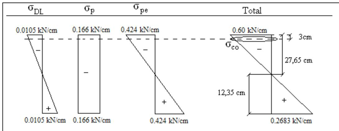
Figure C.1 Stress Distributions without Pre-stressing Losses
