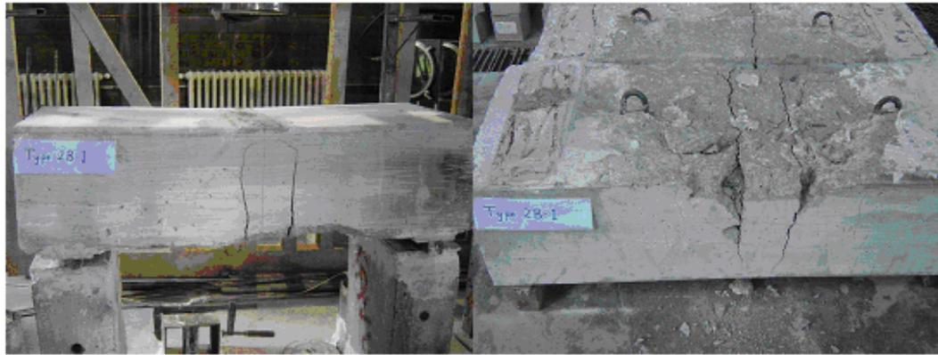
Figure 4.26 Type 2B-1 Specimen after Static Loading Test
