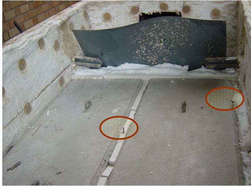
Figure 4.1 Inside of the Furnace and Thermocouple Placements
