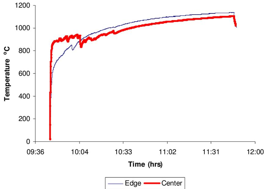
Figure 4.3 Temperature Data Gained from First Fire Test
