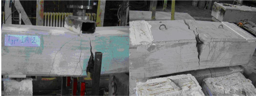
Figure 4.16 Type 1A-2 Specimen after Static Loading Test
