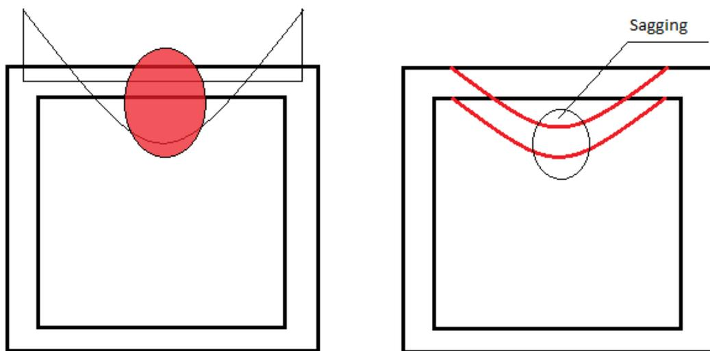
Figure 2.5 Sagging of Cut and Cover Tunnel Roof
