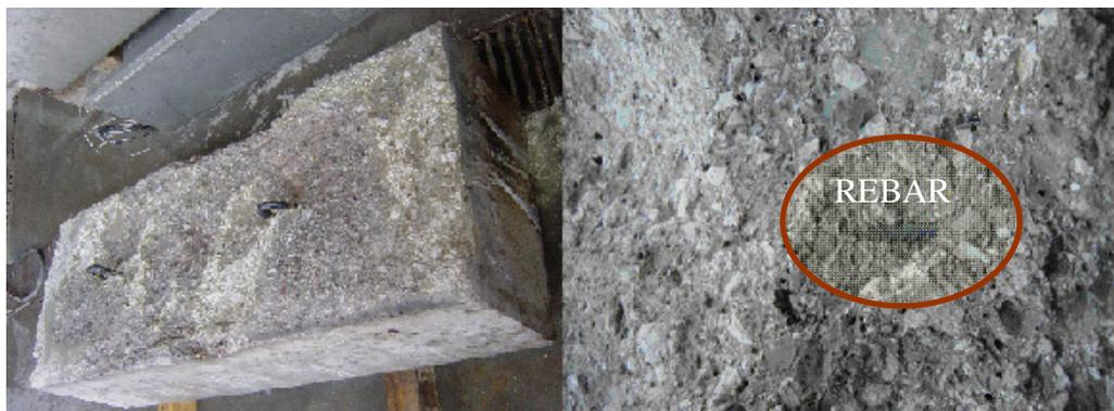
Figure 4.9 Concrete Faces after Fire Test (Type 2B-1)
