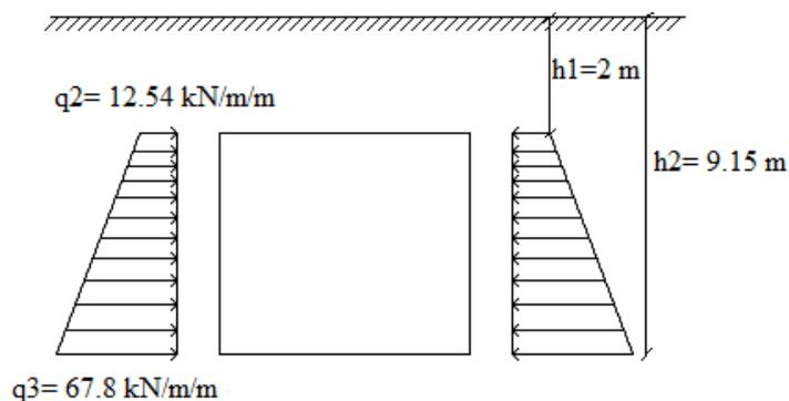
Figure 3.4 Horizontal Soil Load on Tunnel
