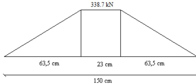
Figure C.2 Load Distributions after Pre-stressing Losses
