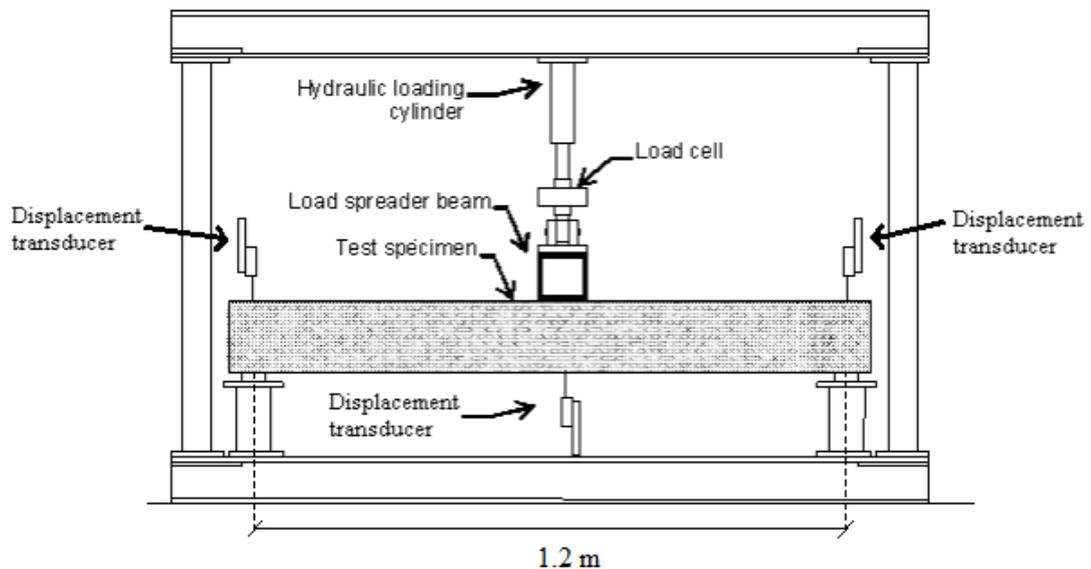
Figure 3.13 Static Load Set-up -1
