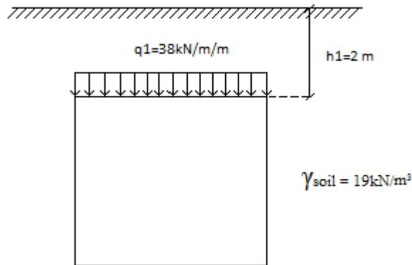
Figure 3.3 Overburden Soil Load on Tunnel
