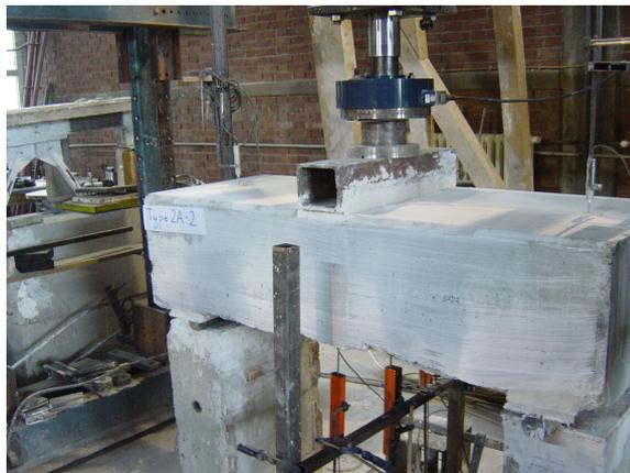
Figure 3.15 Static Load Set-up -2
