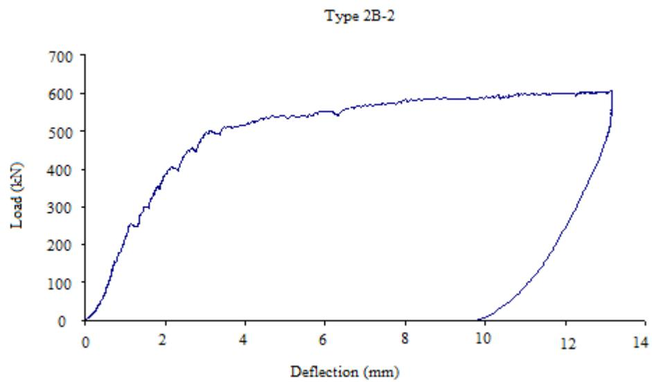
Figure 4.29 Load-Deflection Diagram (Type 2B-2)
