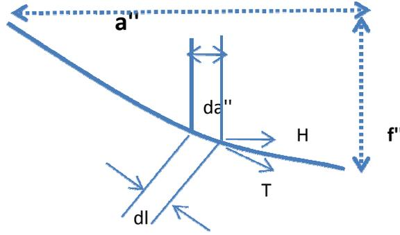
**Figure D.2:**Cable Element.
