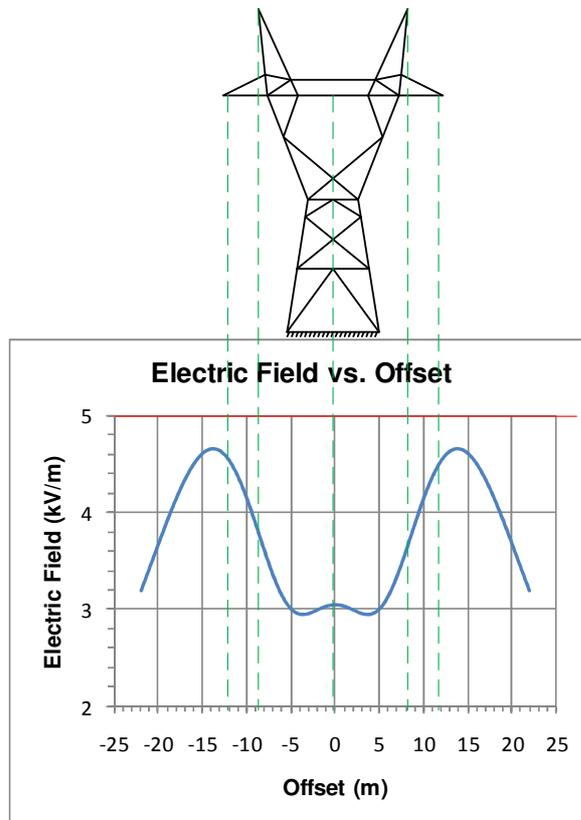
**Figure 5.6:**E field pattern of two successive 3PD (27) type towers, 1m above ground at mid span.
