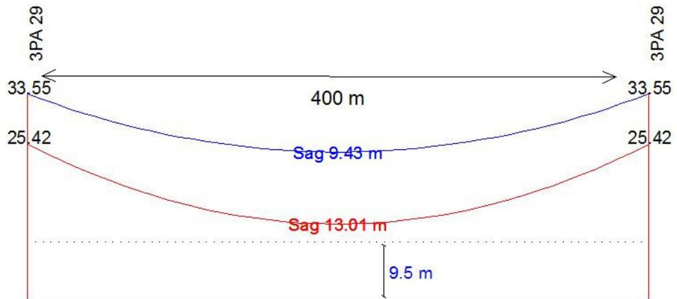
**Figure 5.7:**Two successive 3PA (29) type towers with a span length of 400 m.
