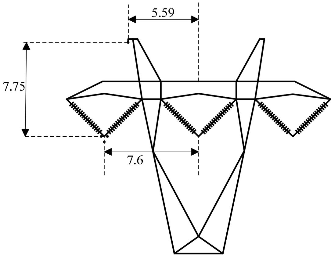
**Figure 3.5:** Top Geometry of Type 3PB tower. (Distances are in m).
