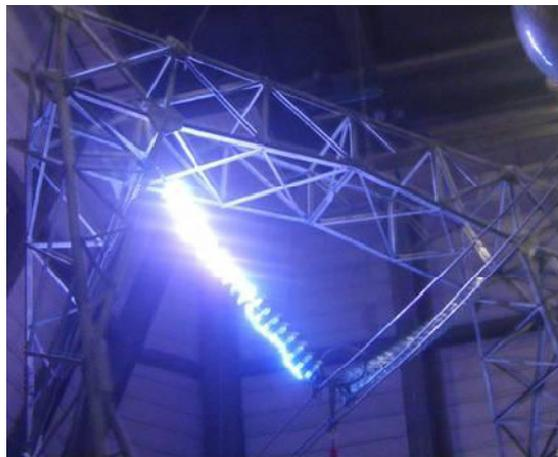
**Figure 3.1:** Discharge along the insulator surface.
