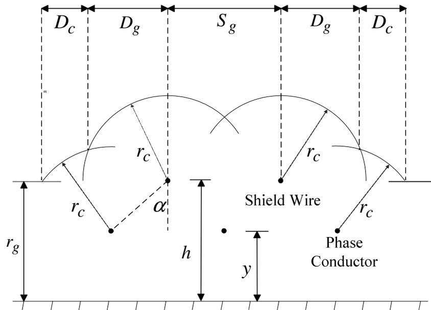
**Figure 3.2:** The Geometric Model, Distances.
