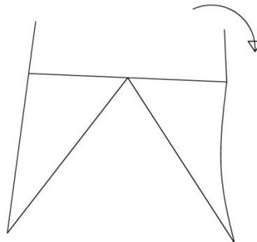
**Figure 4.7** Buckling of the leg.
