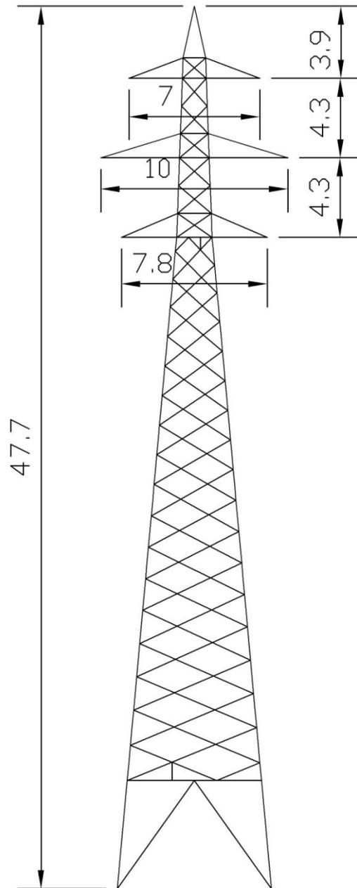
**Figure 4.5** Outline of 2FA type tower. (Distances are in m).
