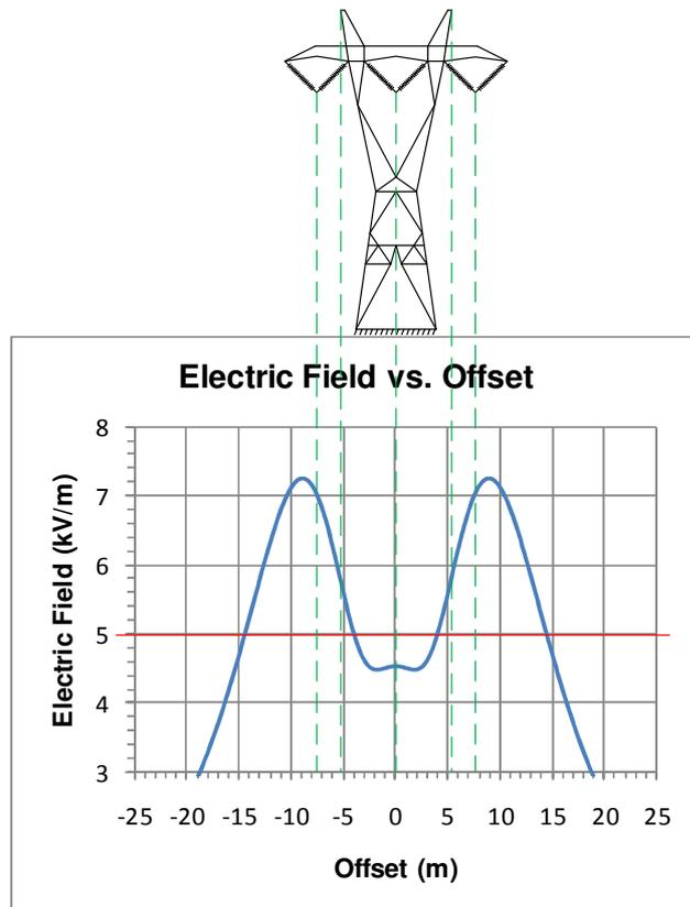
**Figure 5.4:** E field pattern of two successive 3PA (26) type towers, 1m above ground at mid span.
