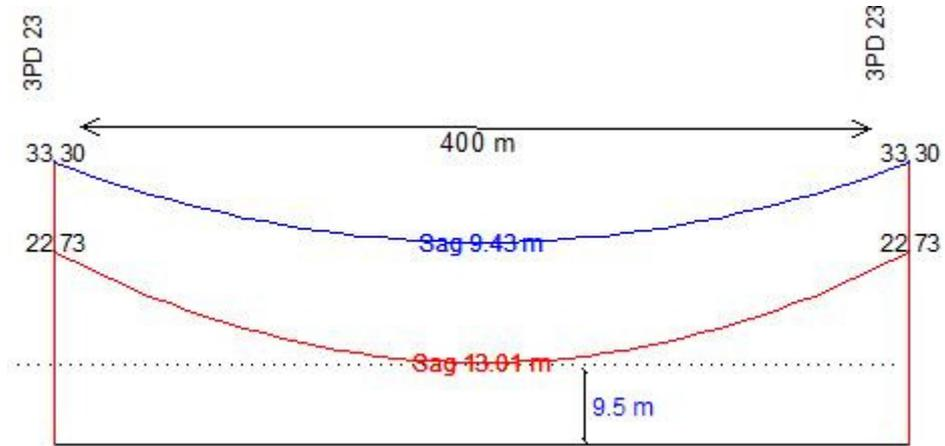
**Figure 5.1:**Two successive 3PD(23) type towers with a span length of 400 m.
