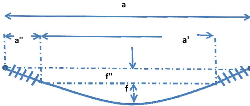
**Figure D.1:** Slack Span.
