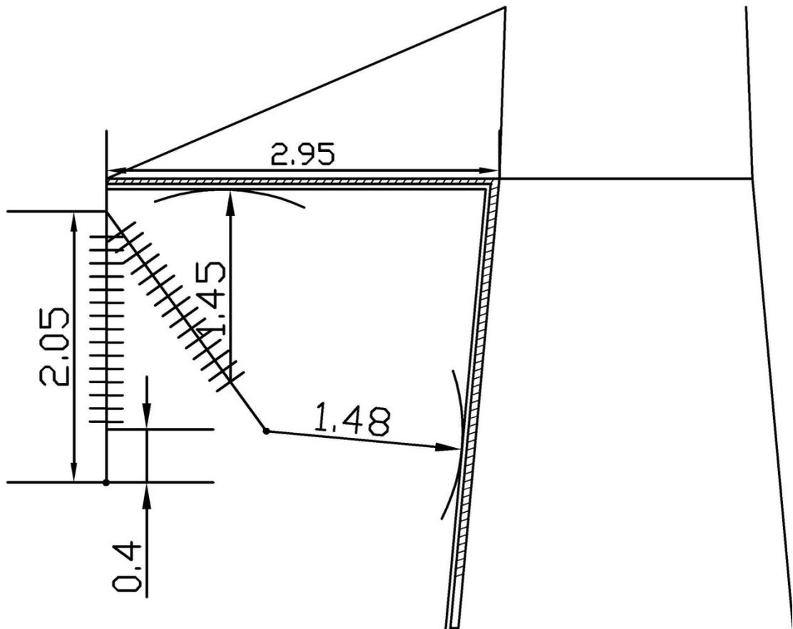
**Figure 4.9** Swing of the insulator set for reduced wind. (Distances are in m).
