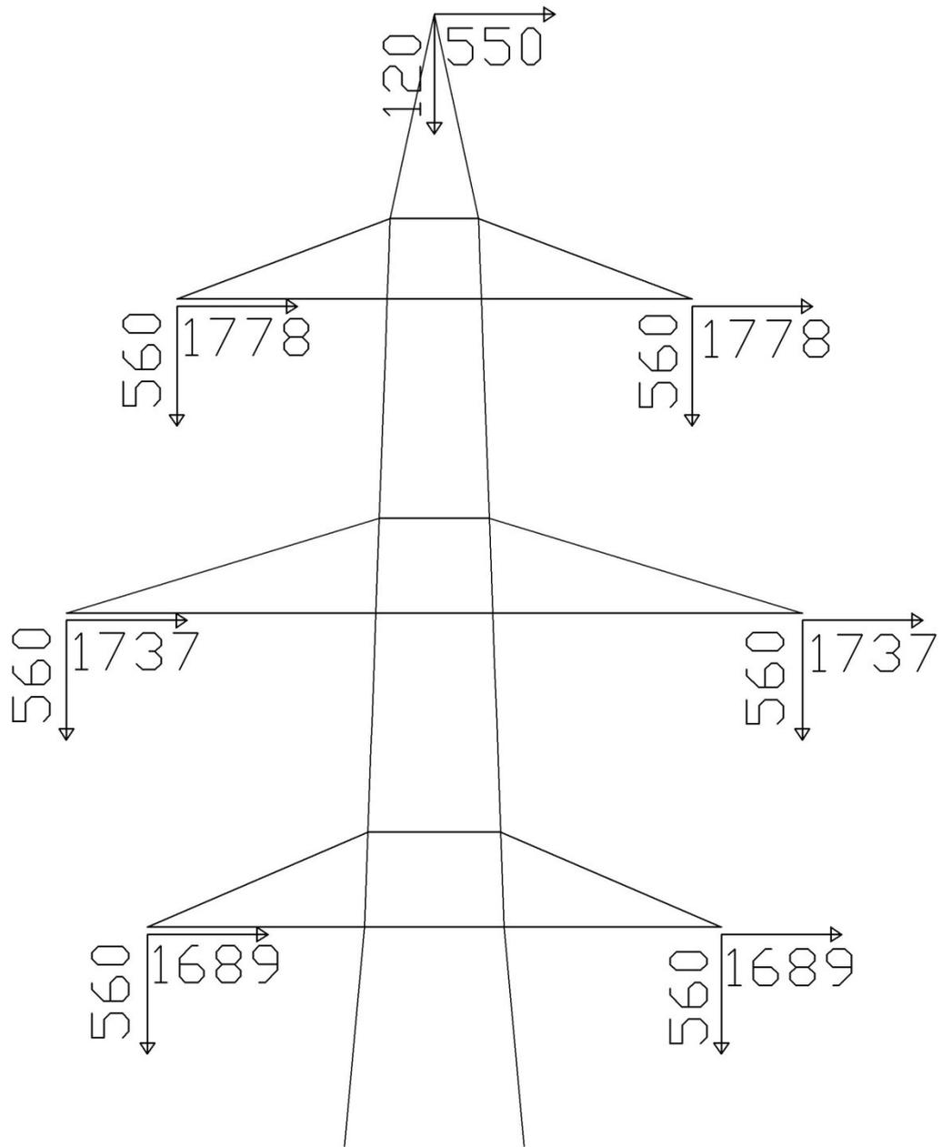
**Figure B.1:** The resultant loads transferred by the conductors and the insulators, in kgf.
