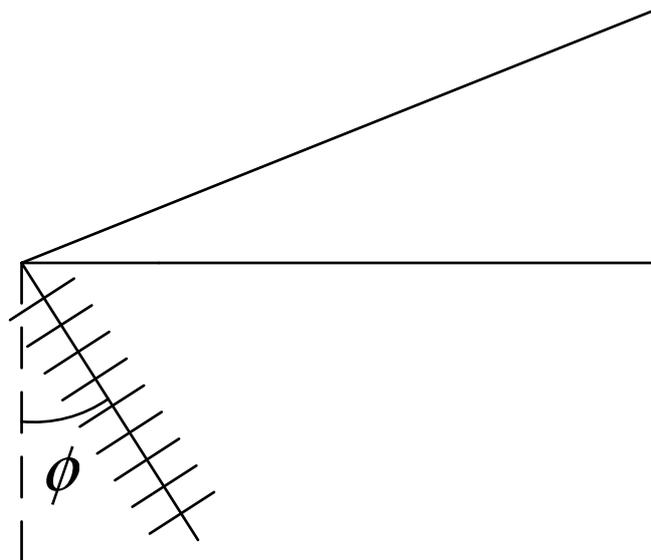
**Figure 4.4** Insulator Swing Angle.
