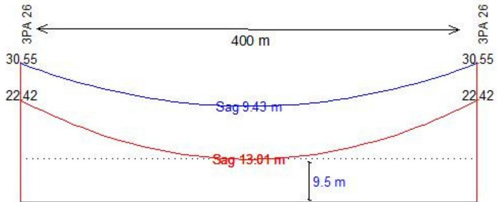
**Figure 5.3:**Two successive 3PA (26) type towers with a span length of 400 m.
