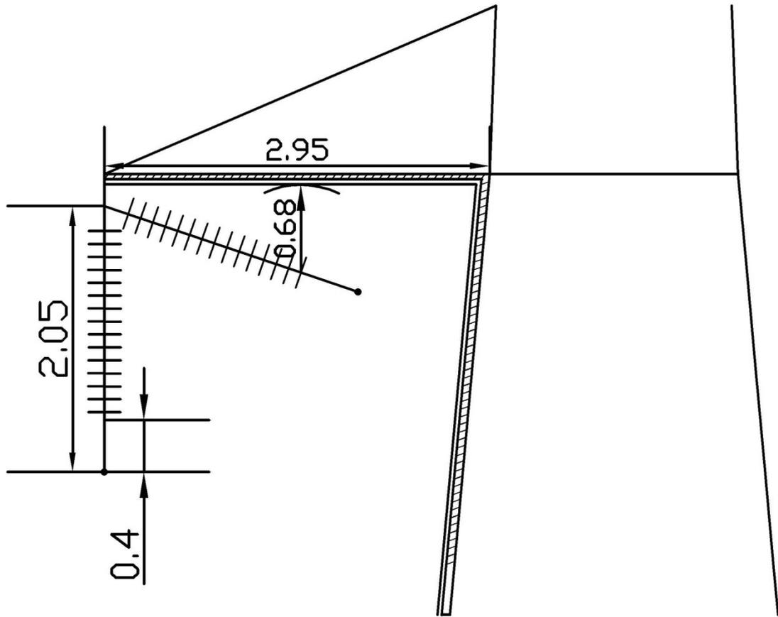
**Figure 4.8** Swing of the insulator set for extreme wind. (Distances are in m).
