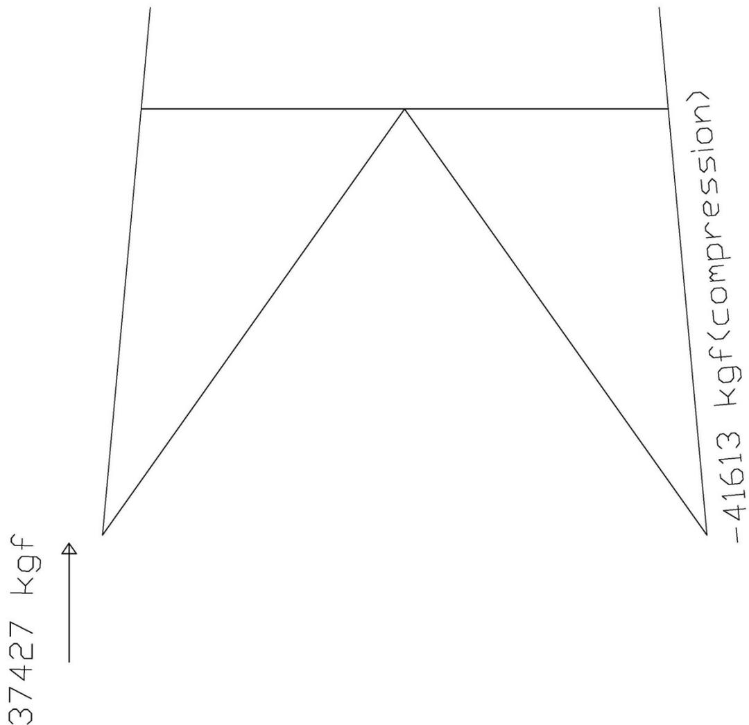
**Figure B.3:** The foundation reaction and the compression force of the leg.
