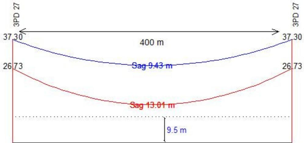
**Figure 5.5:**Two successive 3PD (27) type towers with a span length of 400 m.
