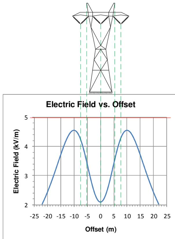
**Figure 5.8:**E field pattern of two successive 3PA (29) type towers, 1m above ground at mid span.
