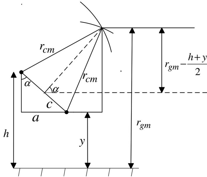
**Figure 3.4:** Finding the Maximum Shielding Failure Current.
