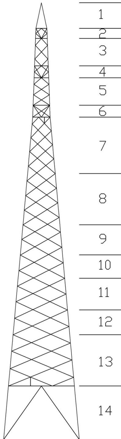
**Figure B.2:** Right view, panels for transverse wind.
