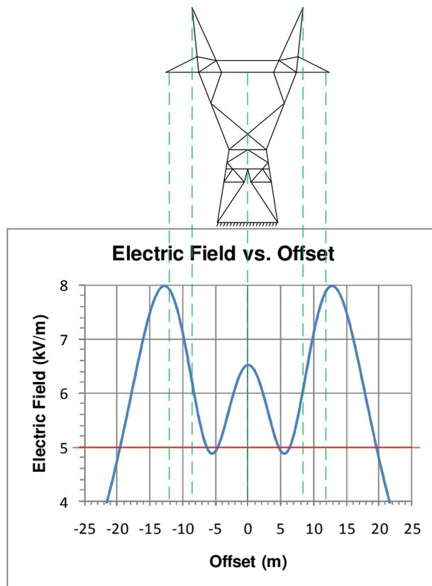
**Figure 5.2:** E field pattern of two successive 3PD (23) type towers, 1m above ground at mid span.
