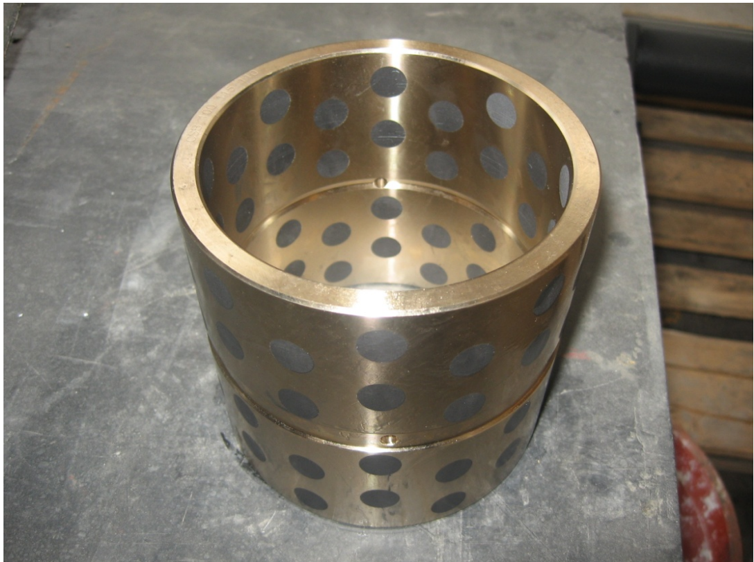
Figure 5.2 – A view of bronze bearing
