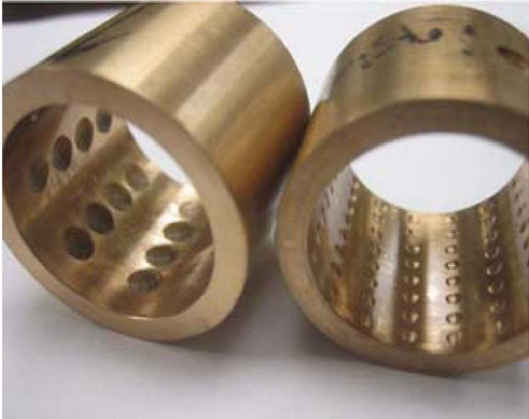
Figure 2.6 – Bearings with dimples [11]
