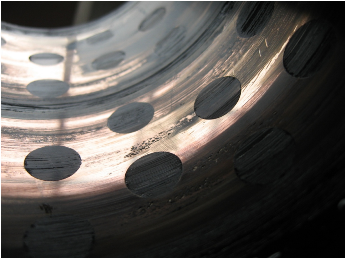
Figure 6.4 – Pit hole formation on the bronze test bearing
