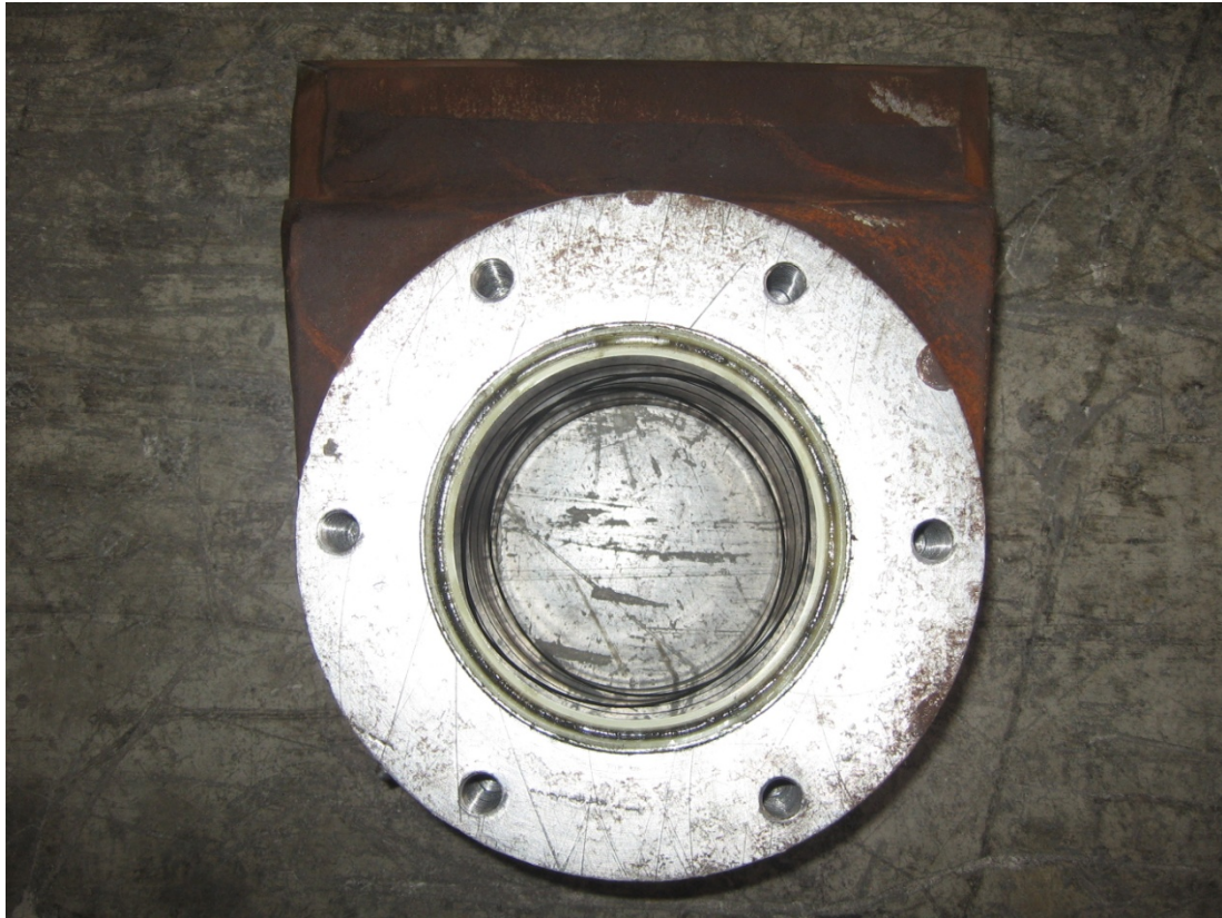
Figure 4.3 – An end view of the test bearing housing
