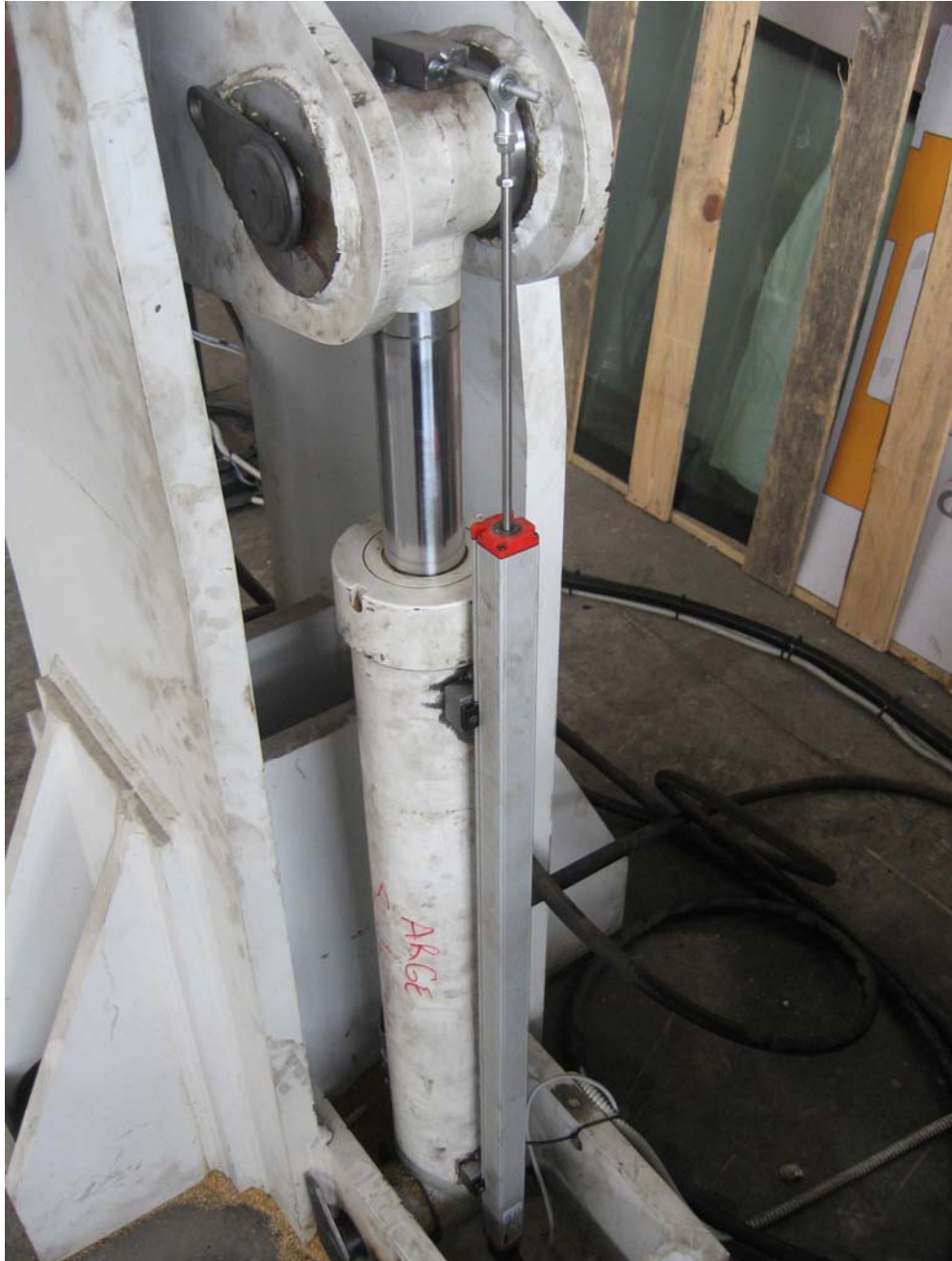
Figure 4.5 – Linear variable differential transformer mounted on oscillating arm
