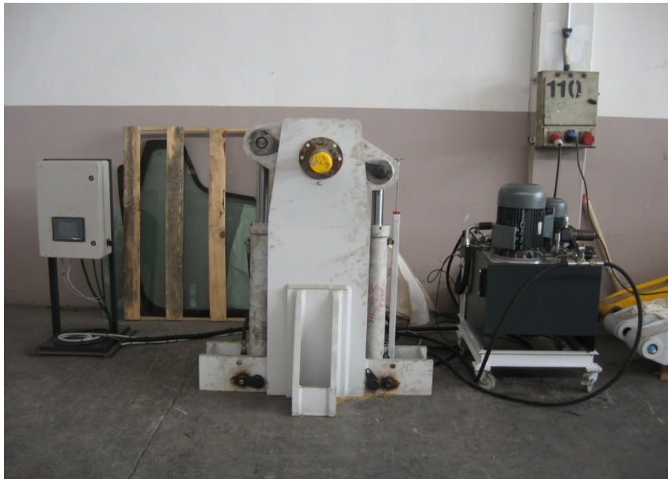
Figure 4.10 – Test bench with hydraulic power pack and control panel
