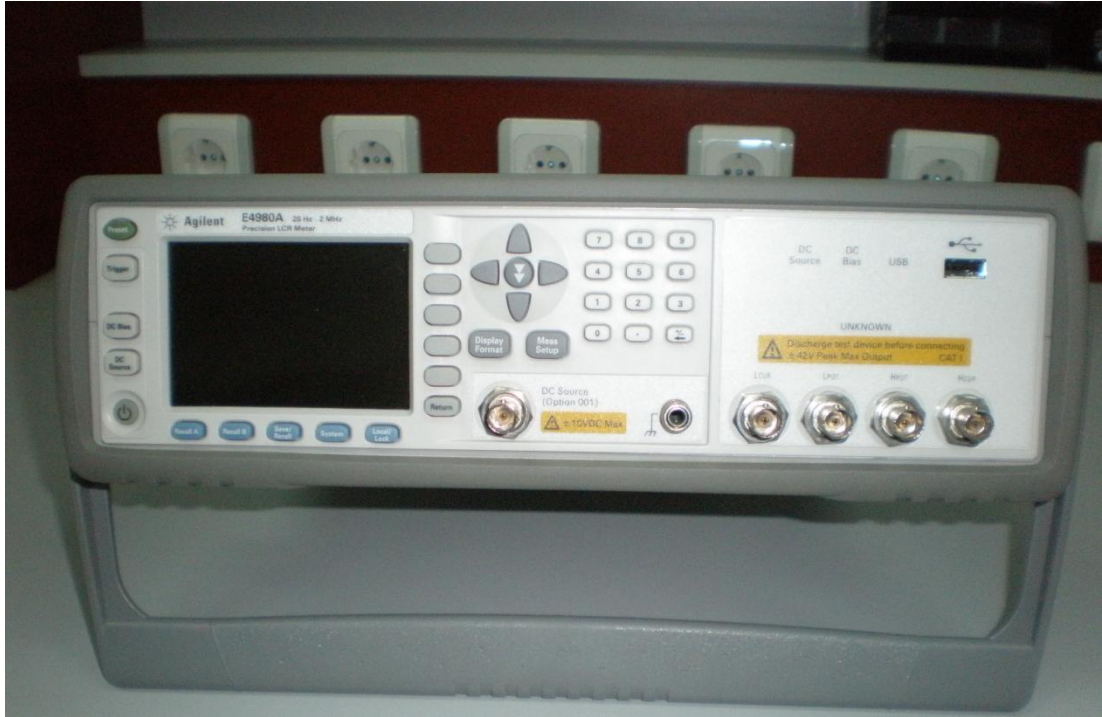
Figure 5.3: Agilent E4980A LCR meter used to measure capacitance changes on both sides of the accelerometer during sensitivity measurements.
