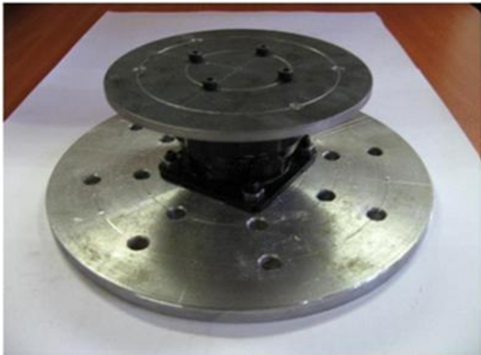
Figure 5.2: Rotating head on which the accelerometer is mounted during the sensitivity tests
