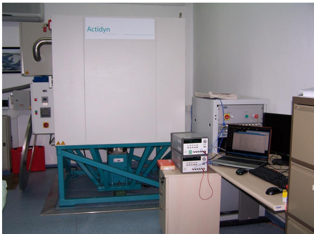
Figure 5.12: Centrifugal test cabin and the exterior test setup for the measurement range detection tests
