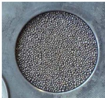
Figure 4.2. Steel Balls with Average 3 mm Diameter (min. 2-max. 4 mm)
