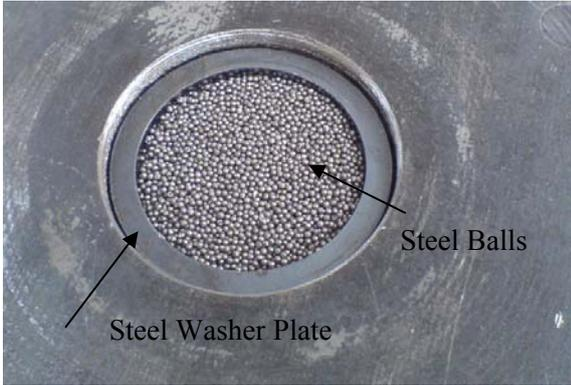
Figure 4.45. Steel Washer Plates with Steel Balls (Washer Hole Diameter: 80 mm)
