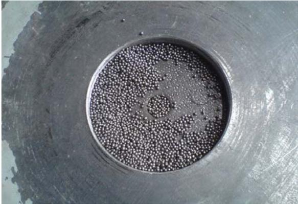
Figure 4.43. Steel Washer Plates with Steel Balls (Washer Hole Diameter: 17.5 mm)
