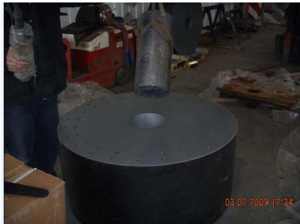
Figure 2.2. Placement of the Lead Core (Photo Courtesy of Alga Spa)
