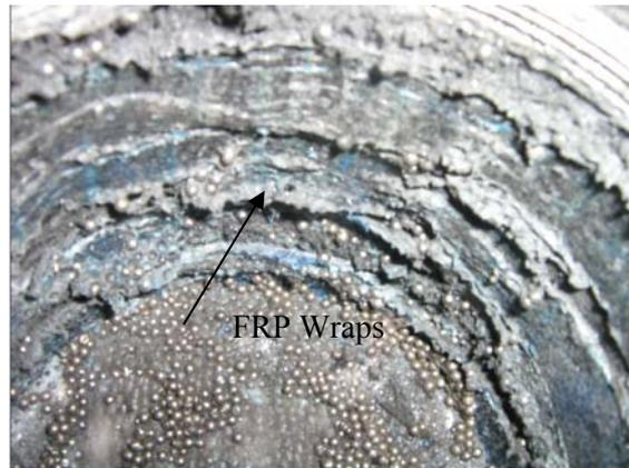
Figure 4.48. FRP Wraps (After Testing)
