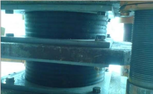
Figure 4.33. Bulged Bearings under  $P_{ver}=500$  kN
