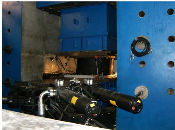
Figure 2.4. Prototype Test of a Big LRB [51]
