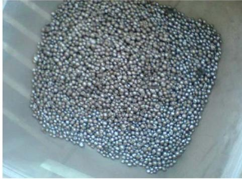
Figure 4.3. Steel Balls with Average 5 mm Diameter (min. 4-max. 6 mm)
