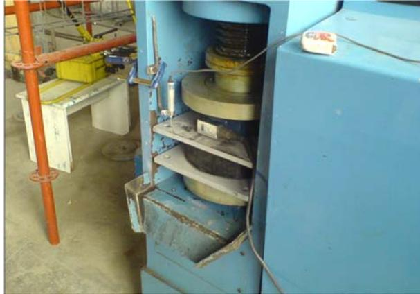
Figure 3.4. View of the Test Equipment Utilized in Vertical Compression Tests
