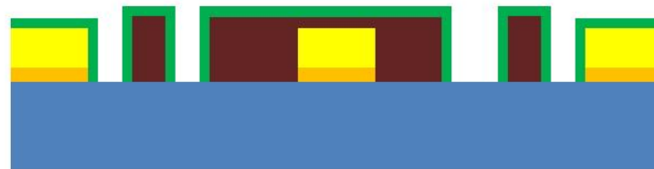
Cr etch, channel forming lithography and parylene-C deposition
