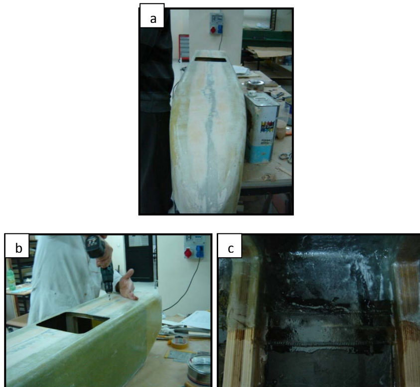
Figure 30: The fuselage assembly with inner structure taken out of the molds (a), Cutting off the access doors (b), Reinforcement of the skin connection line (c)
