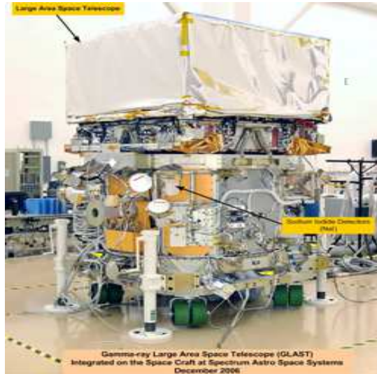
Figure 5.1: The LAT (silver box at the top) was integrated on the spacecraft at General Dynamics Advanced Information Systems in December 2006.
