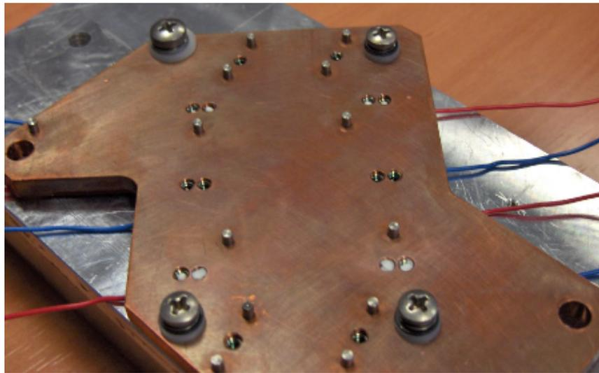
Figure 2.15 The Assembled Base Plate, TEC Module and Heat sink
