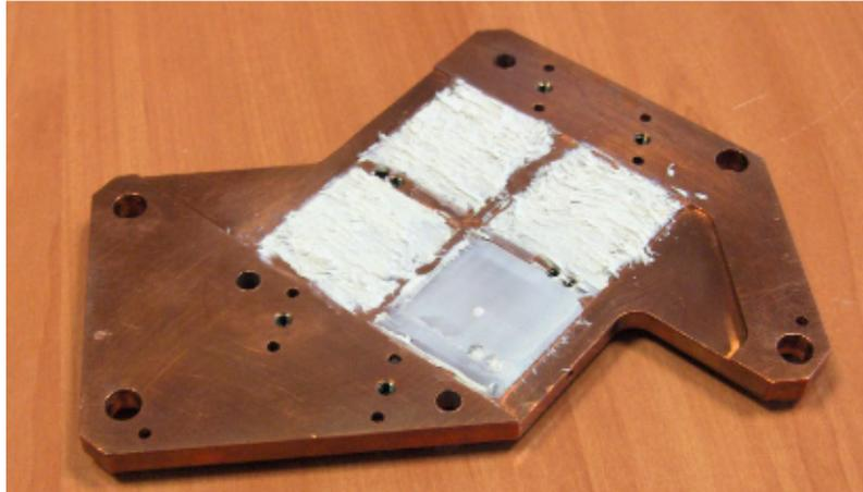
Figure 2.10 Application of the Thermal Grease on the Base Plate
