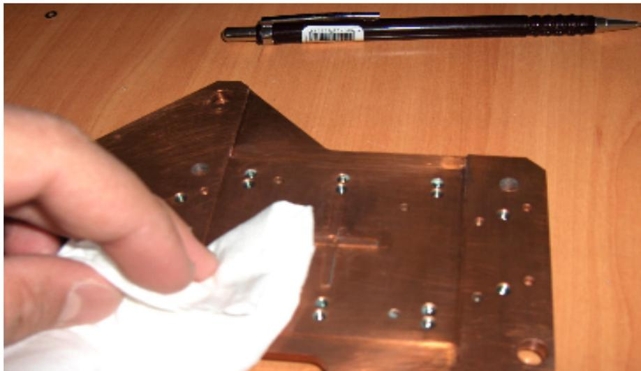
Figure 2.9 Cleaned and Degreased Base Plate
