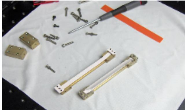
Figure 2.6 Laser Crystal Mounting Components
