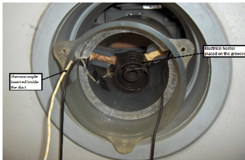
Figure 5.15 Mounted Thermocouple and Heater Component
