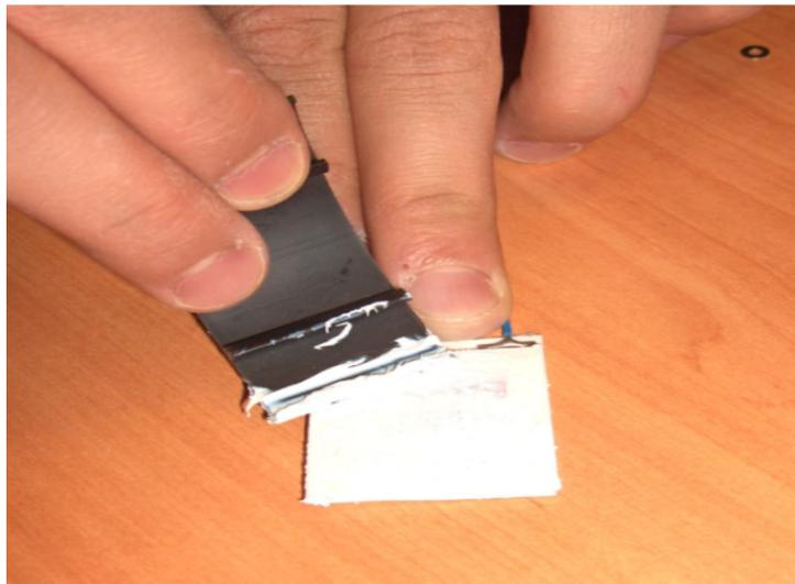
Figure 2.11 Application of the Thermal Grease on the TEC Surface
