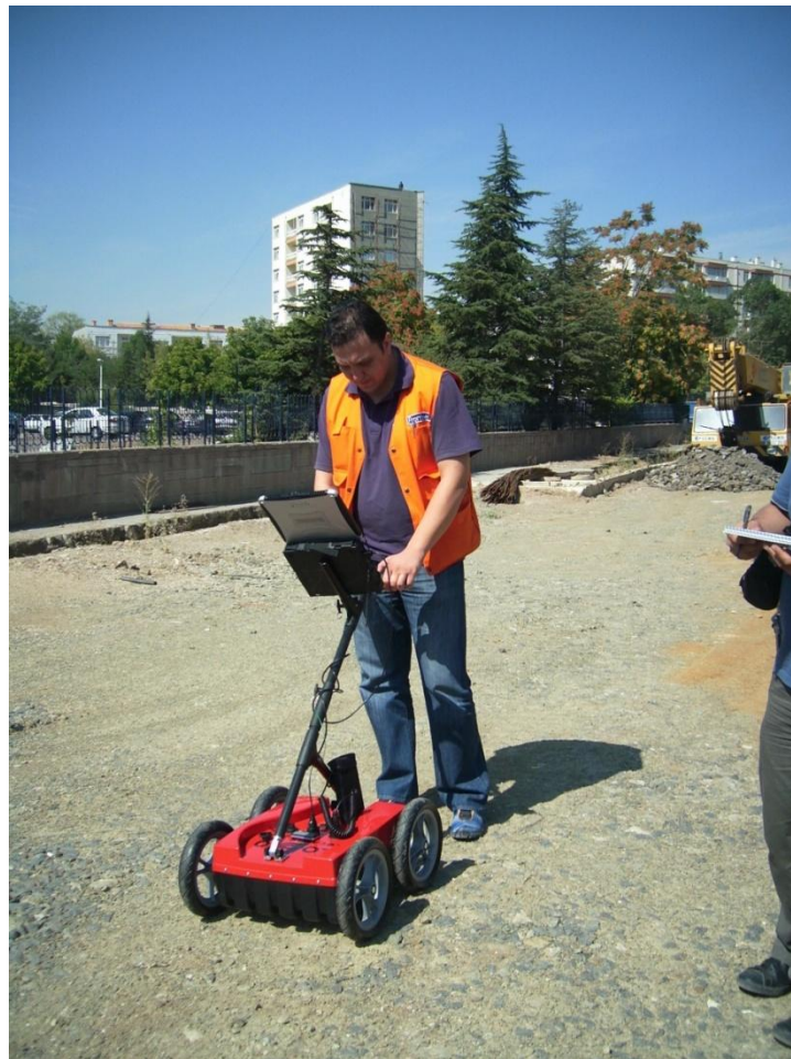
Figure 3.18. Cobra Locator GPR System produced by Radarteam Sweden AB.
