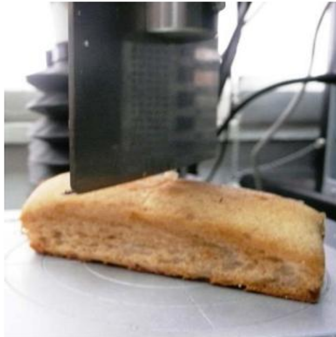
Figure 3.52 Experimental setup for cake cutting experiment
