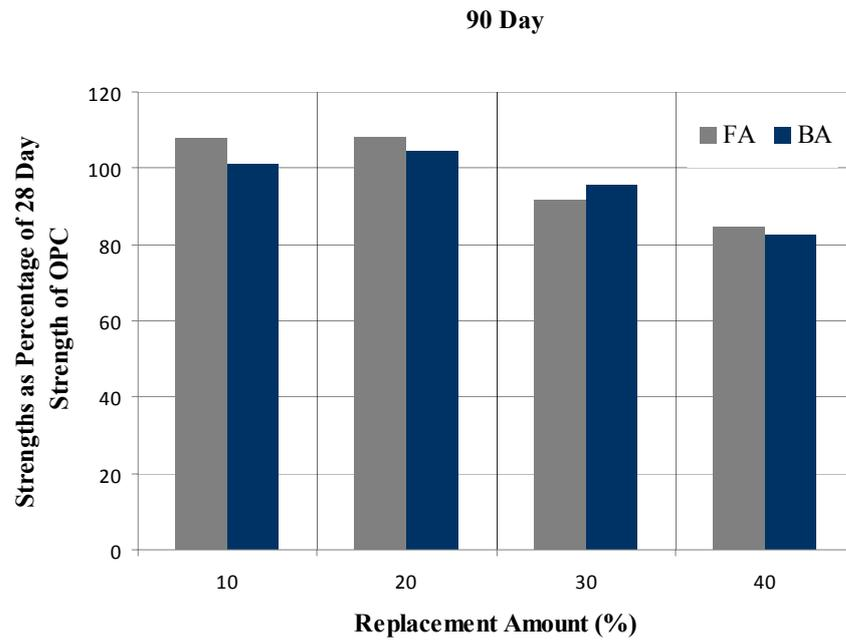
Figure 4.11 Compressive Strengths of Blended Cements at 90<sup>th</sup> Day as Percentage of Strength of OPC at 28<sup>th</sup> Day
