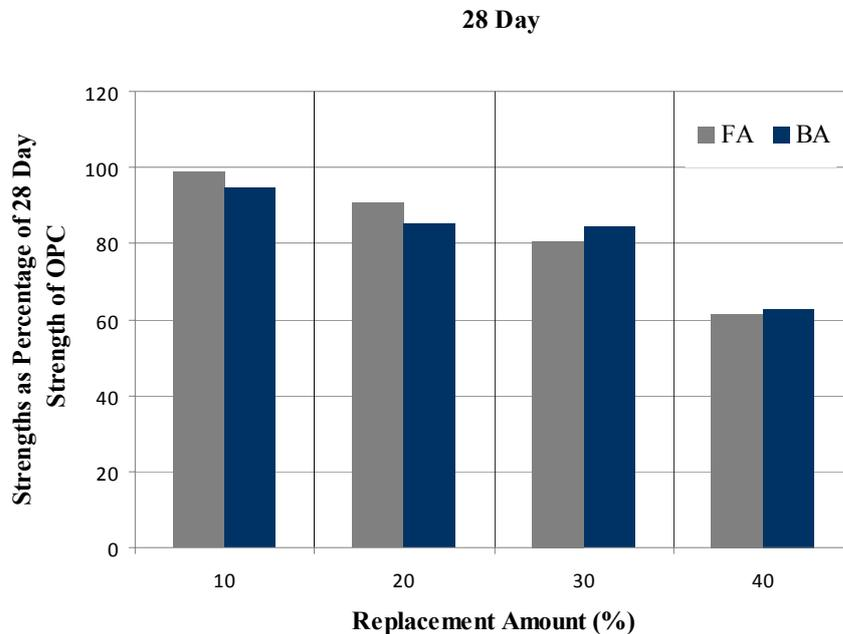
Figure 4.10 Compressive Strengths of Blended Cements at 28<sup>th</sup> Day as Percentage of Strength of OPC at 28<sup>th</sup> Day
