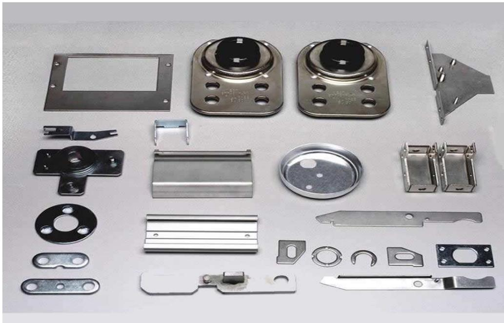
**Figure 1.1 Examples of Sheet Metal Products**
