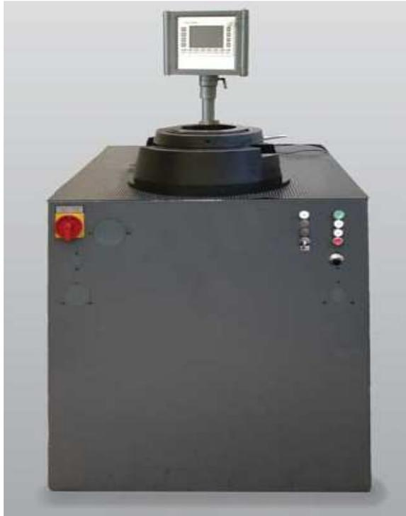
**Figure 6.2 Zwick-Roell Sheet Metal Testing Machine**
