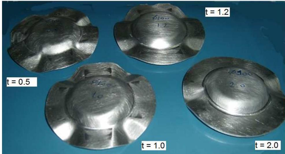
**Figure 5.53 Wrinkling formations for 100 mm diameter blanks**
