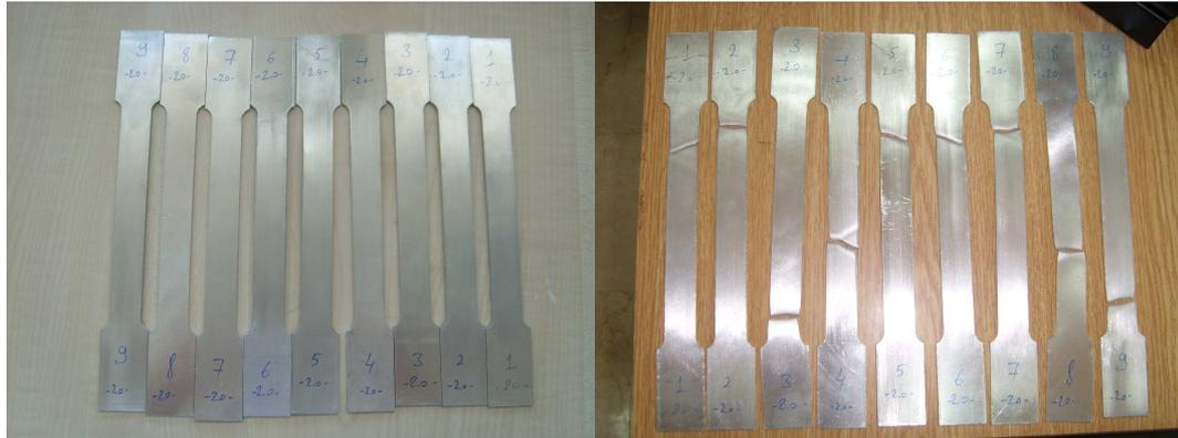
**Figure 5.49 Tension Test specimens, 2 mm thickness, before and after the test**
