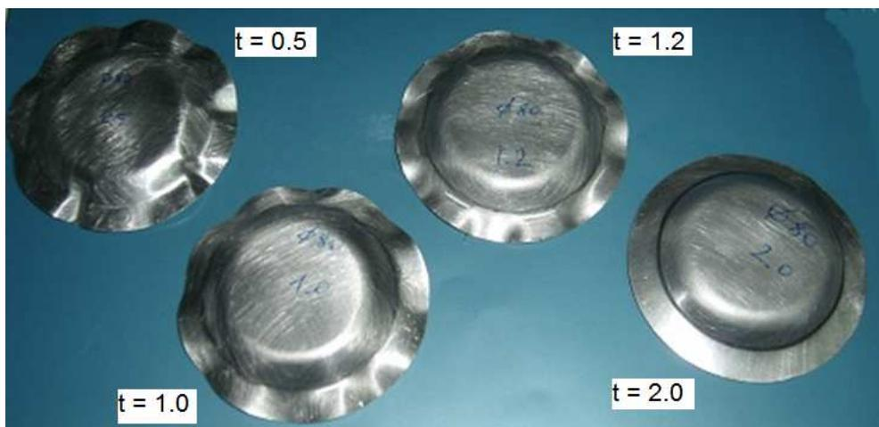
**Figure 5.52 Wrinkling formations for 80 mm diameter blanks**
