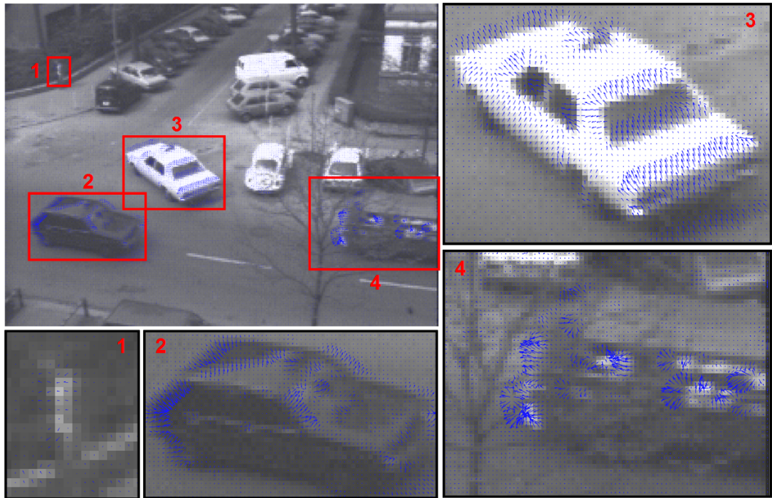
Figure 5.10: OF vectors computed on FPGA hardware for Hamburg Taxi sequence.
