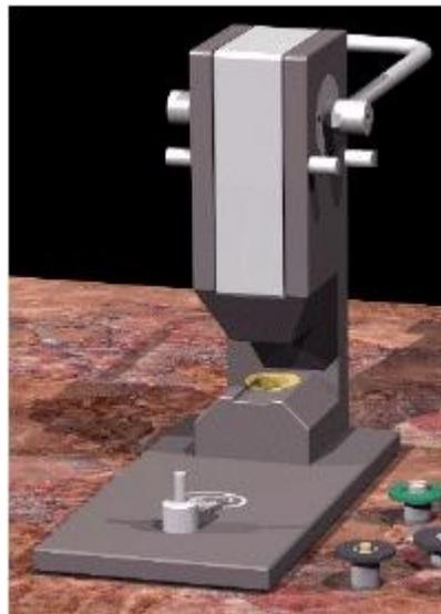
**Figure B.4:** Squeezing instrument of hermetic seal [56]
