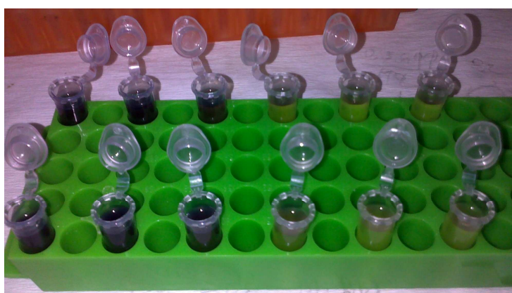
Figure 2.10 Absorbance of the samples (extract and DPPH) were read after 20 min of incubation period, at 517 nm.
