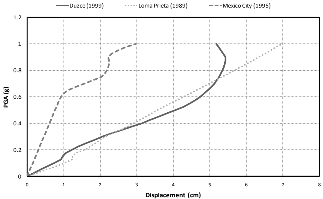
Figure 3.8. IDA curve for nonlinear system ( T_1=0.63\text{sec} , 5% strain hardening and \xi=5\% )
