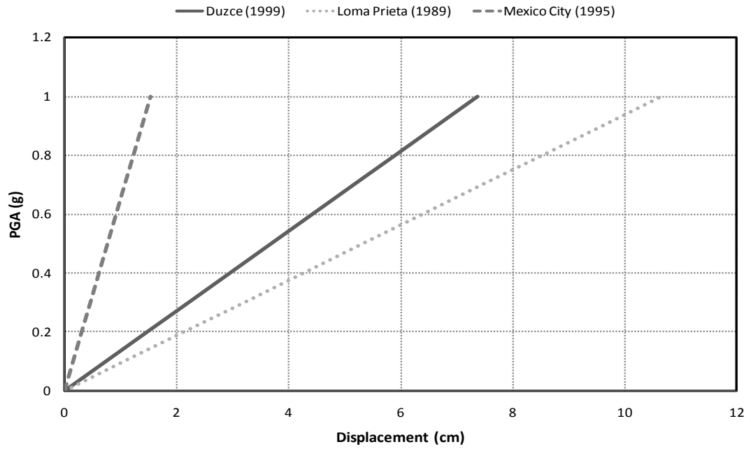
Figure 3.7. IDA curve for linear system ( T_1=0.63\text{sec} and \xi=5\% )
