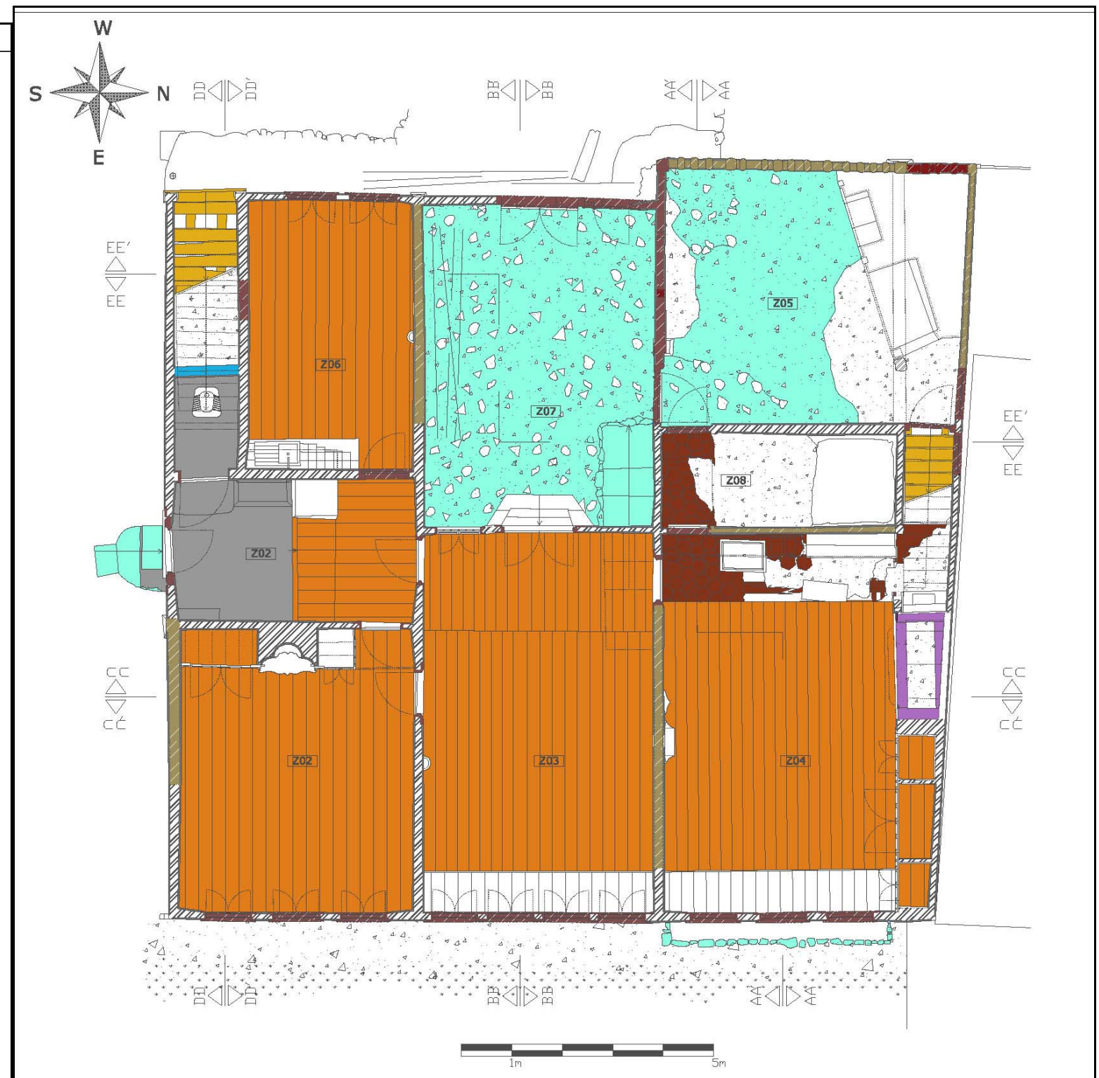
Figure 73: Analysis of Str. Syst. & Const. Tech.; Ground Floor Plan; Scale: 1/100 (presented in 1/50 at Jury)
