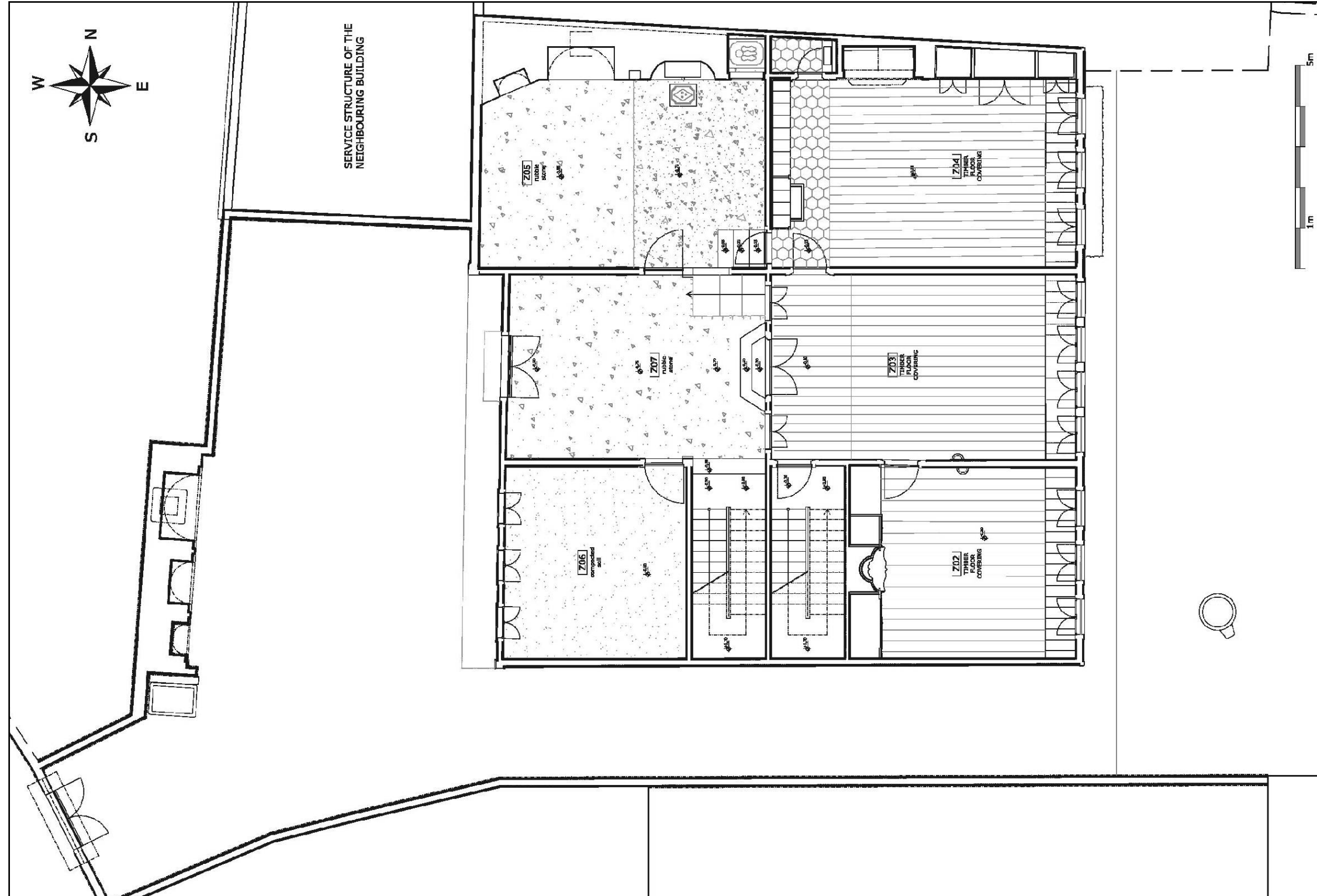
Figure 119: Restitution Phase I – Ground Floor Plan: 1/100 (Presented in 1/50 at Jury)
