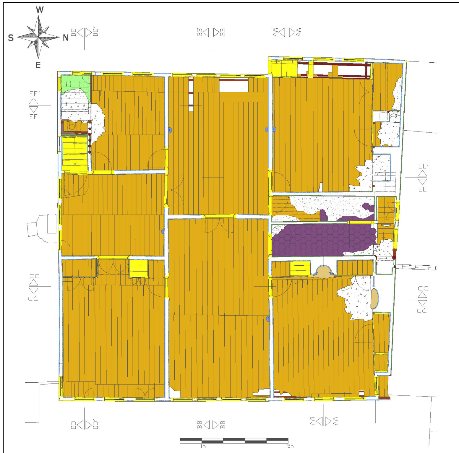
Figure 57: Analysis of Material-First Floor Plan; Scale: 1/100 (Presented in 1/50 at Jury)
