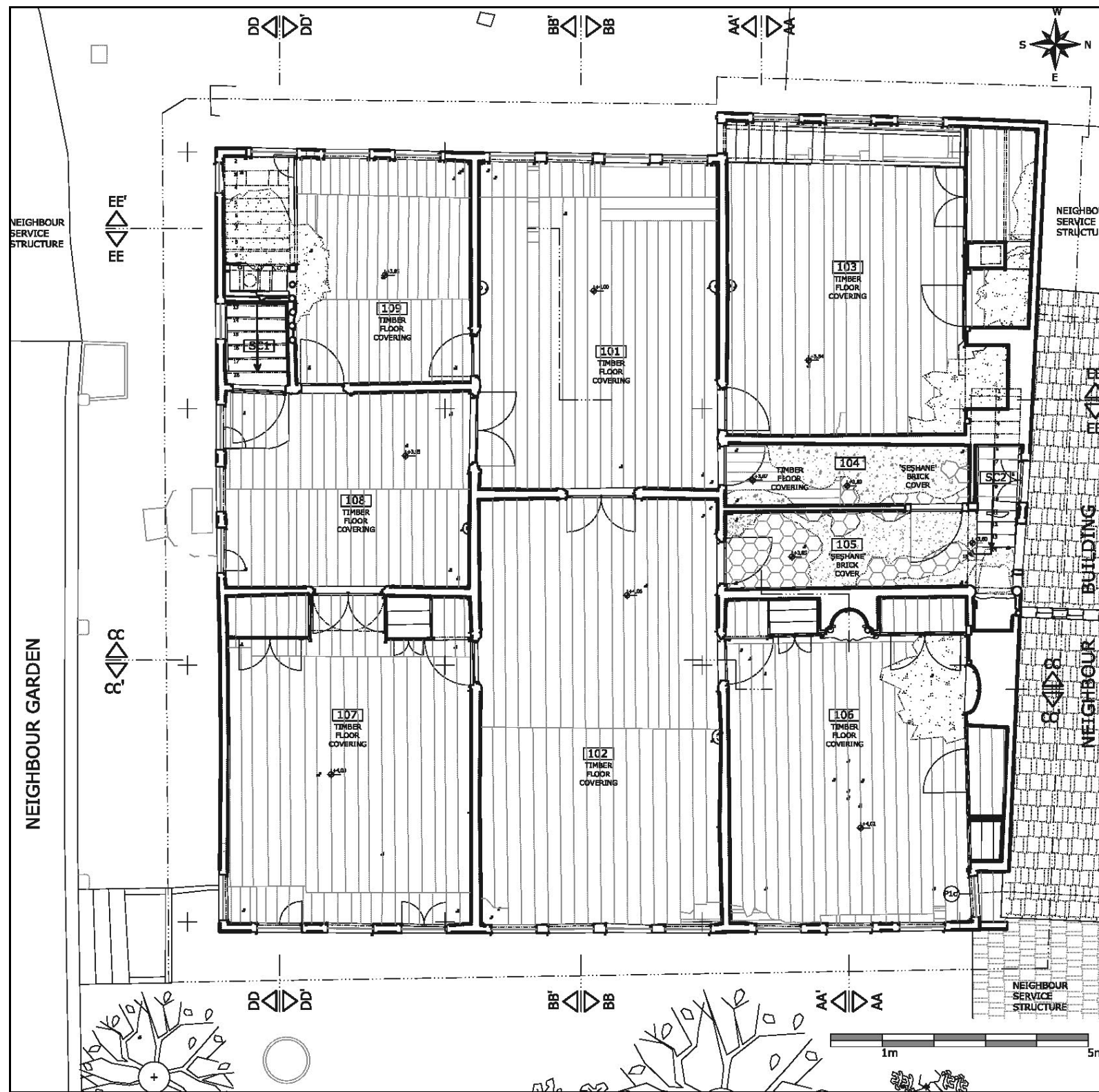
Figure 37: First Floor Flooring Plan: 1/100 (presented in 1/50 at Jury)
