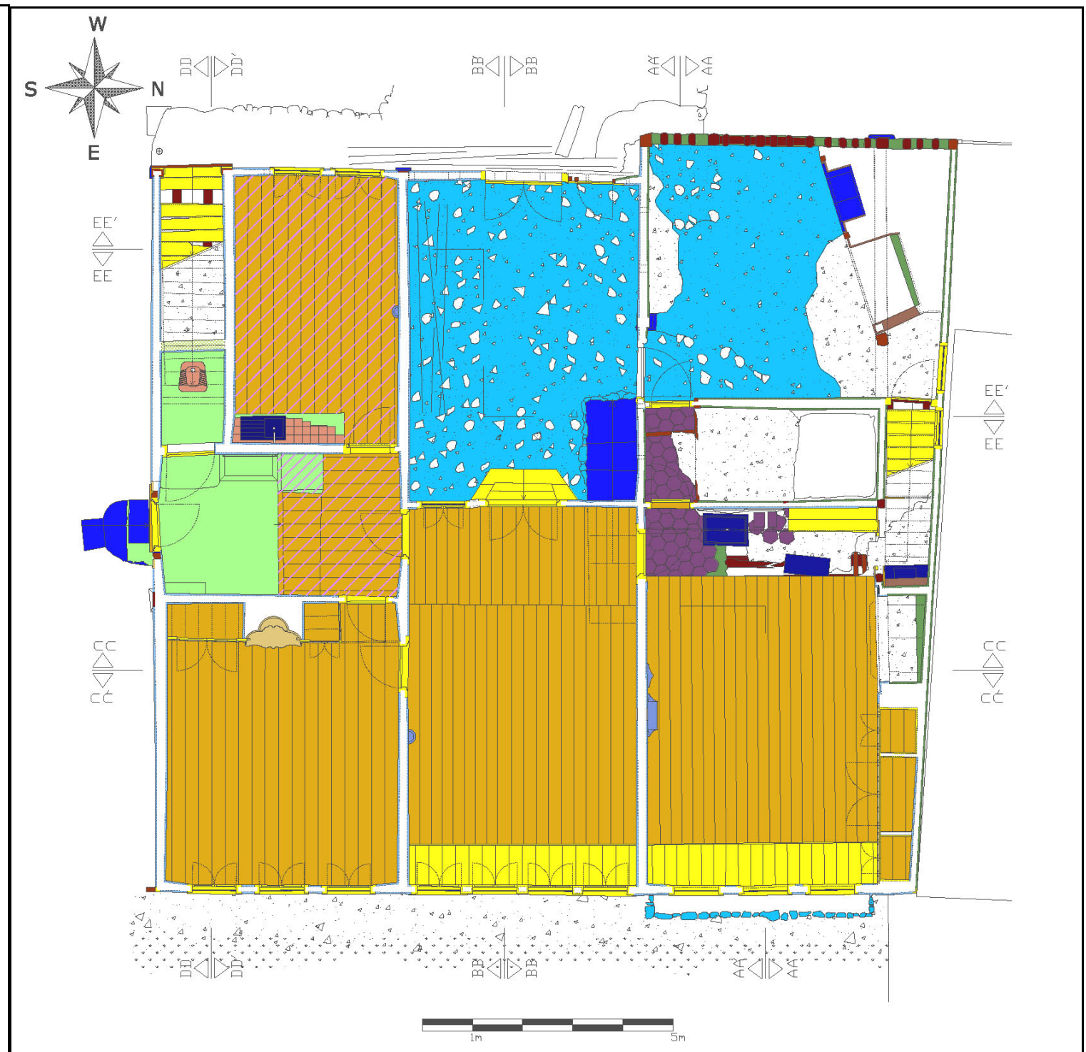
Figure 56: Analysis of Material-Ground Floor Plan; Scale: 1/100 (Presented in 1/50 at Jury)
