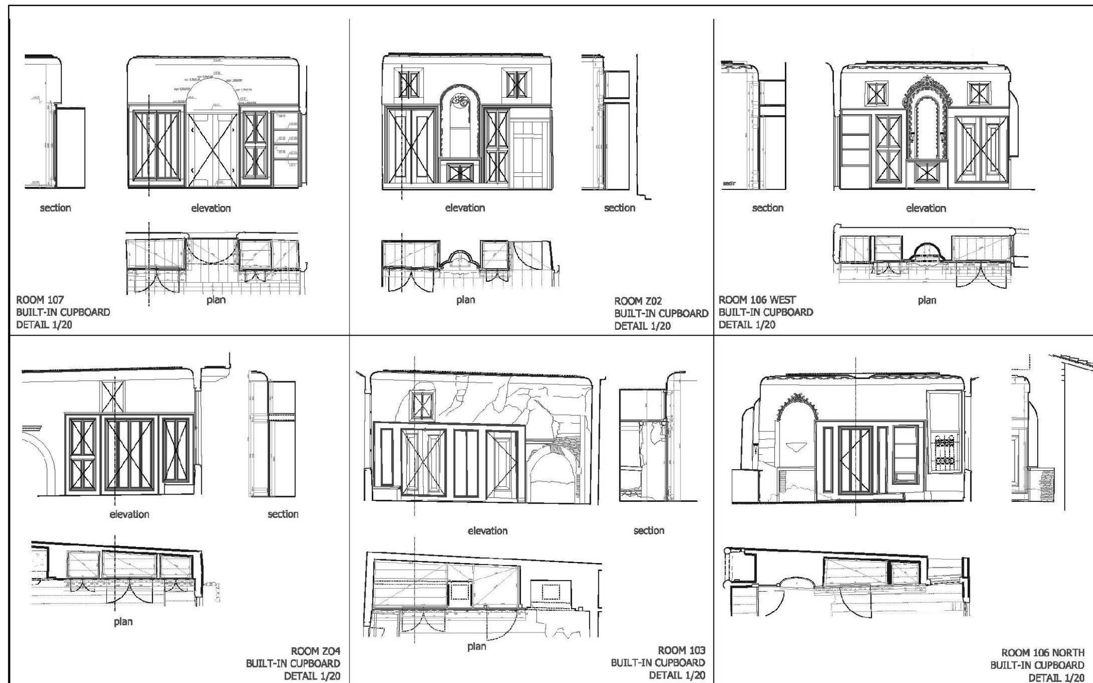
Figure 50: Details of Built-in Cupboards: scaled into 1/100 (presented in 1/20 at Jury)
