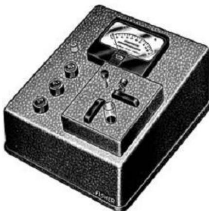
**Figure 1.6** The fluorometer to determine the quinine amount during World War II.
