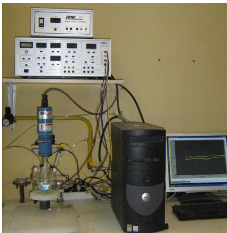
Figure 3.8 Experimental Setup for Cyclic Voltammetry
