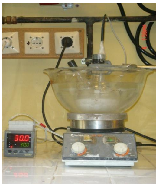
Figure 3.1 Experimental setup for SCMS silica synthesis
