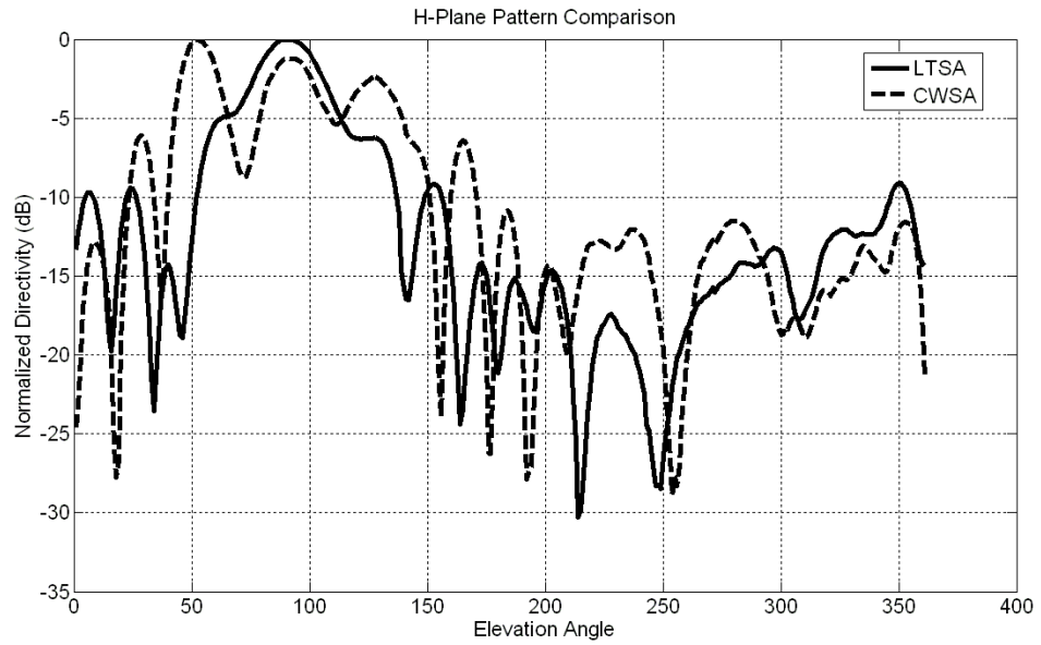
Figure 68 H-Plane Pattern Comparison of LTSA&CWSA with L=3\lambda_0 , W=1\lambda_0 and H=2\lambda_0
