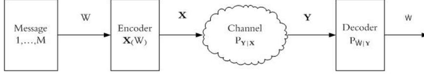
Figure 2.2: Channel model for a communication problem
