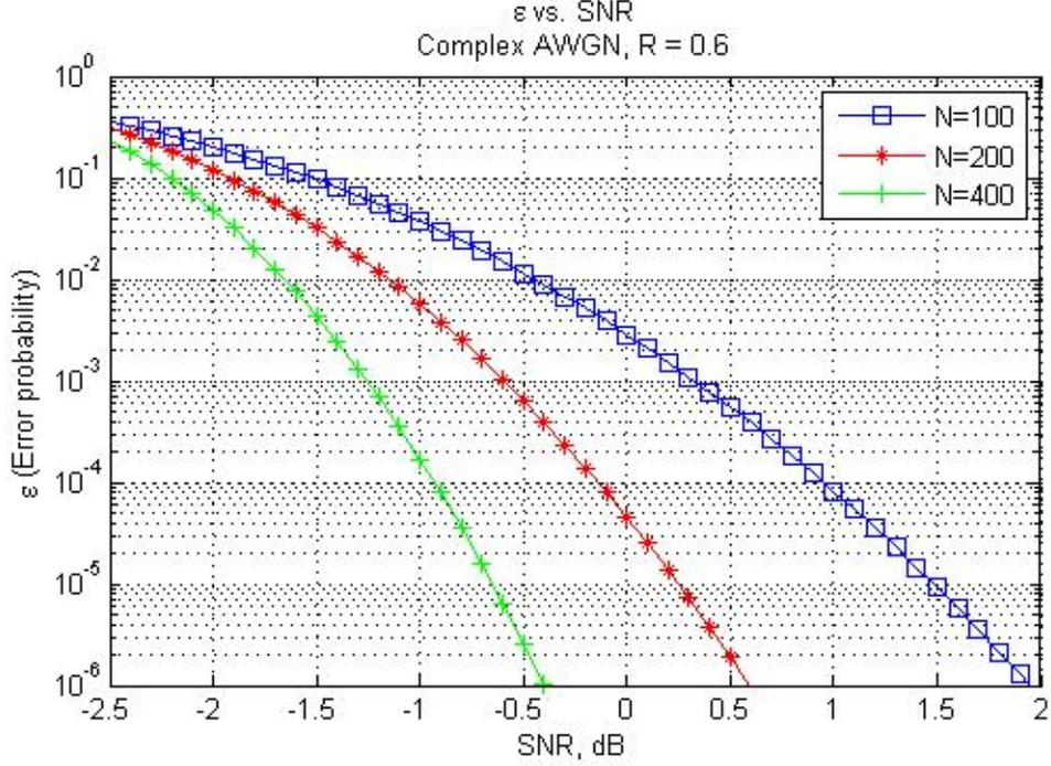
Figure 3.9: Error vs. SNR for Complex AWGN Channel
