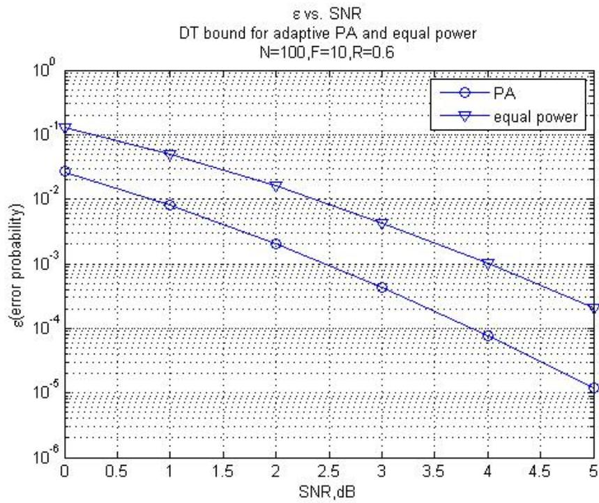
Figure 4.6: Comparison of DT bound for equal and adaptive power allocation,  $F = 10, N = 100$
