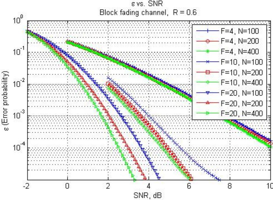
Figure 3.8: Error vs. SNR for Block Fading Channel
