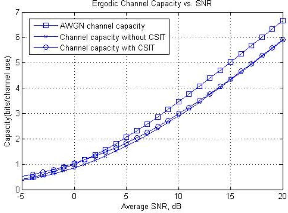
Figure 4.1: Ergodic Channel Capacity in Rayleigh fading
