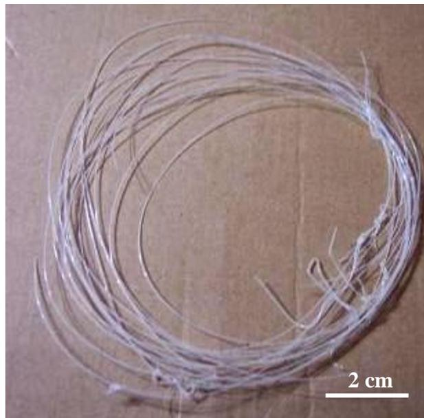
**Figure 3.10.** A ca. 2 m long continuous PHBV filament produced with capillary rheometer. Fiber diameter is 33  $\mu\text{m}$ , scale bar is 2 cm.
