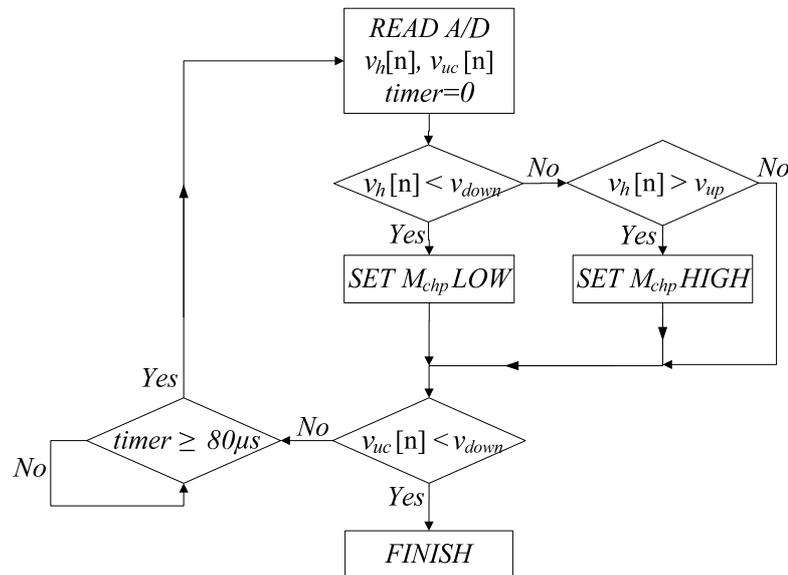
Figure 5.26 Program flow of the DC chopper control structure.
