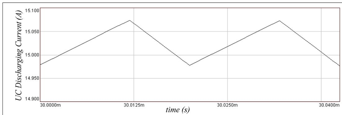
Figure 5.29 Simulation results for the steady-state ripple characteristics of the UC discharging current for a 15A current command considering the PI regulator case.
