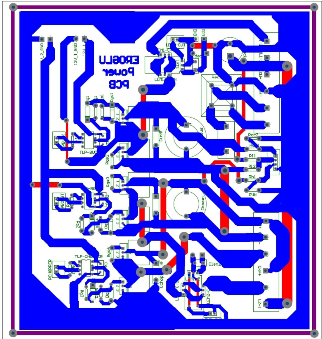
Figure C.2 Circuit layout of the power electronics converter board.
