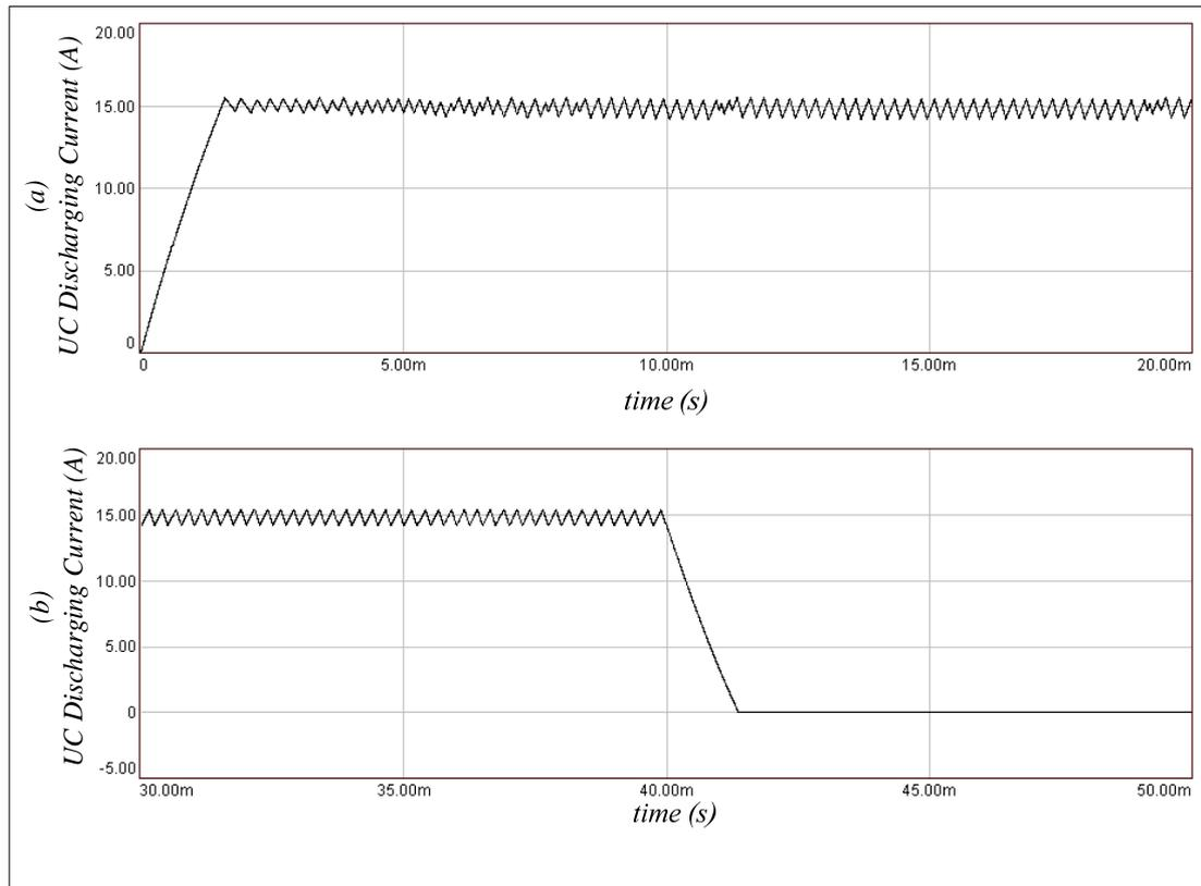
Figure 5.31 Simulation results for the dynamic response of the UC discharging current for a 15A current command considering the hysteresis regulator case:
