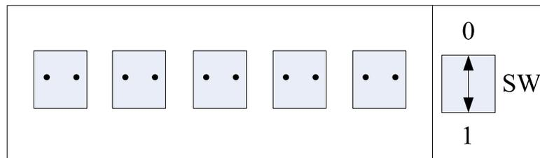
Figure F.4 Structure of the switched multiple sockets.
