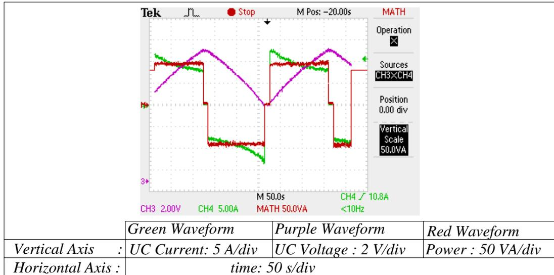
Figure 6.14 Variation of the UC module terminal voltage, applied current, and power for constant power tests.
