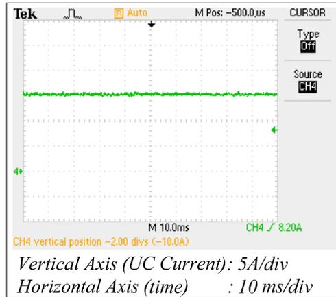
Figure 5.35 Experimental results for the steady-state UC discharging current for a 15A current command considering the PI regulator case.
