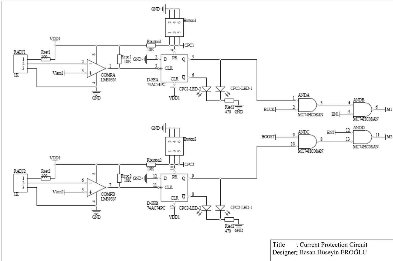
Figure B.3 Schematic diagram of the current protection circuit.
