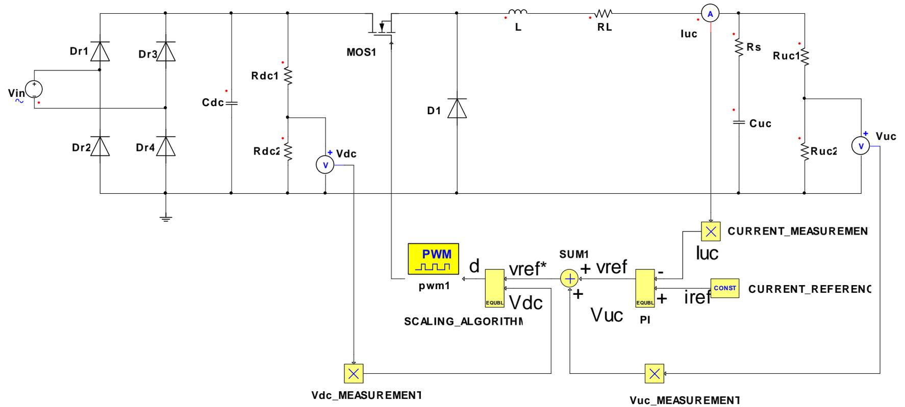
Figure 5.12 Simulation model of UC charging system.
