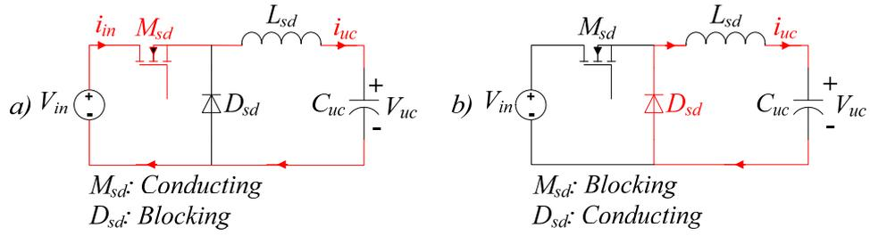
Figure 4.2 Operating modes of a step-down DC-DC converter based UC charger:
