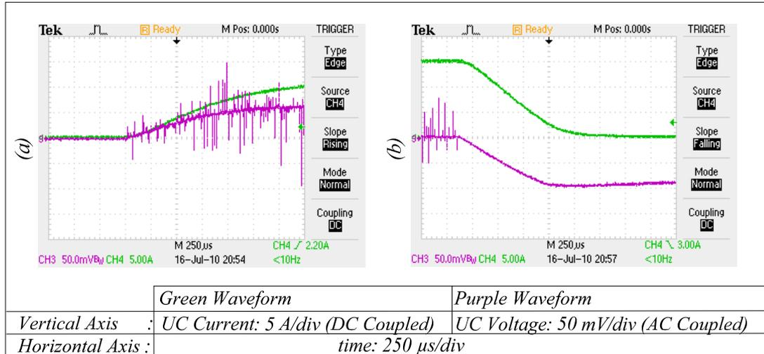
Figure 6.11 Immediate characteristics of the UC module terminal voltage for the charging phase: (a) AC coupled UC module terminal voltage at the beginning of the charging phase, (b) AC coupled UC module terminal voltage at the end of the charging phase.
