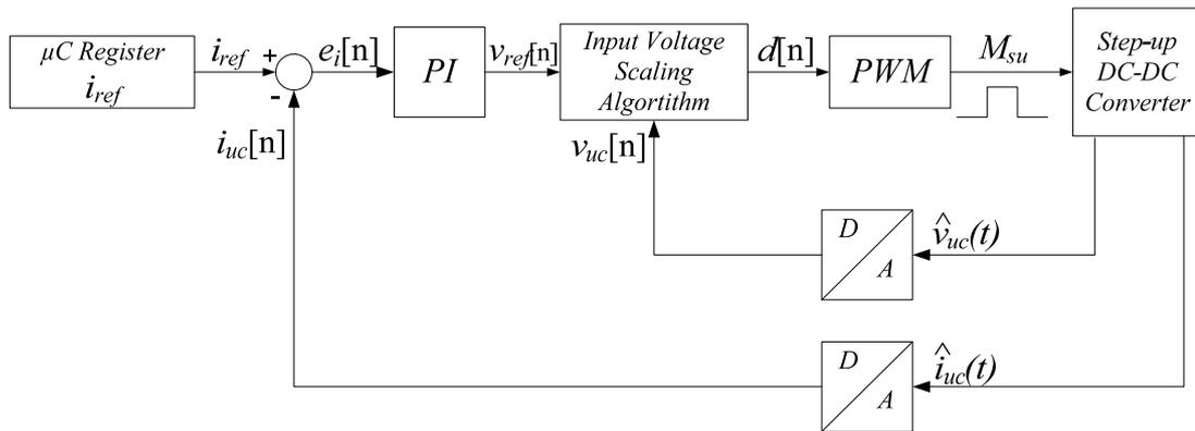
Figure 5.20 Block diagram of the microcontroller based UC discharging current regulator structure with a PI controller.
