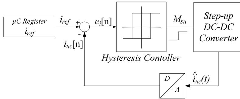
Figure 5.21 Block diagram of the microcontroller based UC discharging current regulator structure with a hysteresis controller.
