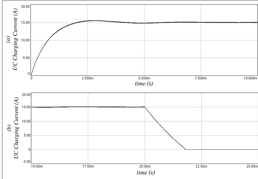
Figure 5.13 Simulation results for the dynamic response of the UC charging current for a 15A current command: (a) UC charging current build-up, (b) UC charging current fall.
