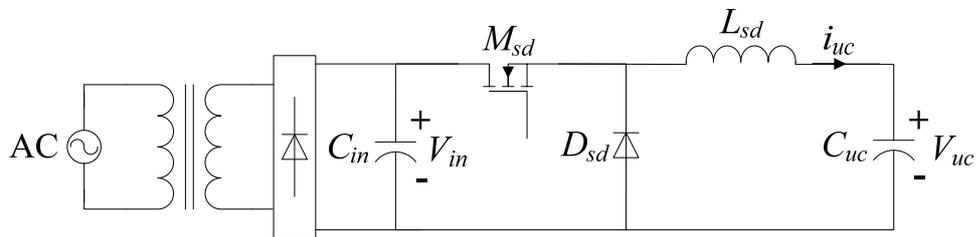
Figure 4.7 Schematic representation of a UC charger supplied by an unregulated DC supply.
