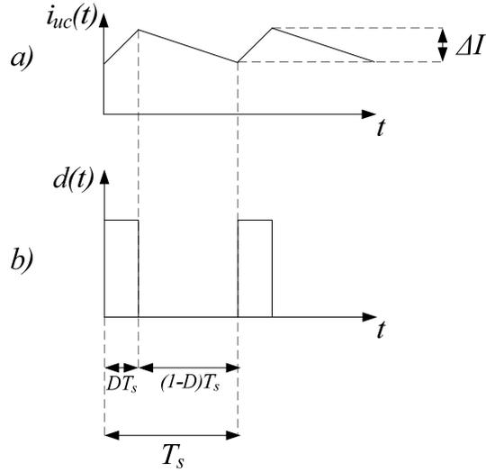
Figure 4.10 A typical steady-state discharging current waveform in CCM for PWM operation of step-up DC-DC converter based UC discharger: (a) discharging current waveform, (b) PWM signal.
