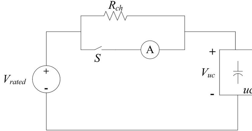
Figure 3.4 Schematic representation of a leakage current test circuit.
