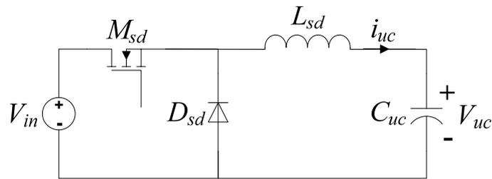
Figure 4.1 Schematic representation of a step-down DC-DC converter based UC charger.
