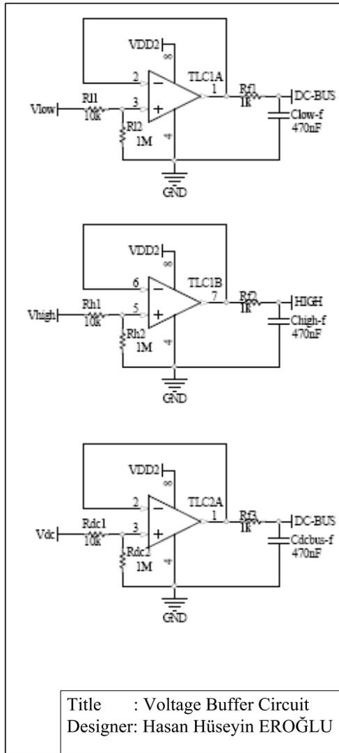
Figure B.4 Schematic diagram of the voltage buffer circuit.
