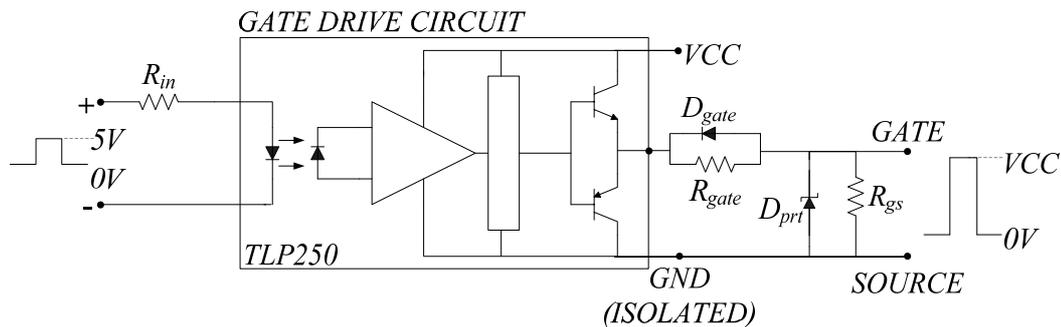
Figure 5.3 Schematic diagram of the gate drive circuit.
