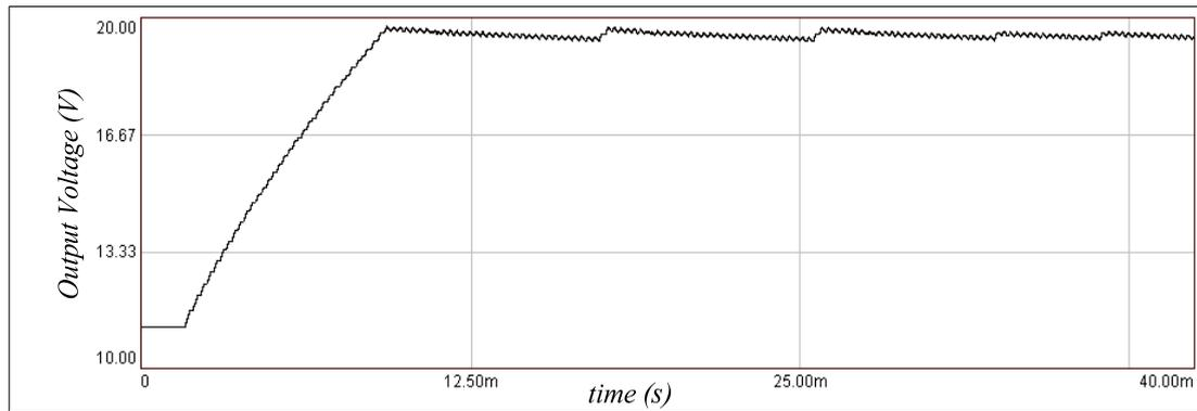
Figure 5.33 Simulation results for the output voltage characteristics of the UC discharging system for a 19.5V set voltage command considering the hysteresis regulator case.
