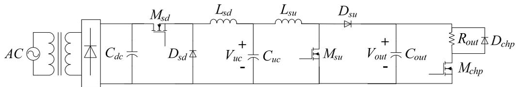
Figure 4.17 Schematic representation of the power electronics converter structure for a loss mechanism based UC test system.
