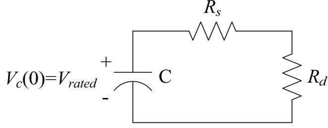
Figure 2.2 Electrical equivalent circuit of a capacitor in discharging mode.
