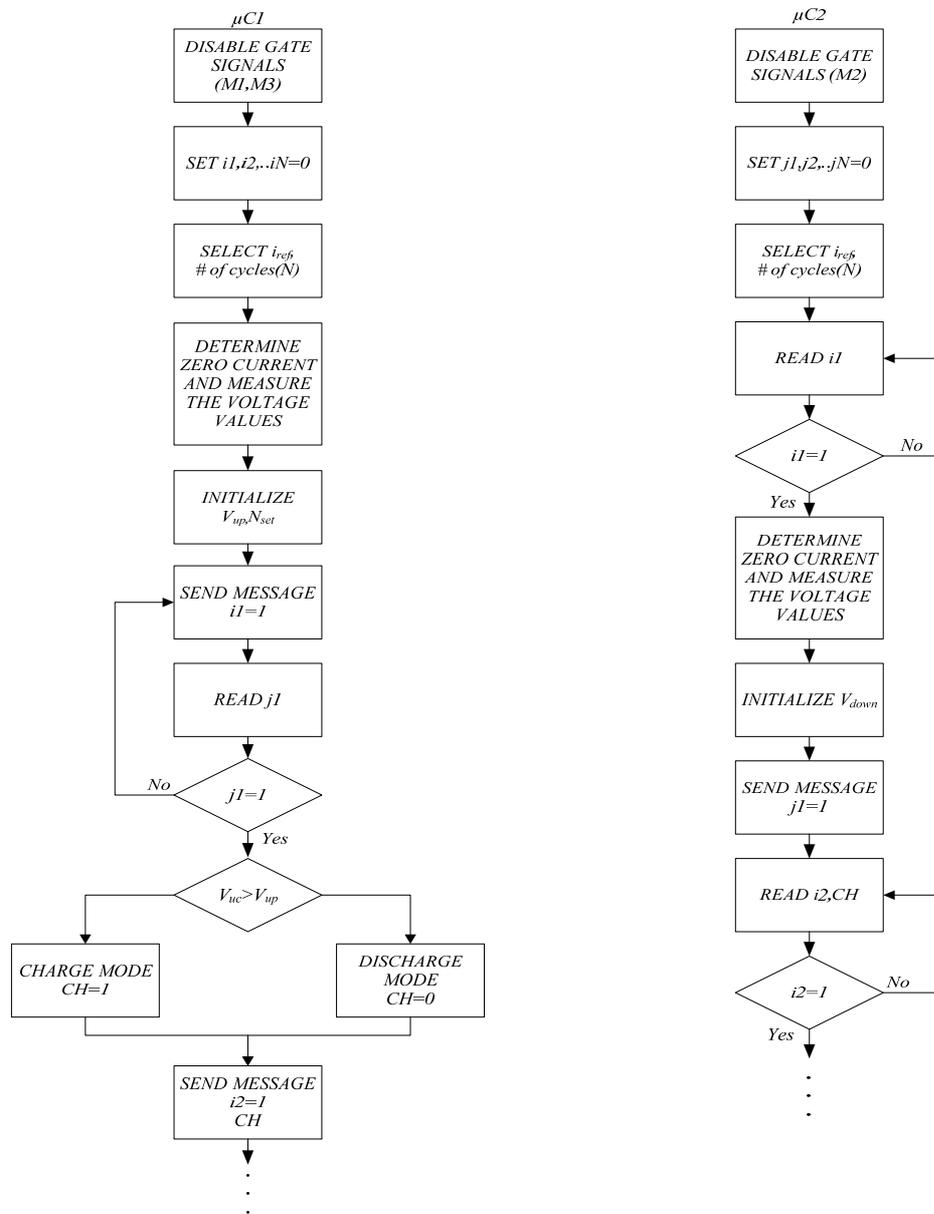
Figure E.1 Software structure of the UC test system (Part 1).
