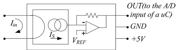
Figure 5.5 Schematic diagram of the current measurement circuit [52].
