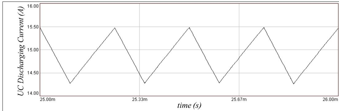
Figure 5.32 Simulation results for the steady-state ripple characteristics of the UC discharging current for a 15A current command considering the hysteresis regulator case.
