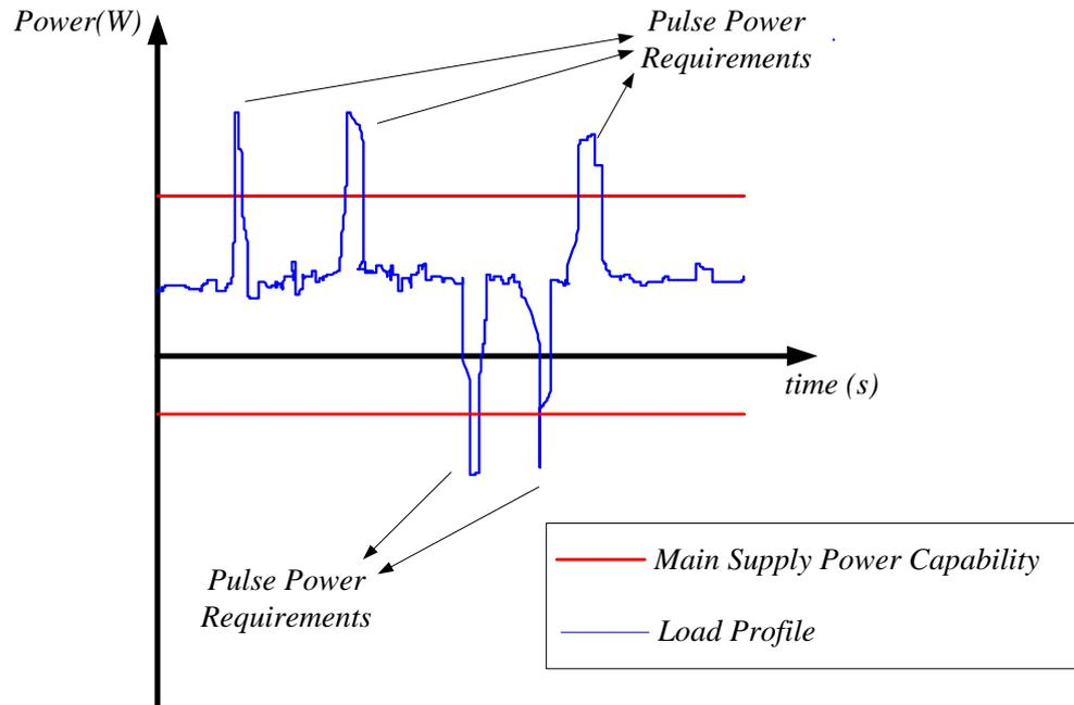
Figure 2.13 A typical load profile with pulse power requirements.
