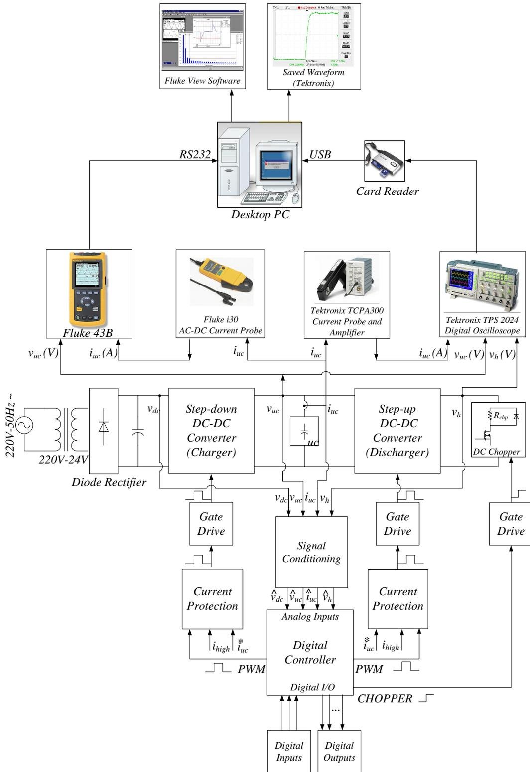
Figure 5.1 Structural diagram of a microcontroller based UC test system.
