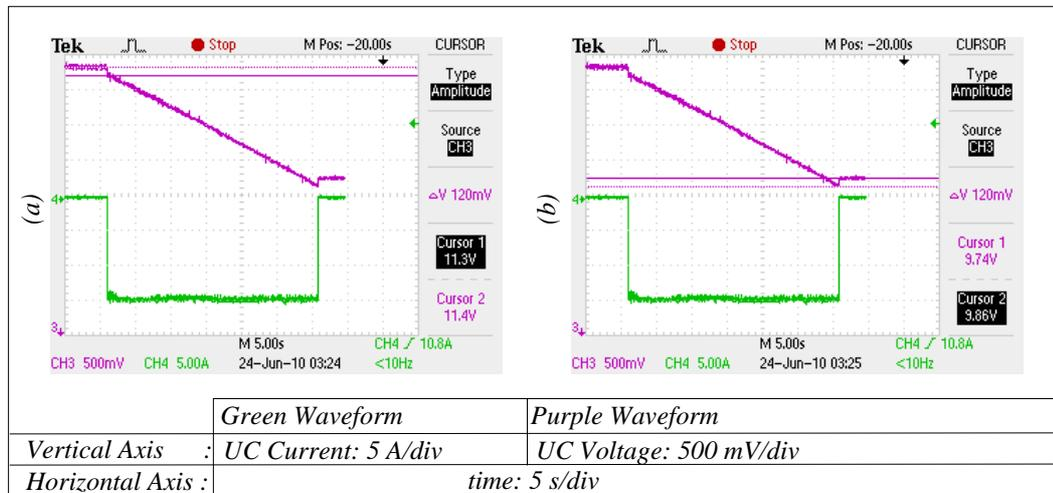
Figure 6.10 Immediate characteristics of the UC module terminal voltage for the discharging phase: (a) measurement of the decrease of the UC module terminal voltage with purple colored voltage cursors at the beginning of the discharging phase, (b) measurement of the increase of the UC module terminal voltage with purple colored voltage cursors at the end of the discharging phase.
