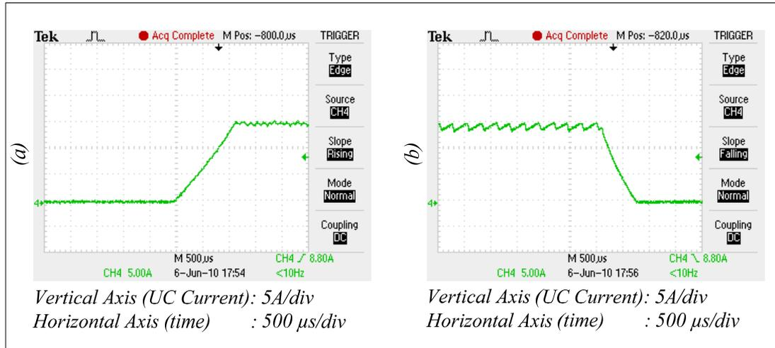
Figure 5.38 Experimental results for the dynamic response of the UC discharging current for a 15A current command considering the hysteresis regulator case:
