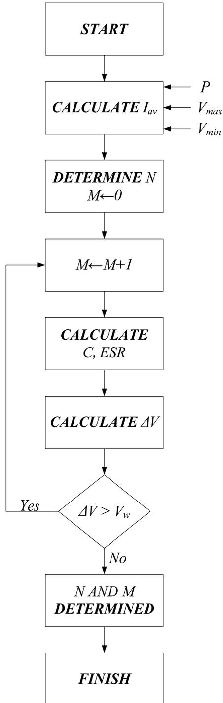
Figure 2.10 Flowchart of a UC module sizing algorithm.
