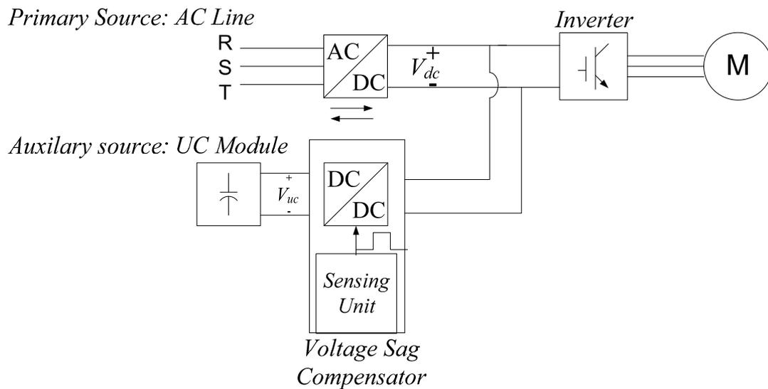
Figure 2.16 Block diagram of a UC assisted riding through system.
