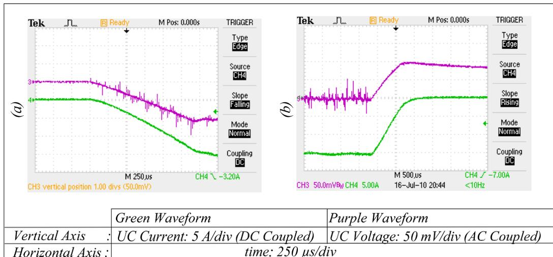
Figure 6.12 Immediate characteristics of the UC module terminal voltage for the discharging phase: (a) AC coupled UC module terminal voltage at the beginning of the discharging phase, (b) AC coupled UC module terminal voltage at the end of the discharging phase.
