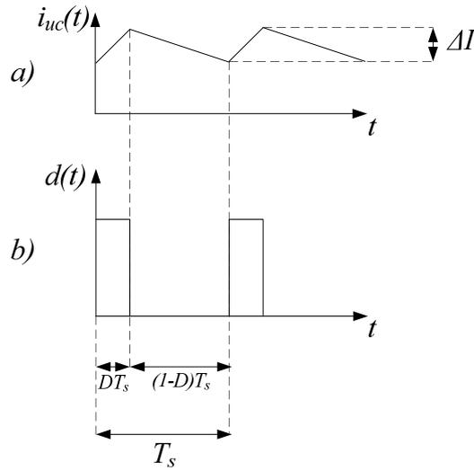
Figure 4.3 A typical steady-state charging current waveform of a step-down DC-DC converter based UC charger in CCM: (a) charging current waveform, (b) PWM signal.
