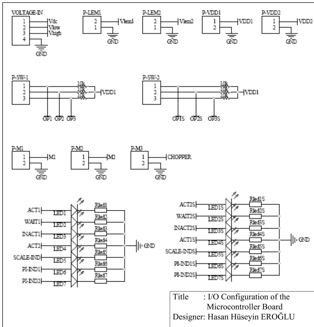
Figure B.1 Schematic diagram of the I/O configuration of the microcontroller board.
