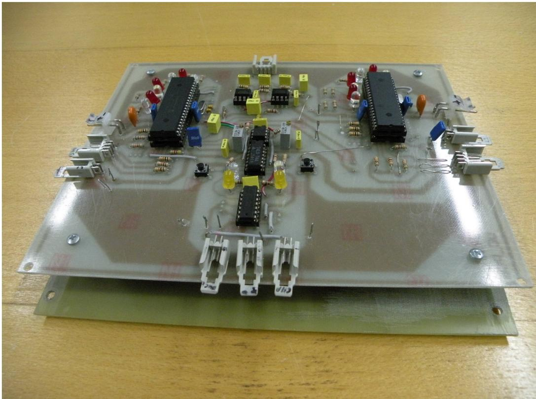
Figure D.1 Photograph of the microcontroller board.
