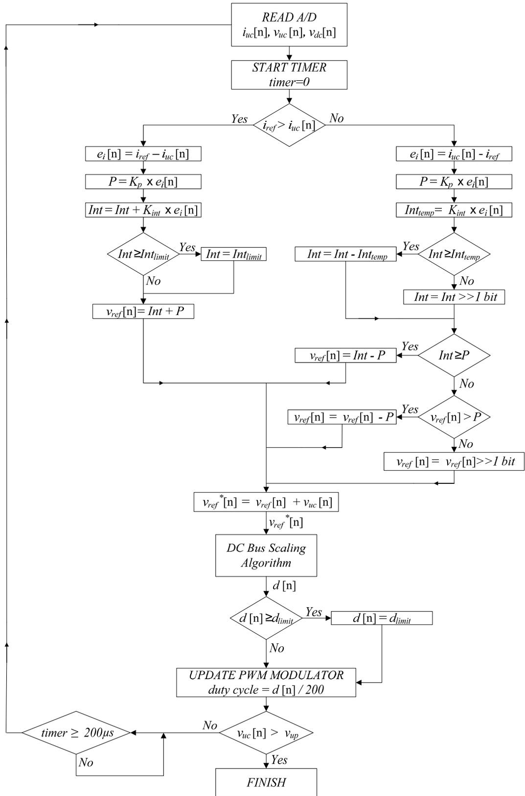
Figure 5.11 Program flow of the UC charging process.
