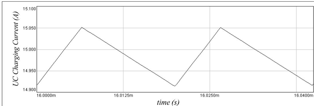
Figure 5.14 Simulation results for the steady-state ripple characteristics of the UC charging current for a 15A current command.
