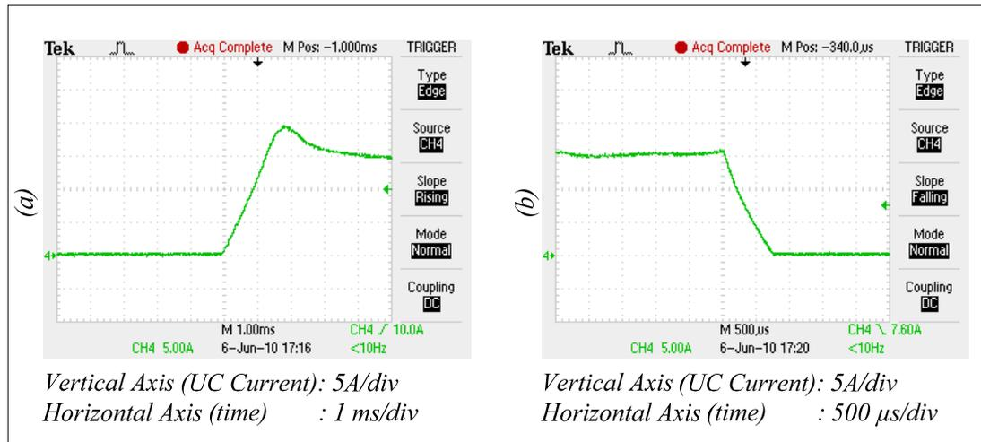
Figure 5.34 Experimental results for the dynamic response of the UC discharging current for a 15A current command considering the PI regulator case:
