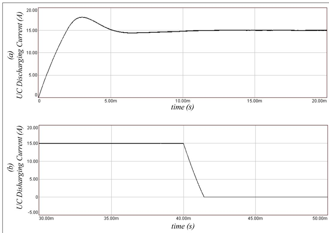
Figure 5.28 Simulation results for the dynamic response of the UC discharging current for a 15A current command considering the PI regulator case:
