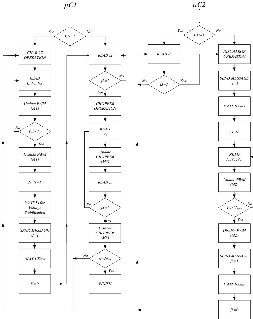
Figure E.2 Software structure of the UC test system (Part 2).
