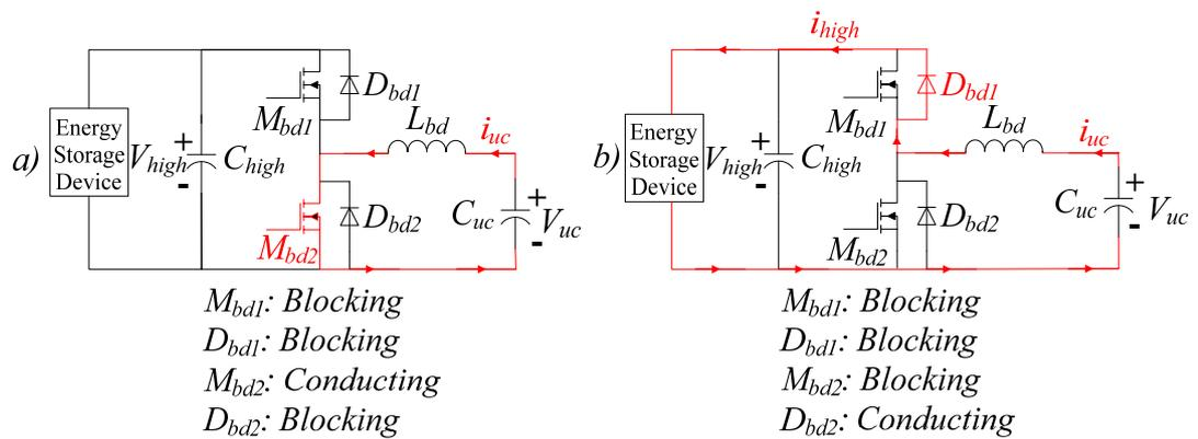
Figure 4.16 Operating modes of a bi-directional DC-DC converter for the discharging phase of the UC: (a)  $M_{bd2}$  is in conduction mode, (b)  $M_{bd2}$  is in blocking mode.
