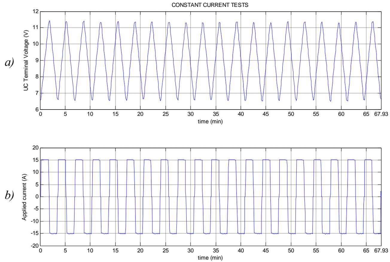
Figure 6.5 Long term variation of the UC module for constant current tests: (a) terminal voltage variation of the UC module, (b) applied current variation.
