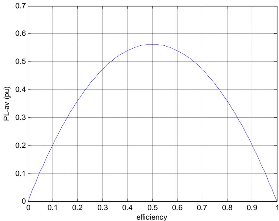
Figure 2.3 Variation of average load power with respect to discharge efficiency.
