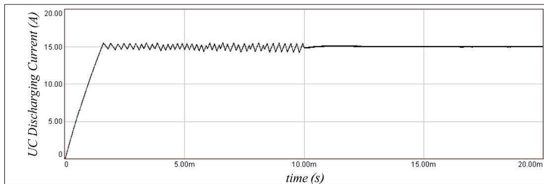
Figure 5.42 Simulation results of the UC discharging system with a hybrid controller structure for a 15A current command.
