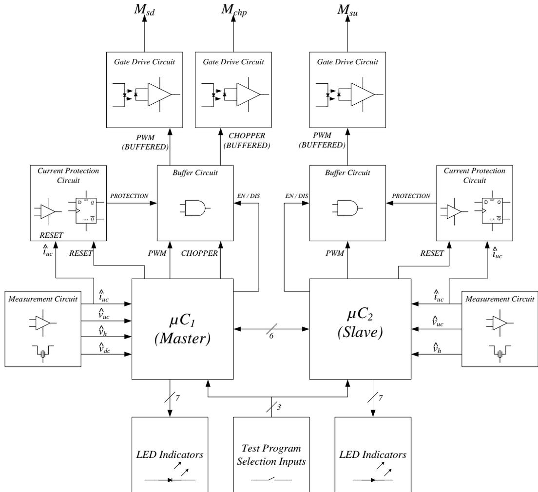
Figure 5.8 I/O diagram of microcontroller based digital controller.
