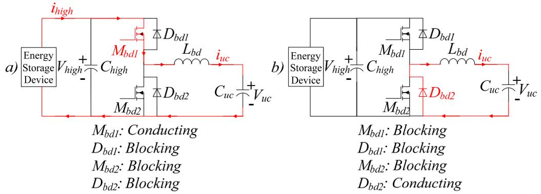
Figure 4.15 Operating modes of a bi-directional DC-DC converter for the charging phase of the UC: (a)  $M_{bd1}$  is in conduction mode, (b)  $M_{bd1}$  is in blocking mode.
