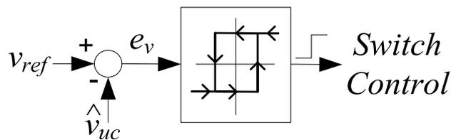
Figure 2.12 Block diagram of switched resistor control structure.
