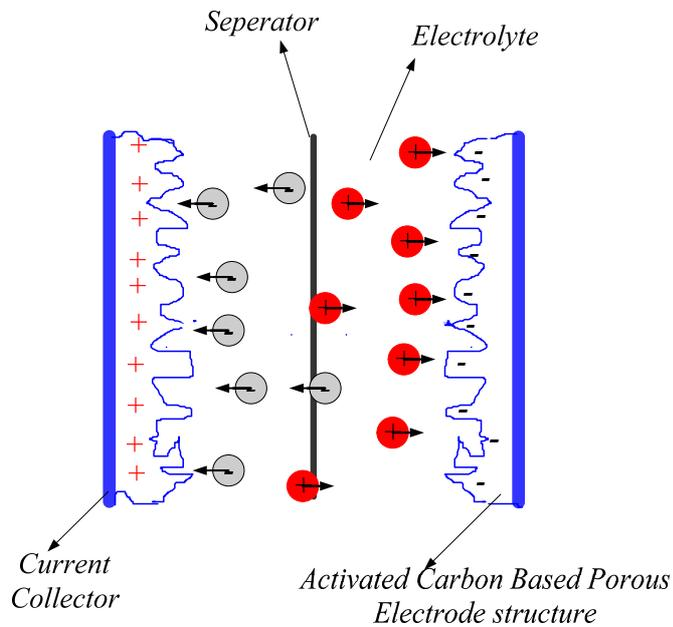
Figure 2.6 Internal structure of a UC [8].
