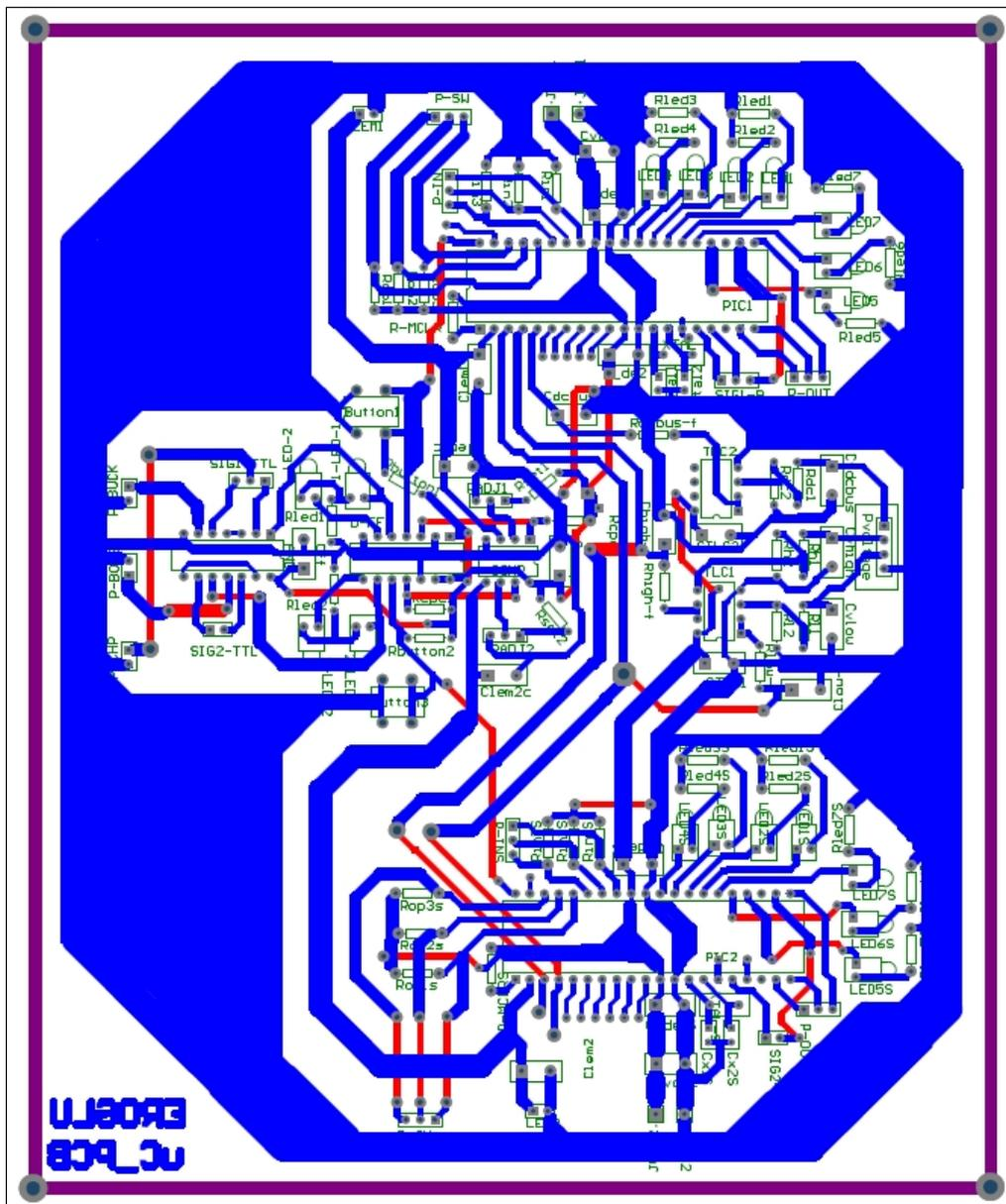
Figure C.1 Circuit layout of the microcontroller board.
