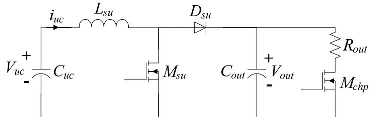
Figure 4.12 Schematic representation of a step-up DC-DC converter based UC charger with a chopper structure.
