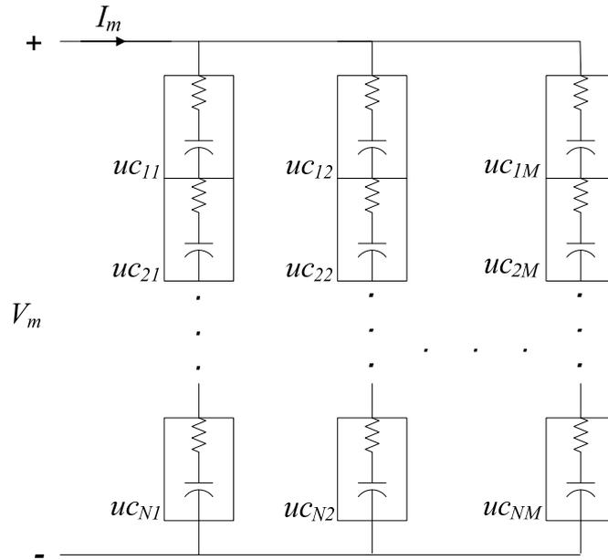
Figure 2.9 Schematic representation of an  $N \times M$  matrix formed UC module.
