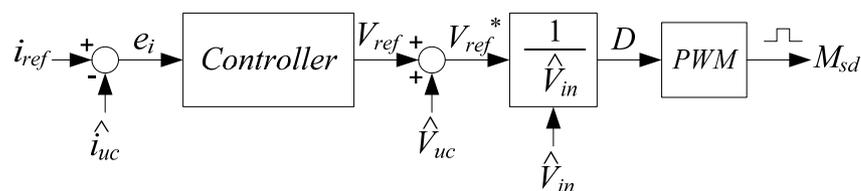
Figure 4.6 Block diagram of a current control structure for a UC charger.
