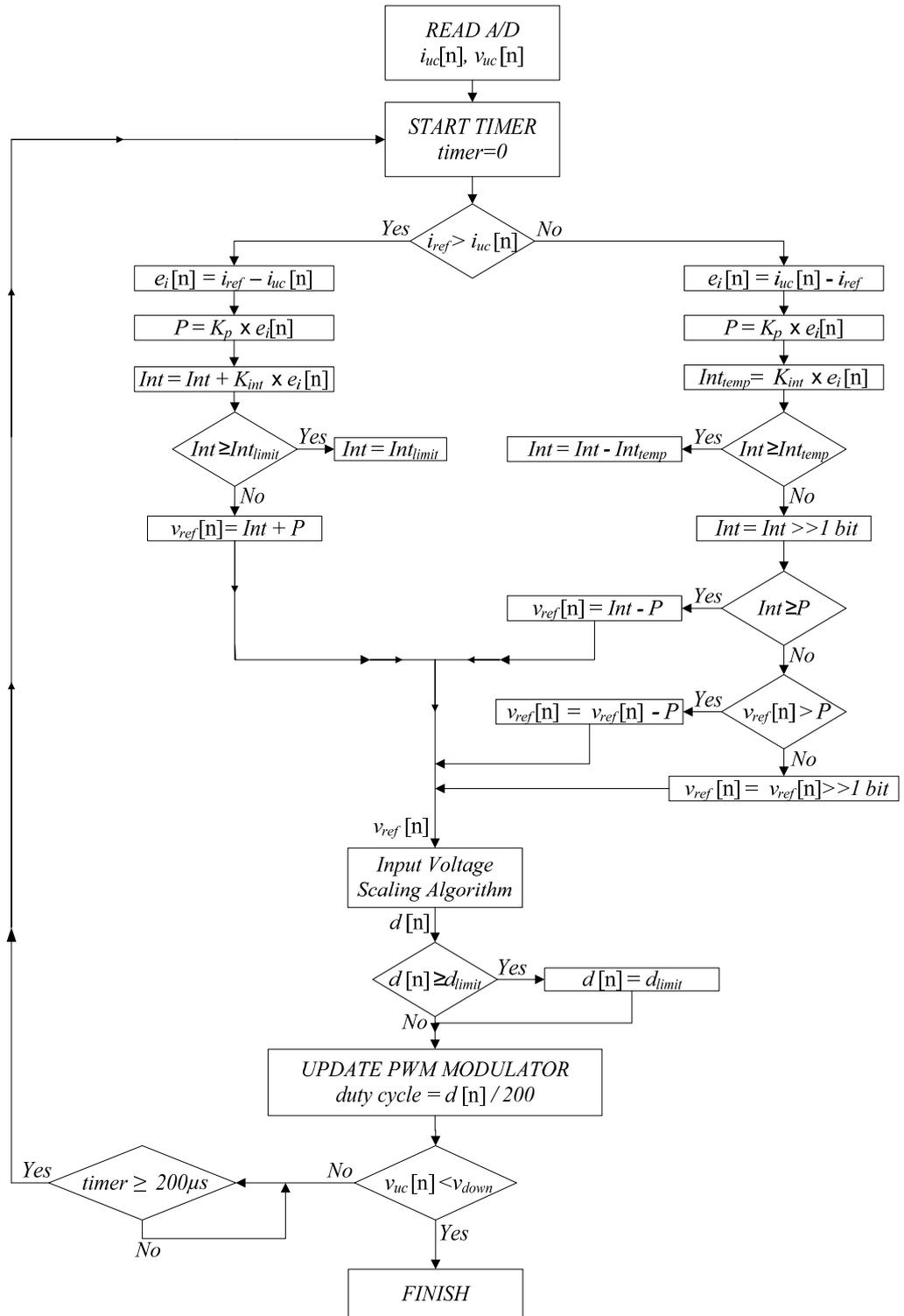
Figure 5.24 Program Flow of the UC discharging current regulator structure with a PI controller.
