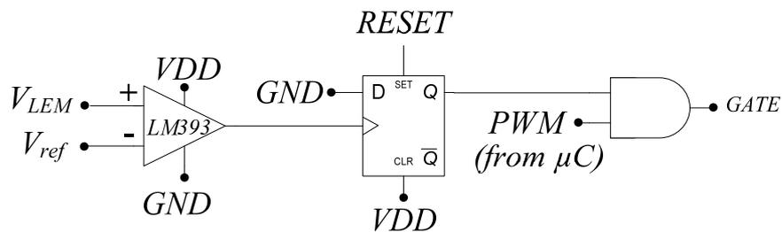
Figure 5.7 Schematic diagram of the current protection circuit.
