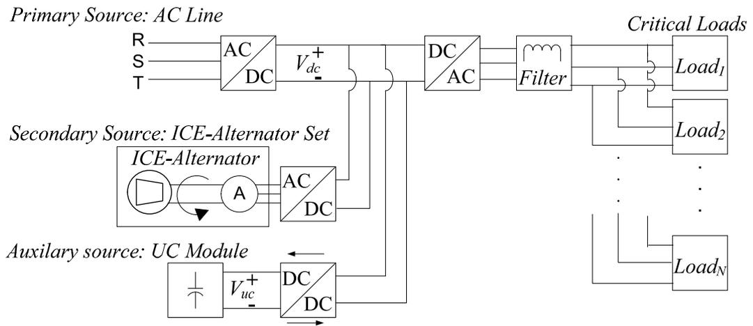
Figure 2.15 Block diagram of a UC assisted UPS application [35].
