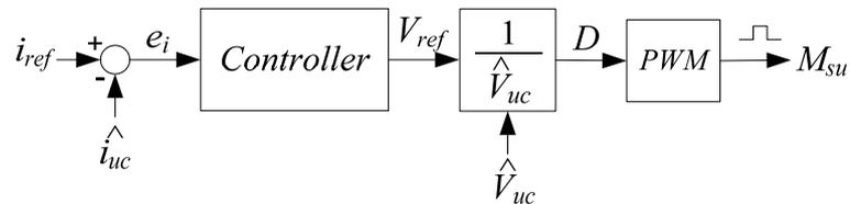
Figure 4.11 Block diagram of a current control structure for a UC discharger.
