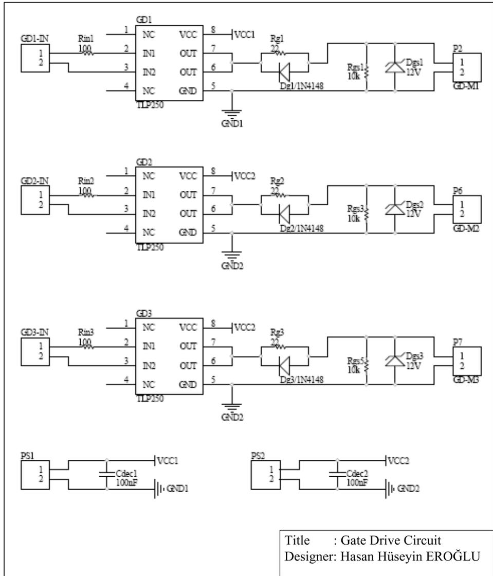
Figure B.6 Schematic diagram of the gate drive circuit.
