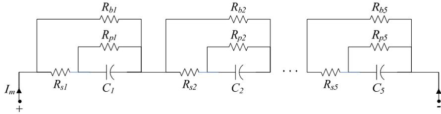
Figure 5.16 Schematic representation of the UC module utilized in the study.
