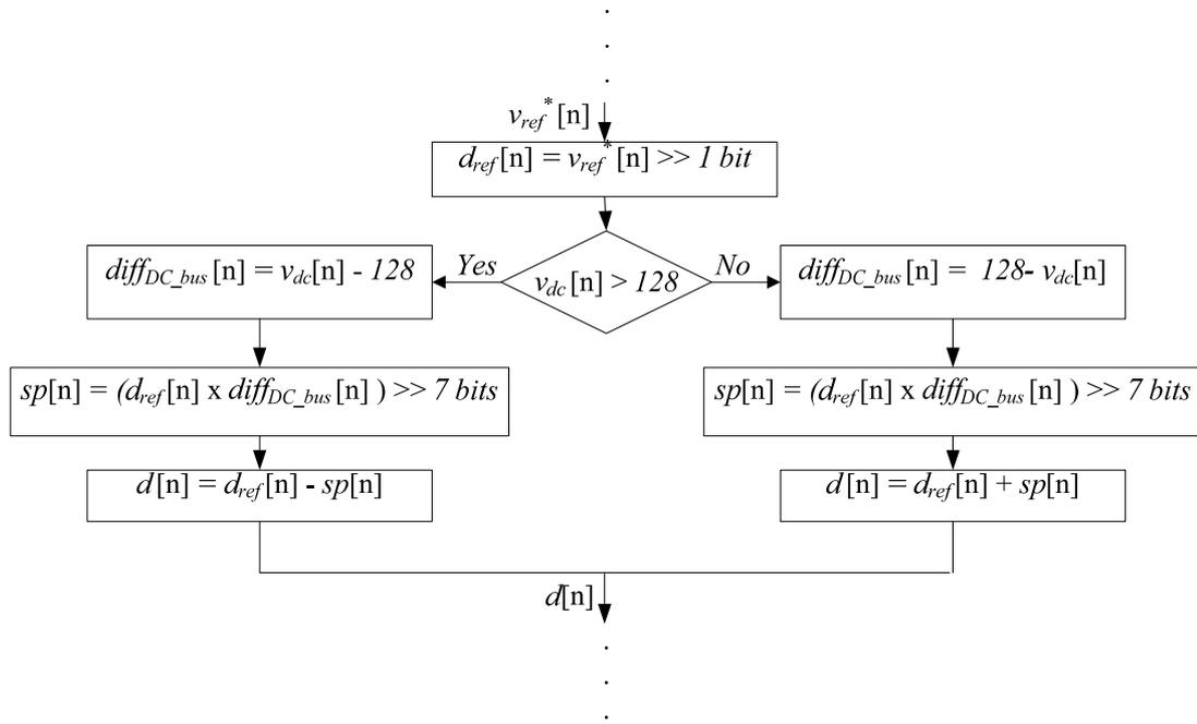
Figure 5.10 Program flow of the DC bus scaling algorithm.
