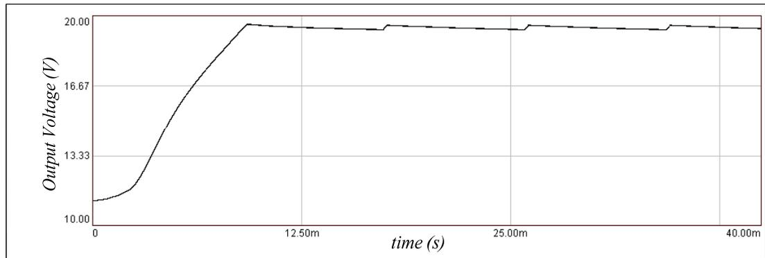
Figure 5.30 Simulation results for the output voltage characteristics of the UC discharging system for a 19.5V set voltage command considering the PI regulator case.
