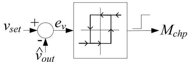
Figure 4.13 Hysteresis control structure for the chopper.
