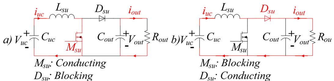
Figure 4.9 Operating modes of a step-up DC-DC converter based UC discharger:
