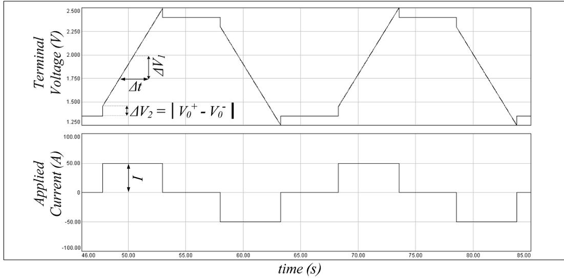
Figure 3.3 A typical voltage and current profile of a UC under constant current test.
