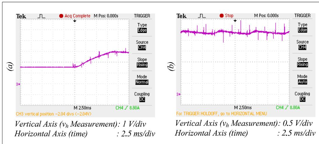
Figure 5.37 Experimental results for the output voltage characteristics of the UC discharging system for a 19.5V set voltage command considering the PI regulator case: (a) output voltage build-up, (b) steady-state variation of output voltage.
