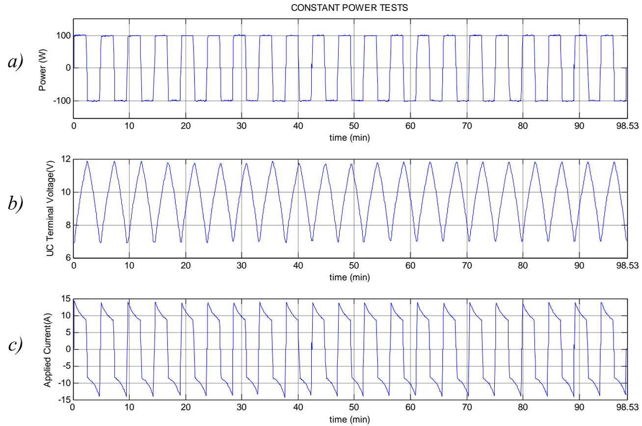
Figure 6.15 Long term variation of the UC module for constant power tests: (a) power variation, (b) terminal voltage variation of the UC module, (c) applied current variation.
