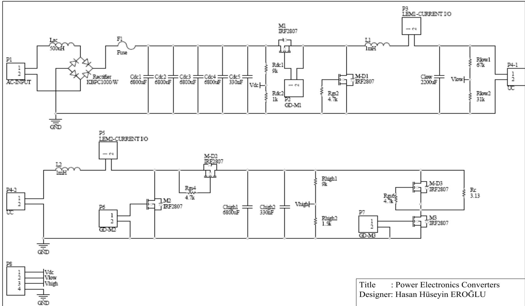
Figure B.5 Schematic diagram of the power electronics converters.
