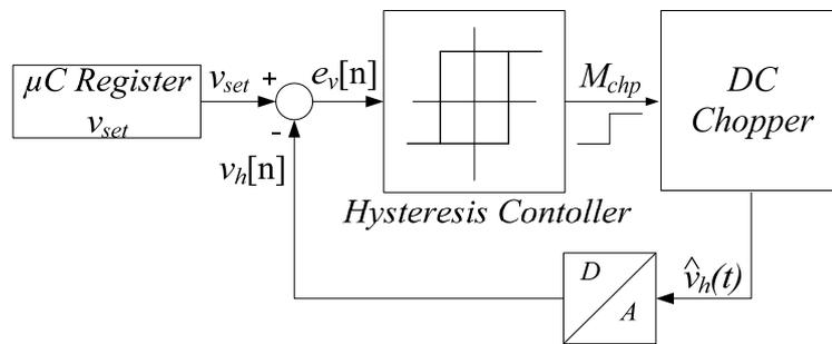
Figure 5.22 Block diagram of the microcontroller based DC chopper control structure with a hysteresis controller.
