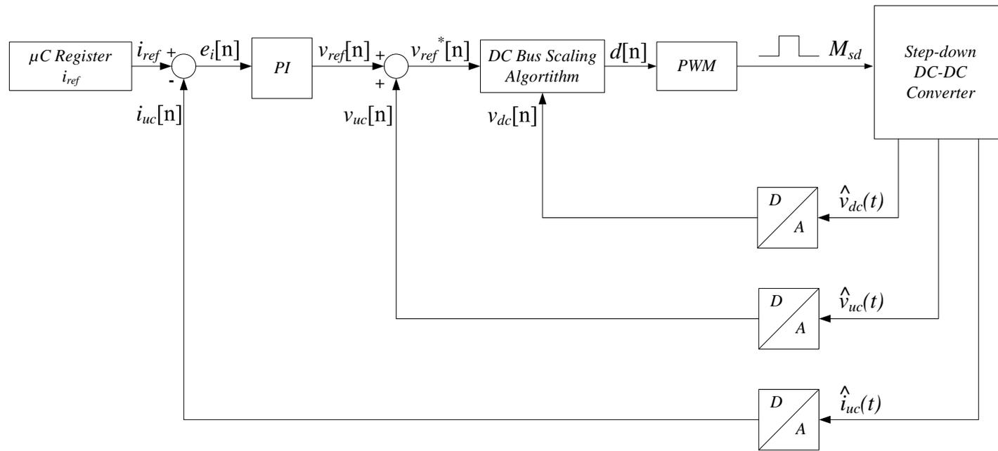
Figure 5.9 Block diagram of the microcontroller based UC charging system.
