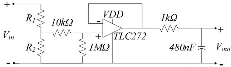
Figure 5.6 Schematic diagram of the voltage measurement circuit.
