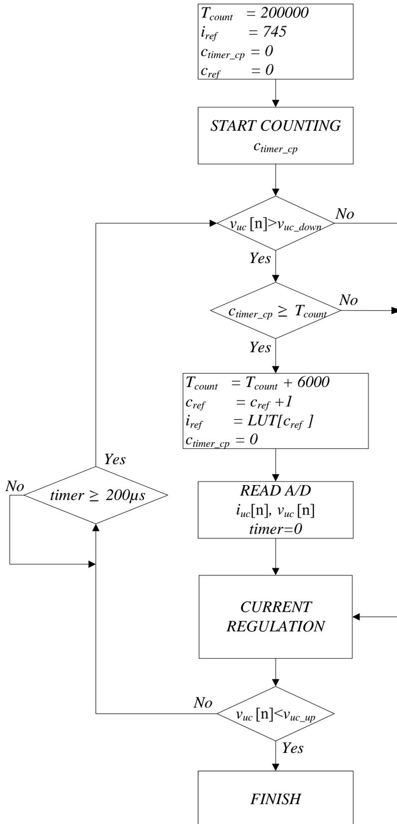
Figure 6.13 Flowchart of the microcontroller implementation of the constant power test procedure for the charging phase of the UC test system.
