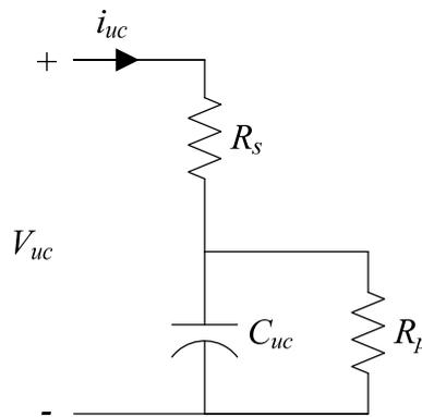
Figure 2.7 Basic electrical equivalent circuit of a UC [21-22].
