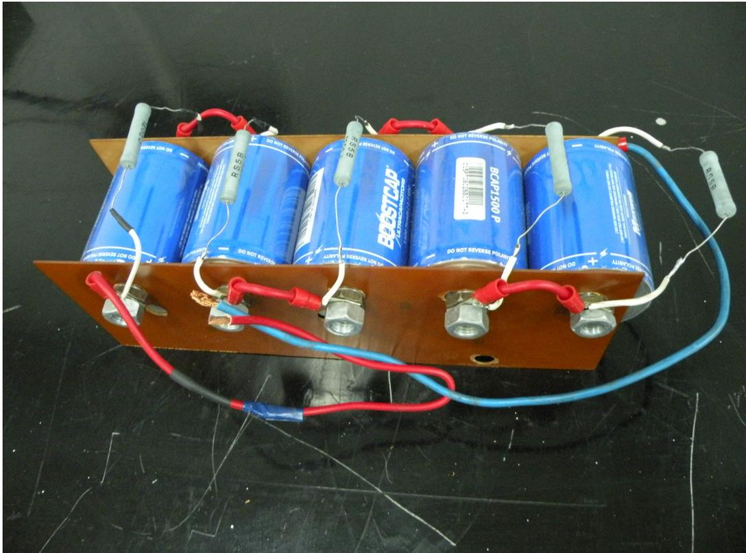
Figure 6.1 The laboratory constructed UC module.
