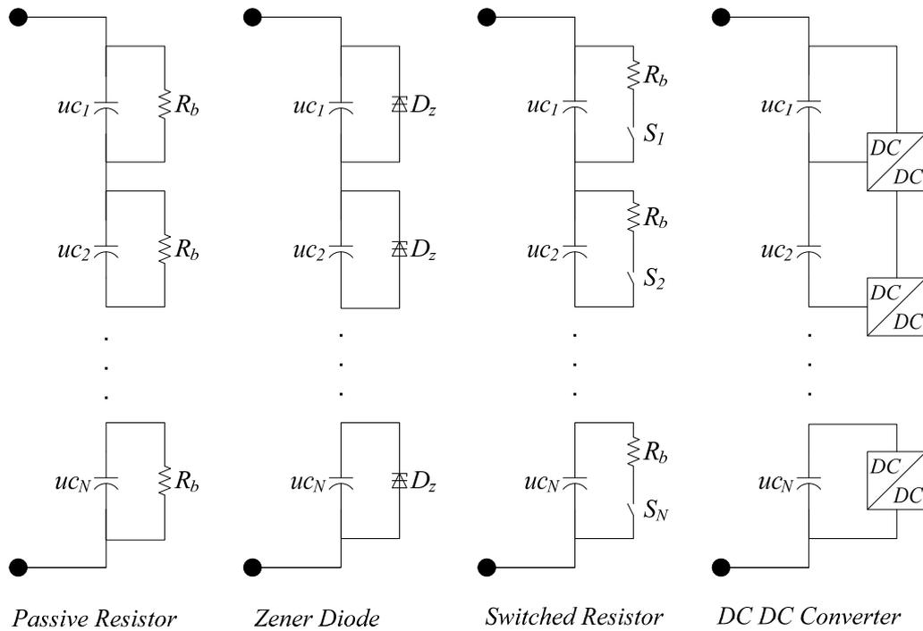
Figure 2.11 Schematic representations of voltage balancing structures [29].
