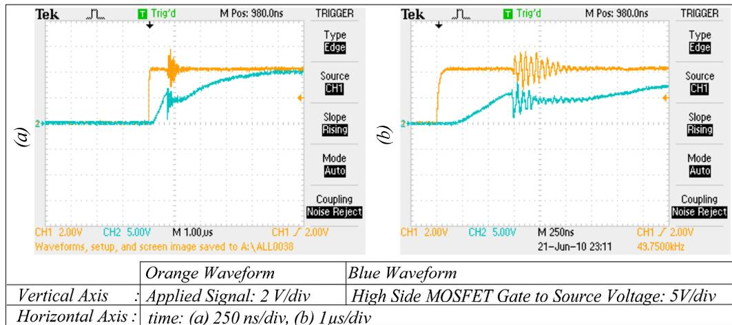
Figure 5.4 High side MOSFET turn on characteristics for a gate resistance value of 200  $\Omega$ : (a) turn on characteristics obtained for a time scale of 1  $\mu$ s/div, (b) turn on characteristics obtained for a time scale of 250ns/div.
