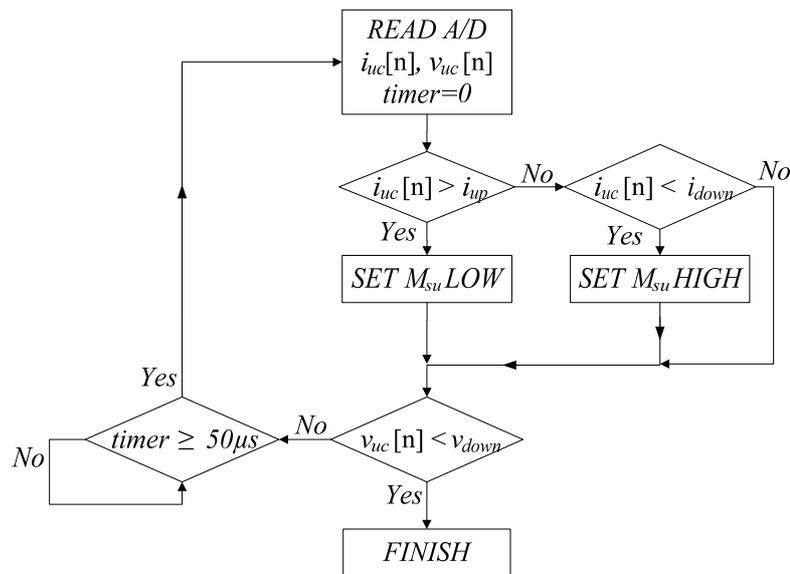
Figure 5.25 Program flow of the UC discharging current regulator structure with a hysteresis controller.
