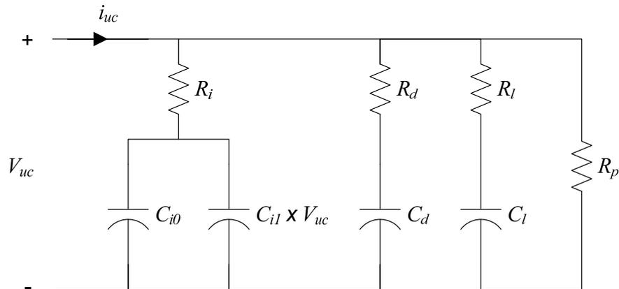
Figure 2.8 Detailed electrical equivalent circuit of a UC [23].
