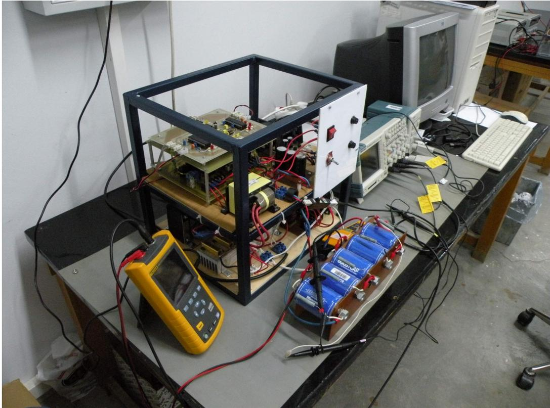
Figure 6.3 The laboratory constructed UC test system.
