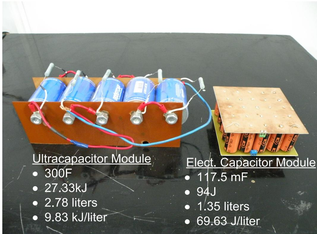
Figure 6.2 Comparison of the laboratory constructed UC and electrolytic capacitor modules.
