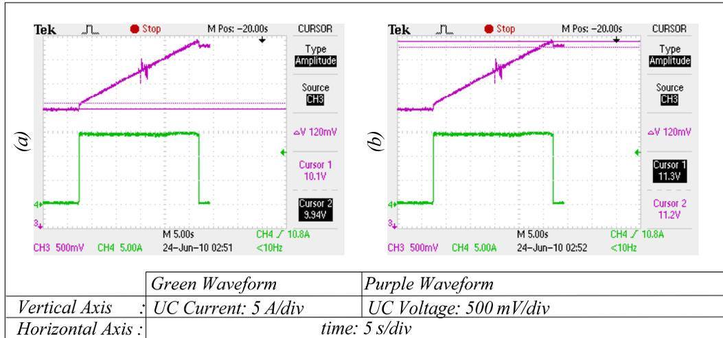
Figure 6.9 Immediate characteristics of the UC module terminal voltage for the charging phase: (a) measurement of the increase of the UC module terminal voltage with purple colored voltage cursors at the beginning of the charging phase, (b) measurement of the decrease of the UC module terminal voltage with purple colored voltage cursors at the end of the charging phase.
