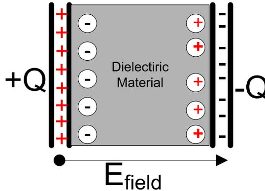
Figure 2.1 Internal structure of a capacitor.
