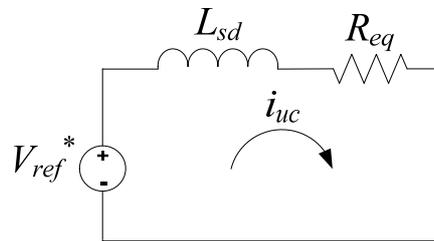
Figure 4.5 Schematic representation of the first order simplified model of the UC charging structure.
