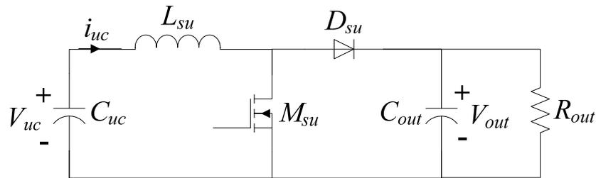
Figure 4.8 Schematic representation of a step-up DC-DC converter based UC discharger.
