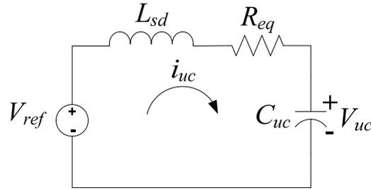
Figure 4.4 Schematic representation of the average model for the UC charging structure.
