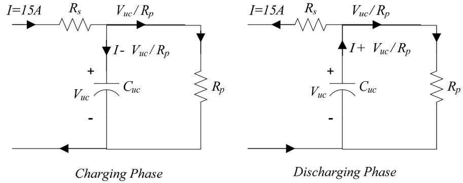
Figure 6.6 Equivalent circuit model of the UC module for the charging and discharging phases.
