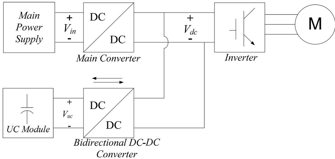
Figure 2.14 Block diagram of a UC assisted electric vehicle application.
