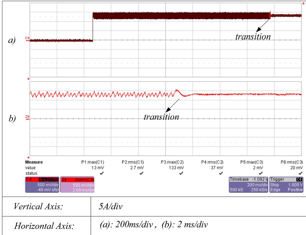
Figure 5.43 Experimental results for the UC discharging system with a hybrid controller structure for a 15A current command: (a) build up and transition behaviour of the UC discharging current, (b) transition behaviour of the UC discharging current (zoomed).
