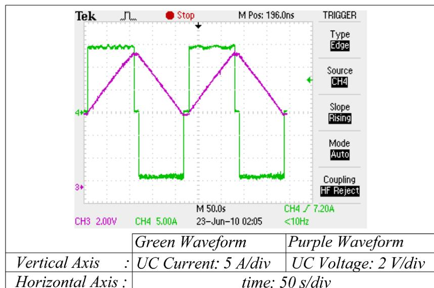
Figure 6.4 Terminal voltage variation of the UC module and applied current for constant current tests.
