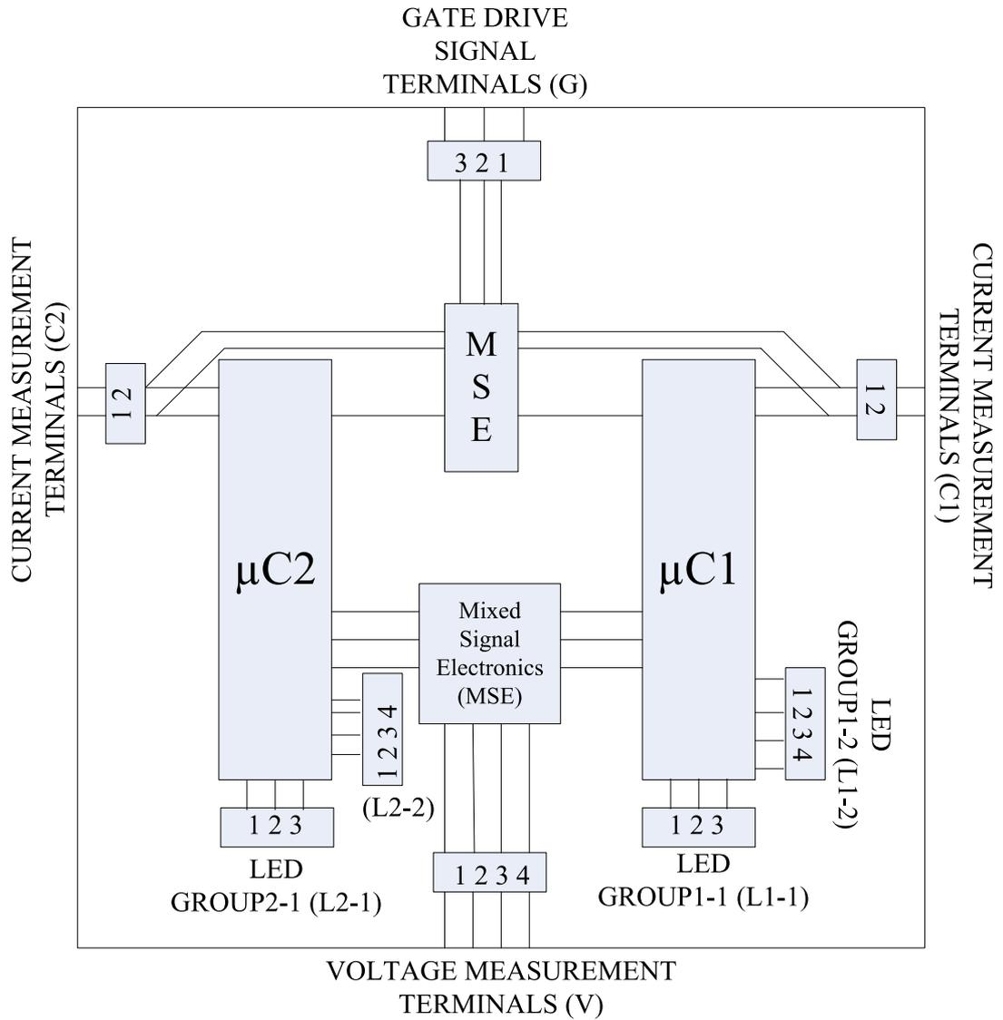
Figure F.1 Block diagram of the microcontroller board.
