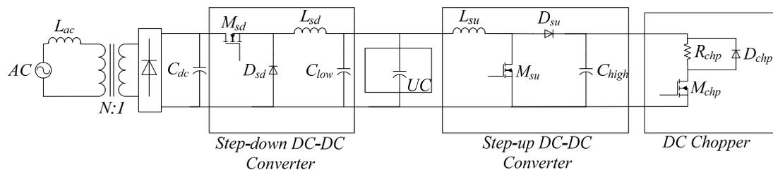
Figure 5.2 Schematic diagram of the power electronics converter structure.
