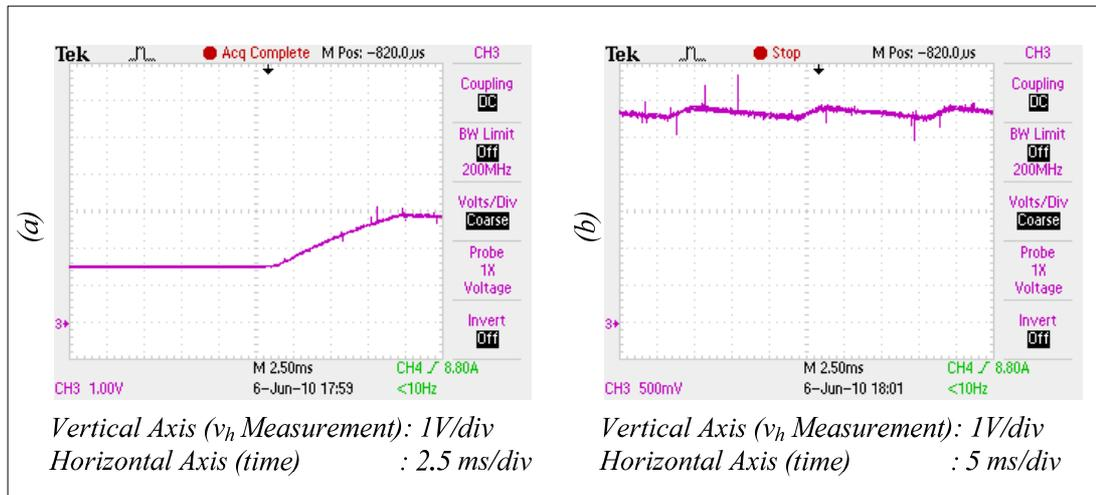
Figure 5.40 Experimental results for the output voltage characteristics of the UC discharging system for a 19.5V set voltage command considering the hysteresis regulator case: (a) output voltage build-up, (b) steady-state variation of output voltage.
