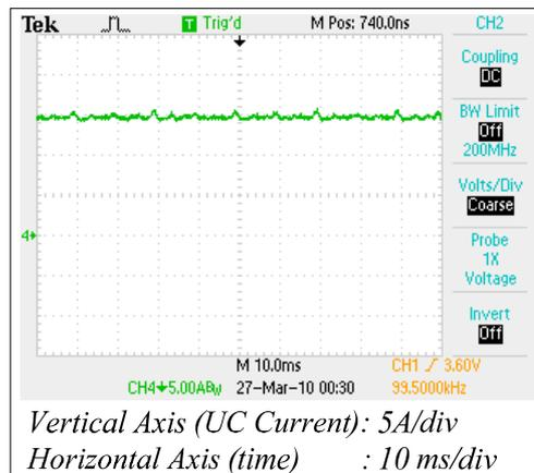
Figure 5.18 Experimental results for the steady-state UC charging current for a 15A current command.
