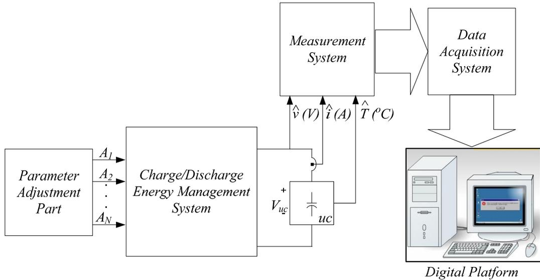
Figure 3.1 Block diagram of a UC test device.
