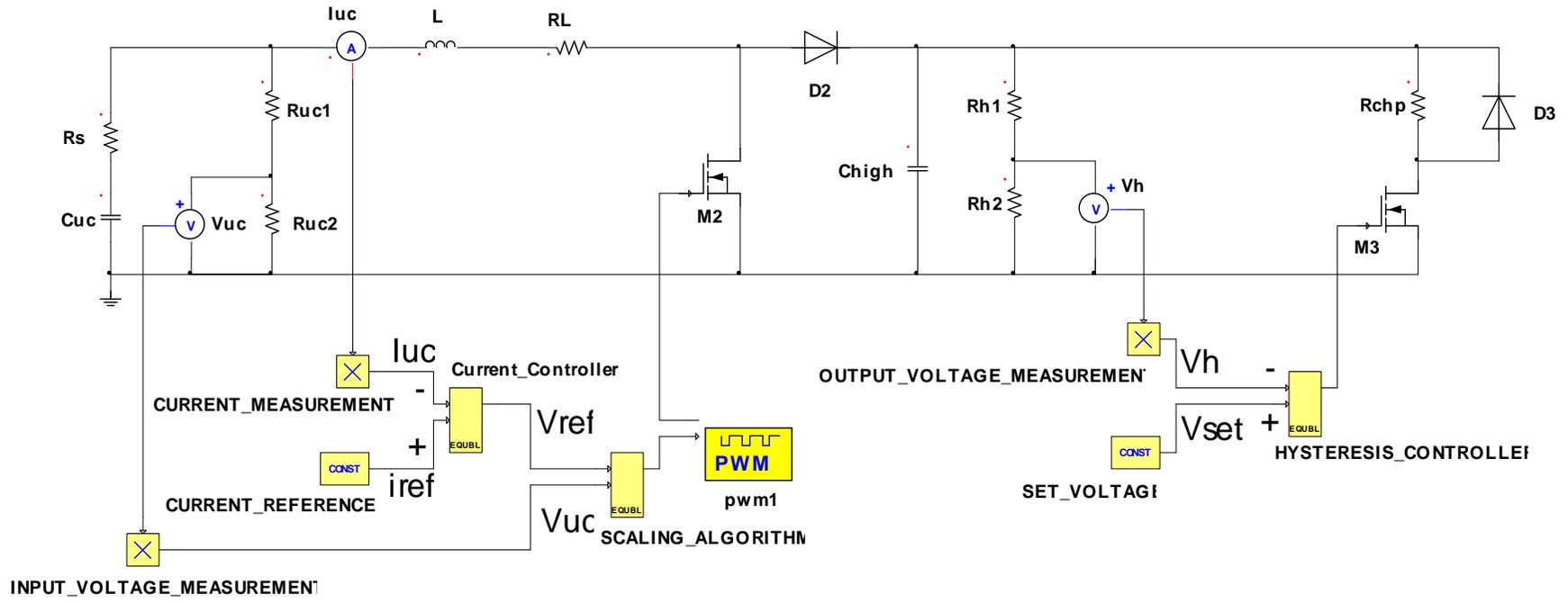
Figure 5.27 Simulation model of the UC discharging system.
