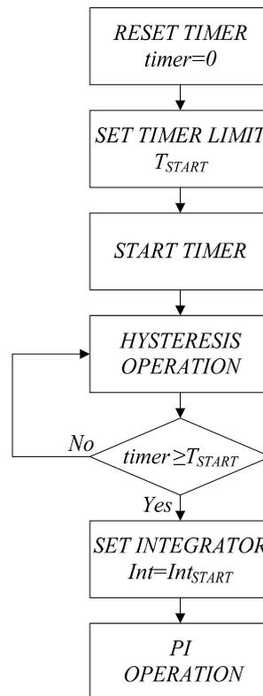
Figure 5.41 Flowchart of the hybrid control structure proposed for the UC discharging system.
