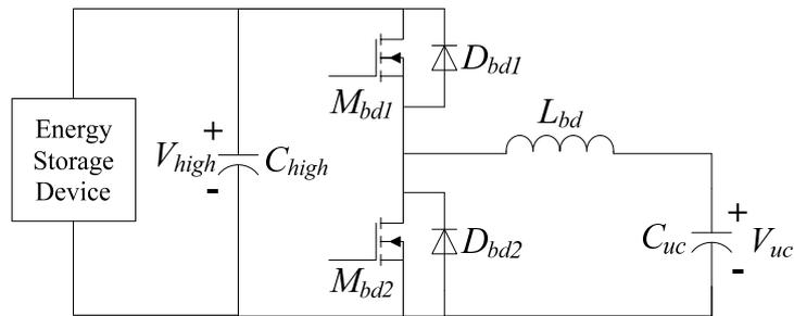
Figure 4.14 Schematic representation of a bi-directional DC-DC converter interfacing a UC to an energy storage device.
