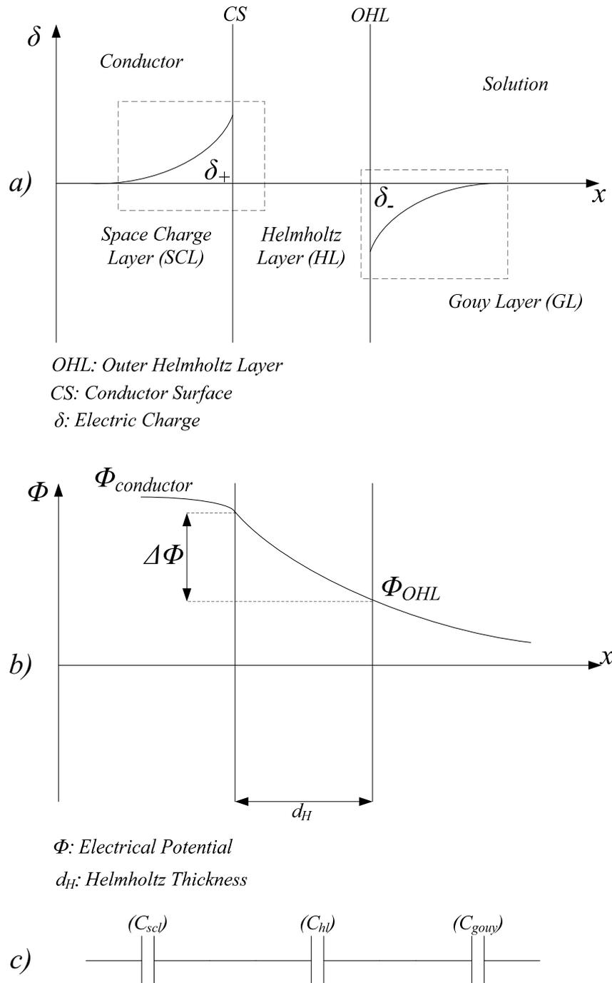
Figure 2.5 Three layer model of the EDL structure: (a) variation of excess charge density, (b) variation of inner potential, (c) capacitor model [17].
