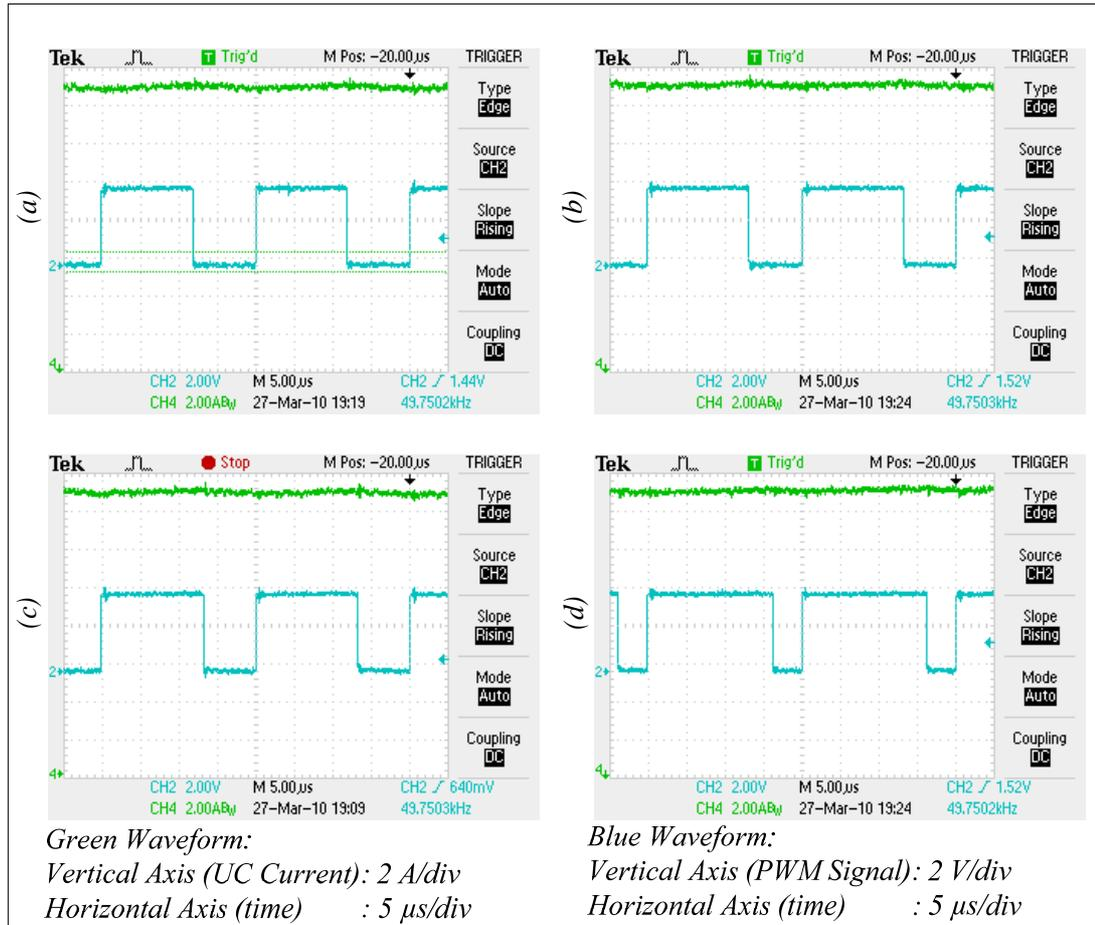
Figure 5.36 Experimental results for the steady-state ripple characteristics of the UC discharging current for a 15A current command considering the PI regulator case:
