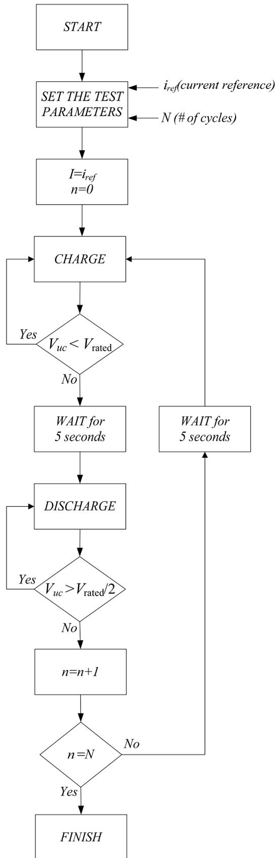
Figure 3.2 Constant current test procedure.
