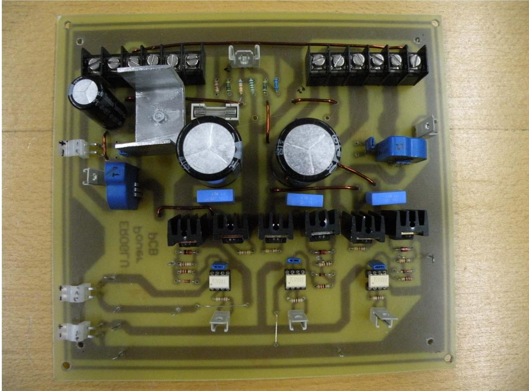
Figure D.2 Photograph of the power electronics converter board.
