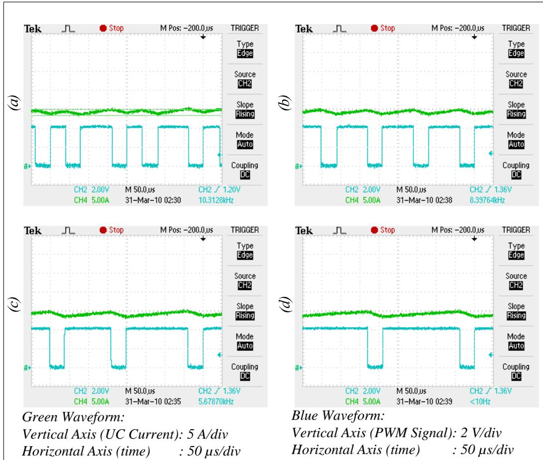
Figure 5.39 Experimental results for the steady-state ripple characteristics of the UC discharging current for a 15A current command considering the hysteresis regulator case: (a)  $V_{uc} = 11.6V$ , (b)  $V_{uc} = 9.80V$ , (c)  $V_{uc} = 7.6V$ , (d)  $V_{uc} = 6.5V$ .
