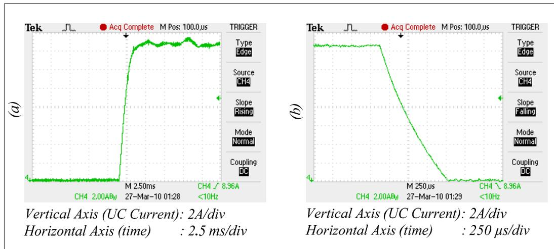
Figure 5.17 Experimental results for the dynamic response of the UC charging current for a 15A current command: (a) UC charging current build-up, (b) UC charging current fall.
