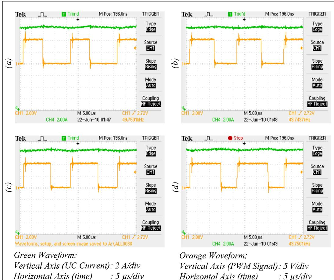
Figure 5.19 Experimental results for the switching signal and steady-state ripple characteristics of the UC charging current for a 15A current command:
