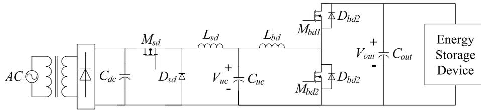
Figure 4.18 Schematic representation of the power electronics converter structure for a bi-directional energy transfer mechanism based UC test system.
