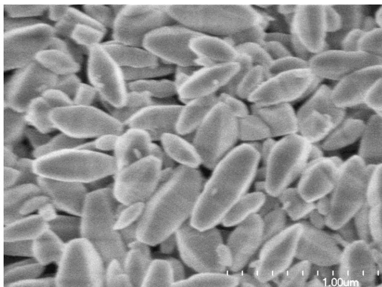
Figure 1.3: SEM image of ETS-10 crystals.
