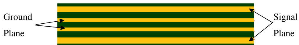
Figure 3.3 Stack up layers of the TPS54610EVM PCB
