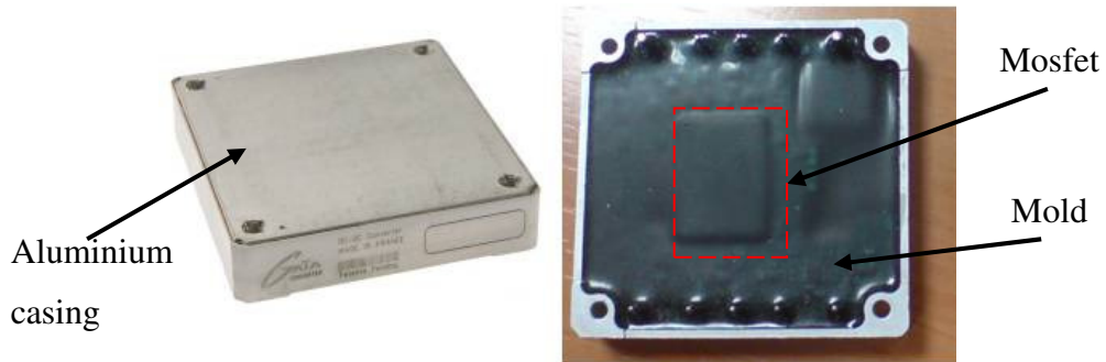
Figure 4.22 Important parts of MGDM-150 DC/DC converters
