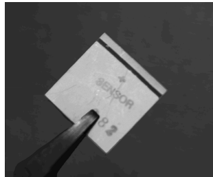
Figure 2.2: Piezoelectric Patch (SensorTech - BM500 PZT Patch)
