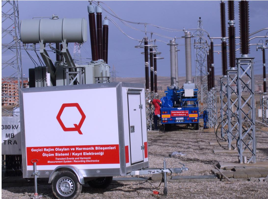
Figure 5.16: Trailers used in measurements at 380 kV
