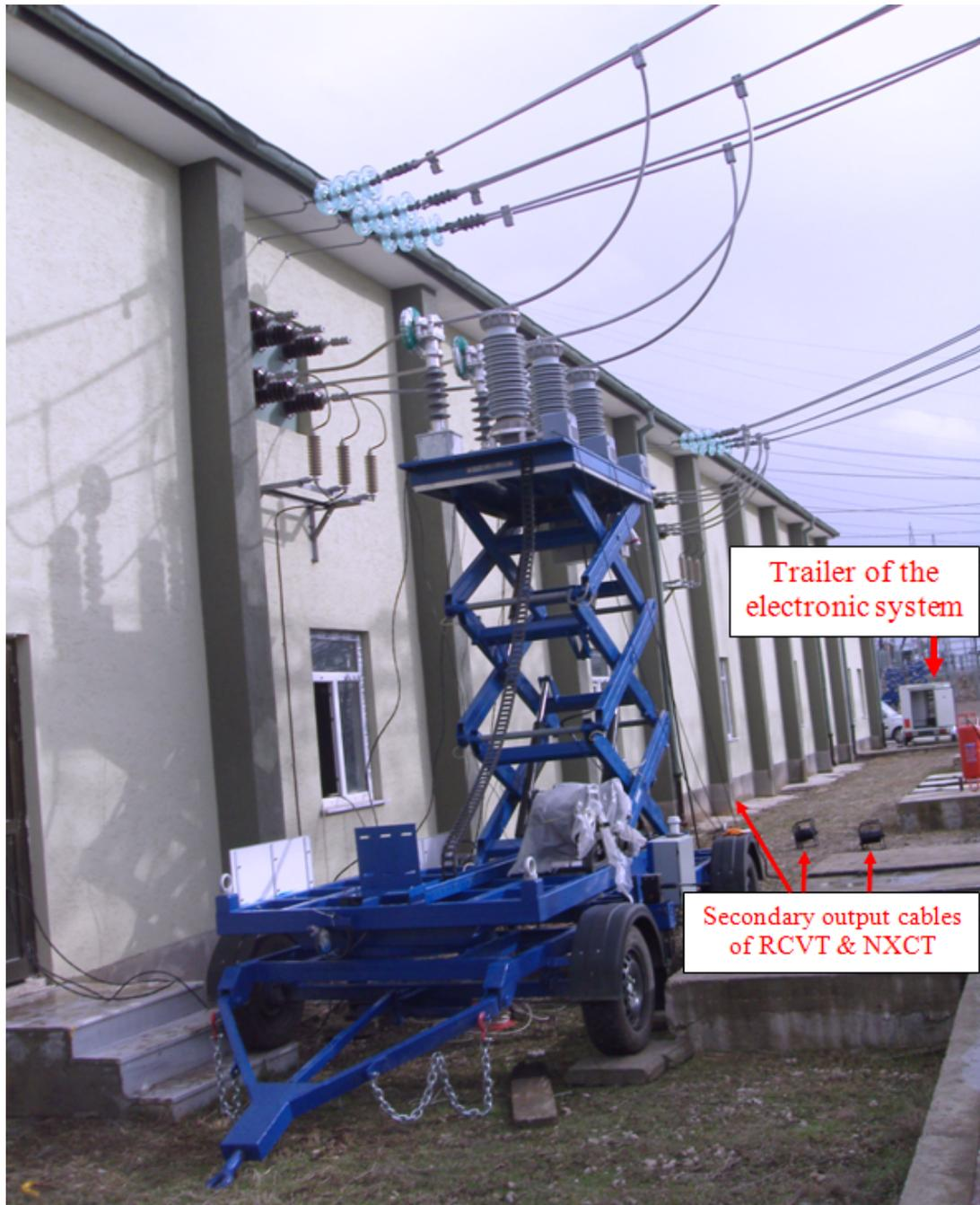
Figure 5.3: Trailers used in measurements at 34.5 kV
