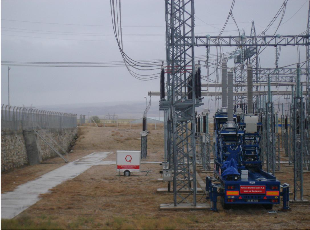
Figure 5.13: Trailers used in measurements at 154 kV
