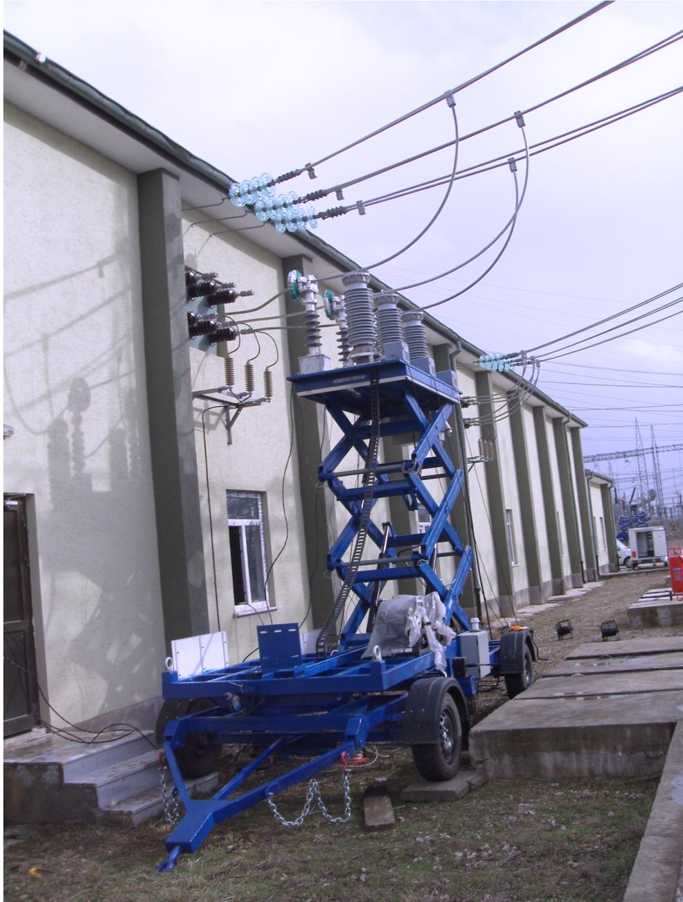
Figure 3.8: Trailer which is used at 36 kV measurements
