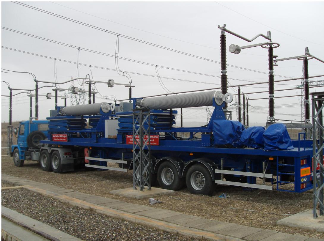
Figure 3.1: 420 kV NXVCT columns are at transportation position
