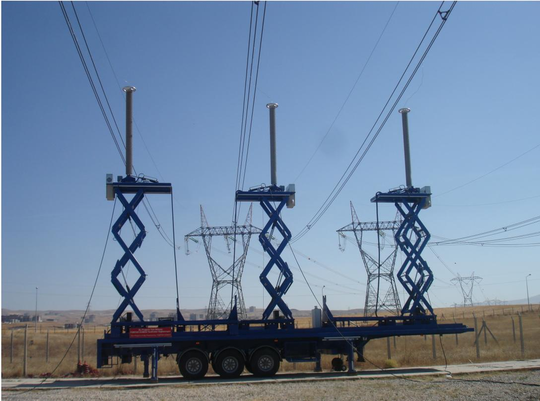
Figure 3.4: 420 kV RCVT columns are raised by the lift
