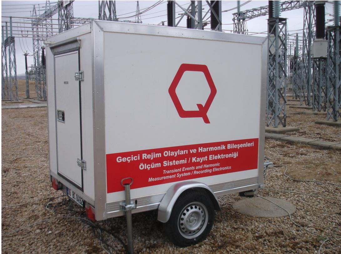
Figure 3.10: Trailer of the Electronic System
