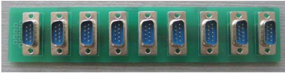
**Figure 6-1** The PCB Bus Used For Both FlexRay and CAN Bus
