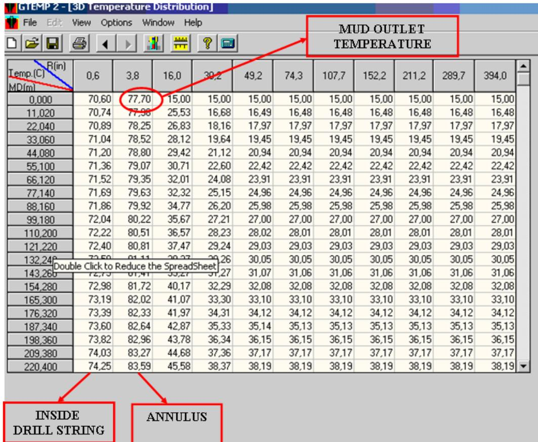
Figure 6.14. 3D Temperature Table at Surface.
