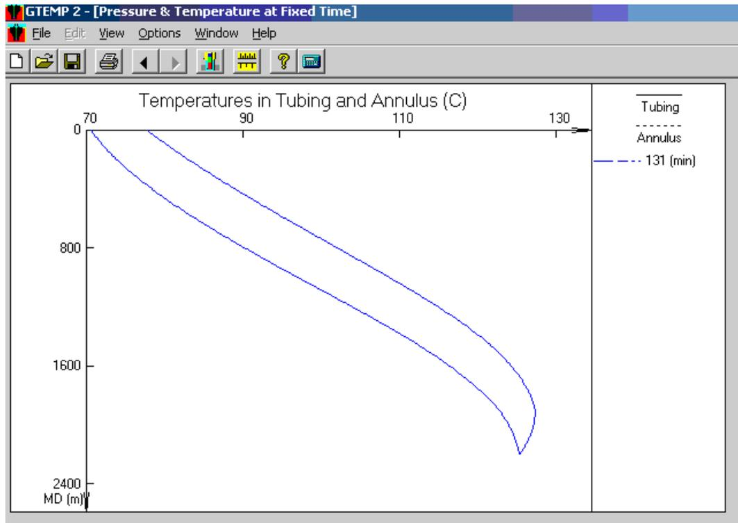
**Figure 6.16. Temperature at Fixed Time Window.**
