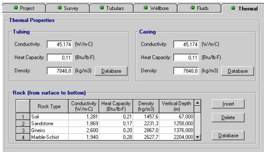
**Figure 6.11. Thermal Page of GTEMP.**
