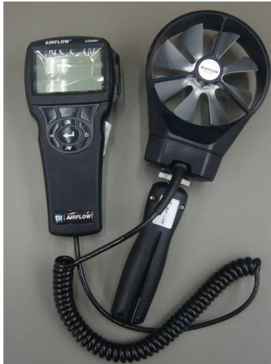
**Figure D.14:** Air velocity meter
