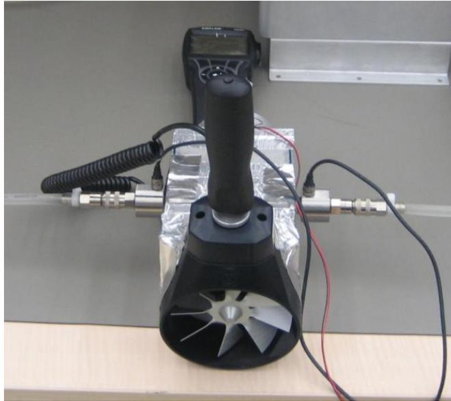
**Figure 4.16:** A view of air velocity meter assembled to the microchannel heat exchanger
