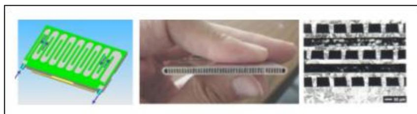
**Figure 1.8:** Schematics of liquid heat sink (left), minichannel heat sink (center), and microchannel heat sink (right) [6]
