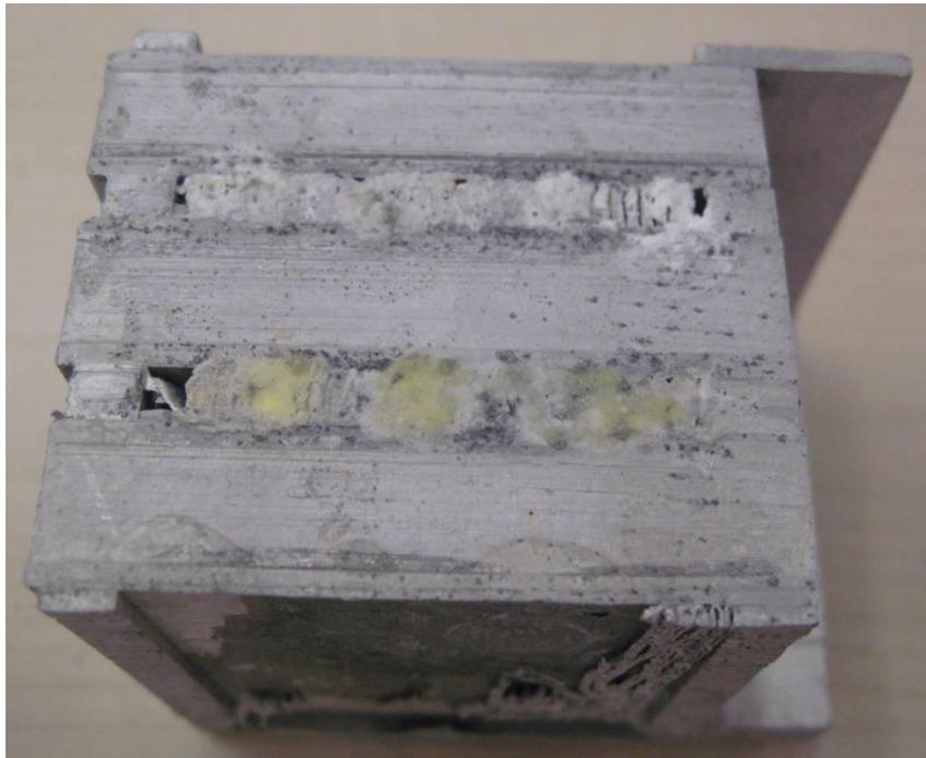
**Figure 4.7:** A view of the second quarter specimen of the preliminary microchannel heat exchanger produced in dip brazing, after being sliced into four specimens
