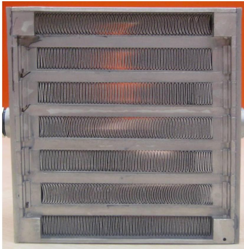
**Figure 4.12:** The test microchannel heat exchanger
