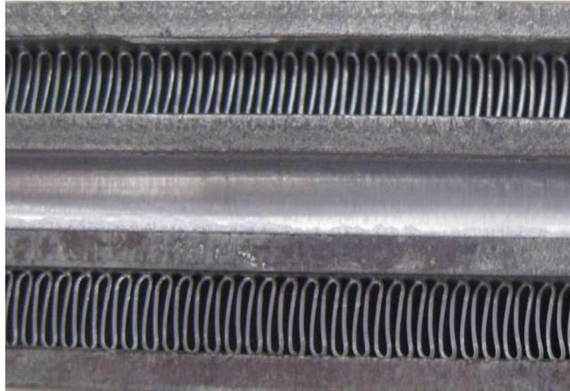
**Figure 4.9:** The test specimen produced in vacuum brazing
