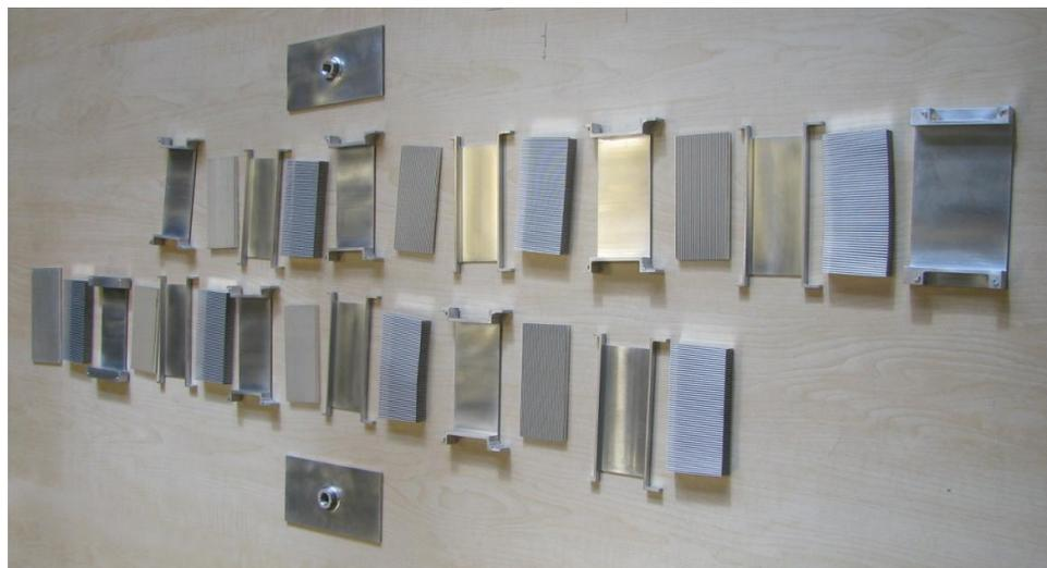
**Figure 4.10:** All parts require to assemble the microchannel heat exchanger in vacuum brazing
