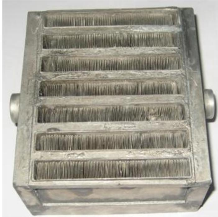
**Figure 4.5:** Secondary heat exchanger in dip brazing
