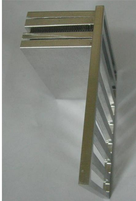
**Figure 4.4:** A view of the assembly step of the preliminary heat exchanger before dip brazing
