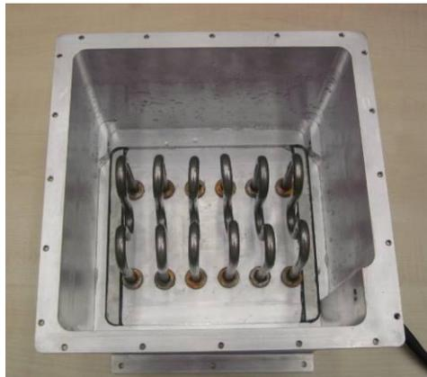
**Figure D.12:** Top view of the heating tank
