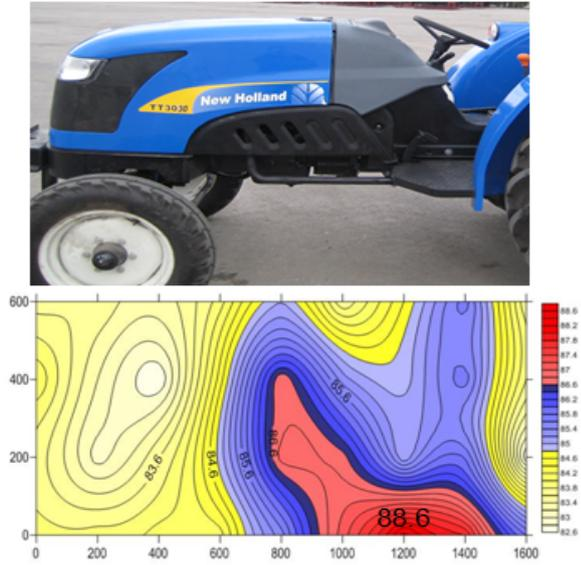
Figure 6.5 The Original Intensity Map of the Left Side at 630 Hz
