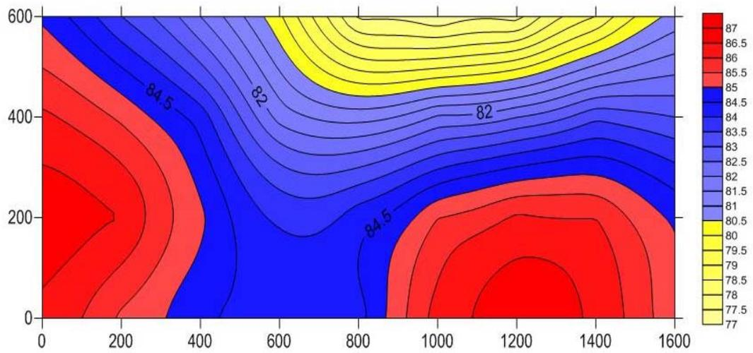
Figure 5.7 The Original Intensity Map of the Left Side of the Tractor at 400 Hz
