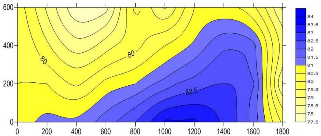
Figure 5.30 The Final Intensity Map of the Left Side of the Tractor at 400 Hz
