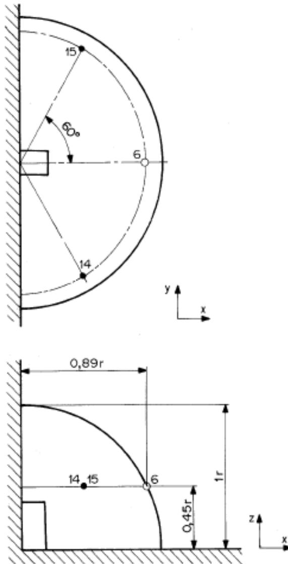
Figure 4.2 The Sketch Showing Microphone Locations of the Test Area [29]
