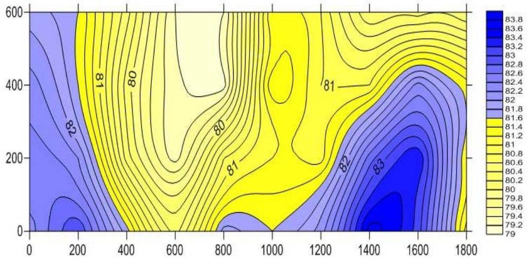
Figure 5.34 The Final Intensity Map of the Left Side of the Tractor at 800 Hz
