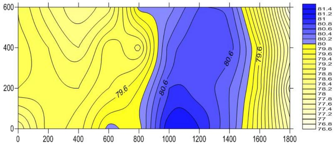
Figure 5.28 The Final Intensity Map of the Left Side of the Tractor at 315 Hz
