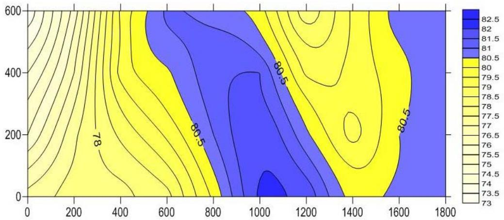
Figure 5.44 The Final Intensity Map of the Right Side of the Tractor at 630 Hz
