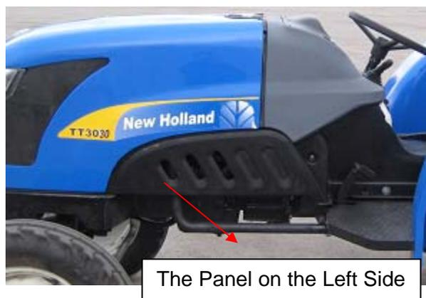
Figure 6.1 The Engine Panel on the Left Side
