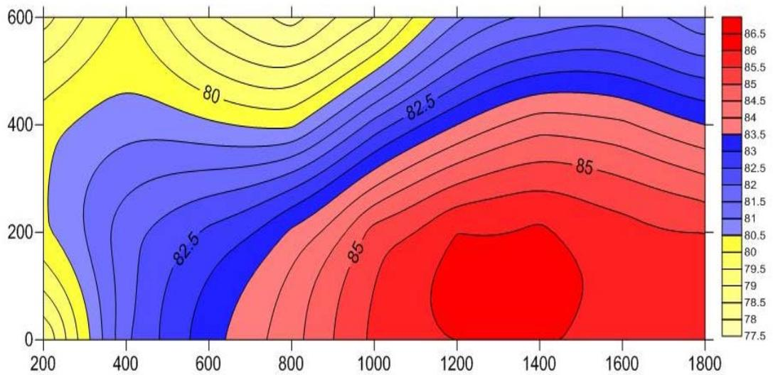
Figure 5.21 The Original Intensity Map of the Right Side of the Tractor at 400 Hz
