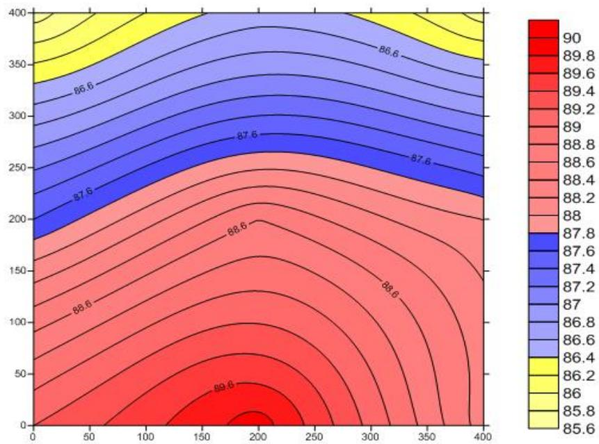
Figure 5.15 The Original Intensity Map of the Front Side of the Tractor at 630 Hz
