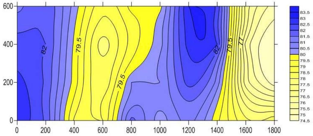
Figure 5.32 The Final Intensity Map of the Left Side of the Tractor at 630 Hz
