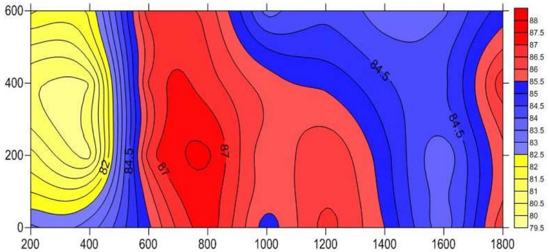
Figure 5.25 The Original Intensity Map of the Right Side of the Tractor at 800 Hz
