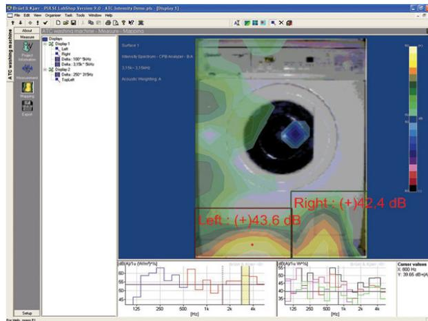
Figure 3.1 The intensity map of a washing machine [33]
