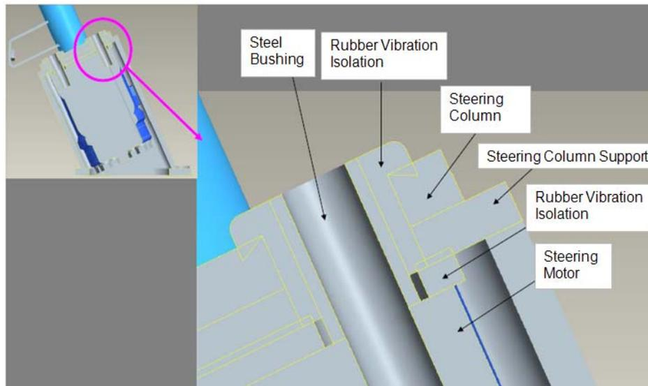
Figure 5.47 A Sectional View of Steering Motor Column and its Support
