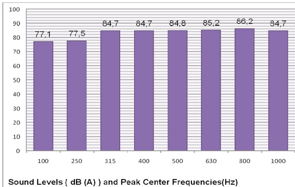
Figure 5.3 Sound Level and Peak Center Frequencies on the Right Side
