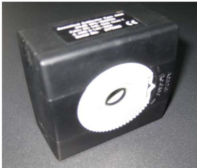
Figure 4.8 The Sound Calibrator
