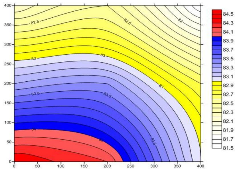
Figure 5.13 The Original Intensity Map of the Front Side of the Tractor at 250 Hz
