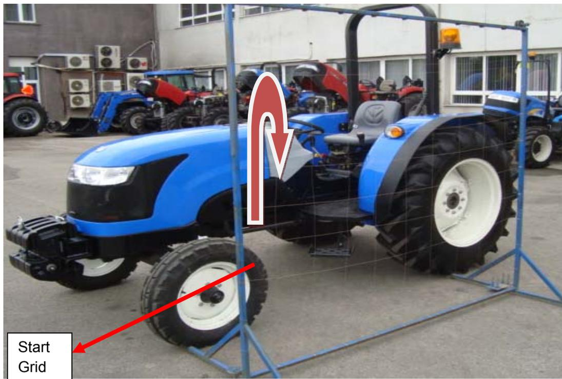
Figure 4.6 The Grid Frame used for Sound Intensity Measurements
