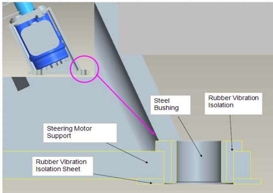
Figure 5.48 A Sectional View of Steering Motor Column and its Support
