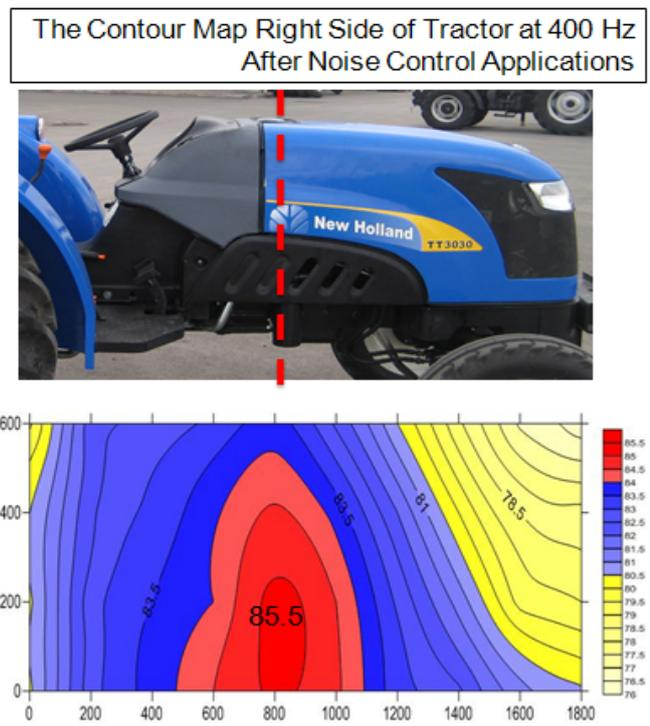
Figure 6.4 The Final Intensity Map of the Right Side at 400 Hz
