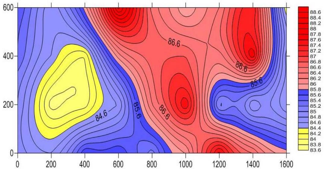
Figure 5.11 The Original Intensity Map of the Left Side of the Tractor at 800 Hz
