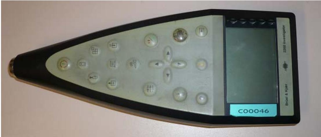
Figure 4.9 The Sound Level Meter
