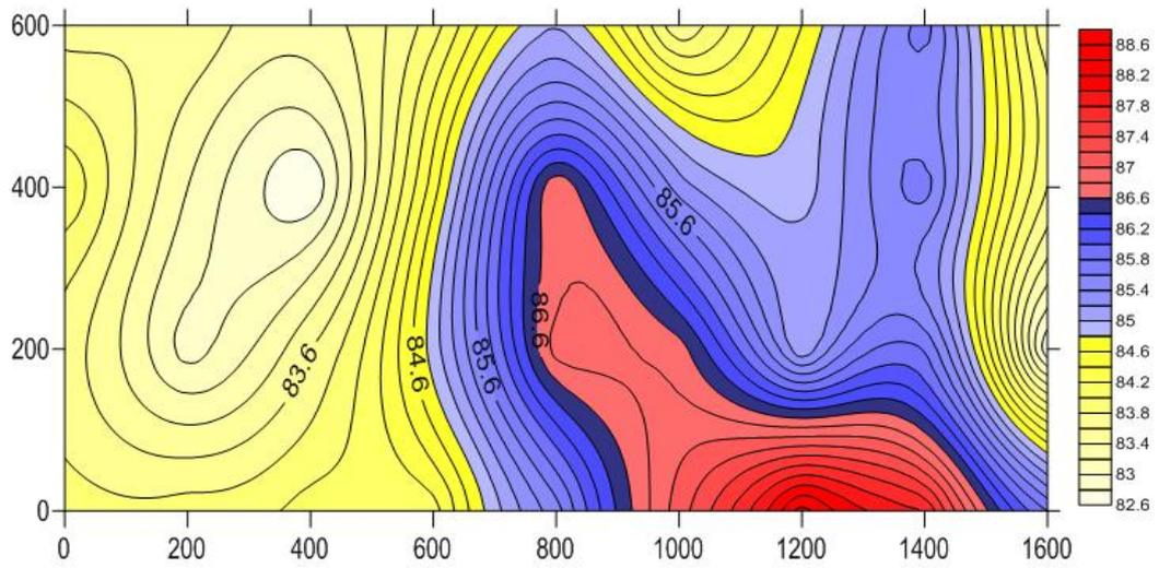
Figure 5.9 The Original Intensity Map of the Left Side of the Tractor at 630 Hz
