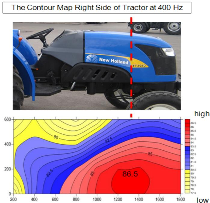
Figure 6.3 The Original Intensity Map of the Right Side at 400 Hz
