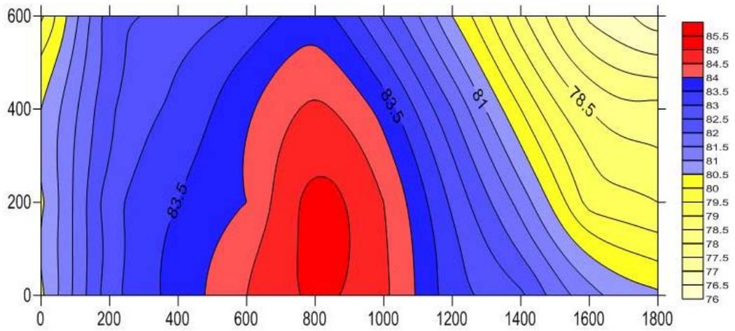
Figure 5.42 The Final Intensity Map of the Right Side of the Tractor at 400 Hz
