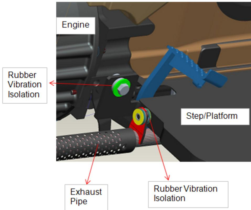
Figure 5.49 The Exhaust Pipe Isolation view taken from 3D Master Model of the Tractor
