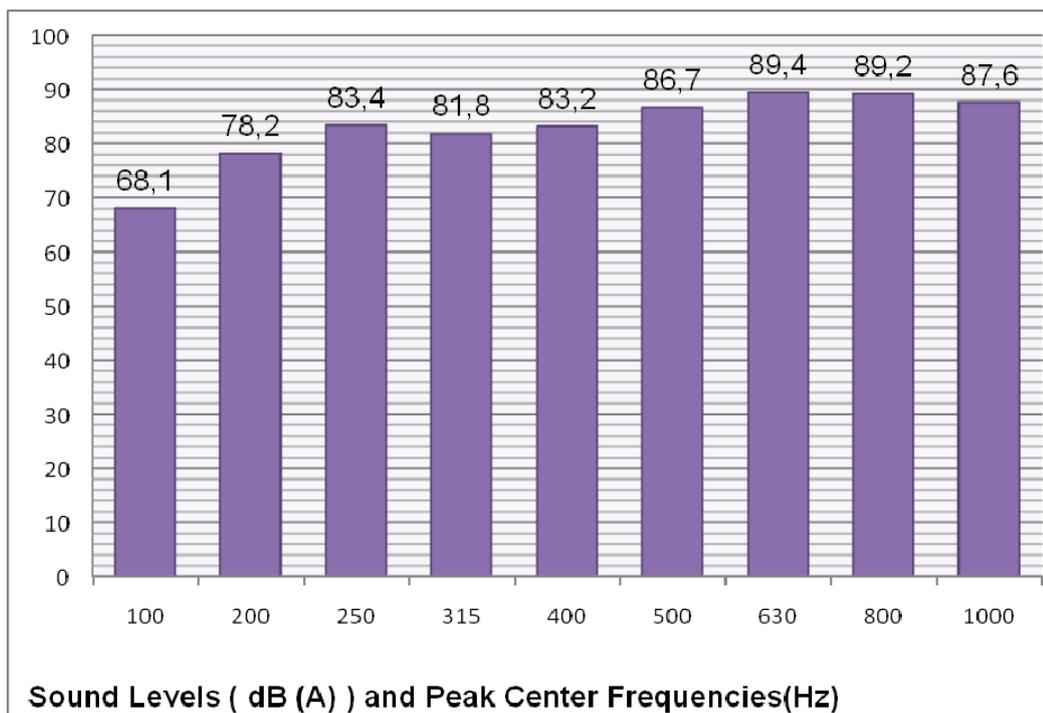
Figure 5.1 Sound Levels and Peak Center Frequencies on the Front Side
