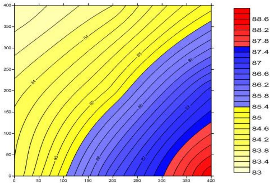
Figure 5.38 The Final Intensity Map of the Front Side of the Tractor at 630 Hz
