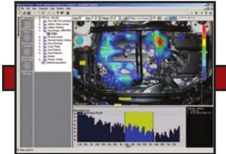
Figure 3.3 The intensity map of an internal combustion engine [35]
