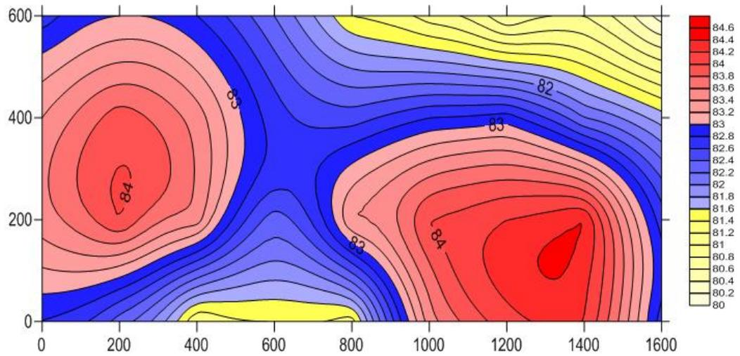
Figure 5.5 The Original Intensity Map of the Left Side of the Tractor at 315 Hz
