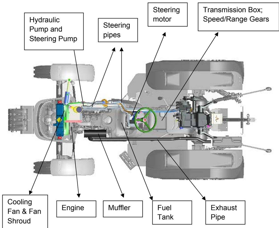
Figure 3.8 Potential Noise Sources on the Tractor
