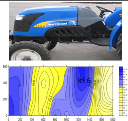
Figure 6.6 The Final Intensity Map of the Left Side at 630 Hz
