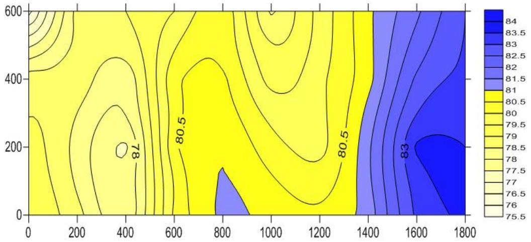
Figure 5.46 The Final Intensity Map of the Right Side of the Tractor at 800 Hz
