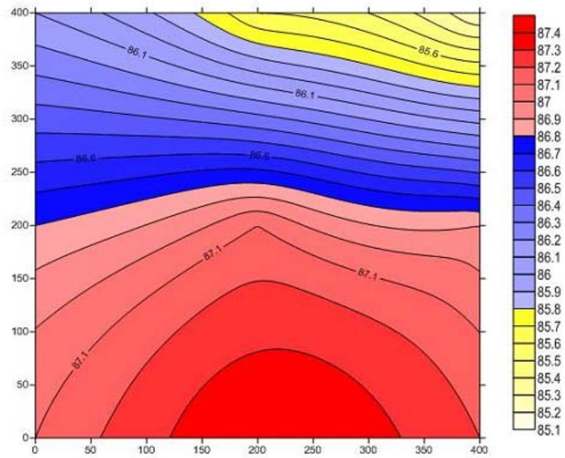
Figure 5.17 The Original Intensity Map of the Front Side of the Tractor at 1000 Hz
