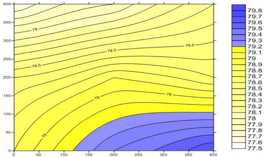
Figure 5.36 The Final Intensity Map of the Front Side of the Tractor at 250 Hz
