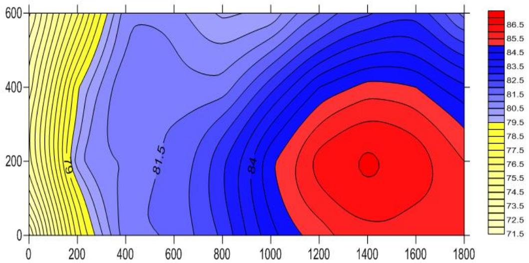
Figure 5.19 The Original Intensity Map of the Right Side of the Tractor at 315 Hz
