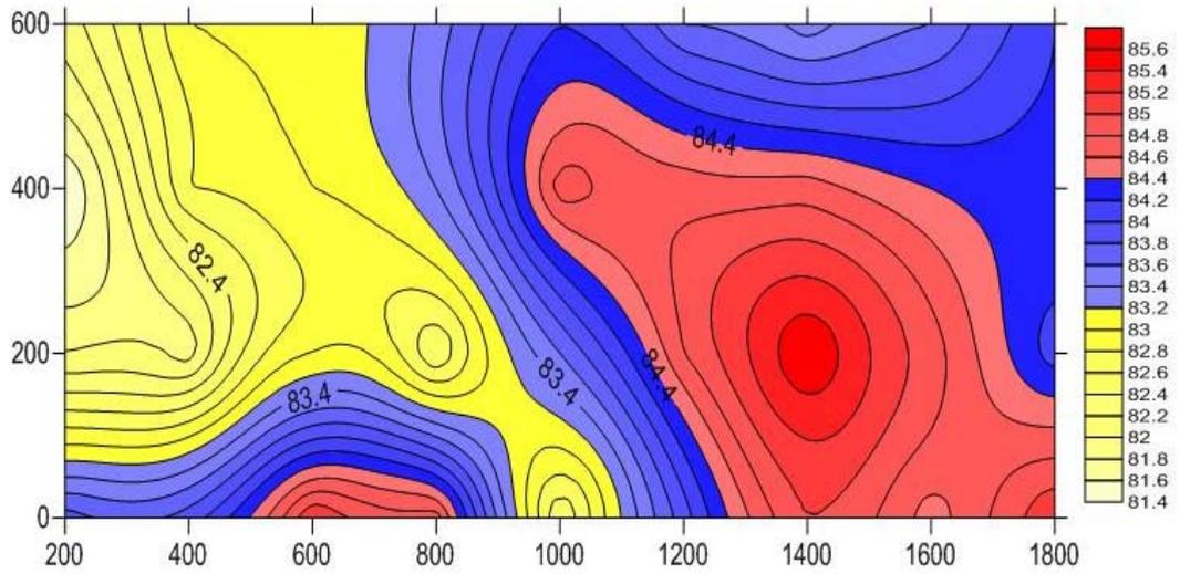
Figure 5.23 The Original Intensity Map of the Right Side of the Tractor at 630 Hz
