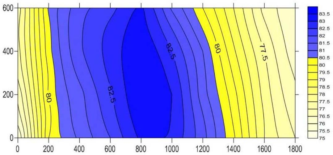
Figure 5.40 The Final Intensity Map of the Right Side of the Tractor at 315 Hz
