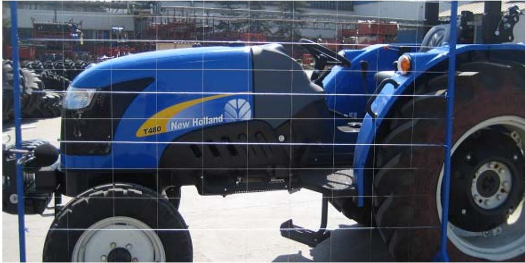
Figure 4.11 The Left Side View of the Test Tractor during Sound Intensity Measurements
