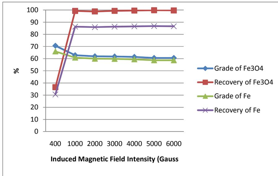
Figure 4.18 Results of the magnetic concentration test for -833 micron material (App. C, Table C.2)
