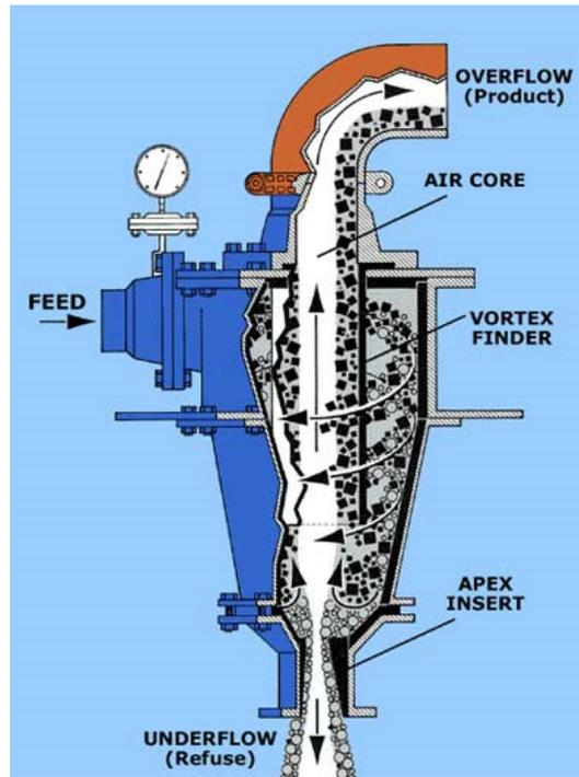
Figure 2.10 Water-only cyclone (www.flsmidthminerals.com)
