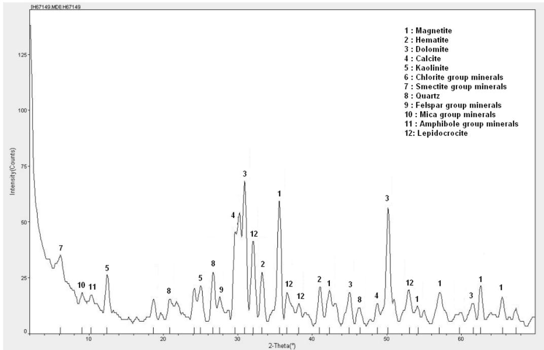
Figure 3.11 XRD pattern of medium grade tailing
