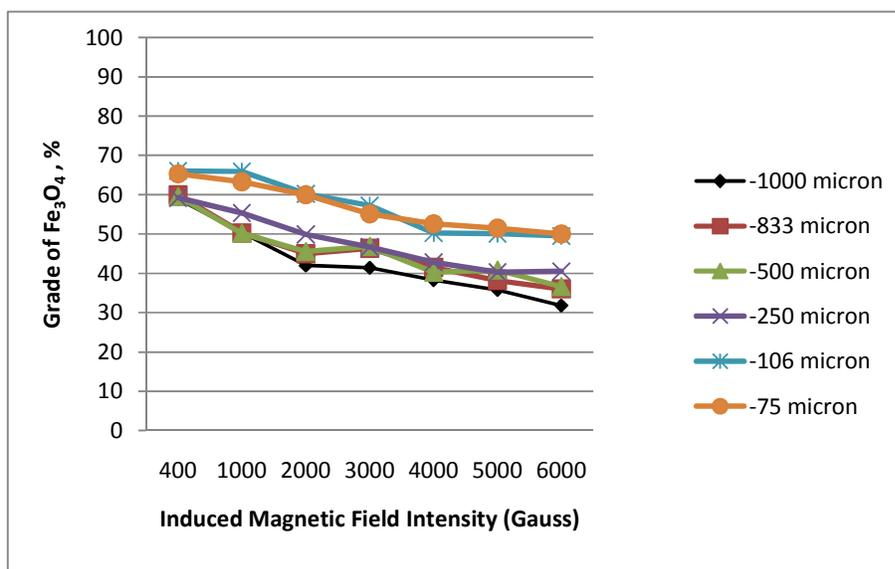
Figure 4.8 Grade of Fe<sub>3</sub>O<sub>4</sub>% versus magnetic field intensity for low grade tailing
