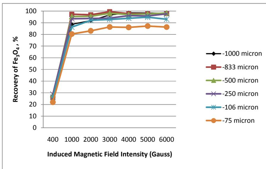
Figure 4.7 Recovery of Fe<sub>3</sub>O<sub>4</sub>% versus magnetic field intensity for low grade tailing
