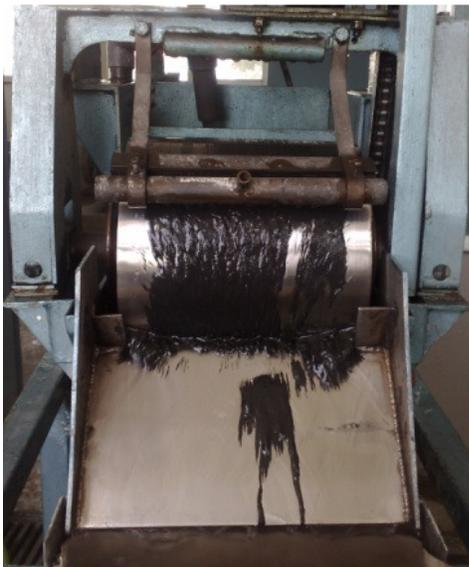
Figure 4.25 Low intensity wet magnetic drum separator
