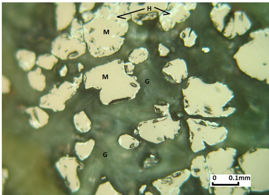
Figure 3.5 Fine grained magnetite (M) is disseminated in the gangue (G) minerals and seen locally as martite; in other words, turned to hematite (H)
