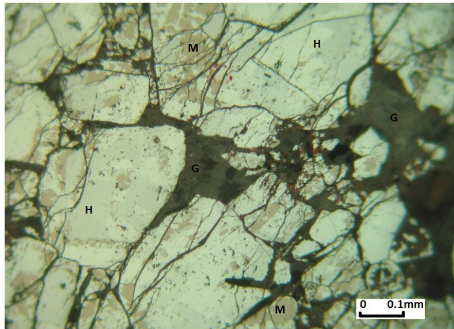
Figure 3.9 The crystals of euhedral and interlocked magnetite (**M**) are intensively altered to martite (**H**). Gangue (**G**) minerals are quartz and calcite
