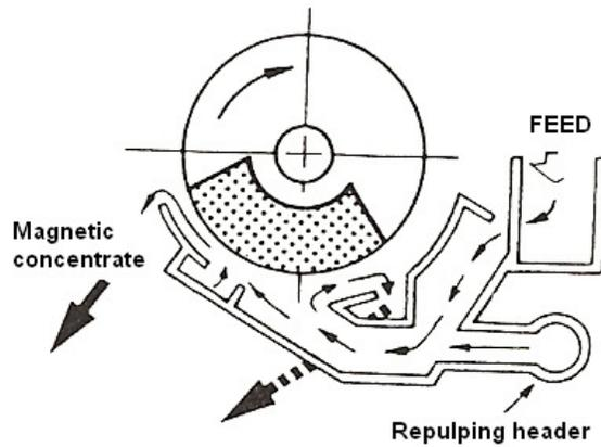
Figure 2.16 Counter-current magnetic separator (Svoboda, 1987)
