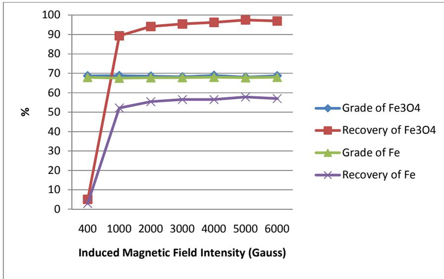
Figure 4.13 Results of the magnetic concentration test for -106 micron material (App. B, Table B.5)
