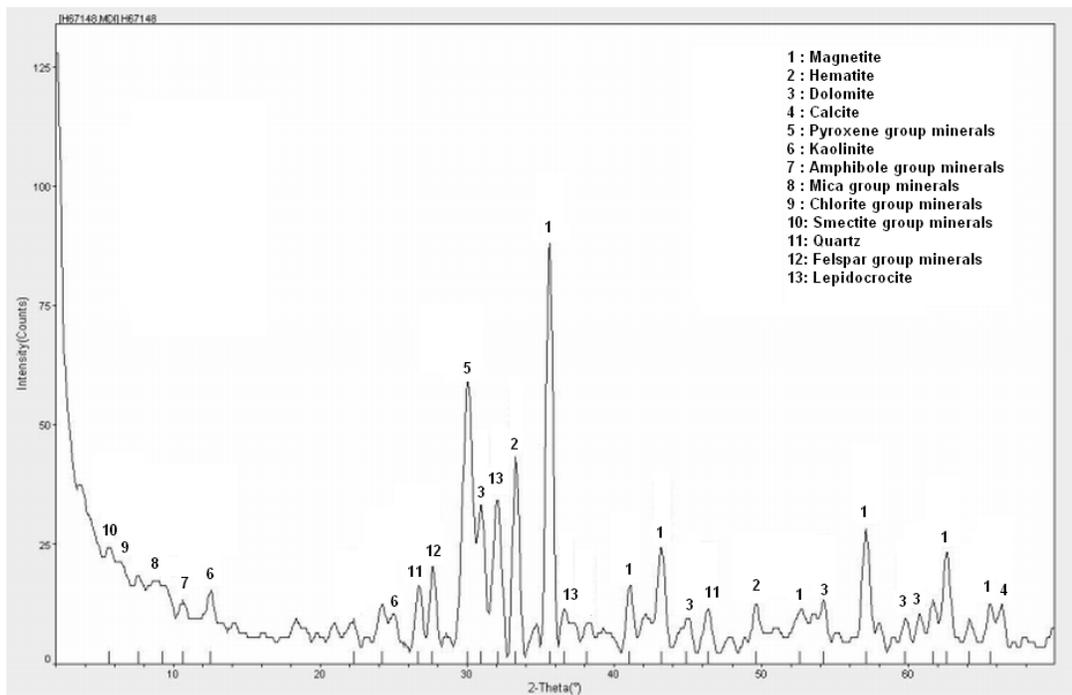
Figure 3.10 XRD pattern of high grade tailing
