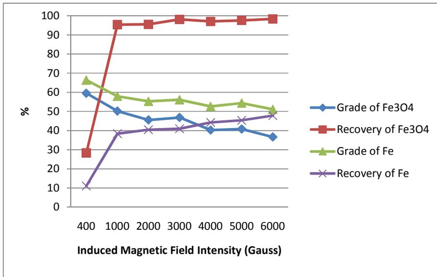
Figure 4.3 Results of the magnetic concentration test for -500 micron material (App. A, Table A.3)
