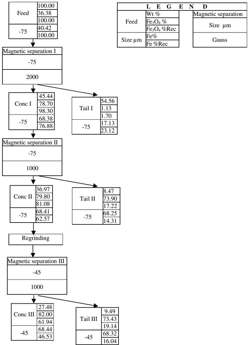
Figure 4.26 Flowsheet followed during the cleaning of magnetite preconcentrate
