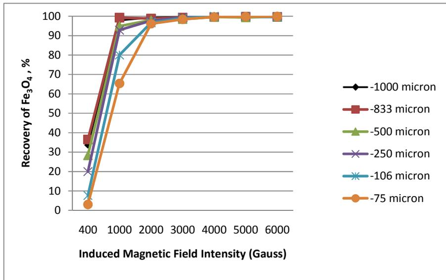
Figure 4.23 Recovery of Fe<sub>3</sub>O<sub>4</sub>% versus magnetic field intensity for high grade tailing
