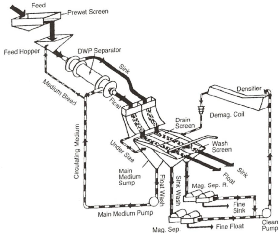
Figure 2.11 HMS circuit with regeneration unit (Wills, 1985)
