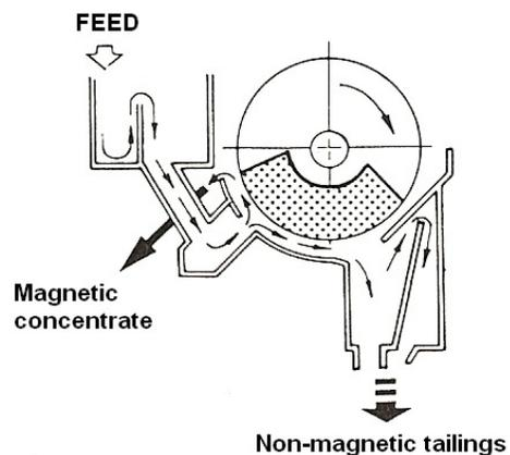
Figure 2.15 Counter-rotation magnetic separator (Svoboda, 1987)
