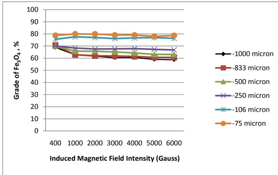
Figure 4.24 Grade of  $\text{Fe}_3\text{O}_4\%$  versus magnetic field intensity for high grade tailing
