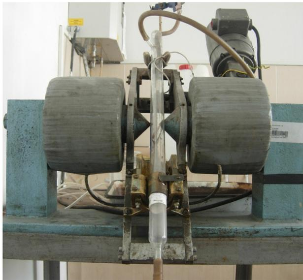
Figure 3.13 Laboratory type Davis tube magnetic concentrator
