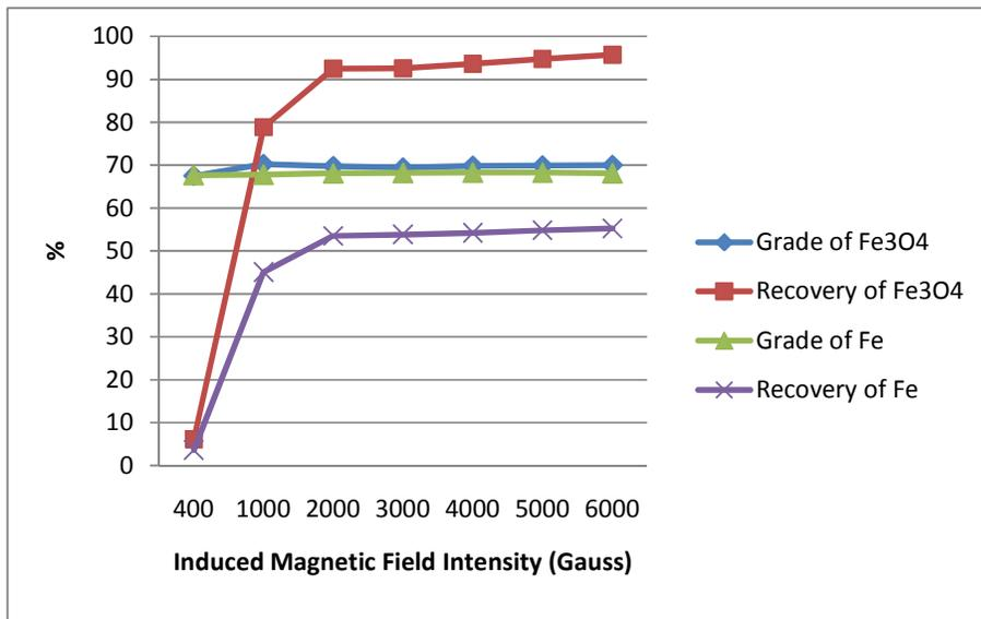
Figure 4.14 Results of the magnetic concentration test for -75 micron material (App. B, Table B.6)
