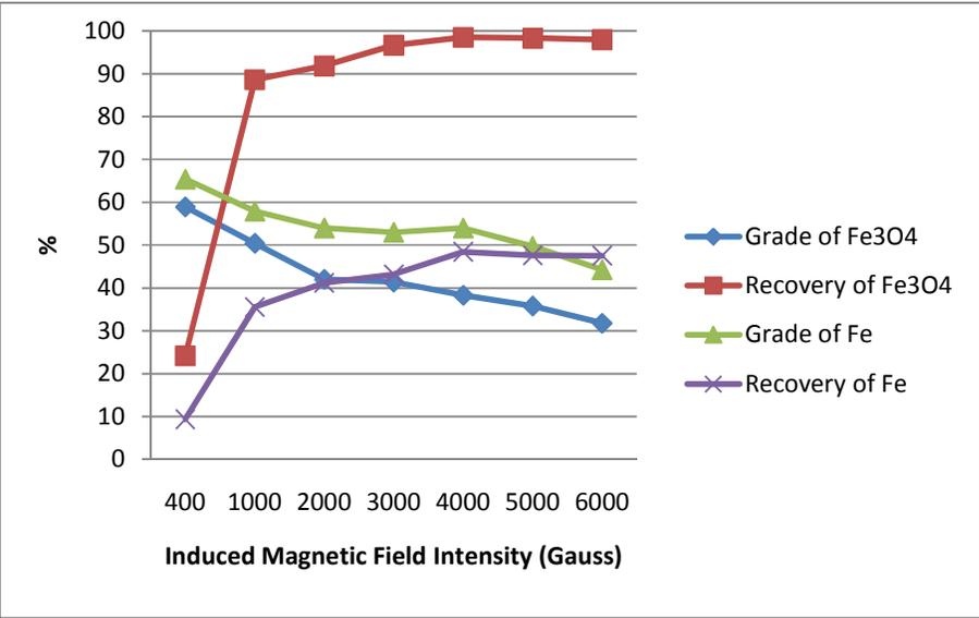
Figure 4.1 Results of the magnetic concentration test for -1000 micron material (App. A, Table A.1)
