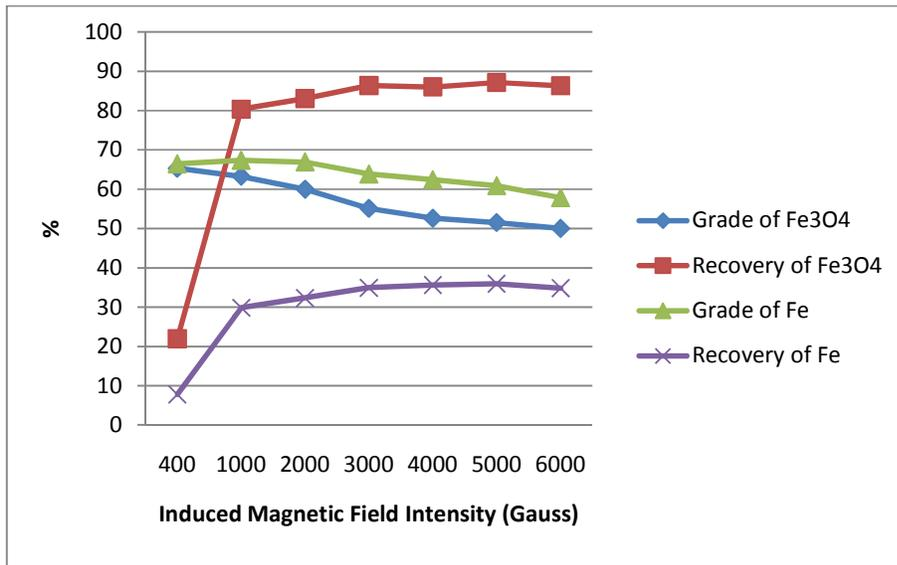
Figure 4.6 Results of the magnetic concentration test for -75 micron material (App. A, Table A.6)
