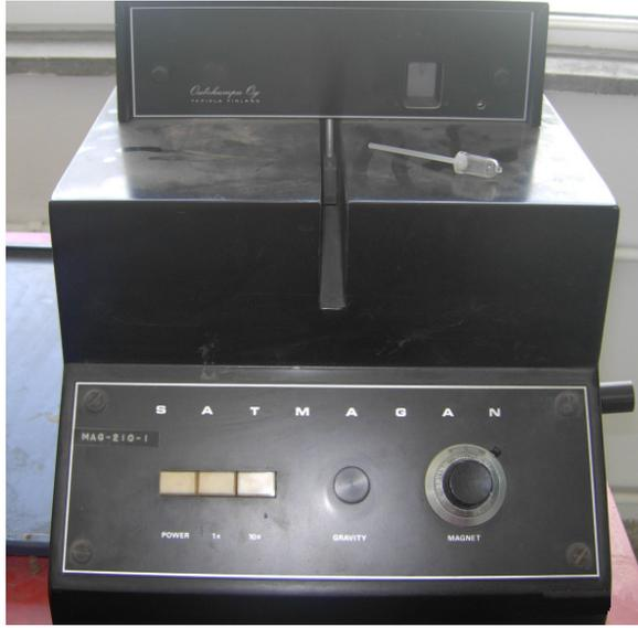
Figure 3.1 Satmagan (saturation magnetic analyzer)
