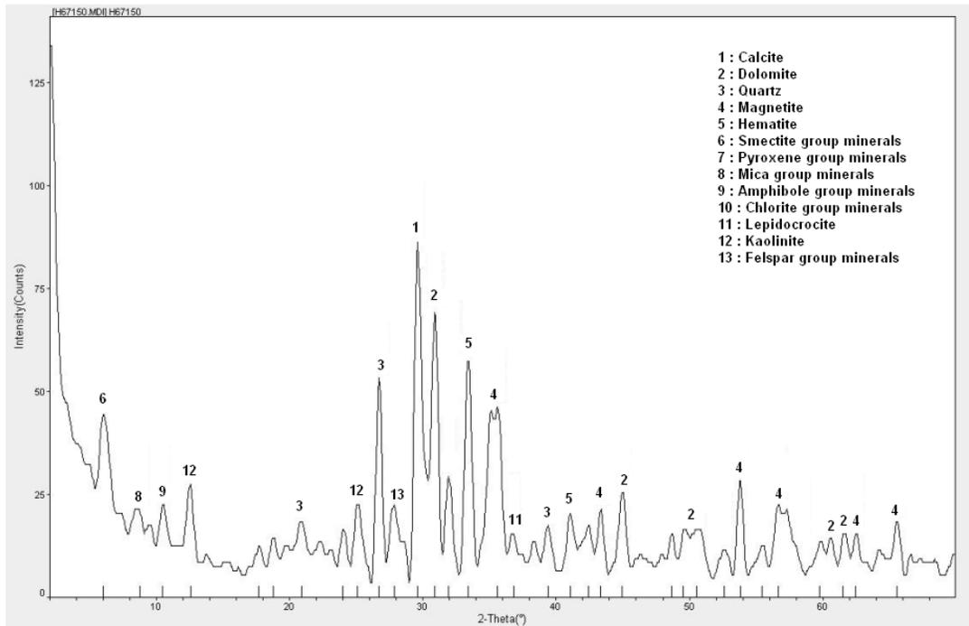
Figure 3.12 XRD pattern of low grade tailing
