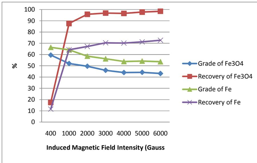
Figure 4.10 Results of the magnetic concentration test for -833 micron material (App. B, Table B.2)
