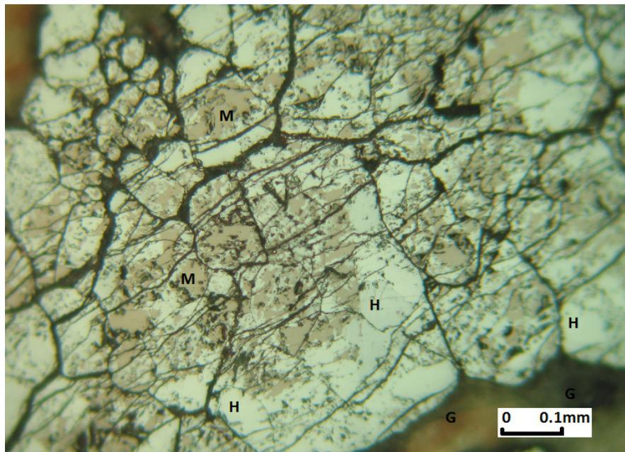
Figure 3.7 Magnetite (**M**) has cataclastic texture. Interlocked magnetite crystals
