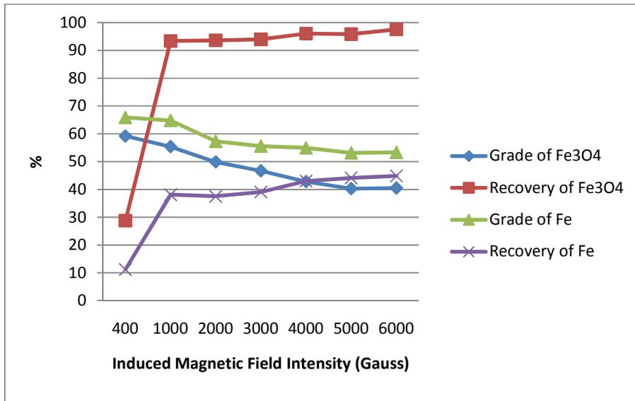
Figure 4.4 Results of the magnetic concentration test for -250 micron material (App. A, Table A.4)
