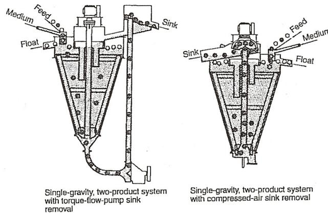
Figure 2.3 Cone separator
