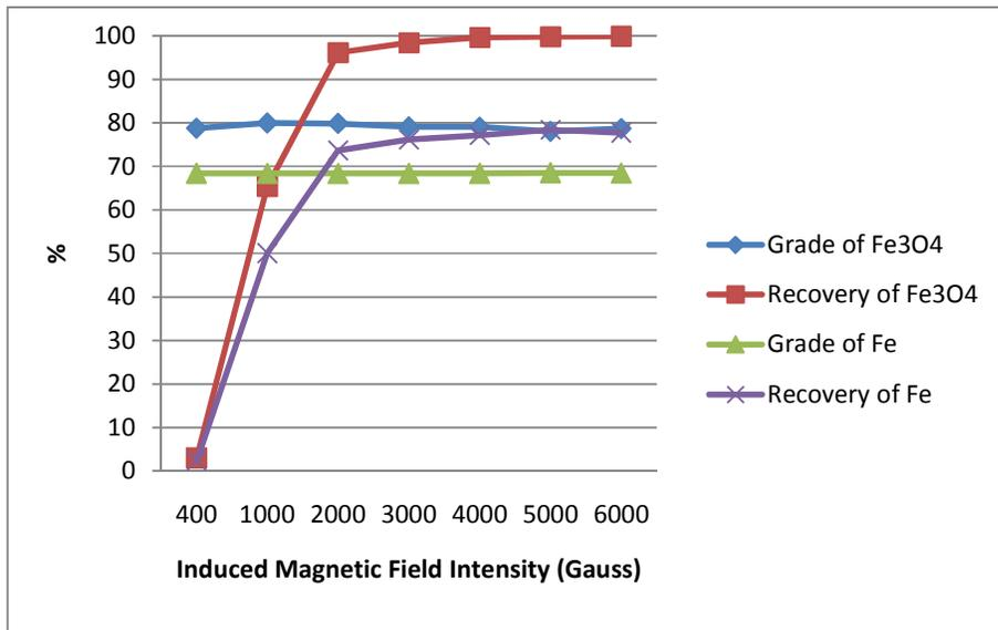
Figure 4.22 Results of the magnetic concentration test for -75 micron material (App. C, Table C.6)
