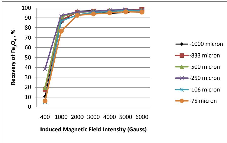
Figure 4.15 Recovery of Fe<sub>3</sub>O<sub>4</sub>% versus magnetic field intensity for medium grade tailing
