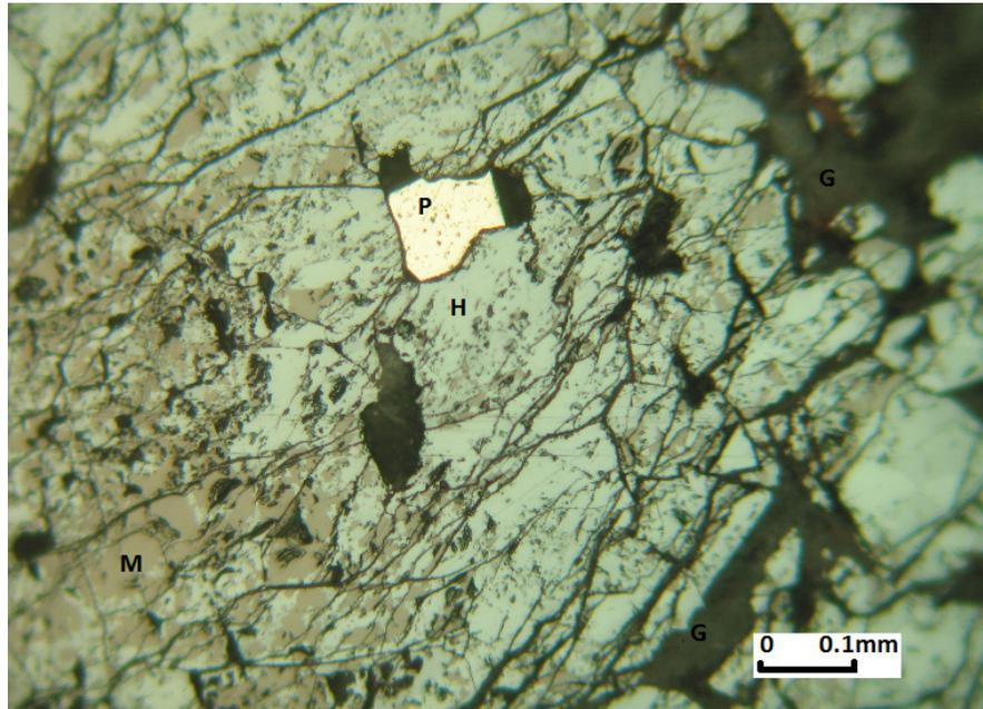
Figure 3.8 Pyrite (**P**) is observed in the fracture of martitized magnetite (**H**)
