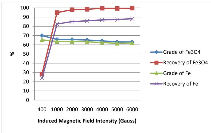
Figure 4.19 Results of the magnetic concentration test for -500 micron material (App. C, Table C.3)
