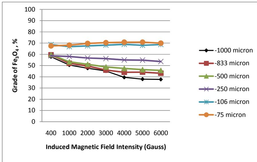
Figure 4.16 Grade of Fe<sub>3</sub>O<sub>4</sub>% versus magnetic field intensity for medium grade tailing
