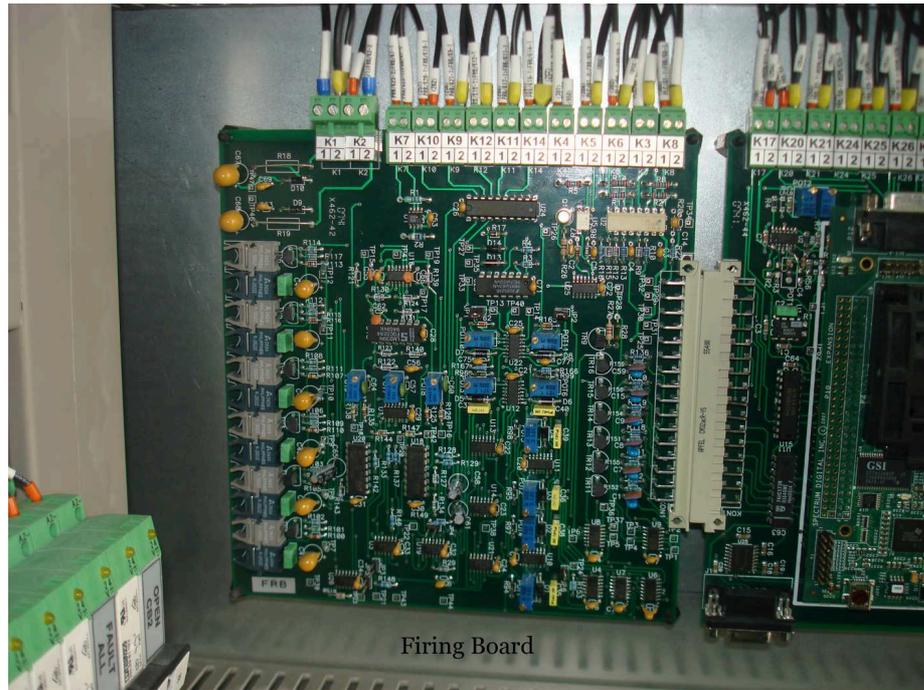
Figure 4.45: Firing Circuit Board
