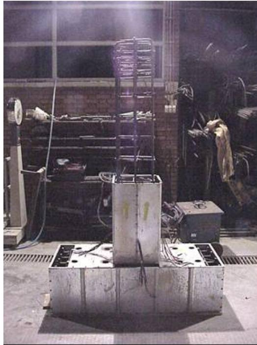
Figure 3.3 Metal formwork of footing and column before casting
