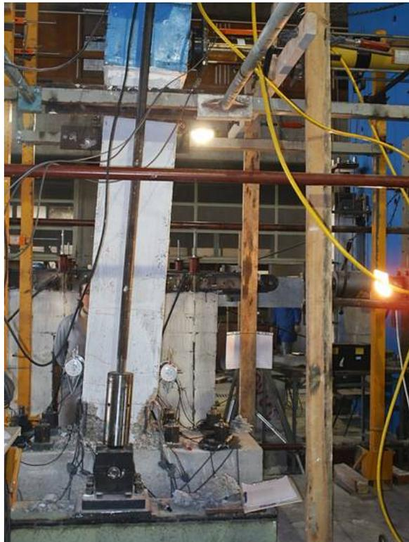
Figure 4.25 North face of Specimen 6PV1 at the last stage of loading
