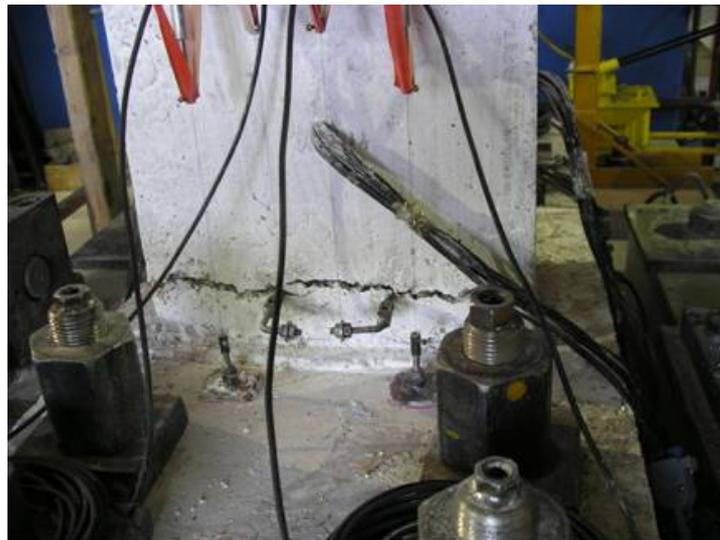
Figure 4.29 Crack opening at the East face of Specimen 7P3\_U
