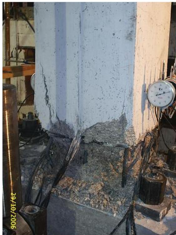
Figure 4.13 View of the specimen at the end of test, North-West faces of Specimen 3P3\_N0.4
