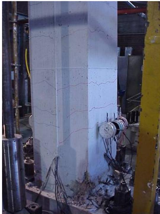
Figure 4.41 Crushing and spalling of concrete at the corners of the South-East face of Specimen 3D4
