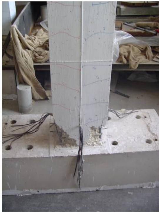
Figure 4.45 North face of Specimen 4D5 at the end of test
