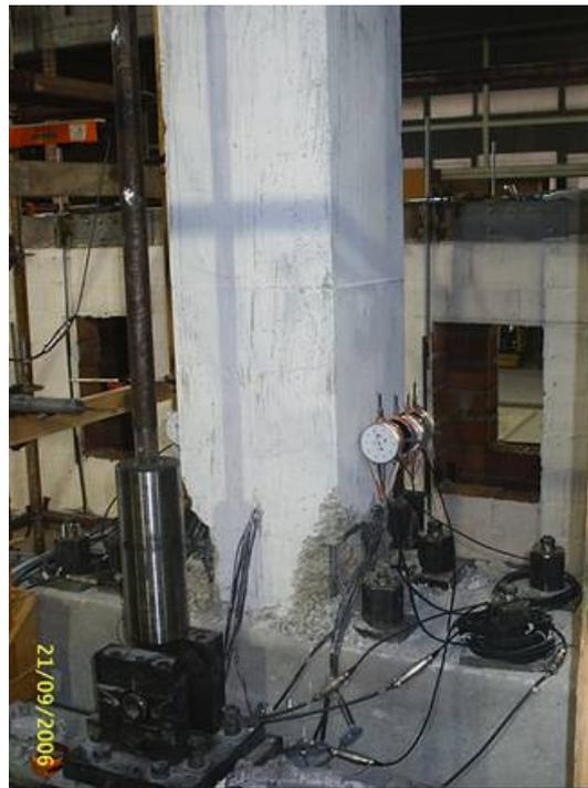
Figure 4.9 Buckling of longitudinal bars, North-West faces of Specimen 2P3
