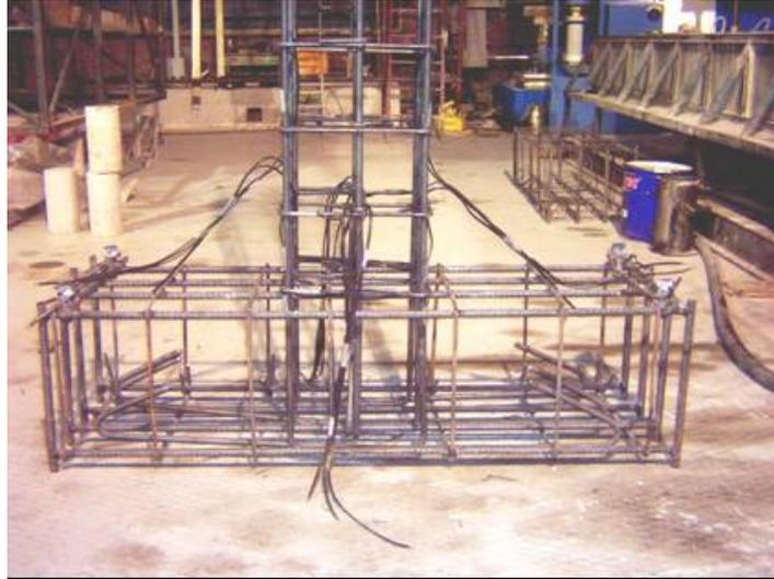
Figure 3.4 Reinforcing cage of a typical Type-1 specimen
