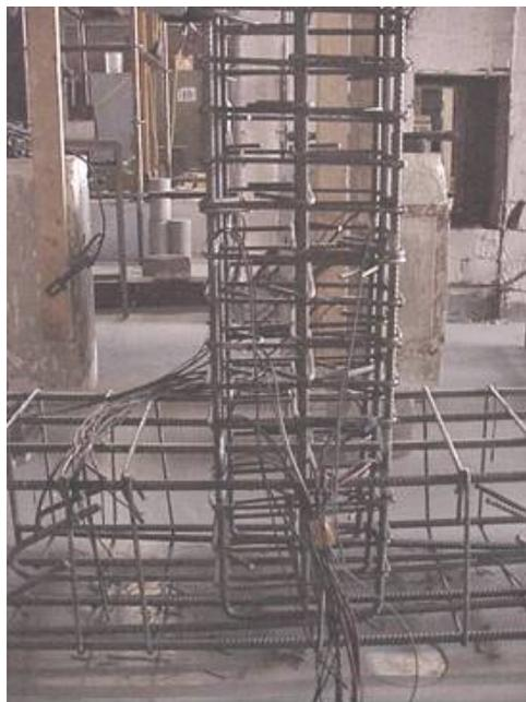
Figure 3.5 Reinforcing cage of a typical Type-2 specimen
