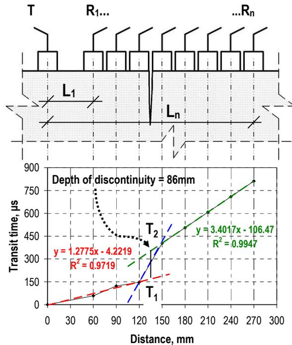
Figure 3.6 Schematic drawing of UPV measurements in indirect transmission mode showing the location of Transmitter, Receiver and the distance between those probes travelled by the ultrasonic wave, L, (at the top); the linear fitting of transit time readings as a function of distance between the centers of transducers (at the bottom).
