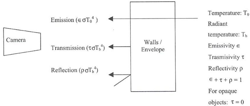
Figure 2.1 Emission, transmission and reflection are the components of radiation detected by infrared camera (Ocana, *et al.*, 2004: 516)
