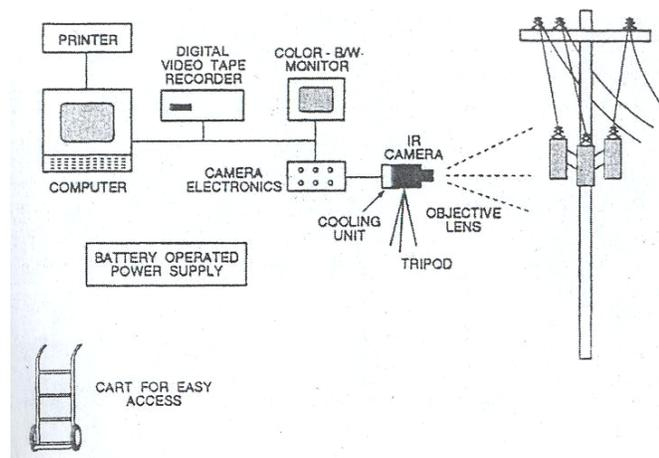
Figure 2.3 Schematic view of experimental setup for passive thermography; infrared camera recorded the IR images as a result of thermal gradient between the examined object and environmental condition (Maldague, 2001: 267)
