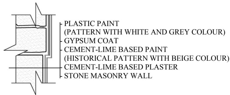
Figure 2.11 Geometric description of wall section showing the order of layers for the arch above the first layer window (Kökdemir and Dirican, 2008: 12)
