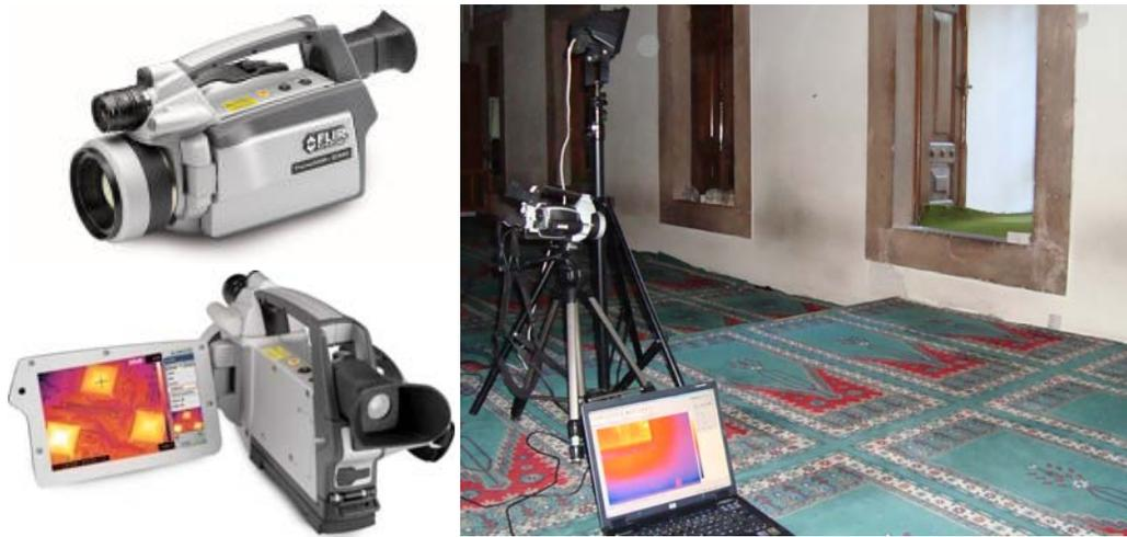
Figure A.1 Views of FLIR ThermaCAM SC640 Infrared Camera from different angles ([www.flir.com.hk](http://www.flir.com.hk) and [www.grimas.hu](http://www.grimas.hu)) (at the left) and experimental set-up for IR imaging controlled by laptop (at the right)
