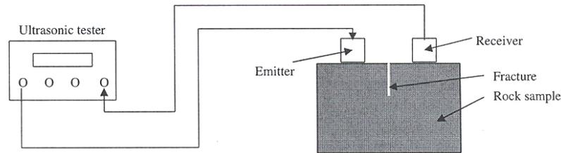
Figure 2.6 Schematic view of pulse velocity measurement by using indirect method for the crack depth estimation (Kahraman, *et al.*, 2008: 13)
