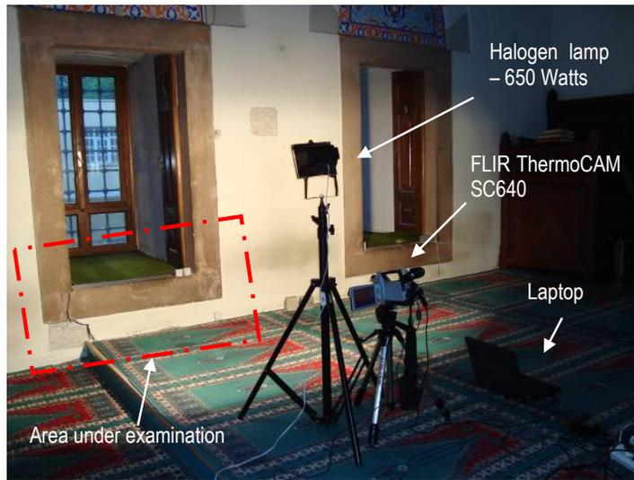
Figure 3.5 The experimental setup used for the sequential IR imaging of wall surfaces under the exposure of heating by halogen lamp: automatically-recording the IR images of target area at 2s intervals with the IR camera controlled by the laptop.
