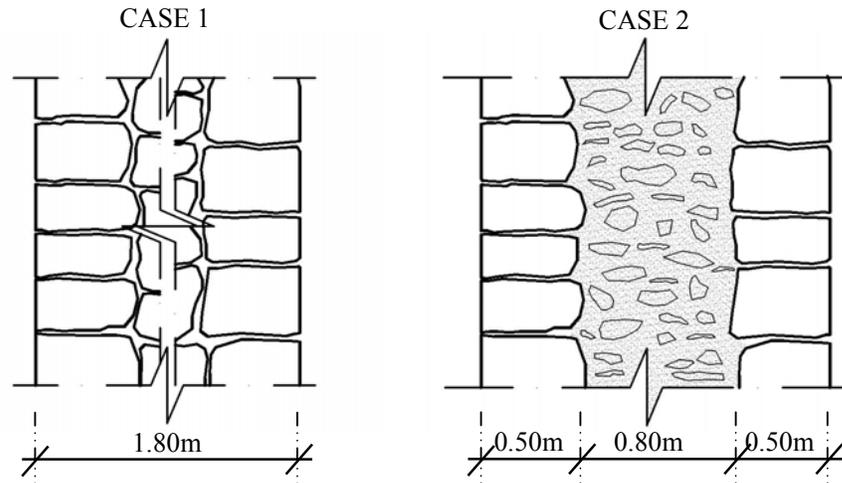
Figure C.1 Geometric description of masonry wall sections ASSUMED for the calculation of overall thermal transmittance,  $U$  value and overall thermal resistance,  $R$  value showing the order and thickness of layers for the Case 1 (at the left) and for the Case 2 (at the right).
