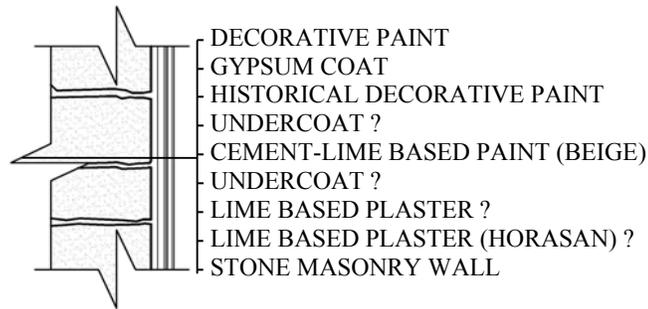
Figure 2.10 Geometric description of wall section showing the order of layers for the decoratively-painted part above the first layer window (Kökdemir and Dirican, 2008: 12)
