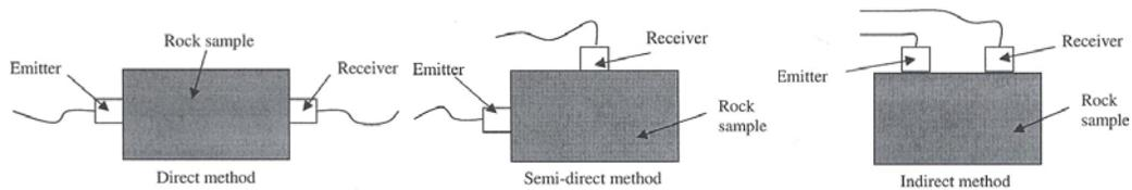
Figure 2.4 Schematic views direct, semi-direct and indirect methods of ultrasonic measurements (Kahraman, *et al.*, 2008: 12)
