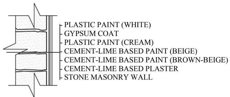
Figure 2.9 Geometric description of wall section showing the order of layers for plastic painted part (Kökdemir and Dirican, 2008: 11)
