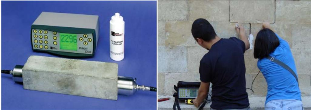
Figure A.3 View of PUNDIT PLUS PC1006 CNS FARNELL ([www.proceq.com](http://www.proceq.com)) (at the left) and experimental set-up of ultrasonic testing in indirect transmission mode (at the right).
