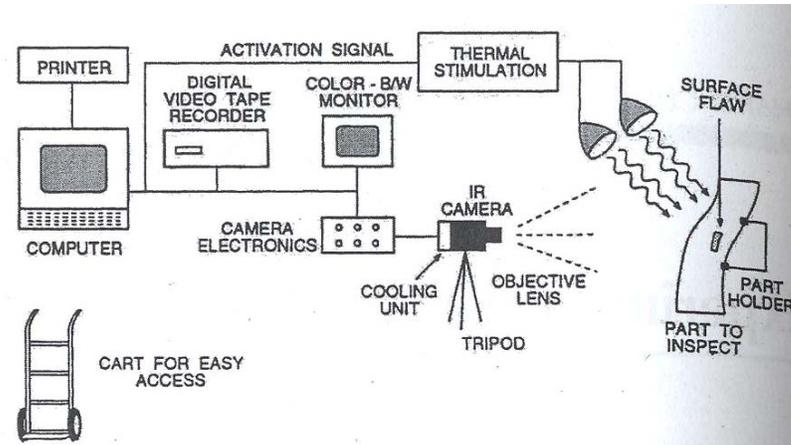
Figure 2.2 Schematic view of experimental setup for active thermography; examined surface is heated while infrared camera recording image and IR images are controlled from the computer (Maldague, 2001: 266)
