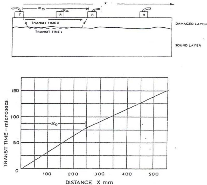
Figure 2.5 Schematic diagram of indirect measurement method (at the top) showing the depth of damaged layer and transit time versus distance graph of the same case (at the bottom) showing the difference on slope as a result of damage (Christaras, 1999: 134)
