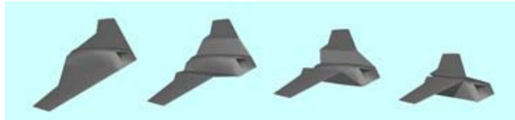
Figure 2.2.6: Folding Wing Concept (Image: Lockheed Martin)
