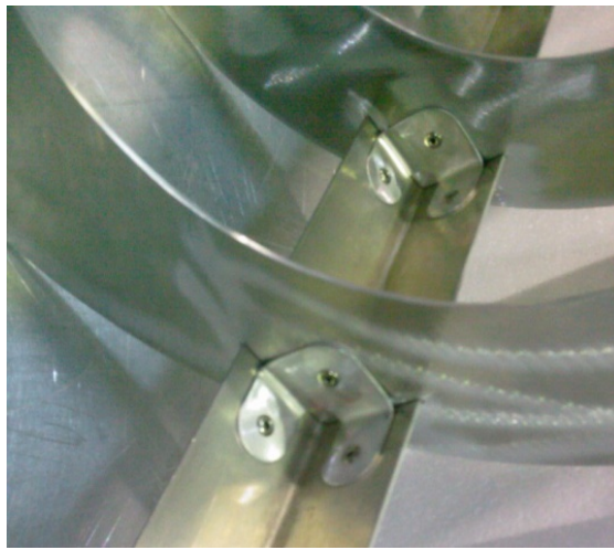
Figure 6.8.1: Fittings, Longeron and Frame Connection View 1
