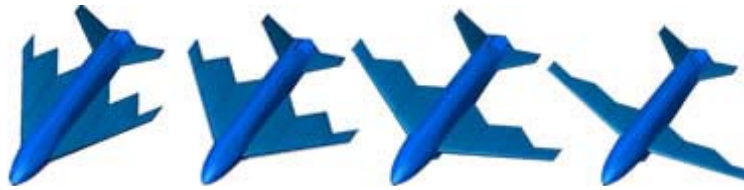
Figure 2.2.5: Sliding Skins Concept (Image: NexGen)
