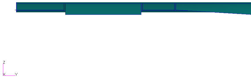
Figure 4.4.10: View from Trailing Edge of the Model of the Wing with Twisted Outer Control Surface
