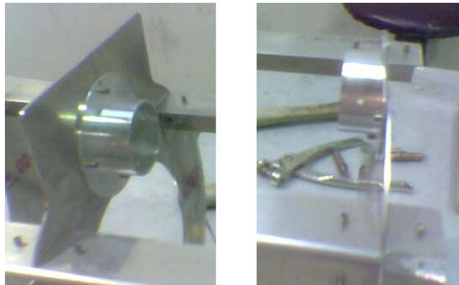
Figure 6.8.7: Fitting and Frame Connection for the fourth (left) and the fifth Frame (right)
