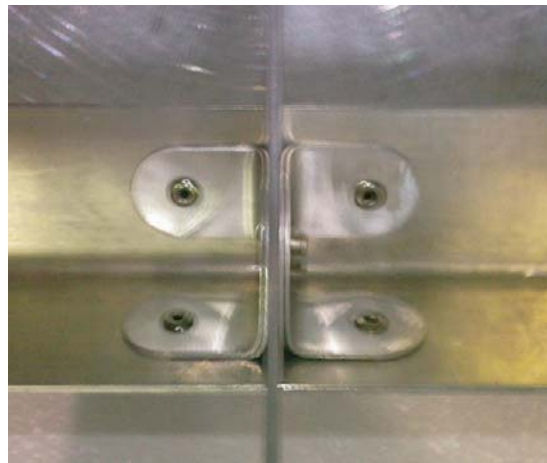
Figure 6.8.2: Fittings, Longeron and Frame View 2
