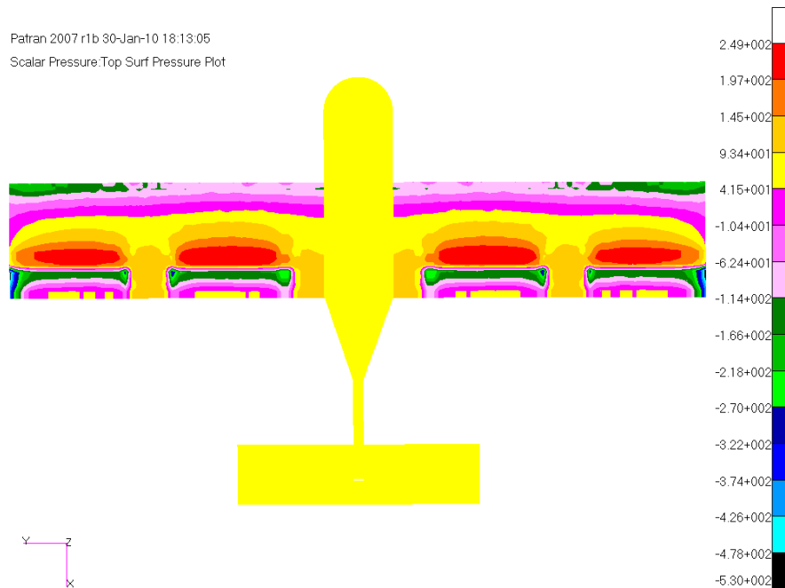
Figure 6.6.1: Pressure Boundary Condition (Bottom View)
