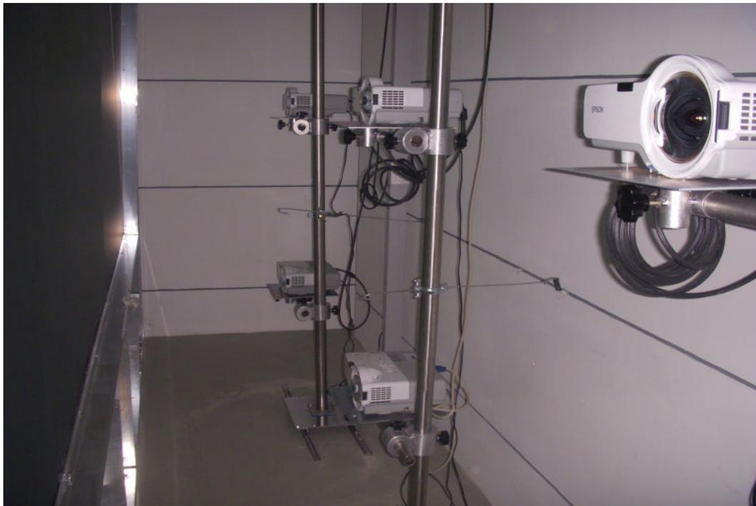
Figure 52 Back-projection large-screen display comprised of six back-projectors and seamless plexiglas wall.
