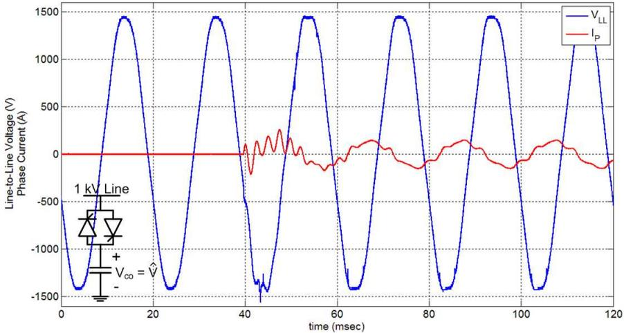
Figure 4.14: Resultant line-to-line voltage and phase current of the turn-on transient with thyristor when the capacitors are initially charged.
