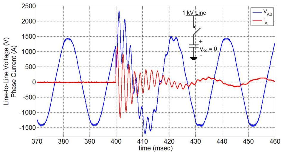
Figure 4.4: Resultant line-to-line voltage and phase current of the turn-on transient with contactor when the capacitors are initially discharged.
