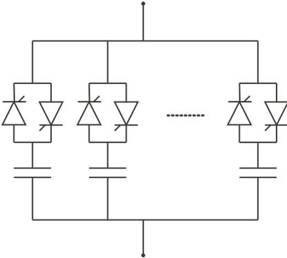
Figure 2.2: Representation of an ideal TSC branch. Each phase may include more than one thyristor/capacitor combination to increase the reactive power variation. The number of branches depends on the reactive power required.
