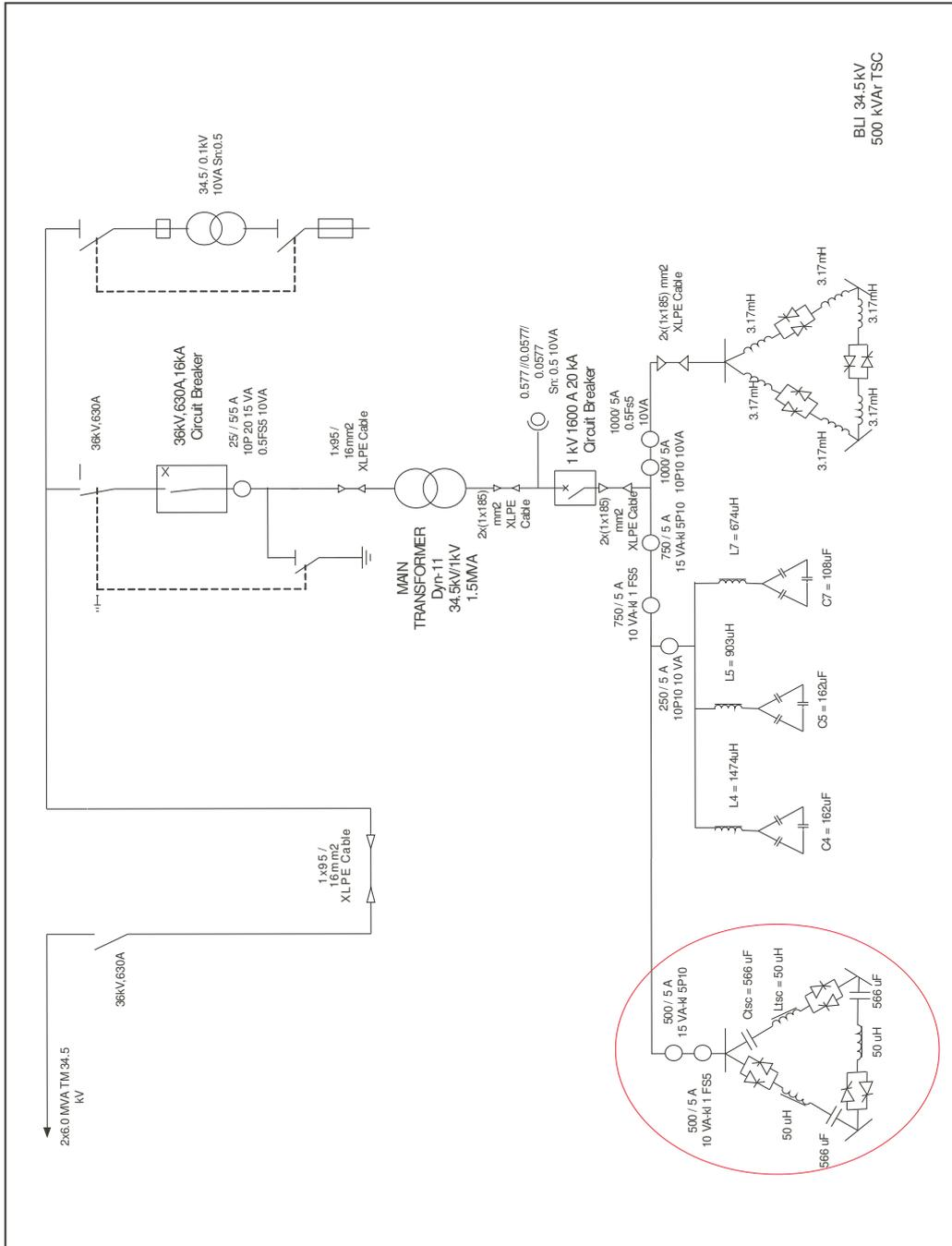
Figure 4.27: Single Line Diagram of the electrical network installed in BLI.
