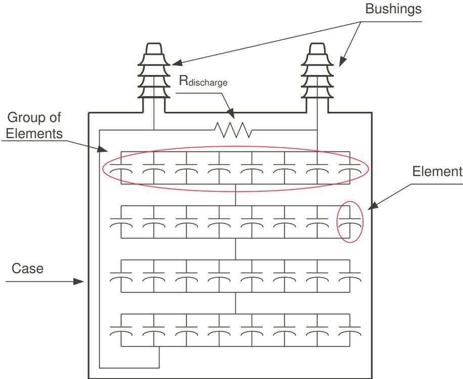
Figure 3.5: Capacitor internal structure.
