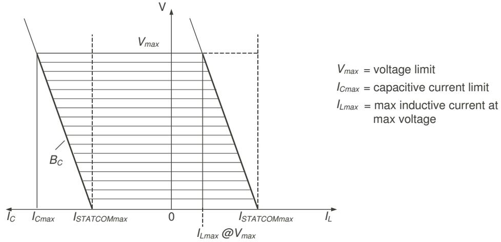
Figure 2.19: The  $V - I$  characteristics of TSC and STATCOM combination, [6]
