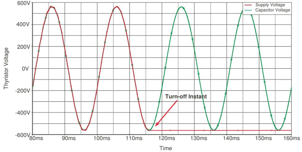
Figure 3.2: Voltage variation during switch-off process.
