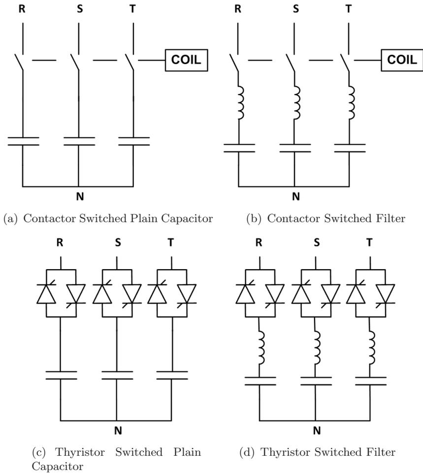
Figure 4.2: Circuit representations of four different switching scheme.
