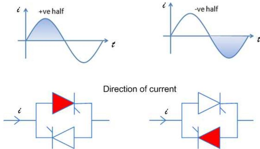
Figure 3.13: The current distribution of back-to-back connected thyristors in the steady state.
