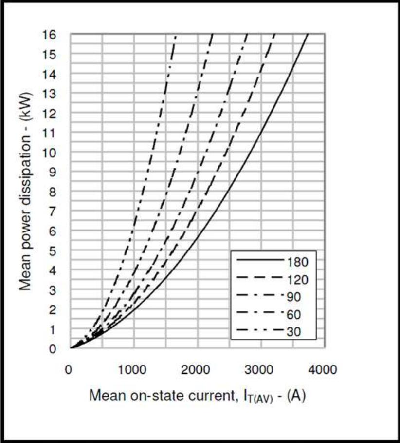
Figure B.1: On-state power dissipation curve of the thyristor.
