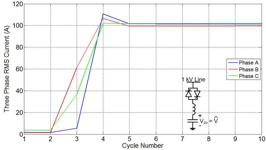
Figure 4.23: Resultant settling time of the turn-on transient with thyristor.
