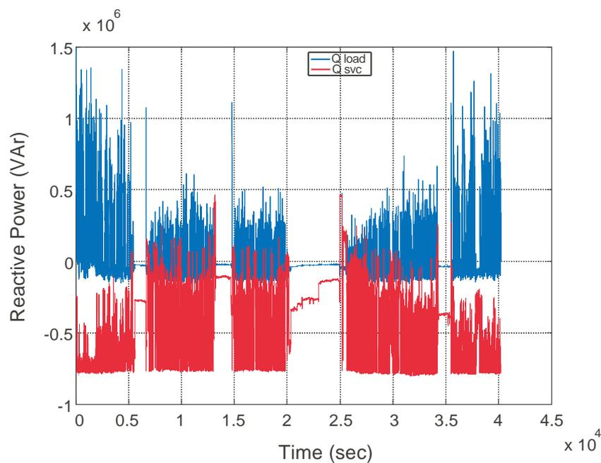
Figure 4.40: Reactive power compensation performance of TSC working in parallel to TCR.
