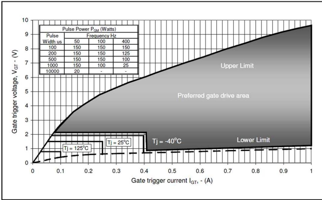
Figure B.3: Gate characteristics curve of the thyristor.
