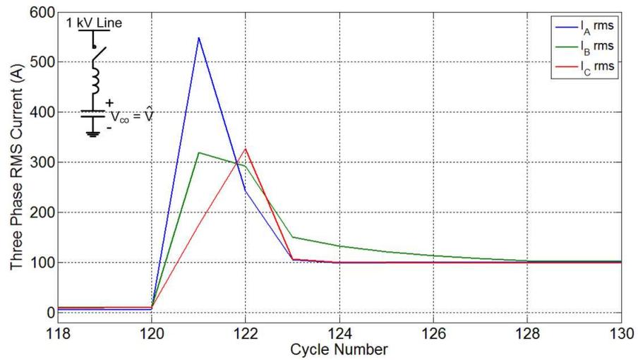
Figure 4.9: Resultant settling time of the turn-on transient with contactor.
