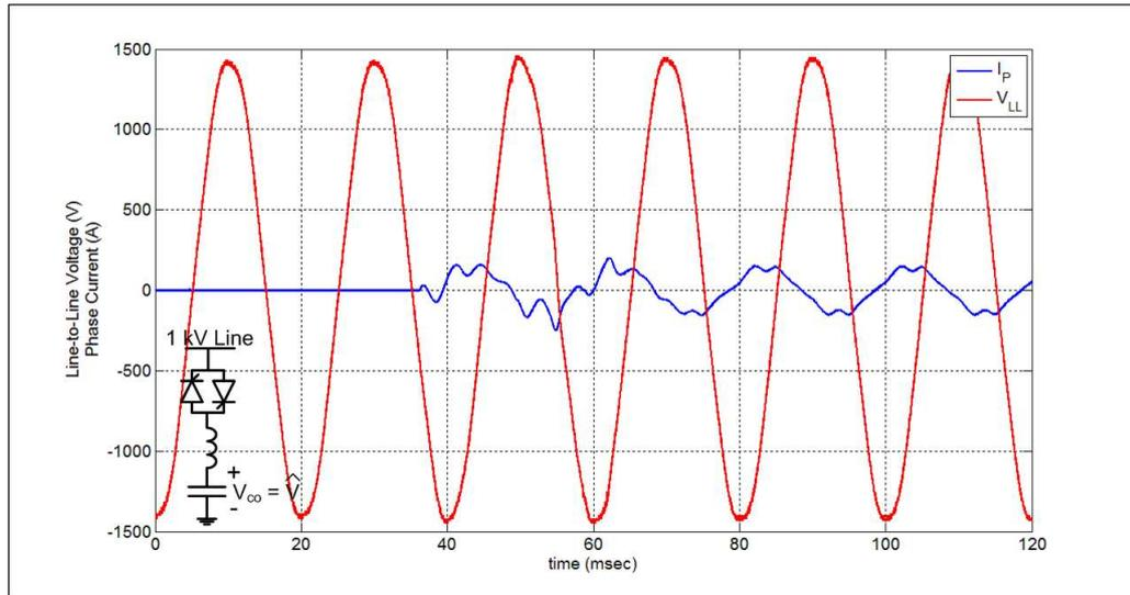
Figure 4.21: Resultant line-to-line voltage and phase current of the turn-on transient with thyristor when the capacitors are initially charged.
