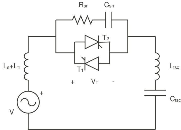
Figure 3.10: Equivalent circuit for snubber design for TSC.
