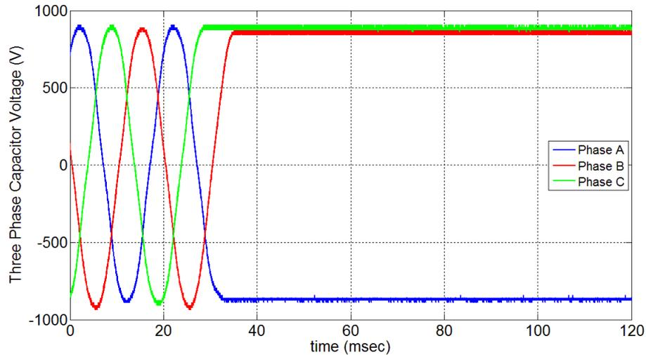
Figure 4.26: Resultant  $3\phi$  Capacitor Waveforms of the turn-off transient with thyristor.
