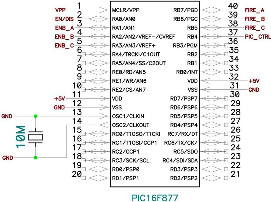
Figure 3.16: The connection scheme of the microcontroller, type PIC16F877.
