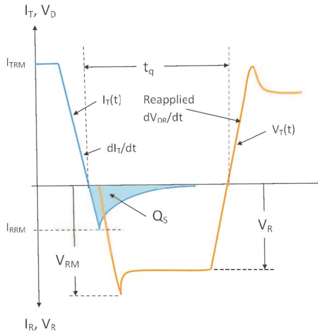
Figure 3.11: Thyristor turn-off waveforms, [43].
