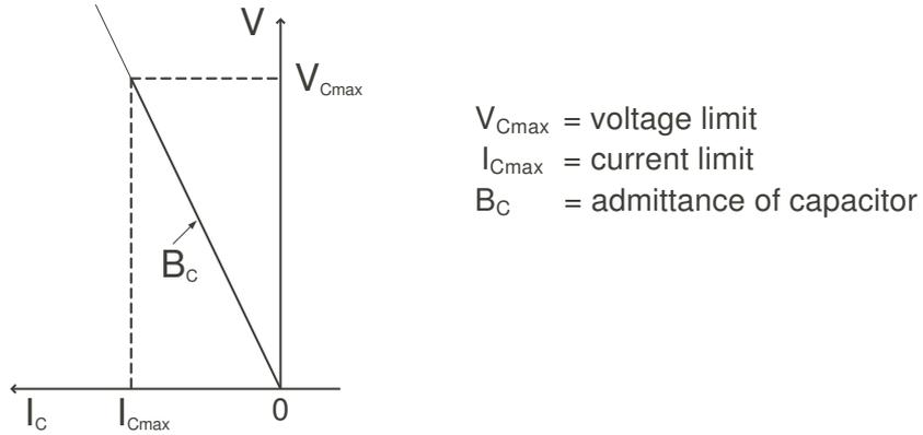
Figure 2.5: Operating  $V - I$  area of a single TSC [6].
