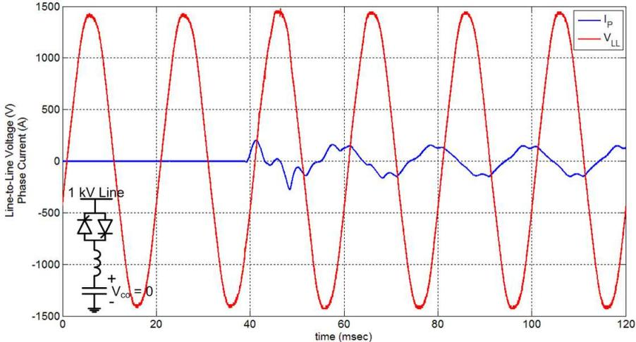
Figure 4.20: Resultant line-to-line voltage and phase current of the turn-on transient with thyristor when the capacitors are initially discharged.
