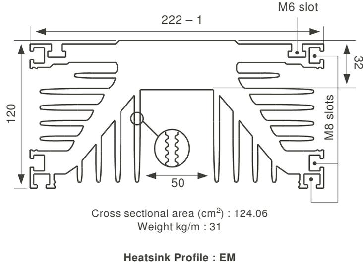
Figure 3.12: Heatsink profile for the reduction of junction temperature.
