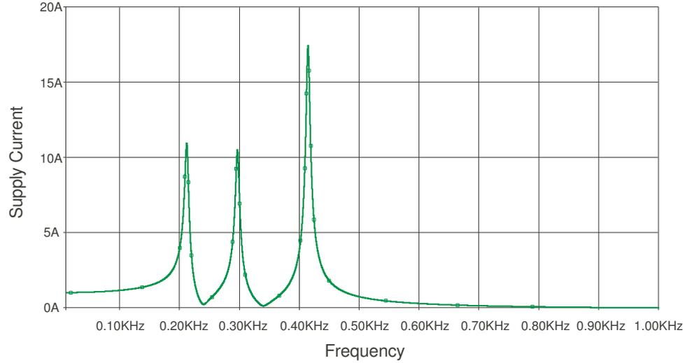
Figure 3.8: Frequency characteristics of TSC and the passive filter located in TKI, Orhaneli/Bursa. The passive filters are tuned to 5<sup>th</sup> (240 Hz) and 7<sup>th</sup> (340 Hz) harmonics.
