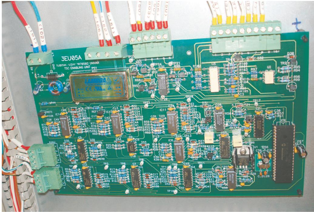
Figure 3.15: The view of EU control card designed for TSC.
