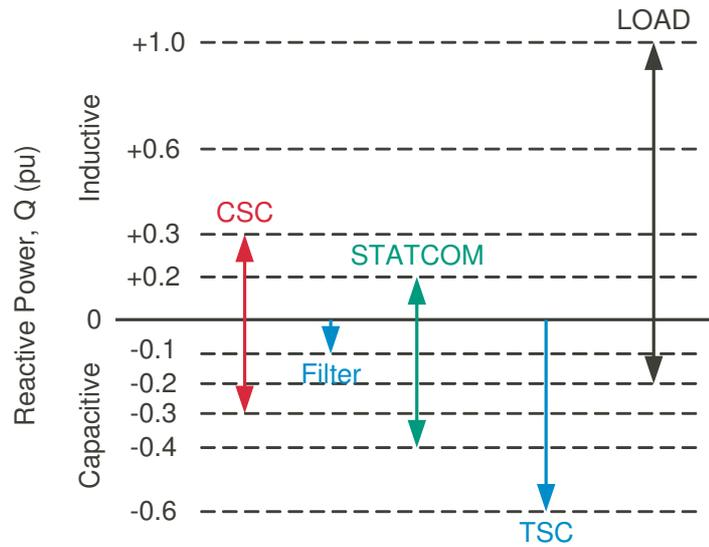
Figure 2.20: Power generation capability of TSC and CSC based STATCOM for optimum system performance.
