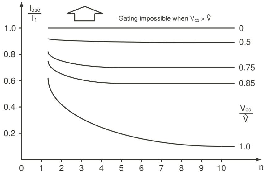
Figure 2.12: Amplitude of oscillatory current component - thyristors gated when  $v = V_{co}$ , [35].
