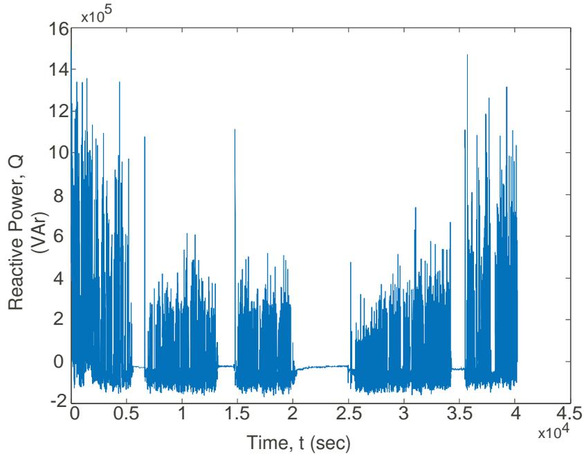
Figure 3.1: Load Characteristics of excavators in Orhaneli, Bursa.
