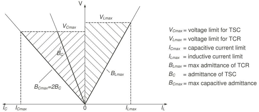
Figure 2.16: The  $V - I$  characteristics of TSC and TCR combination, [6]
