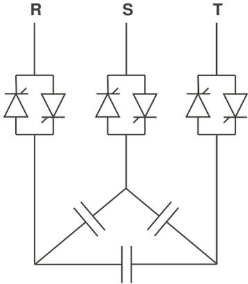
Figure 2.3: Alternative Arrangement of TSC: Delta Connected Capacitor Banks.
