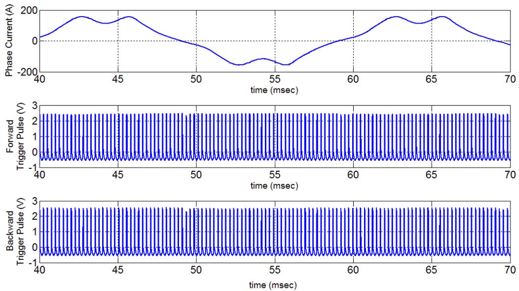
Figure 4.25: Firing pulses and current waveforms of a back-to-back connected thyristor pair during steady-state.
