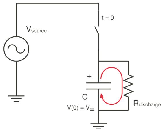
Figure 3.3: Discharge resistor connection diagram.
