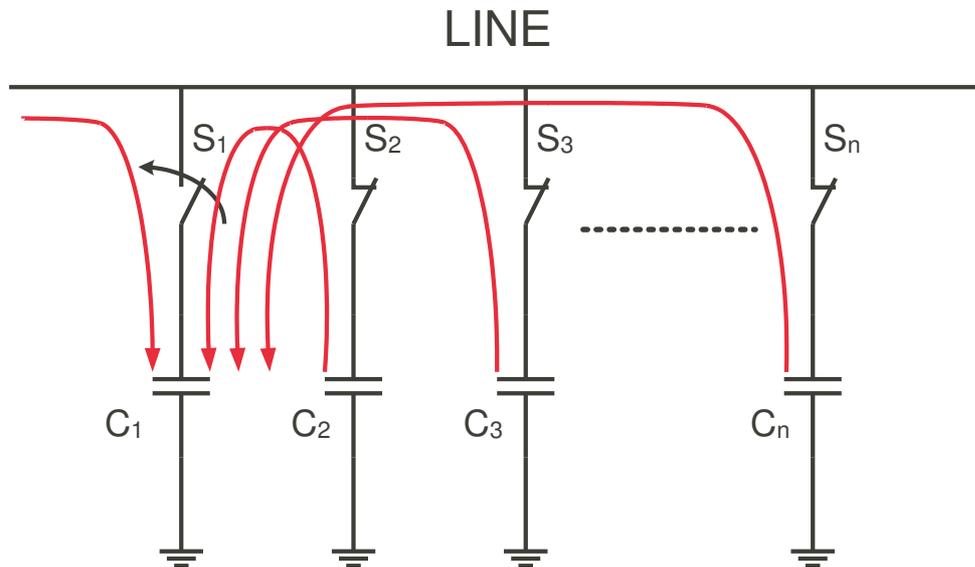
Figure 2.10: The illustration of inrush current paths drawn by the stage turned on lastly. The rest of the stages are already conducting and charged to the supply voltage.
