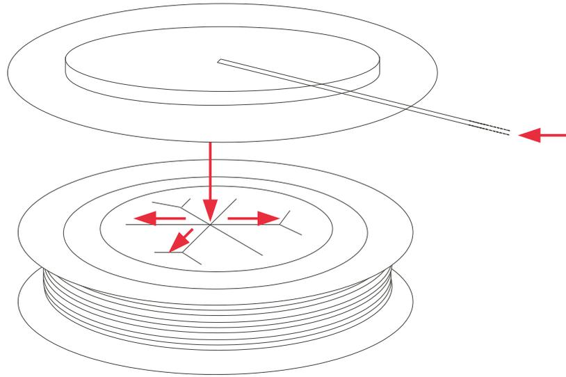
Figure 3.9: Thyristor gate triggering.
