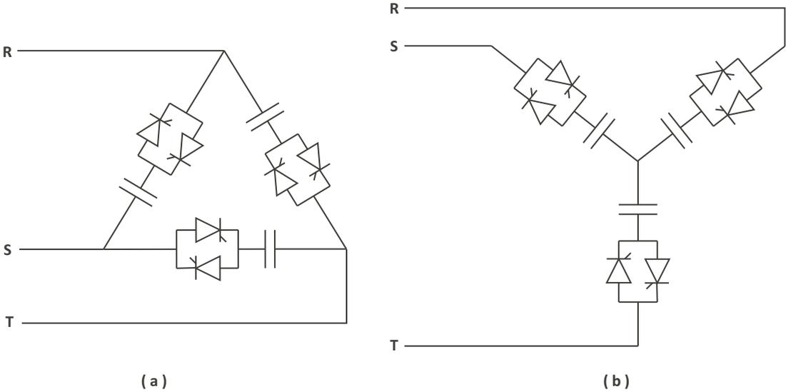
Figure 2.1: Various configuration of Thyristor Switched Capacitor Circuit (a) Delta Connection, (b) Wye Connection.
