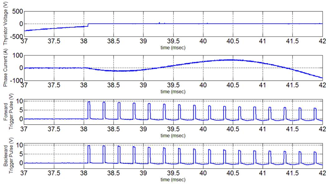
Figure 4.24: Firing pulses, voltage and current waveforms of a back-to-back connected thyristor pair at the instant of switching.
