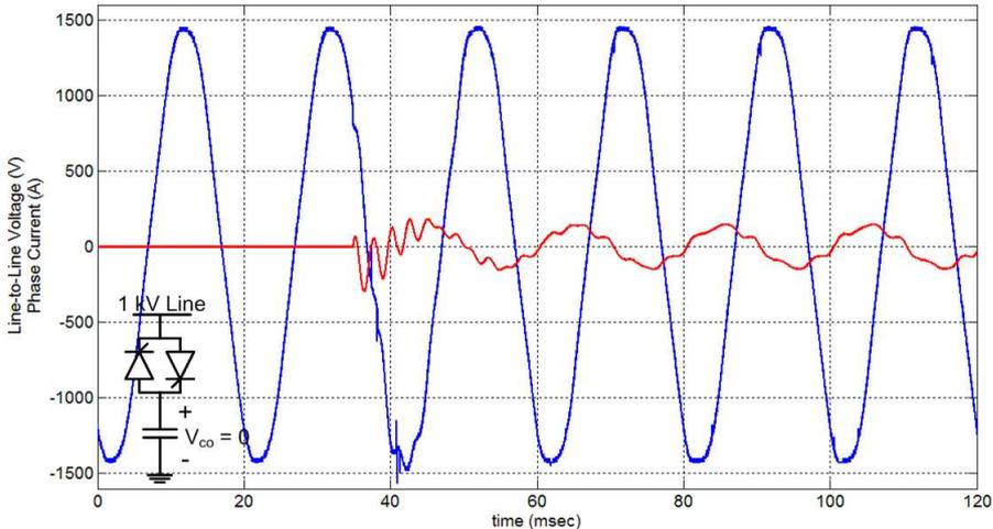
Figure 4.13: Resultant line-to-line voltage and phase current of the turn-on transient with thyristor when the capacitors are initially discharged.
