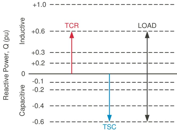
Figure 2.17: Power generation capability of TSC and TCR for optimum system performance.
