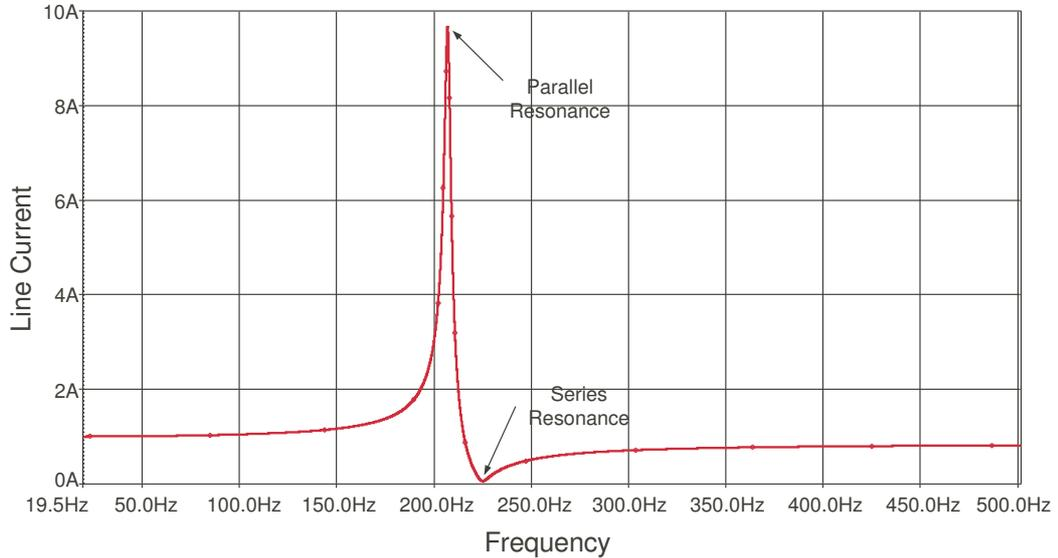
Figure 2.6: Frequency diagram of a  $3\phi$  power system consisting of 300 MVA power supply, 1 MVA 34.5/1 kV Transformer ( $U_k = 5.2\%$ ), 160 kVAr  $5^{th}$  harmonic filter. 1 A is injected to the system as a harmonic source on the load side.
