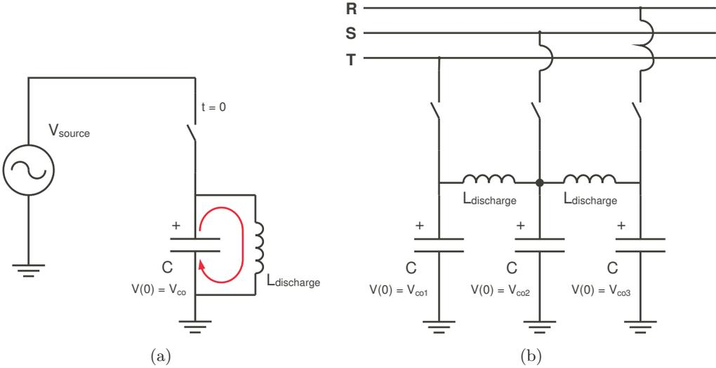
Figure 3.4: Discharge reactor connection diagram (a) parallel to each capacitor, (b) across two phases.
