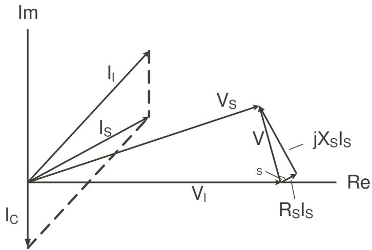
Figure 2.9: (a) Equivalent circuit representation of an electrical system and phasor diagrams (b) without compensator, (c) with compensator for zero voltage difference.
