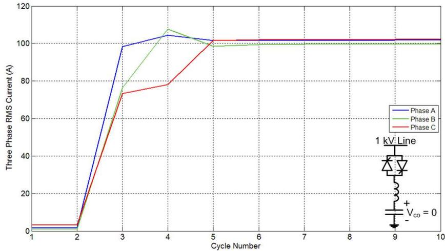
Figure 4.22: Resultant settling time of the turn-on transient with thyristor.
