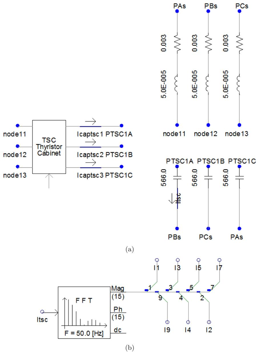
Figure 3.7: PSCAD model of the (a) TSC circuit, (b) harmonic extraction.
