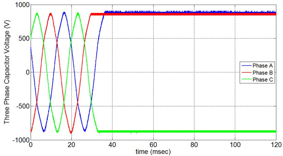
Figure 4.17: Resultant  $3\phi$  Capacitor Waveforms of the turn-off transient with thyristor.
