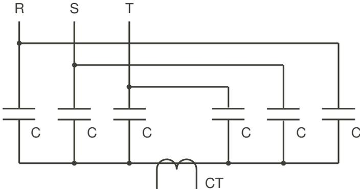
Figure 3.6: Double-star connection for unbalance protection.
