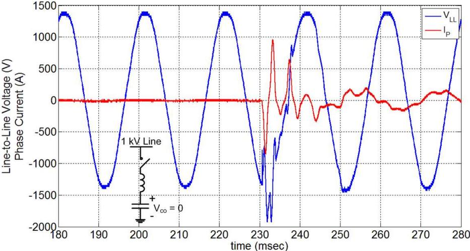
Figure 4.8: Resultant line-to-line voltage and phase current of the turn-on transient with contactor when the capacitors are initially discharged.
