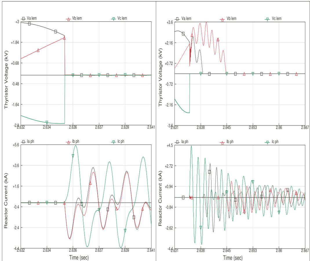
Figure 4.37: Current waveforms through the reactor during a misfire and their effects on the thyristor voltage.
