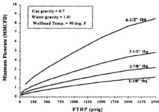
Figure 4.4 – Critical Flowrates for Different Tubing Sizes<sup>9</sup>
