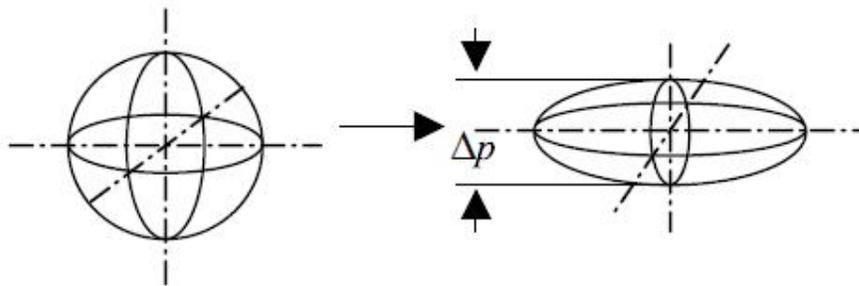
Figure 2.1 – Shape of entrained drop movement in high-velocity gas<sup>4</sup>
