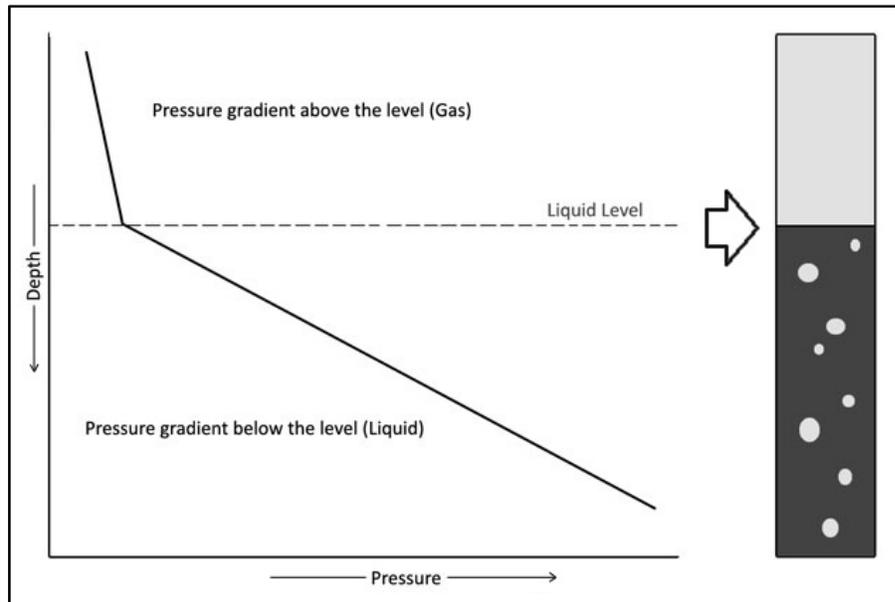
Figure 4.2 – A Typical Pressure Survey Graph
