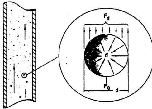
Figure 4.3 – Liquid Droplet Movement<sup>1</sup>
