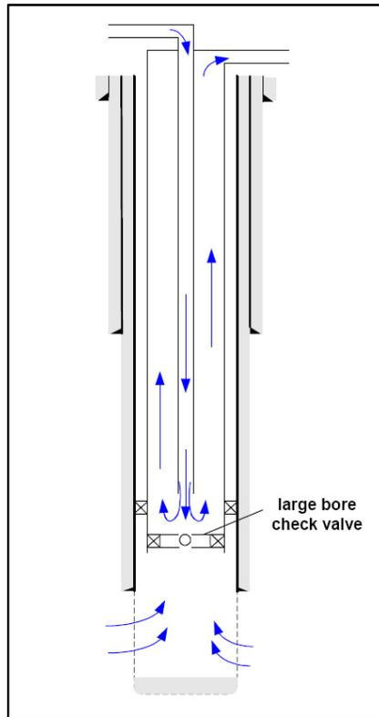
Figure 4.18 – Continuous Gas Lift Schematic<sup>14</sup>
