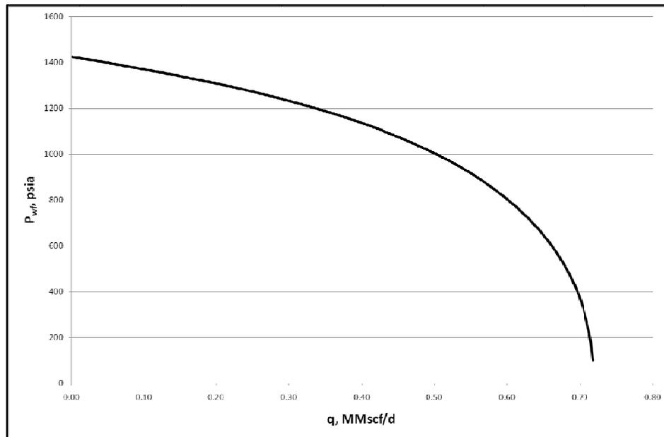
Figure C.2 – IPR curve of Well #28
