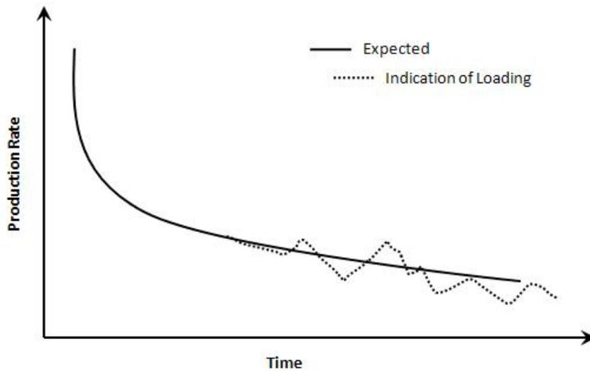
Figure 4.1 – A Typical Gas Well Decline Curve along with Indication of Loading
