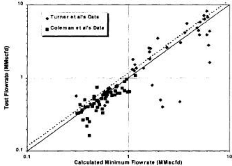
Figure 4.5 – Critical Gas Flowrates for Turner & Coleman<sup>9</sup>
