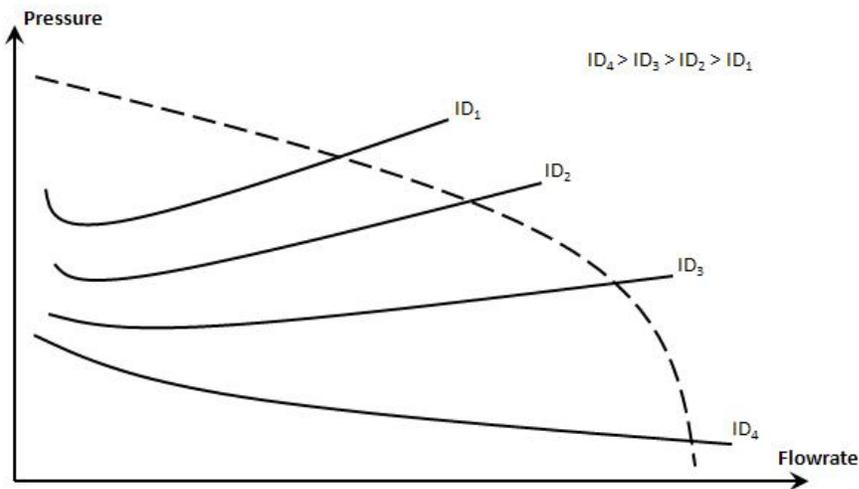
Figure 4.8 – Nodal Analysis Graph for Different Tubing Sizes<sup>10</sup>
