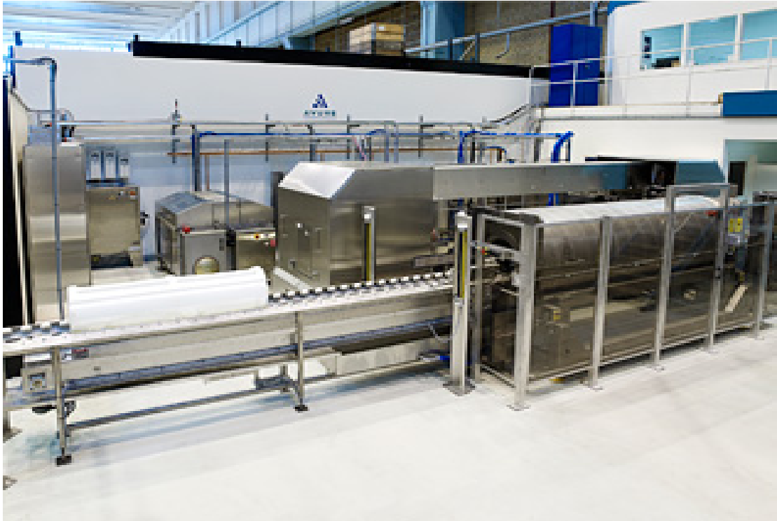
Figure 1.2 Industrial Scale HHP Equipment Which Runs for Batch Operations
