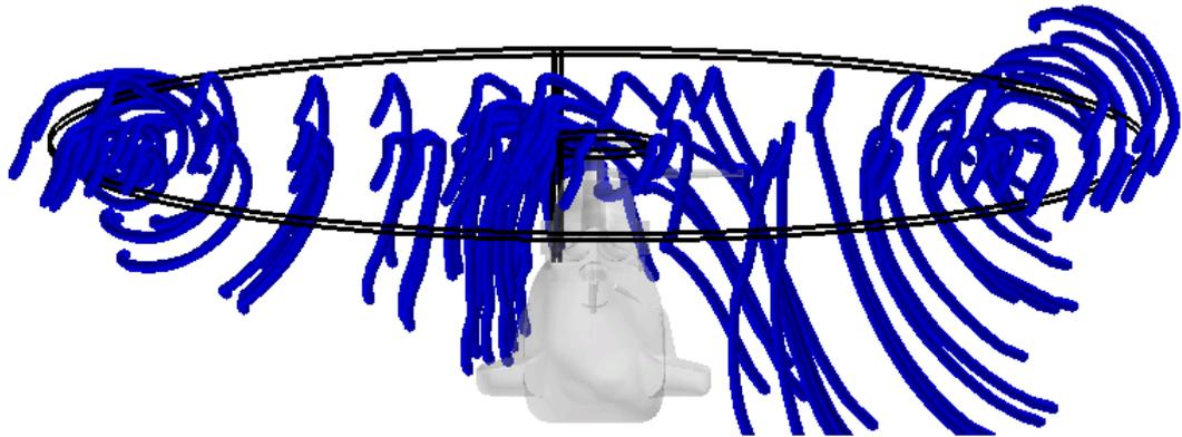
**Figure 88-Main rotor streamlines and tip effect, forward view**
