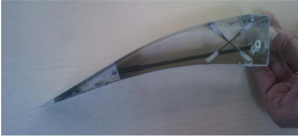
Figure 3.14: Hingeless Control Surface Prototype Camber Increase
