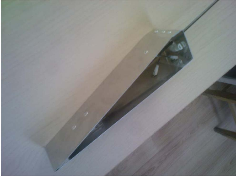
Figure 3.13: Hingeless Control Surface Prototype
