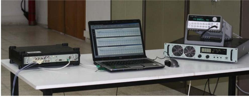
Figure 4.38: Analysis Equipment Used in the Experimental Modal Analysis
